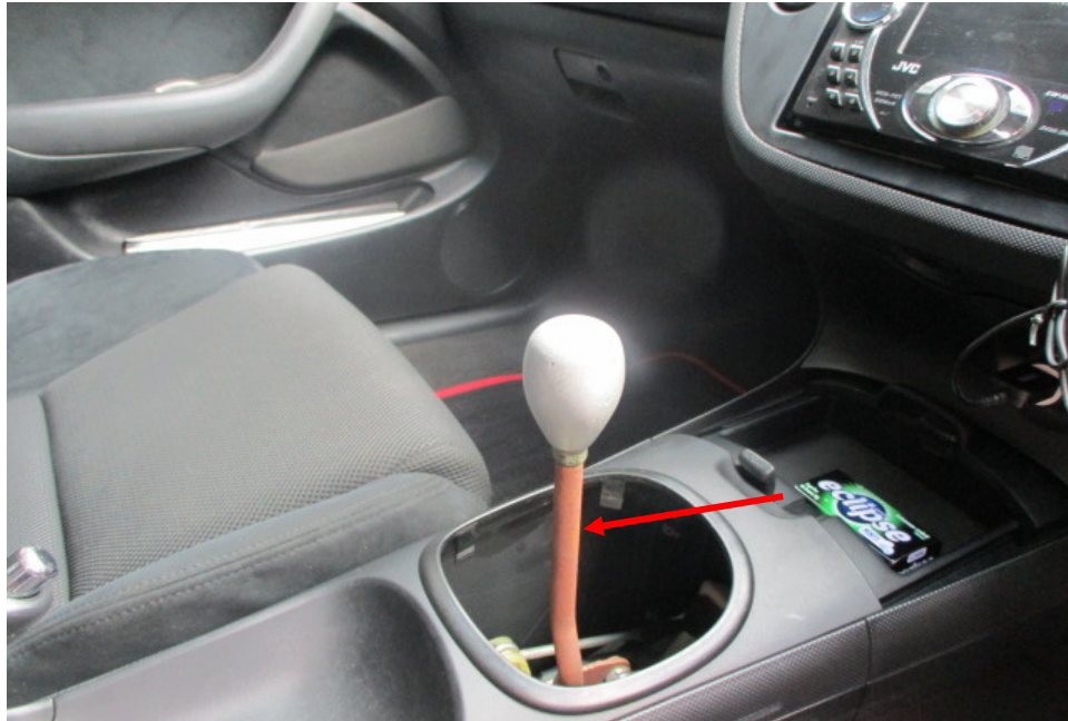
Photo 12 shows the gear shifter (arrowed) that was fitted on the Motor Car, for manually selecting the transmission gear to be engaged. The gear selector cables from the underside of the Motor Car (refer to photograph 10 & 11 above) connects to this gear shifter through the floorboard.
