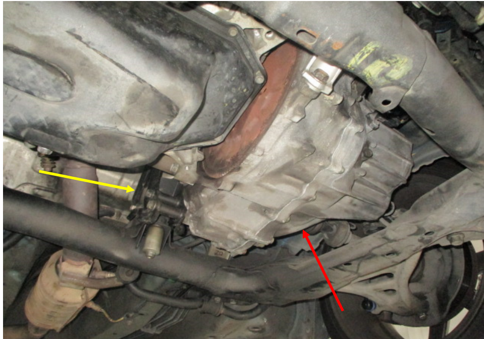
Photo 4 shows another view of the transmission assembly (red arrow) that was fitted on the Motor Car. This was at the input side where the transmission assembly is bolted onto the crankshaft side of the engine block. The transmission assembly of the Motor Car was supported by 3 brackets. One at the front of the transmission assembly, one at the rear of the transmission assembly (yellow arrow) while the other was at the left side of the transmission assembly.
