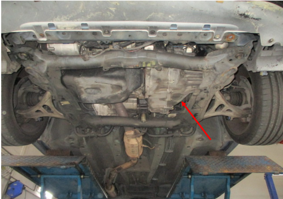
Photo 2 shows a general view of the transmission assembly (arrowed) that was fitted on the Motor Car. The input side of the transmission assembly is bolted to the crankshaft side of the engine block. The left and right drive shafts were securely fitted from the main shaft, located inside the transmission assembly, to the front left wheel and front right wheel respectively. There was no crack and/or hole observed on the housing of the transmission assembly.
