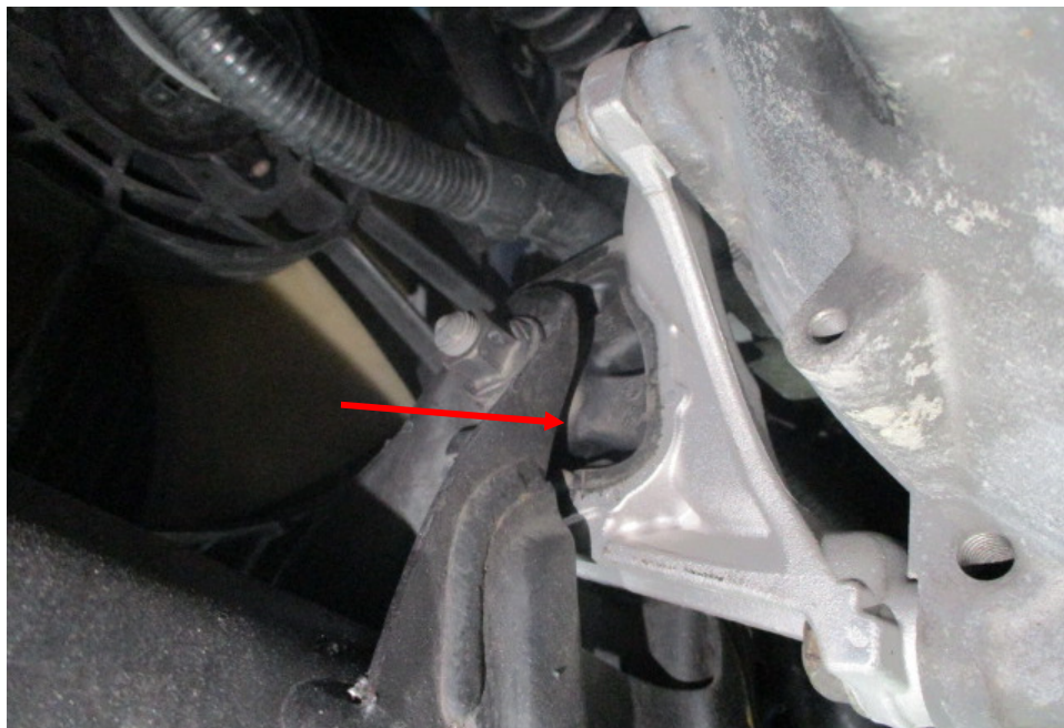
Photo 7 shows a closer view of the bracket supporting the front of the Motor Car's transmission assembly. This bracket was mounted onto the engine cross member. The bracket was with rubber bushings (arrowed) that absorbs any vibrations arising from the rotation of the transmission gears, minimising any stress to the bracket and correspondingly also minimise any stress to the engine crossmember.
