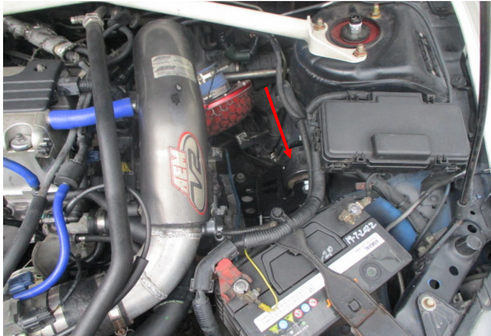
Photo 8 shows the bracket (arrowed) supporting the left side of the Motor Car's transmission assembly. This bracket was mounted onto the left side front chassis, adjacent to the left side front wheel house of the Motor Car. The bracket was with rubber bushings that absorbs any vibrations arising from the rotation of the transmission gears, minimising any stress to the bracket and correspondingly also minimise any stress to the engine crossmember.
