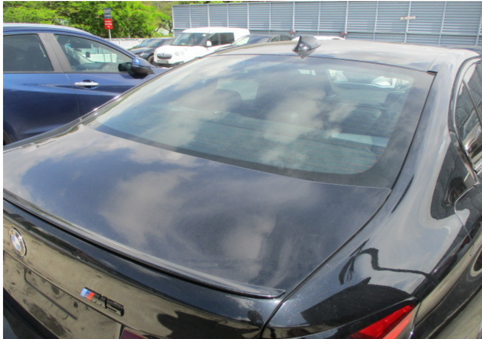
Photo 14 shows a closer view of the Motor Car's rear bootlid, rear right outer "C" pillar and rear windscreen. The body parts at the right side portion of the Motor Car were visually examined and it was observed that the repair/restoration works carried out to the damaged area of the Motor Car (refer to photograph 3 above) were reasonably adequate and in order.
