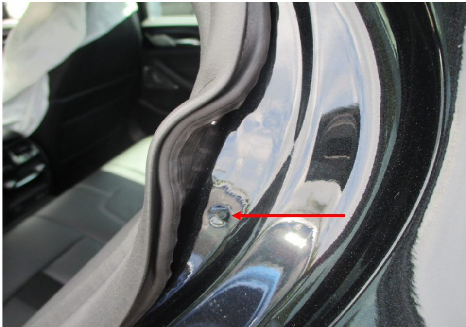
Photo 35 shows the left side "C" pillar of the Motor Car. I did not find any weld marks other than original spot weld marks (arrowed) on the left side "C" pillar of the Motor Car, which indicates that there was no re-welding works carried out. In general, I had found all the non-detachable body panels of the Motor Car to be originally fitted at the time of my inspection.
