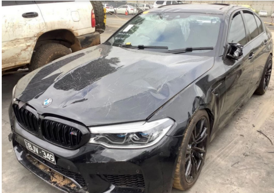
Photo 1 shows the front left body of the Motor Car (photograph provided to me). The photographs provided to me had showed damage to the left side portion of the Motor Car. The front bumper, front bonnet, front left fender, front left outer "A" pillar and left wing mirror were amongst the body parts that were observed to have been damaged.
