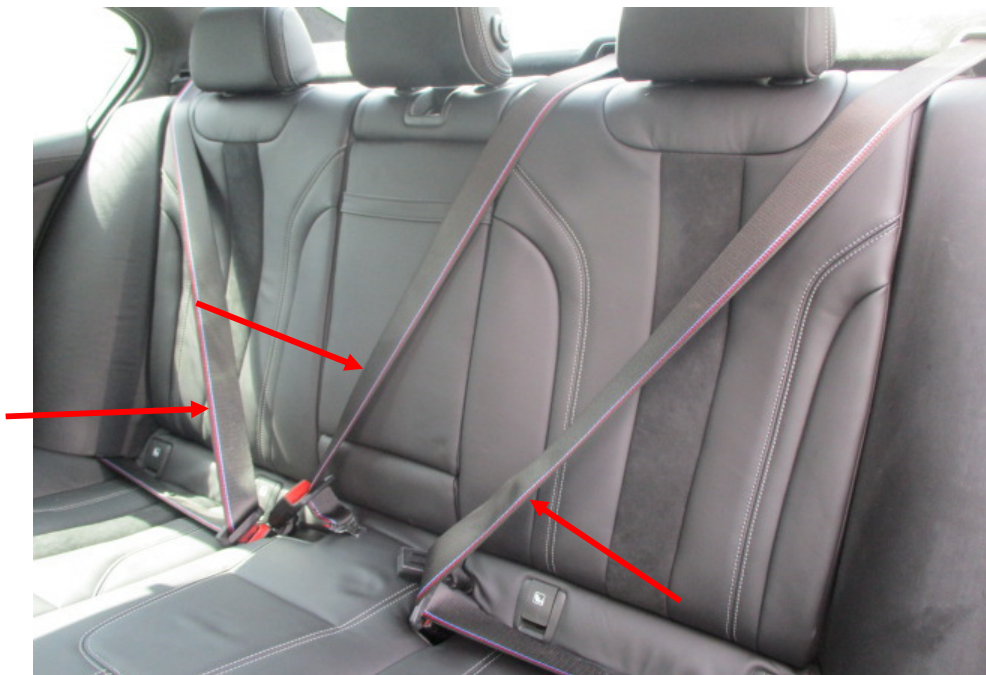
Photo 21 shows the rear seats of the Motor Car. All the seats of the Motor Car were secured via seat rails to the floorboard. They were also fitted with a retractable seat belt reel and a pre-tensioner. The seat belts (arrowed) were tested and were able to be fastened into the respective pre-tensions that were fitted on the side of each individual seat.
