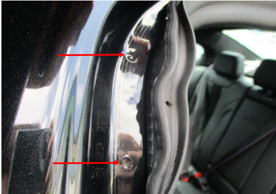
Photo 36 shows the left side "B" pillar of the Motor Car. I did not find any weld marks other than original spot weld marks (arrowed) on the left side "B" pillar of the Motor Car, which indicates that there was no re-welding works carried out. In general, I had found all the non-detachable body panels of the Motor Car to be originally fitted at the time of my inspection.
