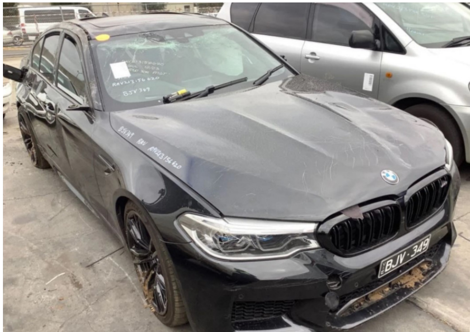
Photo 2 shows the front right body of the Motor Car (photograph provided to me). The photographs provided to me had showed damage to the right side portion of the Motor Car. The front right outer "A" pillar and right wing mirror were amongst the body parts that were observed to have been damaged. The Motor Car's roof panel and front windscreen were also observed to be damaged.
