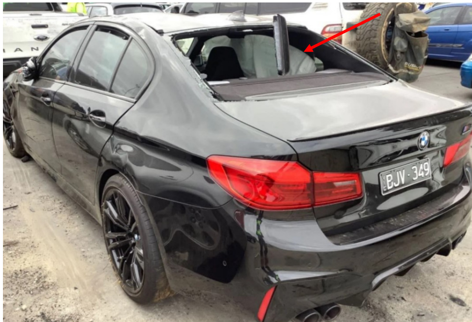
Photo 4 shows the rear left body of the Motor Car (photograph provided to me). The photographs provided to me had showed damage to the left side portion of the Motor Car. The rear left fender, rear left door and rear left outer "C" pillar were amongst the body parts that were observed to have been damaged. The Motor Car's roof panel and rear windscreen were also observed to be damaged. The right curtain airbag was deployed (arrowed).
