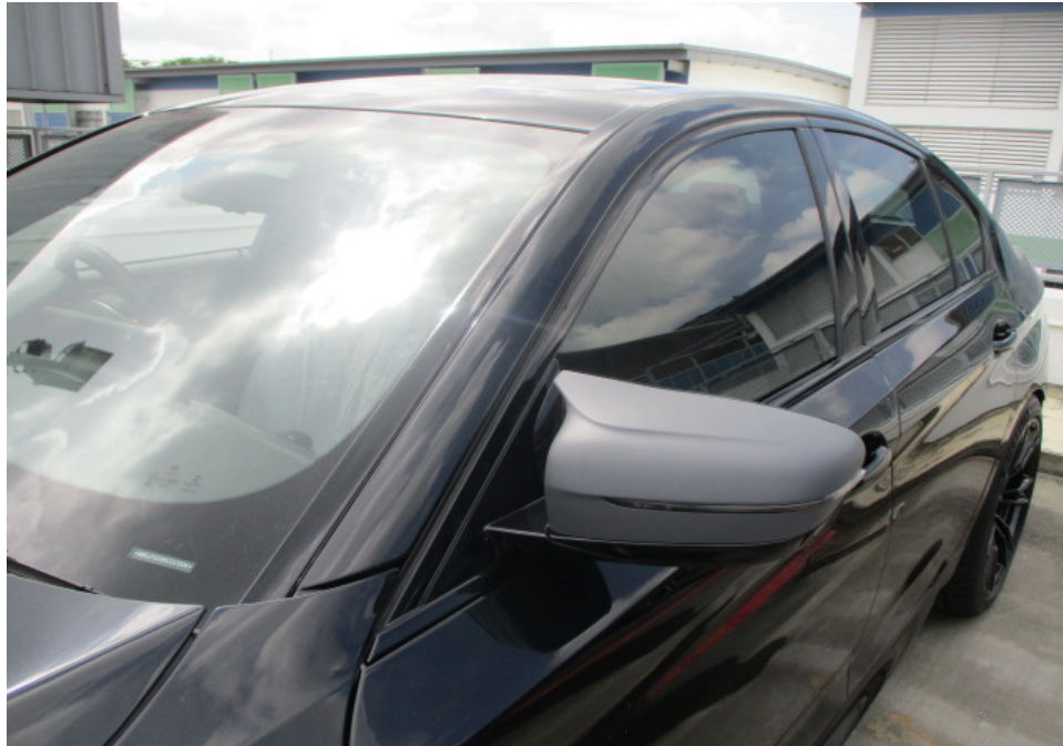
Photo 8 shows a closer view of the Motor Car's left side wing mirror, front left outer "A" pillar and front windscreen. The body parts at the left side portion of the Motor Car were visually examined and it was observed that the repair/restoration works carried out to the damaged area of the Motor Car (refer to photograph 1 above) were reasonably adequate and in order.
