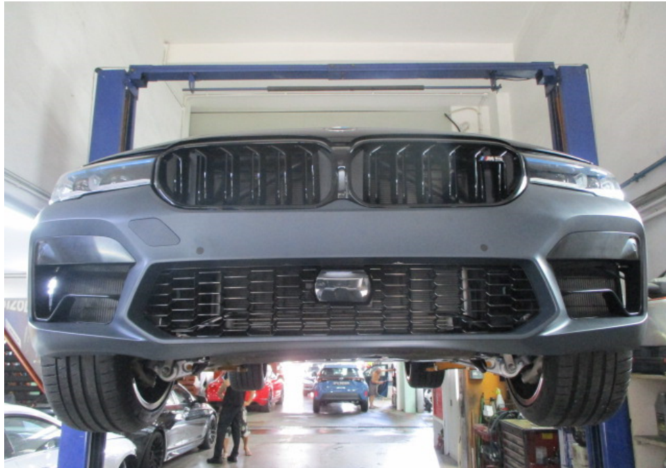
Photo 24 shows the Motor Car hoisted up for checks on its undercarriage. There was no sign(s) or indication(s) of fluid leakage and/or fluid stain(s) on the underside of the Motor Car. The undercarriage components of the Motor Car were also all observed to be intact and secured in an appropriate manner.
