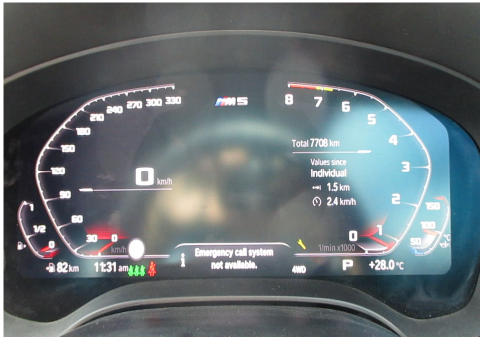
Photo 23 shows the respective warning lights no longer illuminated, indicating that there is no fault detected to the ABS, SRS, IAS, TPM and DSC systems of the Motor Car during the self-test. These electronic systems were hence in working condition at the time of my inspection.
