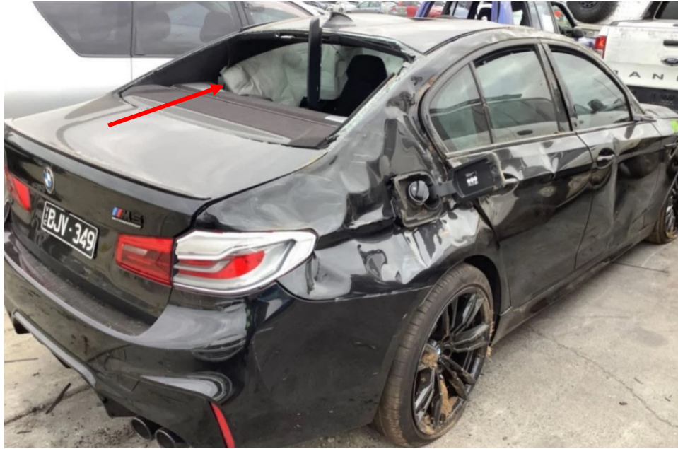
Photo 3 shows the rear right body of the Motor Car (photograph provided to me). Apart for the left side portion, damage was also seen to the right side portion of the Motor Car. Body parts damaged include the right side wing mirror, front right door, rear right door, rear right outer "C" pillar, rear right fender, rear right taillamp, rear bumper and fuel filler cover amongst others. The Motor Car's roof panel and rear windscreen were also observed to be damaged. The left curtain airbag was deployed (arrowed).
