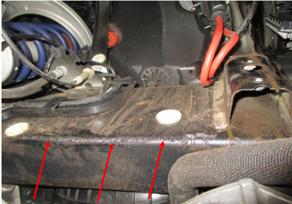
Photo 34 shows the chassis/structural body at the underside front right of the Motor Car. I did not find any weld marks other than original spot weld marks on the chassis/structural body of the Motor Car. The original factory sealant (arrowed) at the joints along the chassis/structural body was untouched, indicating no work was done on the chassis/structural body of the Motor Car and that the chassis/structural body was originally fitted.
