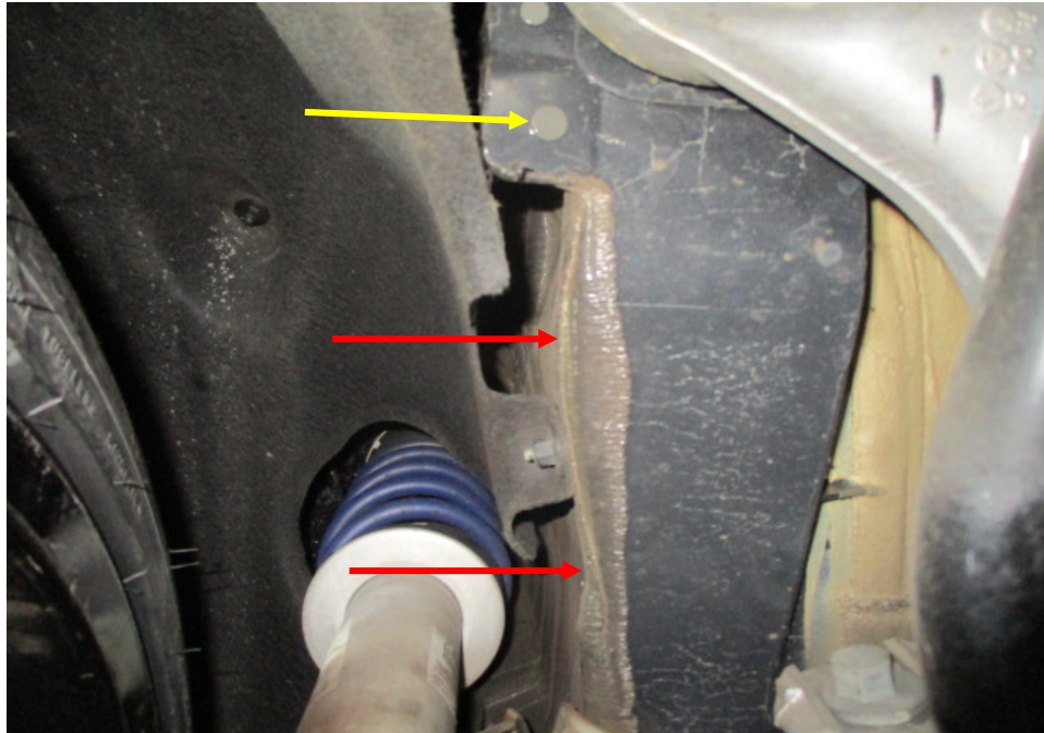
Photo 32 shows the chassis/structural body at the underside rear left of the Motor Car. I did not find any weld marks other than original spot weld marks (yellow arrow) on the chassis/structural body of the Motor Car. The original factory sealant (red arrow) at the joints along the chassis/structural body was untouched, indicating no work was done on the chassis/structural body of the Motor Car and that the chassis/structural body was originally fitted.
