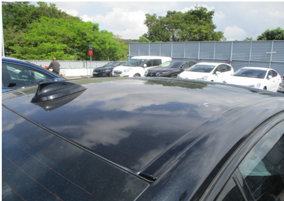
Photo 15 shows a closer view of the Motor Car's rear right outer "C" pillar and roof panel. The body parts at the right side portion of the Motor Car were visually examined and it was observed that the repair/restoration works carried out to the damaged area of the Motor Car (refer to photograph 3 above) were reasonably adequate and in order.
