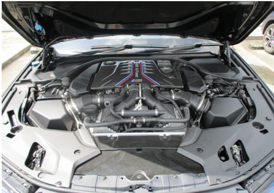
Photo 19 shows a general view of the Motor Car's engine compartment at the time of my inspection. The various parts and components inside the engine compartment were all observed to be intact and properly fitted. There was also no sign(s) or indication(s) of fluid leak and/or fluid stain found inside the engine compartment.
