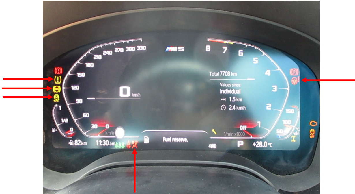
Photo 22 shows the warning lights for the various electronic safety features appearing on the instrument panel of the Motor Car during its self-test when the engine is cranked, in particular the ABS, SRS, IAS, TPM and DSC lights (arrowed).
