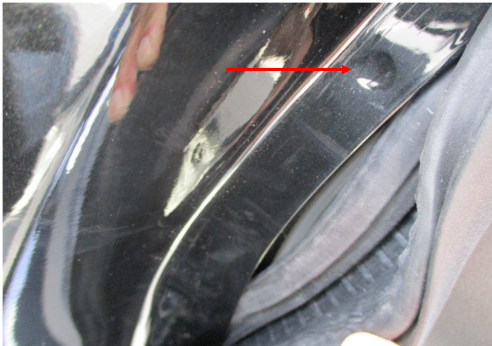
Photo 37 shows the left side "A" pillar of the Motor Car. I did not find any weld marks other than original spot weld marks (arrowed) on the left side "A" pillar of the Motor Car, which indicates that there was no re-welding works carried out. In general, I had found all the non-detachable body panels of the Motor Car to be originally fitted at the time of my inspection.
