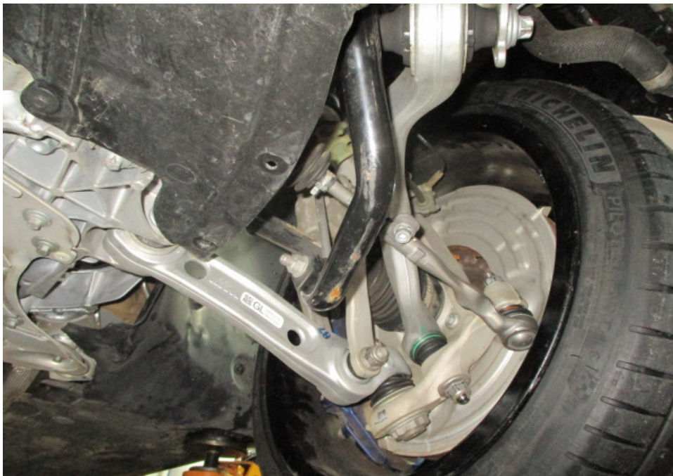
Photo 27 shows the various undercarriage components at the front left wheel of the Motor Car. The mechanical components, control arms and linkages were all found to be intact and secured in an appropriate manner.
