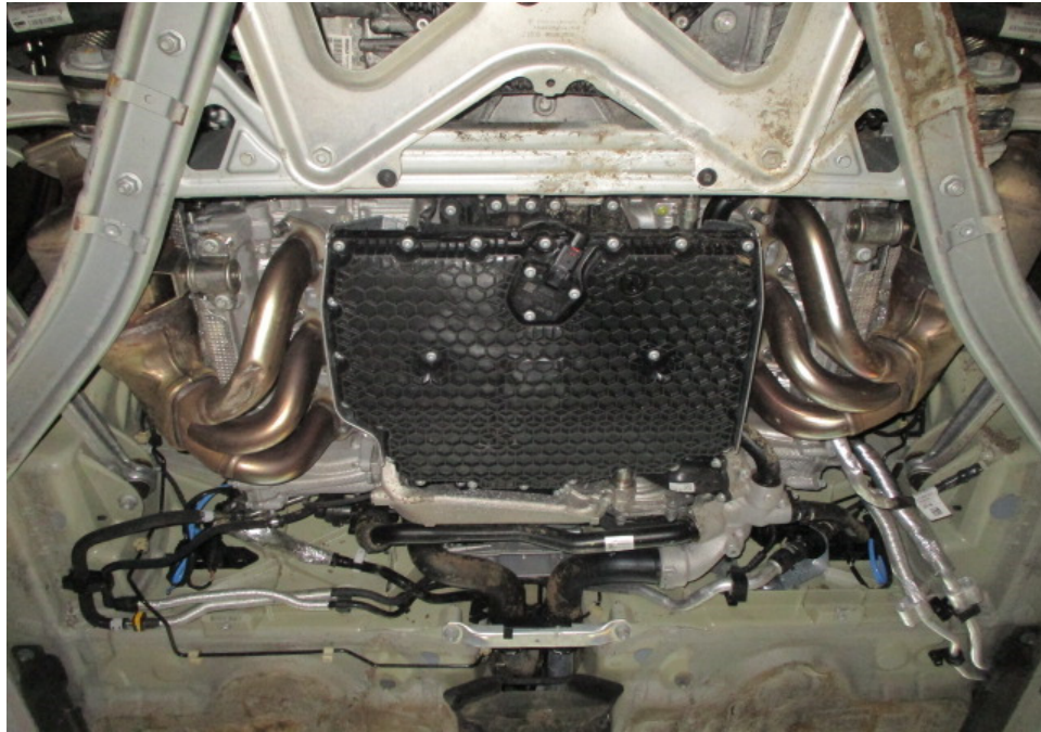
Photo 32 shows the Motor Car's exhaust manifolds. My examination of the Motor Car's exhaust system revealed no sign(s) or indication(s) of any cut or weld marks along its exhaust pipes, on its resonator boxes, on its catalytic converters and on its rear mufflers.
