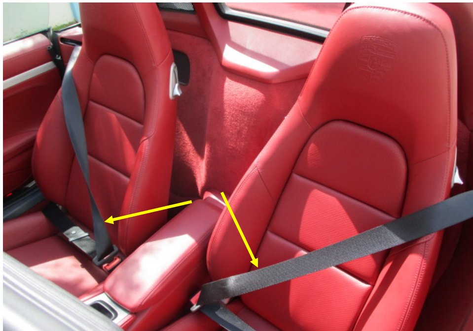
Photo 23 shows the seats of the Motor Car. All the seats of the Motor Car were secured via seat rails to the floorboard. They were also fitted with a retractable seat belt reel and a pre-tensioner. The seat belts (arrowed) were tested and were able to be fastened into the respective pre-tensions that were fitted on the side of each individual seat.
