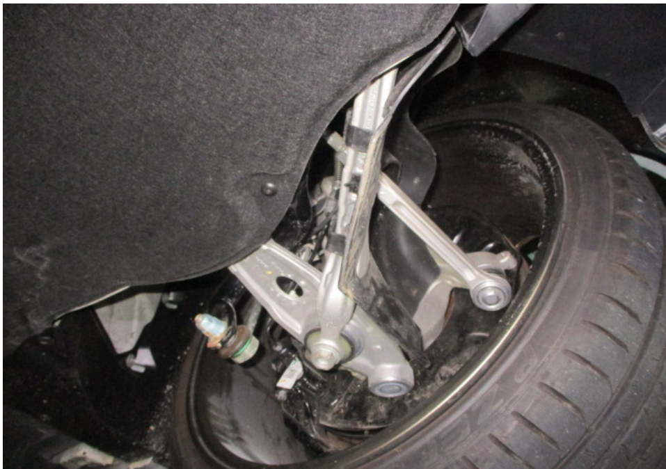
Photo 29 shows the various undercarriage components at the front left wheel of the Motor Car. The mechanical components, control arms and linkages were all found to be intact and secured in an appropriate manner.
