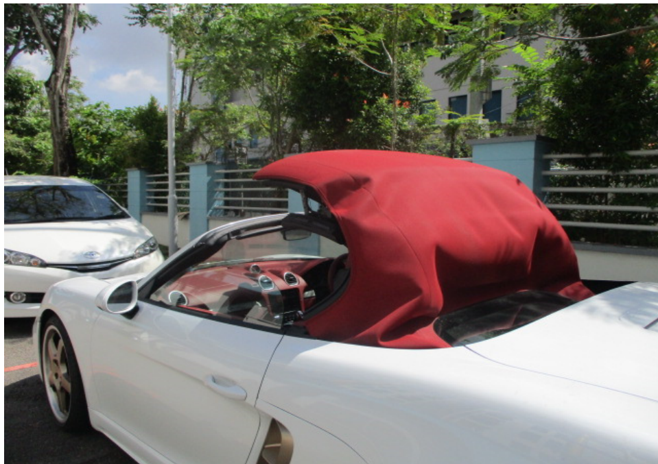
Photo 19 shows the Motor Car's soft top roof being tested. It was observed that as a safety feature, the soft top roof could only open and close when the Motor Car was in a stationary position or at low travelling speed. When opened, the soft top roof is completely folded into the rear compartment with no parts protruding out of the Motor Car's body. The soft top roof was also found adequately secured to the "A" pillar after closing.
