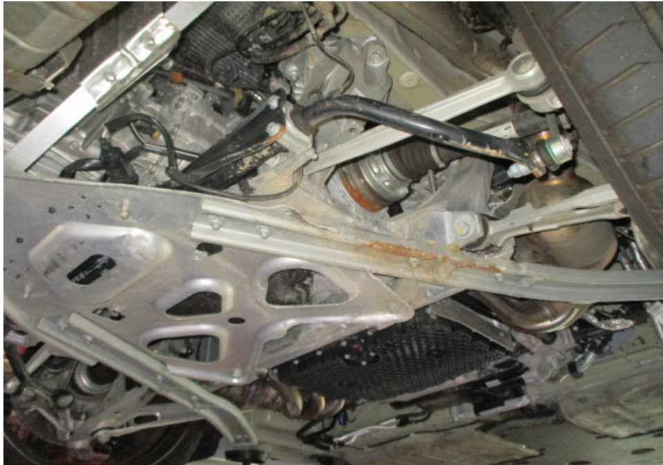
Photo 34 shows another view of the Motor Car's engine compartment. The engine compartment was at the rear underside of the Motor Car. The various parts and components inside the engine compartment were all observed to be intact and properly fitted. There was also no sign(s) or indication(s) of fluid leak and/or fluid stain found inside the engine compartment.
