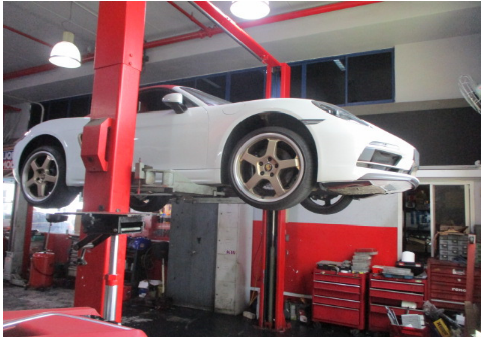
Photo 26 shows the Motor Car hoisted up for checks on its undercarriage. There was no sign(s) or indication(s) of fluid leakage and/or fluid stain(s) on the underside of the Motor Car. The undercarriage components of the Motor Car were also all observed to be intact and secured in an appropriate manner.
