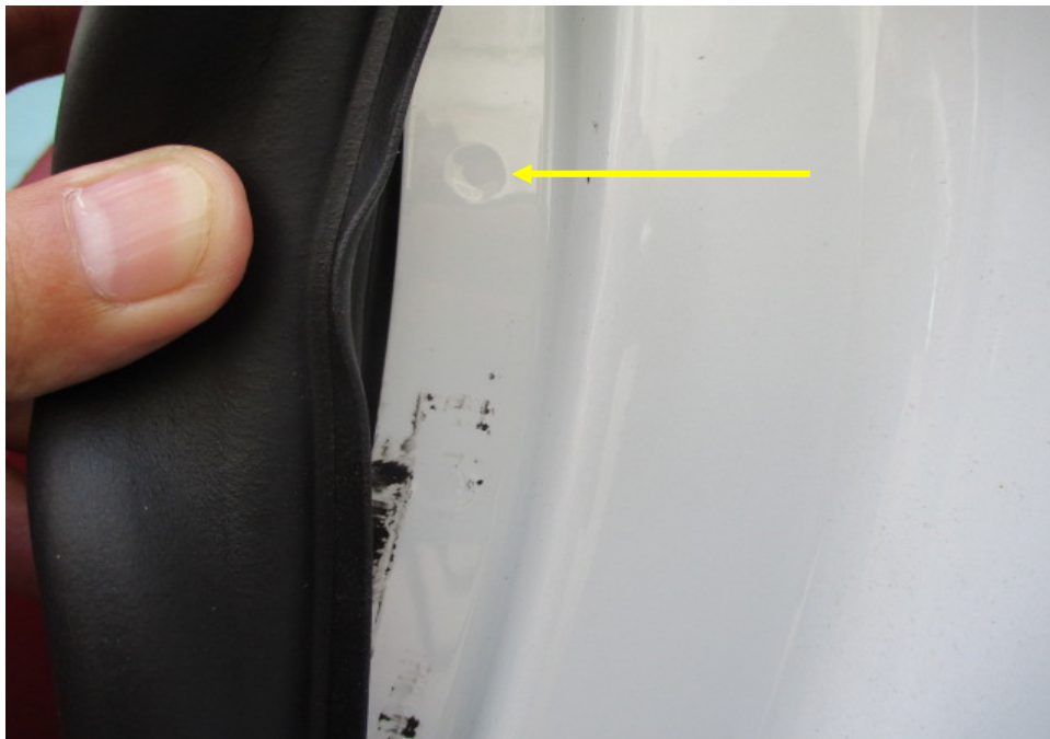
Photo 39 shows the rear left body panel of the Motor Car. I did not find any weld marks other than original spot weld marks (arrowed) on the rear left body panel of the Motor Car, which indicates that there was no re-welding works carried out. In general, I had found all the non-detachable body panels of the Motor Car to be originally fitted at the time of my inspection.
