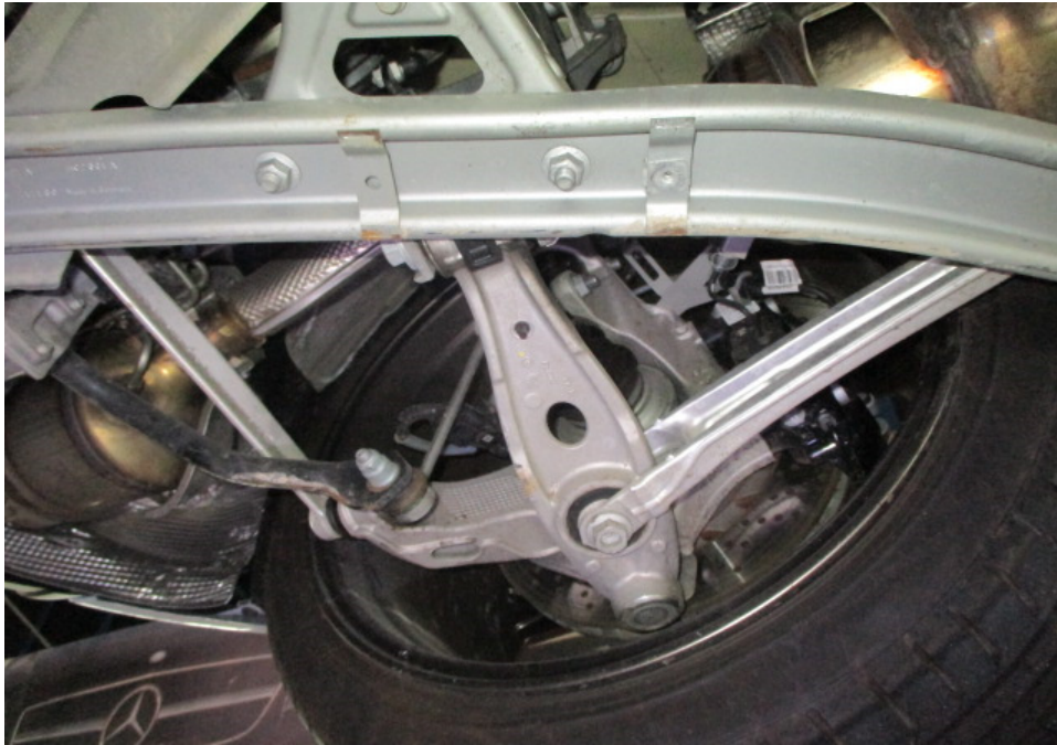
Photo 28 shows a general view of the control arms and linkages at the rear left wheel of the Motor Car. I did not observe any fluid leak and/or fluid stain on the underside of the Motor Car. All of the Motor Car's undercarriage components were observed to be intact and secured in an appropriate manner.
