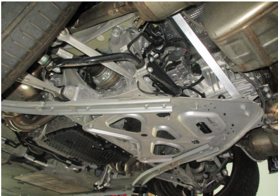
Photo 33 shows a general view of the Motor Car's engine compartment. The engine compartment was at the rear underside of the Motor Car. The various parts and components inside the engine compartment were all observed to be intact and properly fitted. There was also no sign(s) or indication(s) of fluid leak and/or fluid stain found inside the engine compartment.
