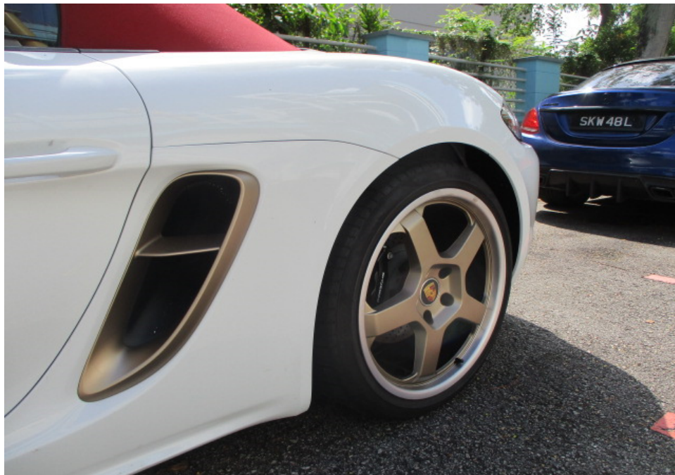
Photo 9 shows a closer view of the Motor Car's rear body panel, rear left side air duct, rear left wheel rim and left side rocker panel garnish. The body parts along the entire left side portion of the Motor Car were visually examined and it was observed that the repair/restoration works carried out to the damaged area of the Motor Car (refer to photograph 2 above) were reasonably adequate and in order.
