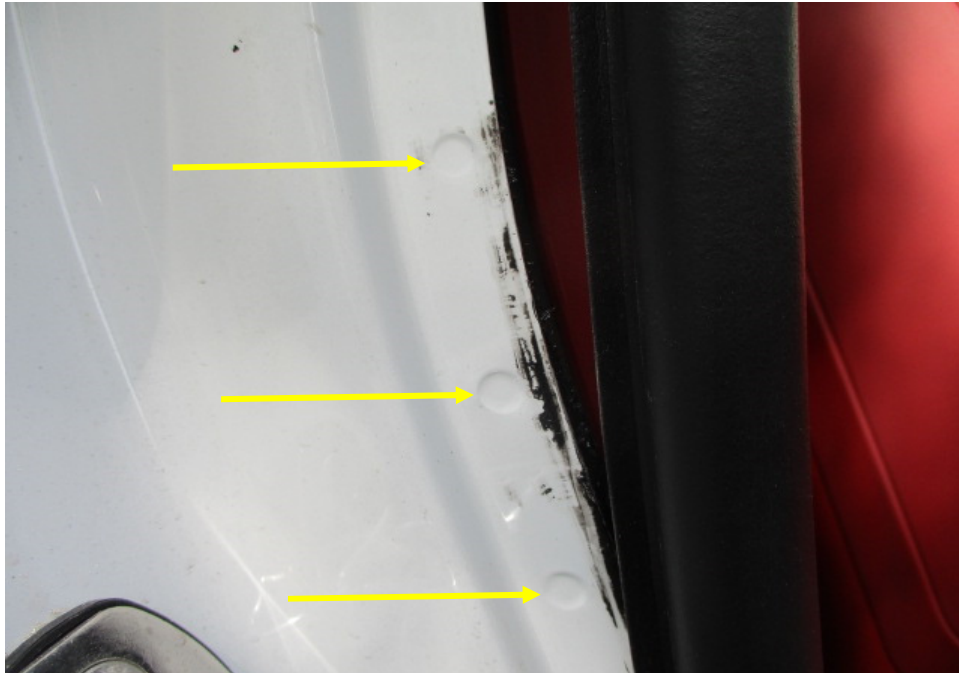
Photo 42 shows the rear right body panel of the Motor Car. I did not find any weld marks other than original spot weld marks (arrowed) on the rear right body panel of the Motor Car, which indicates that there was no re-welding works carried out. In general, I had found all the non-detachable body panels of the Motor Car to be originally fitted at the time of my inspection.
