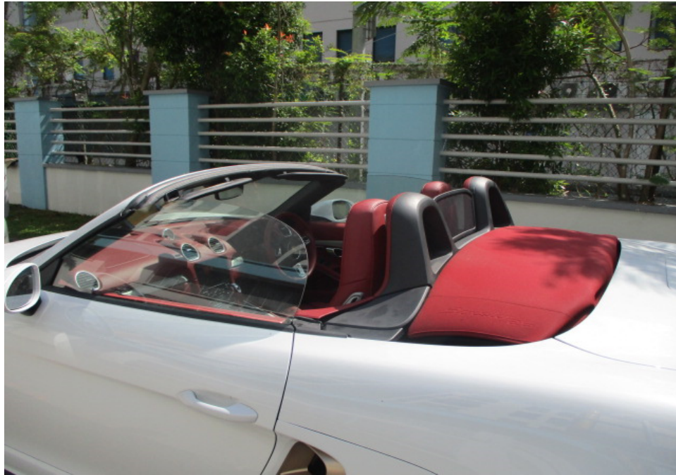
Photo 20 shows the Motor Car with its soft top roof completely folded. It was observed that as a safety feature, the soft top roof could only open and close when the Motor Car was in a stationary position or at low travelling speed. When opened, the soft top roof is completely folded into the rear compartment with no parts protruding out of the Motor Car's body. The soft top roof was also found adequately secured to the "A" pillar after closing.
