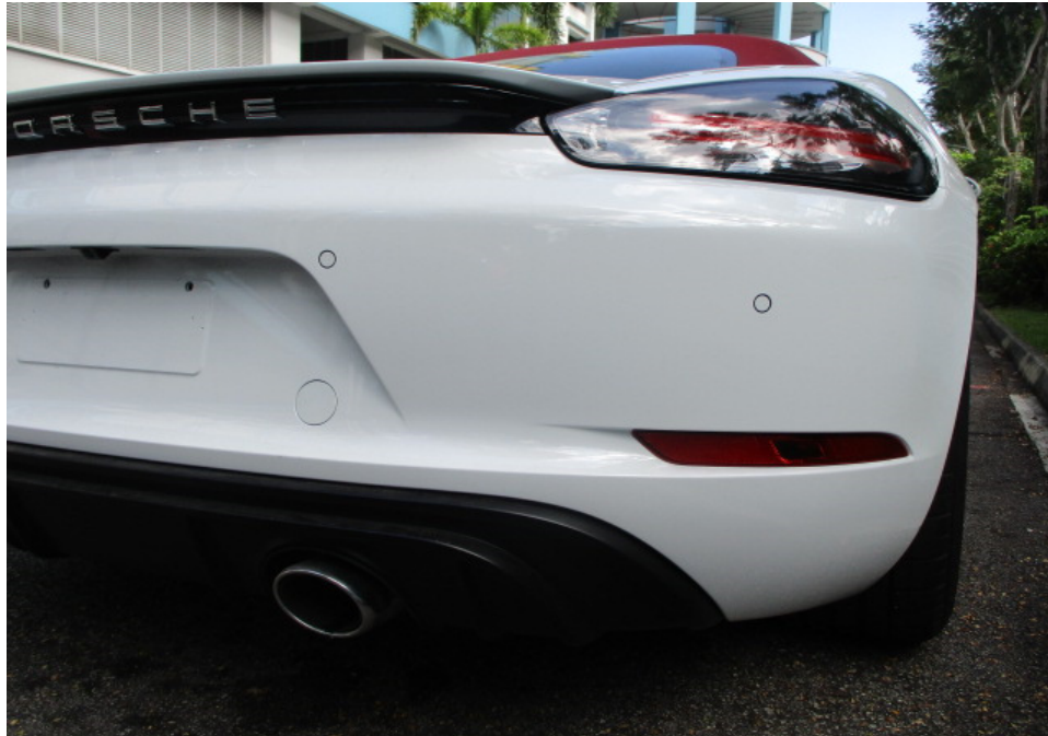
Photo 16 shows a closer view of the Motor Car's rear bumper, rear bumper lower cover, rear bumper right reflector, rear bumper sensors and rear right taillamp. The body parts at the rear portion of the Motor Car were visually examined and it was observed that the repair/restoration works carried out to the damaged area of the Motor Car (refer to photograph 3 above) were reasonably adequate and in order.
