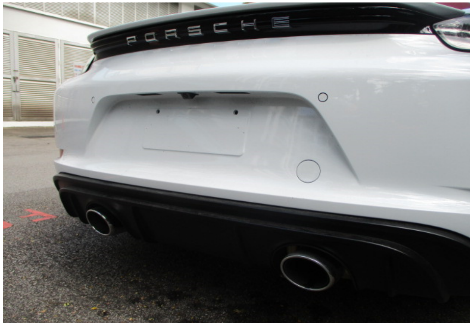
Photo 17 shows a closer view of the Motor Car's rear bumper, rear bumper lower cover and rear bumper sensors. The body parts at the rear portion of the Motor Car were visually examined and it was observed that the repair/restoration works carried out to the damaged area of the Motor Car (refer to photograph 3 above) were reasonably adequate and in order.
