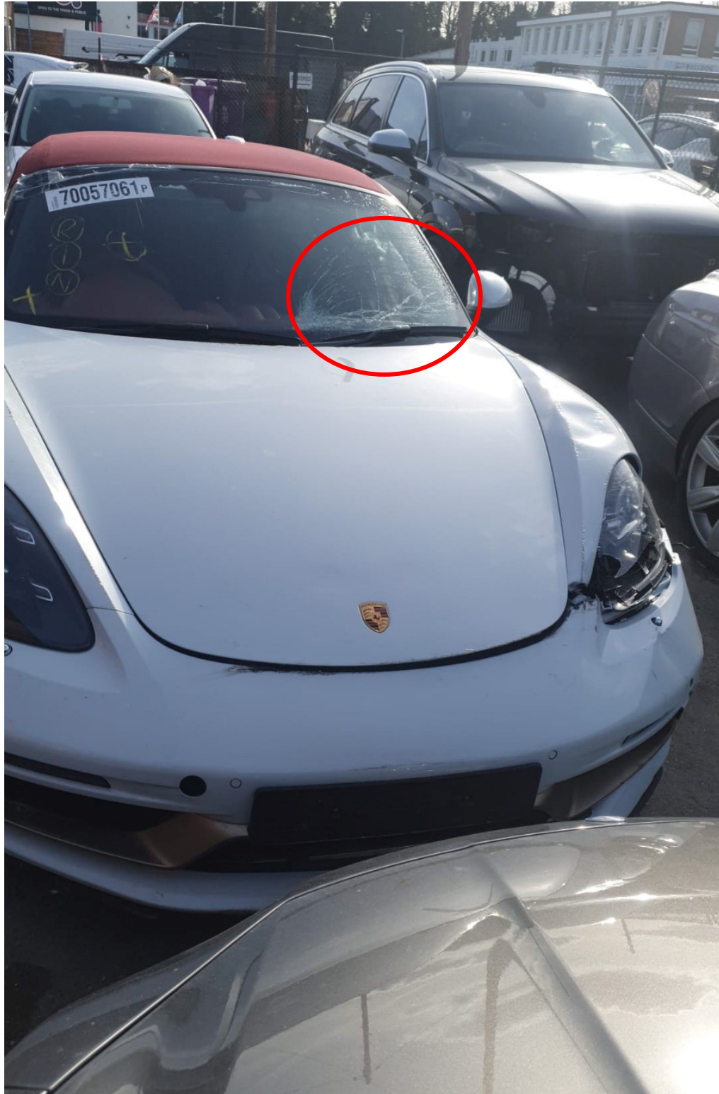
Photo 1 shows the frontal body of the Motor Car (photograph provided to me). The photographs provided to me had showed damage along the entire left side portion and rear portion of the Motor Car. The front bumper, front left headlamp, front left fender and front windscreen (circled) were amongst the body parts that were observed to have been damaged.
