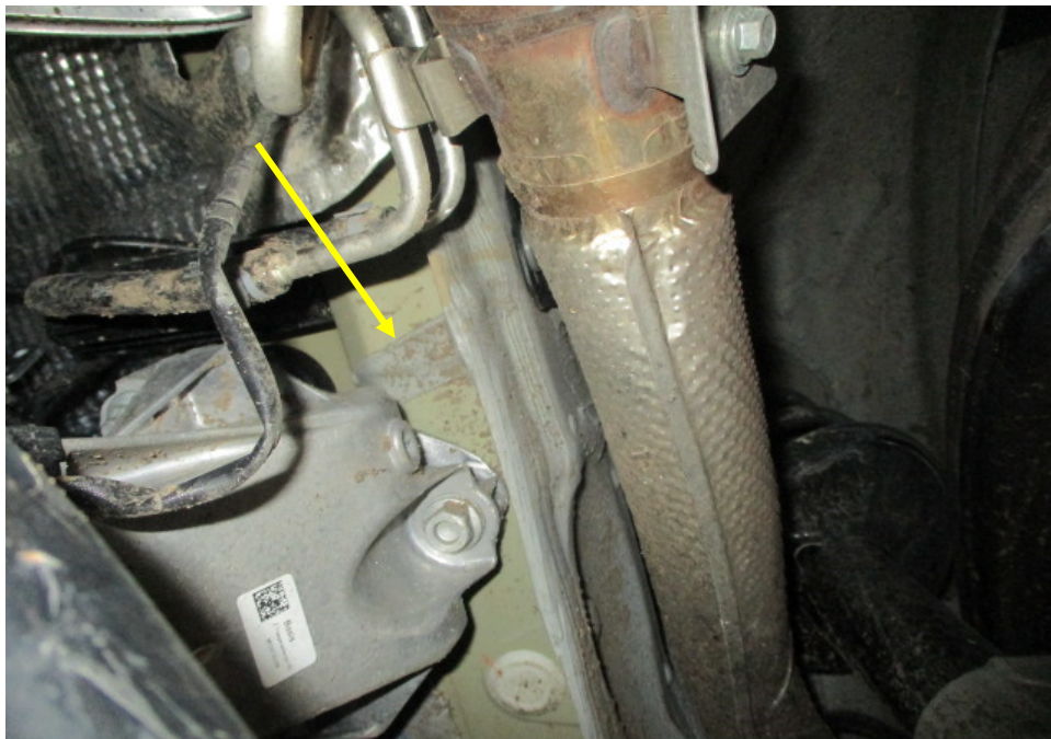
Photo 35 shows the chassis/structural body at the underside rear right of the Motor Car. I did not find any weld marks other than original spot weld marks on the chassis/structural body of the Motor Car. The original factory sealant (arrowed) at the joints along the chassis/structural body was untouched, indicating no work was done on the chassis/structural body of the Motor Car and that the chassis/structural body was originally fitted.
