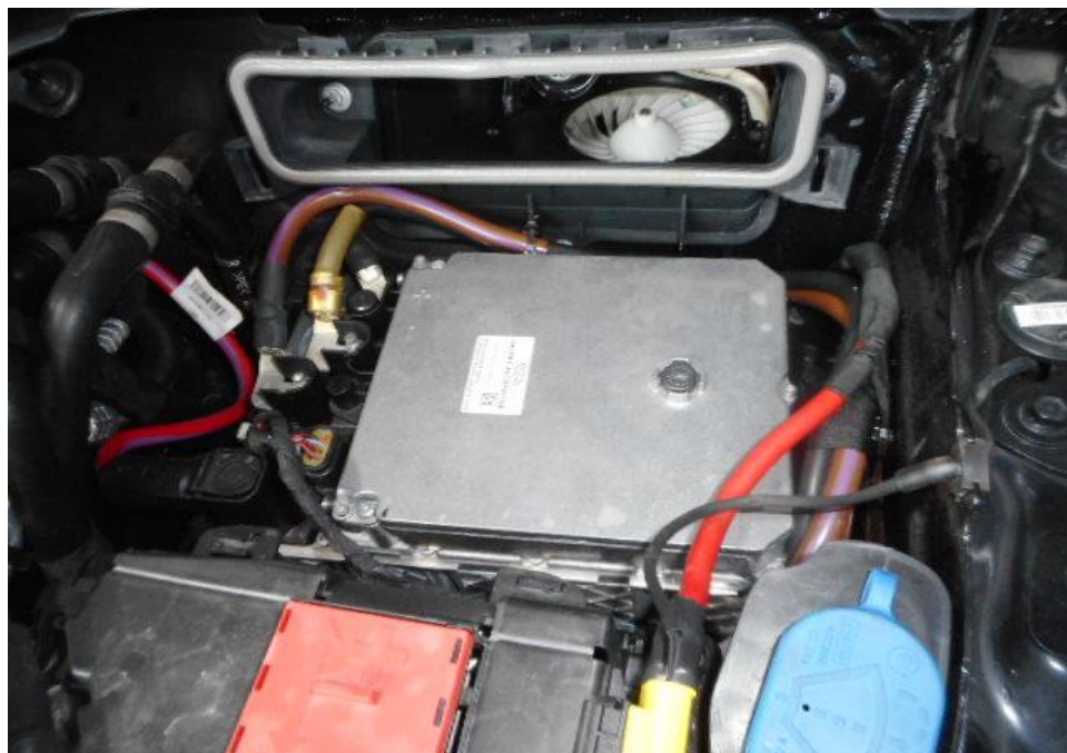
Photo 5 shows the general view of the 48v battery and its components in the engine compartment portion of the Insured Vehicle at the time of our inspection. The 48v battery and its components is observed to be unaffected and by any signs of accident.
