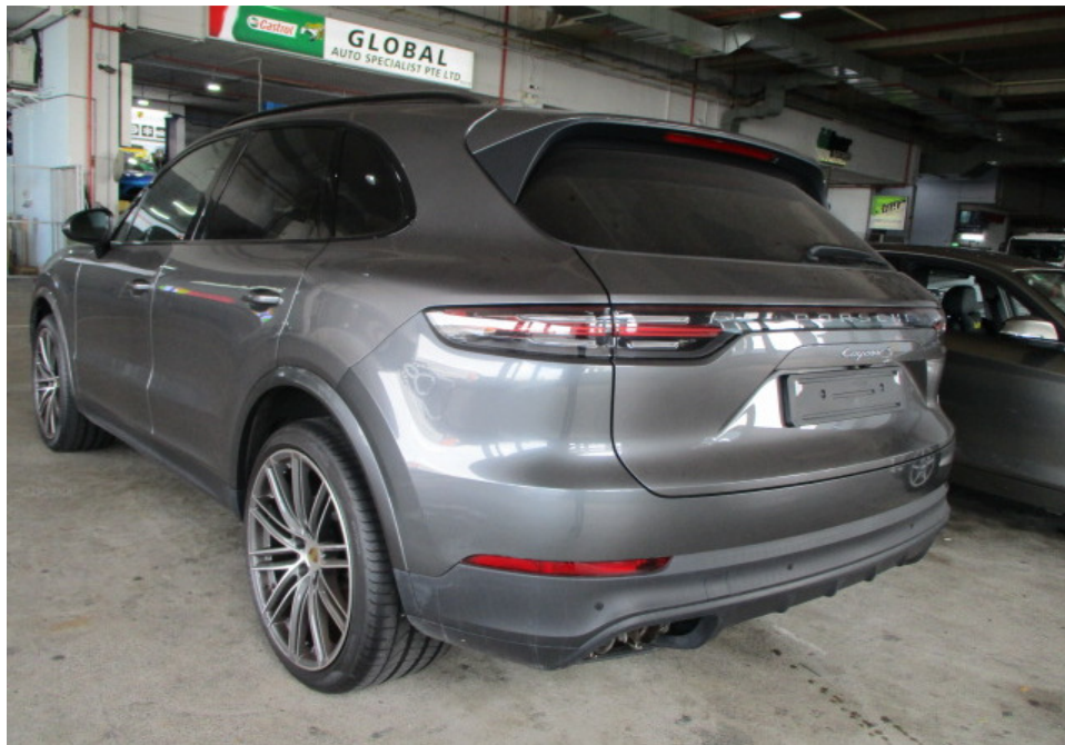
Photo 7 shows a general view of the rear left body of the Motor Car at the time of my inspection. The Motor Car was observed to be in a relatively good general condition with no loose exterior fittings observed. The body parts at the rear left portion of the Motor Car were visually examined and it was observed that the repair/restoration works carried out to the damaged area of the Motor Car (refer to photograph 1, 2 & 5 above) were reasonably adequate and in order.
