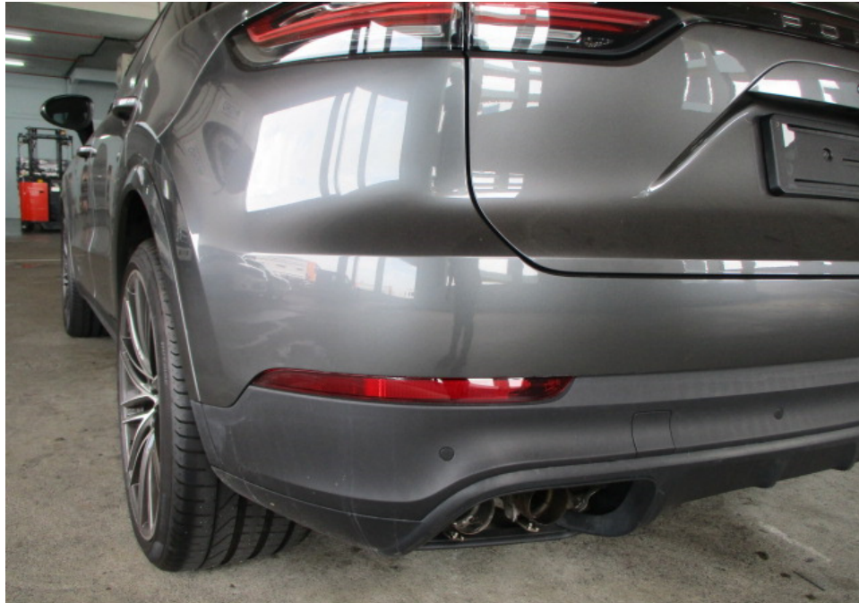
Photo 8 shows a closer view of the Motor Car's rear bumper, rear bumper lower cover, rear bumper lower garnish, rear bumper left sensors and rear bumper left reflector at the time of my inspection. The body parts at the rear left portion of the Motor Car were visually examined and it was observed that the repair/restoration works carried out to the damaged area of the Motor Car (refer to photograph 1, 2 & 5 above) were reasonably adequate and in order.
