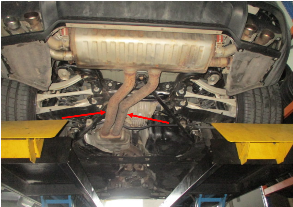
Photo 25 shows the rear section of the Motor Car's exhaust system. My examination of the Motor Car's exhaust system revealed no sign(s) or indication(s) of any cut or weld marks along its exhaust pipes (arrowed), on its rear muffler, on its centre resonator boxes and on its catalytic converters.
