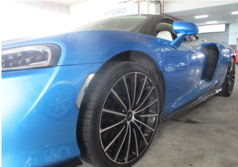
Photo 9 shows a closer view of the Motor Car's front bumper left reflector, front left fender and front left wheel rim at the time of my inspection. The body parts at the front left portion of the Motor Car were visually examined and it was observed that the repair/restoration works carried out to the damaged area of the Motor Car (refer to photograph 1 above) were reasonably adequate and in order.
