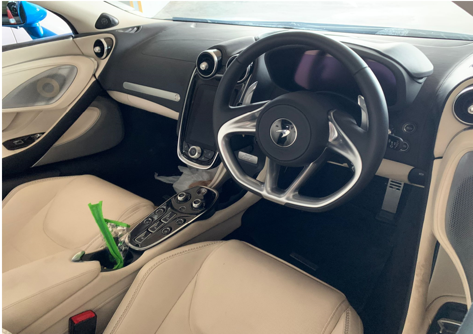
Photo 5 shows the interior compartment of the Motor Car (photograph provided to me). The various parts and components within the interior compartment were all intact and unaffected. The Motor Car's airbag(s) was not deployed as seen from the photographs that were provided to me.
