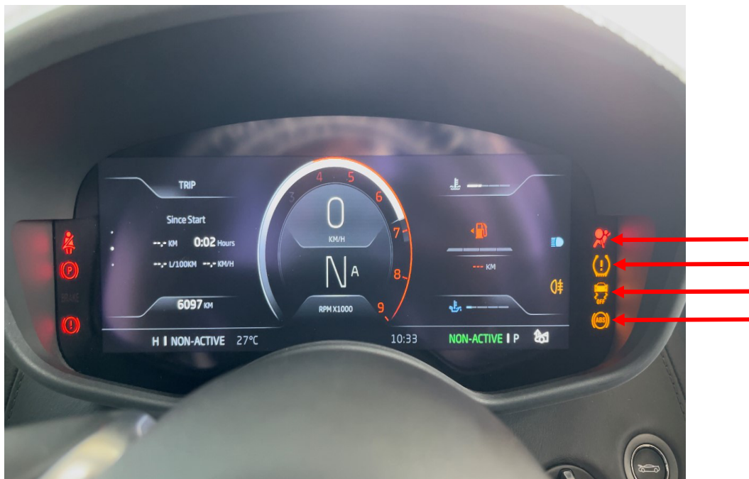
Photo 18 shows the warning lights for the various electronic safety features appearing on the instrument panel of the Motor Car during its self-test when the engine is cranked, in particular the ABS, SRS, TPM and TCS lights (arrowed).
