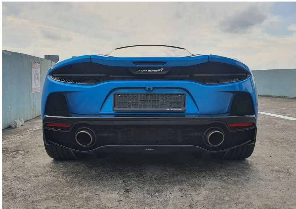
Photo 14 shows a general view of the rear body of the Motor Car at the time of my inspection, with its rear bumper and rear under cover re-fitted. The Motor Car was observed to be in a relatively good general condition with no loose exterior fittings observed. The mileage of the Motor Car recorded at the time of my inspection was 6,097km.
