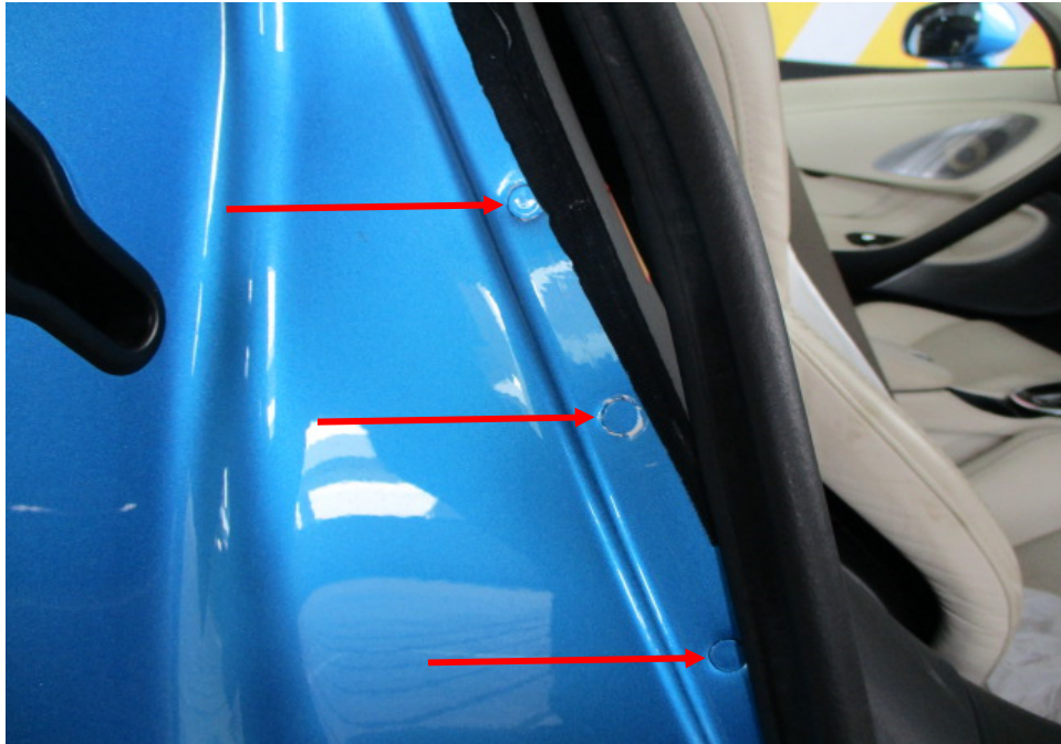
Photo 35 shows the right side rear body panel of the Motor Car. I did not find any weld marks other than original spot weld marks (arrowed) on the right side rear body panel of the Motor Car, which indicates that there was no re-welding works carried out. In general, I had found all the non-detachable body panels of the Motor Car to be originally fitted at the time of my inspection.
