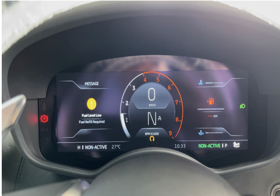
Photo 19 shows the respective warning lights no longer illuminated, indicating that there is no fault detected to the ABS, SRS, TPM and TCS systems of the Motor Car during the self-test. These electronic systems were hence in working condition at the time of my inspection.
