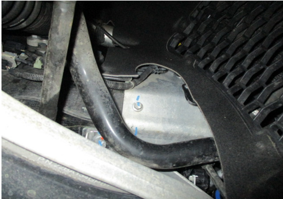
Photo 31 shows the aluminium chassis/structural body at the underside front right of the Motor Car. I did not find any weld marks other than original spot weld marks on the chassis/structural body of the Motor Car. The original factory sealant at the joints along the chassis/structural body was untouched, indicating no work was done on the chassis/structural body of the Motor Car and that the chassis/structural body was originally fitted.
