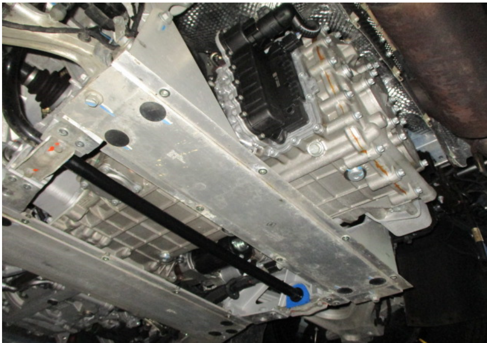
Photo 26 shows the Motor Car's engine compartment as viewed from the rear underside of the Motor Car. The various parts and components inside the engine compartment were all observed to be intact and properly fitted. There was also no sign(s) or indication(s) of fluid leak and/or fluid stain found inside the engine compartment.
