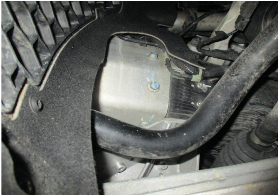
Photo 30 shows the aluminium chassis/structural body at the underside front left of the Motor Car. The original factory sealant at the joints along the chassis/structural body was observed to be untouched. In general, I had found no work was carried out on the chassis/structural body of the Motor Car. The aluminium chassis/structural body of the Motor Car was originally fitted.
