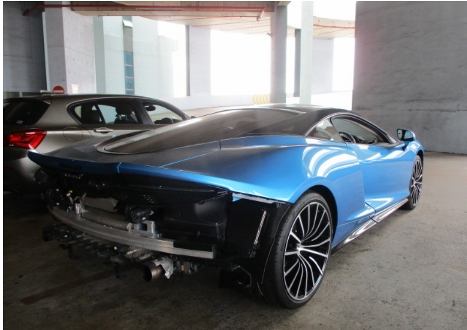
Photo 13 shows a general view of the rear right body of the Motor Car at the time of my inspection, with its rear bumper and rear under cover removed to facilitate checks of its engine compartment and exhaust system. Overall, the Motor Car was observed to be in a relatively good general condition with no loose exterior fittings observed.
