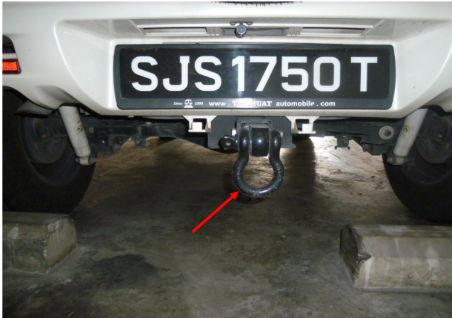
Photo 14 shows the tow hook found to be fitted on the rear portion of the Insured Vehicle at the time of our inspection (arrowed). The tow hook fitted on the Insured Vehicle was not the standard type for the Insured Vehicle.
