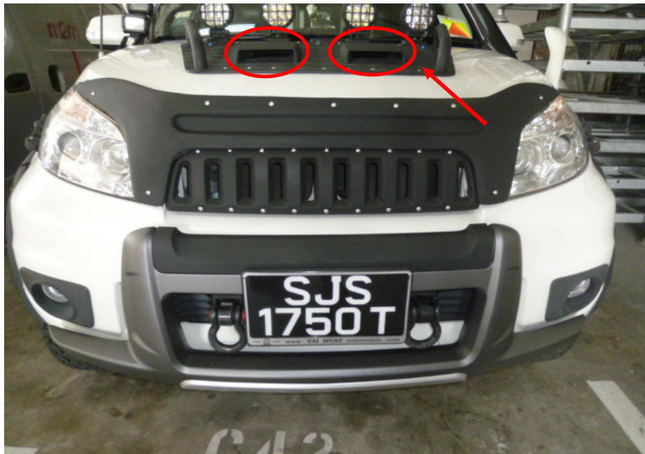
Photo 17 shows a general view of the front bonnet of the Insured Vehicle at the time of our inspection. An aftermarket checkered plate (arrowed) with air scoops (circled) were found fitted.
