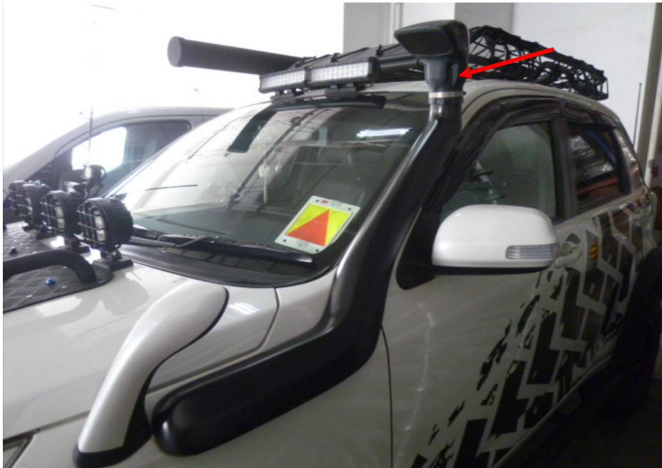
Photo 8 shows a close up view of the non- standard snorkel fitted onto the Insured Vehicle upon our inspection (arrowed).
