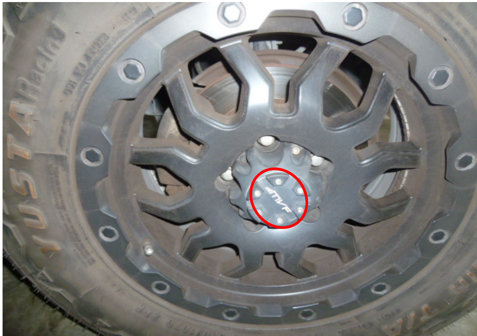
Photo 15 shows the non-standard rim found to be fitted on the Insured Vehicle at the time of our inspection. The 16-inch alloy rims fitted on the Insured Vehicle were not the standard type for the Insured Vehicle. The brand of the rim was 'MVF' (circled).
