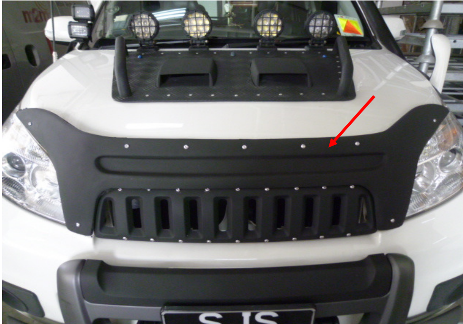
Photo 19 shows the front bonnet guard found to be fitted on the Insured Vehicle at the time of our inspection (arrowed). The front bonnet guard fitted onto the Insured Vehicle was not the standard type for the Insured Vehicle. We noted that the front grille rack was fitted on the Insured Vehicle post- accident.
