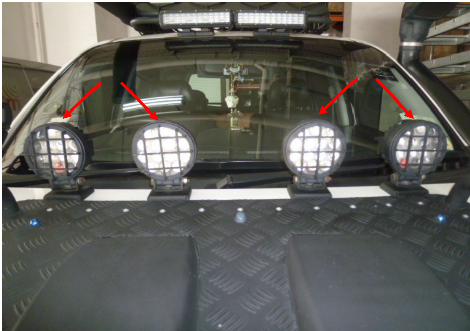
Photo 11 shows the spot lamps additionally fitted onto the front bonnet of the Insured Vehicle upon our inspection (circled). However upon closer inspection, we observed that the spot lamps were not connected.
