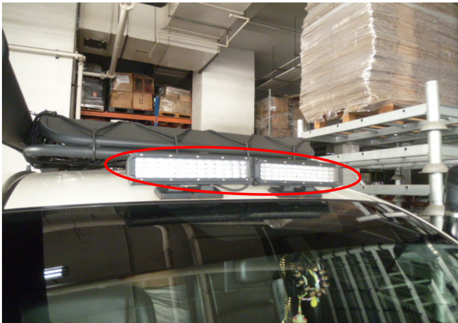
Photo 9 shows the spot lamps additionally fitted onto the roof of the Insured Vehicle upon our inspection (circled). However upon closer inspection, we observed that the spot lamps were not connected.
