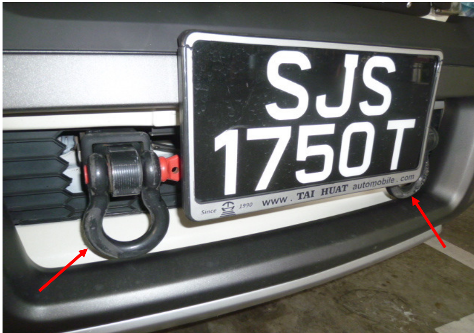
Photo 13 shows the tow hooks found to be fitted onto the frontal portion of the Insured Vehicle at the time of our inspection (arrowed). The tow hooks fitted on the Insured Vehicle were not the standard type for the Insured Vehicle.
