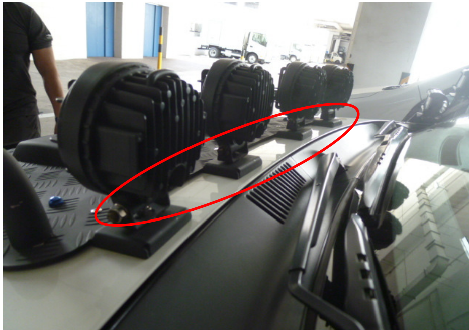
Photo 12 shows the spot lamps additionally fitted onto the front bonnet of the Insured Vehicle upon our inspection. However upon closer inspection, we observed that the spot lamps were not connected (circled).
