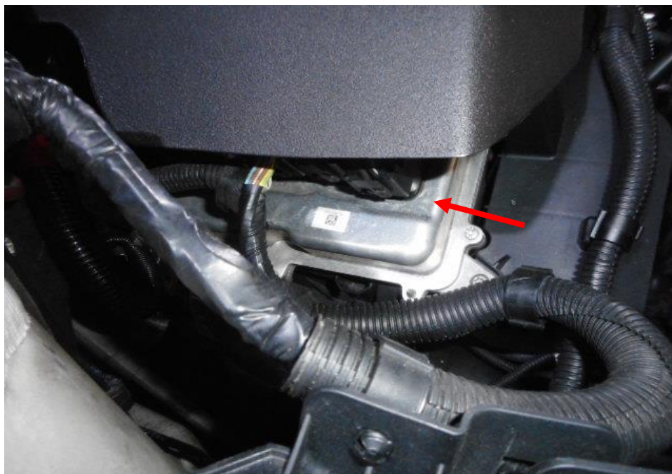
Photo 5 shows the general view of the vehicle electrical control unit (ECU) (arrowed) in the engine compartment portion which was mounted onto the engine of the Insured Vehicle at the time of our inspection. The vehicle electrical control unit is observed to be unaffected and by any signs of accident.
