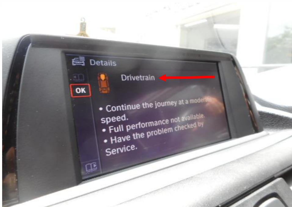
Photo 6 shows the conducted ECU diagnosis of the Insured Vehicle at the time of our inspection. There was an engine drivetrain error (arrowed) on the Insured Vehicle and the engine was not producing sufficient engine power during our test drive.
