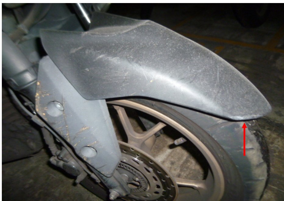
Photo 6 shows a closer view of the grazed front mudguard which was amongst the body parts at the front body of the Motorcycle that had sustained damage as a result of the accident (arrowed).
