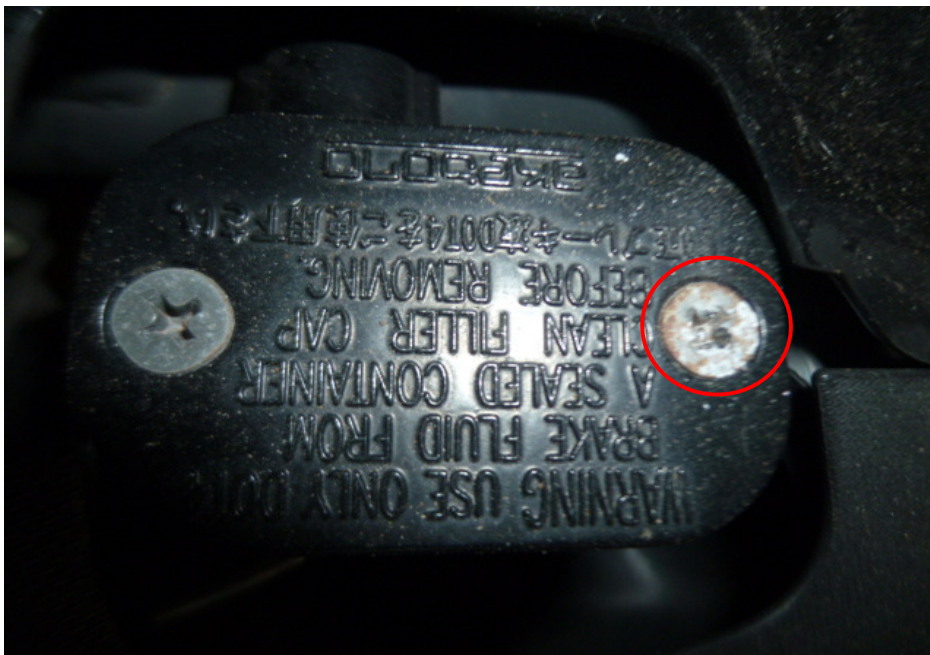
Photo 27 shows the brake fluid reservoir cover for the front brake of the Motorcycle. We were unable to examine whether the front brake fluid was without contamination due to a worn out screw (circled).
