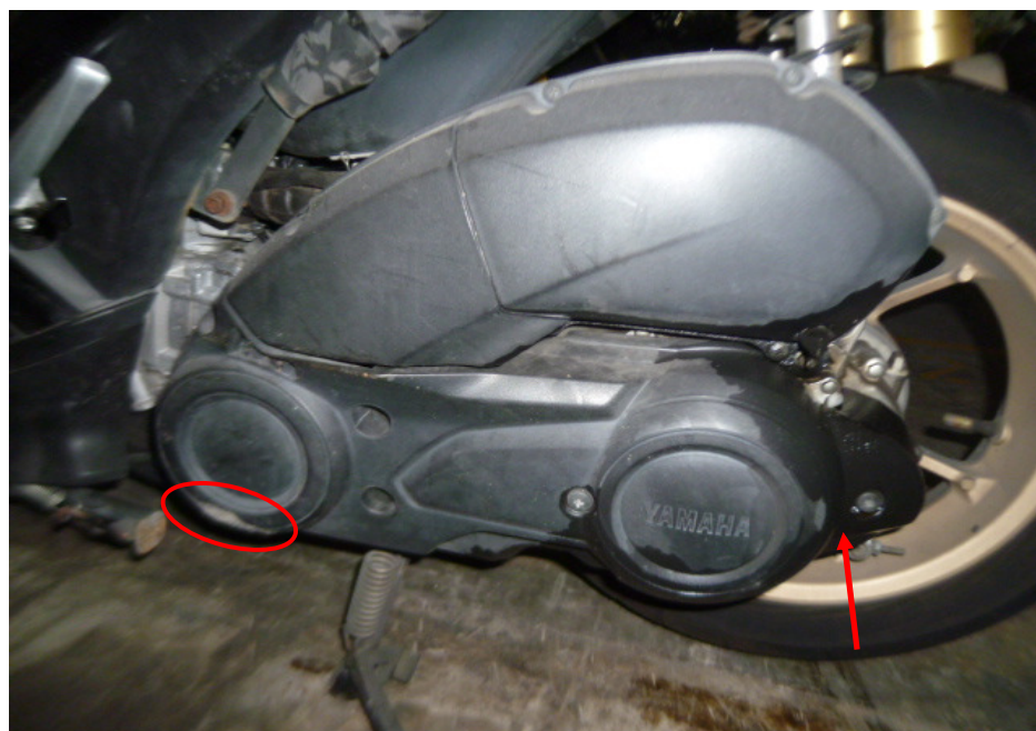
Photo 19 shows the drive train of the Motorcycle which was found to be intact without any misalignment. However the drive train cover had sustained damages of grazing nature as a result of the accident (circled). Upon closer examination of the Motorcycle's left engine area, we had observed fluid leak around the left engine area of the Motorcycle (arrowed).
