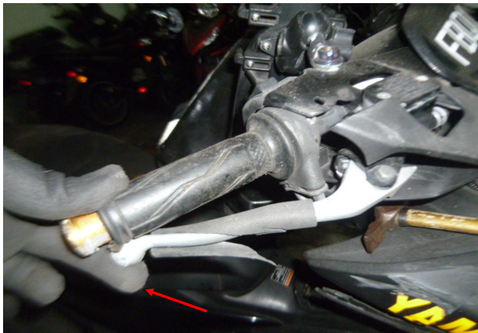
Photo 29 shows the broken right hand brake lever as a result of the accident (arrowed). We were unable to conduct static brake tests on the front braking system of the Motorcycle due to the broken right hand lever. Hence we were unable to indicate if there was any leakage of pressure/vacuum in the front brake system.
