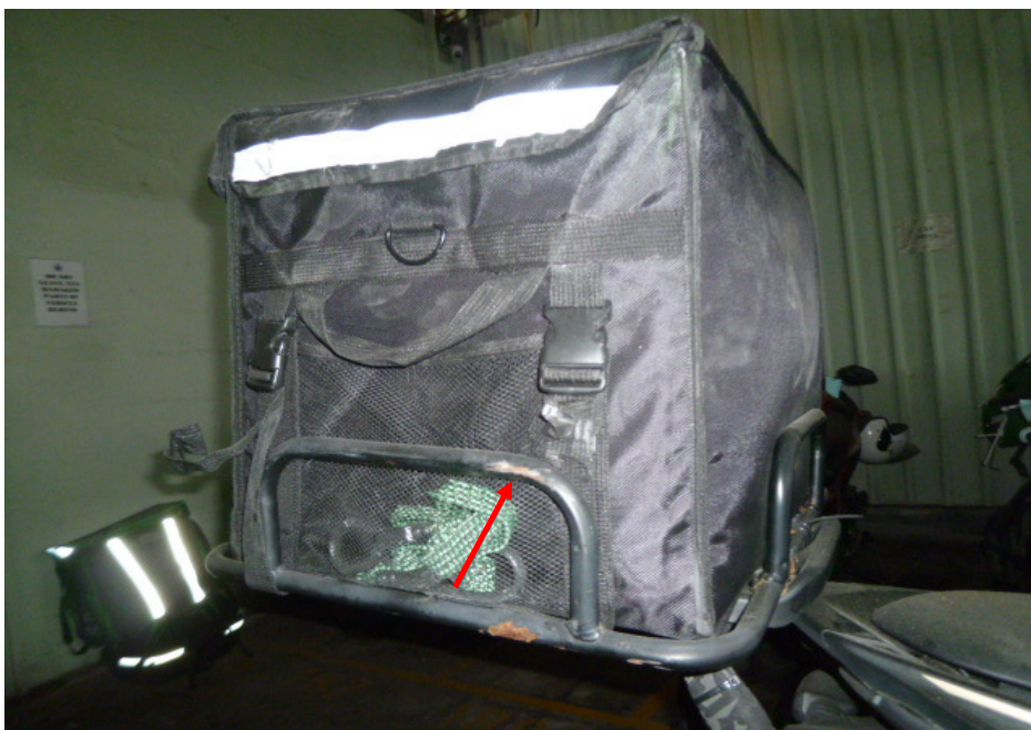
Photo 14 shows the grazed top box rack of the Motorcycle as a result of the accident (arrowed).
