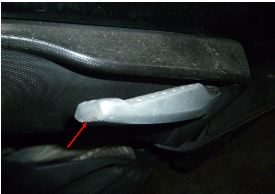
Photo 13 shows a general view of the grazed right pillion foot peg of the Motorcycle as a result of the accident (arrowed).
