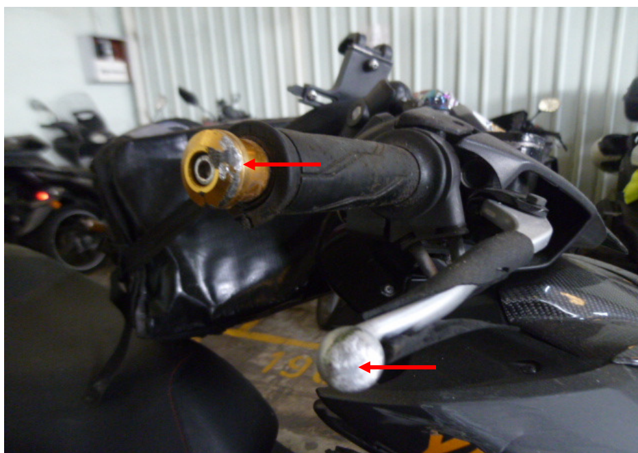
Photo 8 shows a closer view of the right handlebar end and front brake lever of the Motorcycle which were observed to be damaged due to the accident (arrowed).
