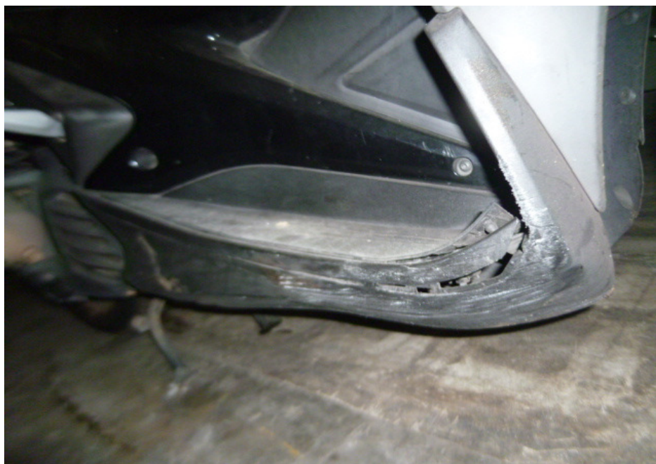
Photo 12 shows a close-up view of the cracked right bottom cowling of the Motorcycle as a result of the accident.
