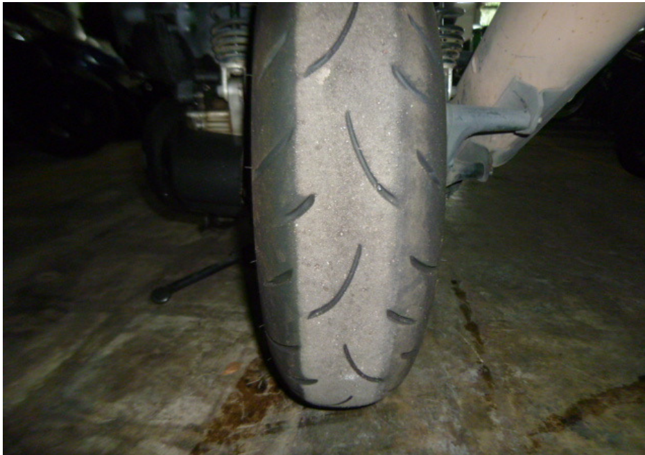
Photo 17 shows the condition of the Motorcycle's rear tyre. The rear tyre was observed to be in serviceable condition with remaining tread depth of approximately 2mm. The tyre was also observed to be sufficiently inflated for vehicular operation. We did not observe any tear, burst mark(s) and/or punctured hole(s) on the sidewalls as well as across the tread of the rear tyre.
