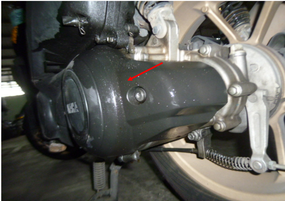
Photo 20 shows the fluid leak observed around the left engine area of the Motorcycle (arrowed).
