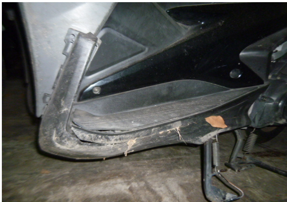
Photo 11 shows a close-up view of the cracked left bottom cowling of the Motorcycle as a result of the accident.
