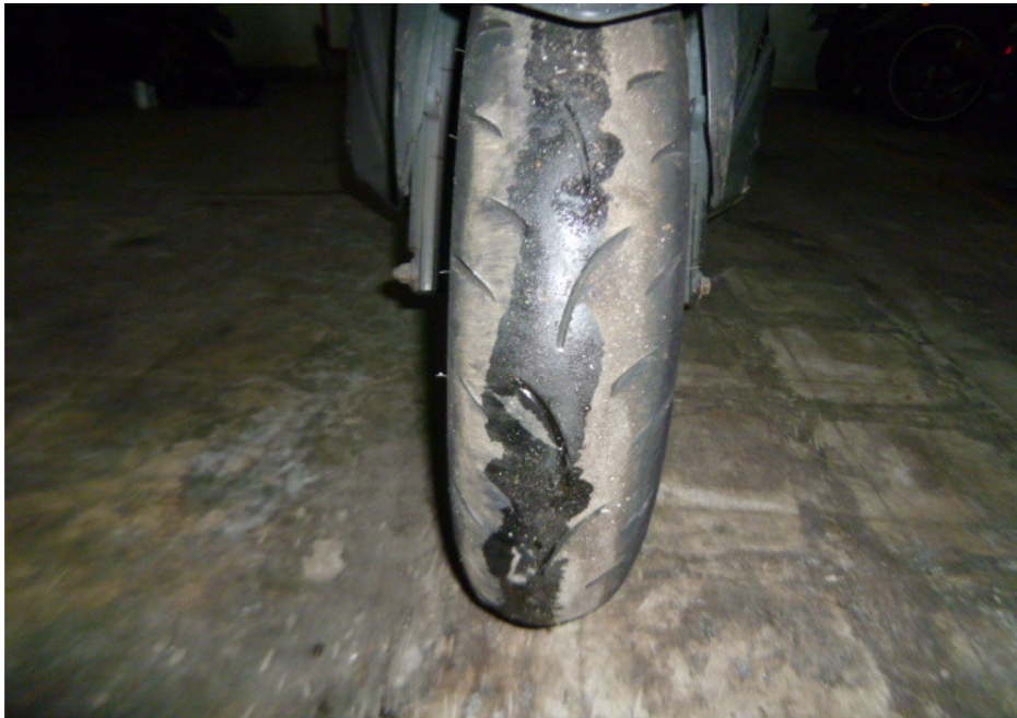
Photo 16 shows the condition of the Motorcycle's front tyre. The front tyre was observed to be in serviceable condition with remaining tread depth of approximately 3mm. There was no tear, burst mark(s) and/or punctured hole(s) on the sidewalls as well as across the tread of the front tyre. The tyre was also observed to be sufficiently inflated for vehicular operation.
