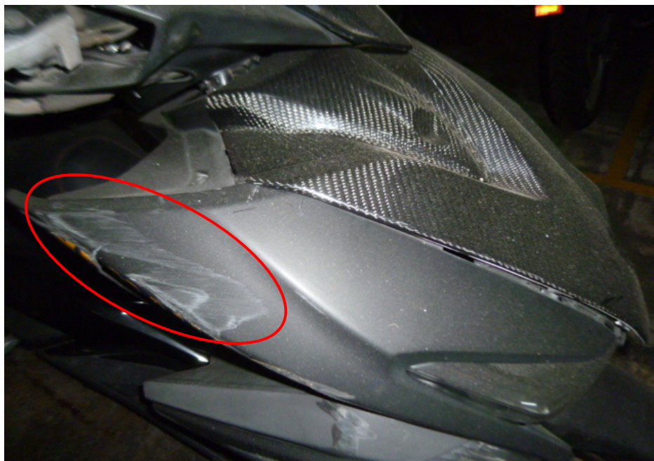
Photo 5 shows the grazed front cowling of the Motorcycle as a result of the accident (circled).
