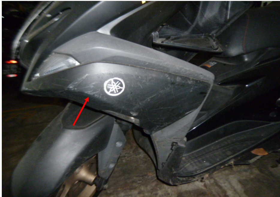
Photo 9 shows the grazed left cowling of the Motorcycle as a result of the accident (arrowed).
