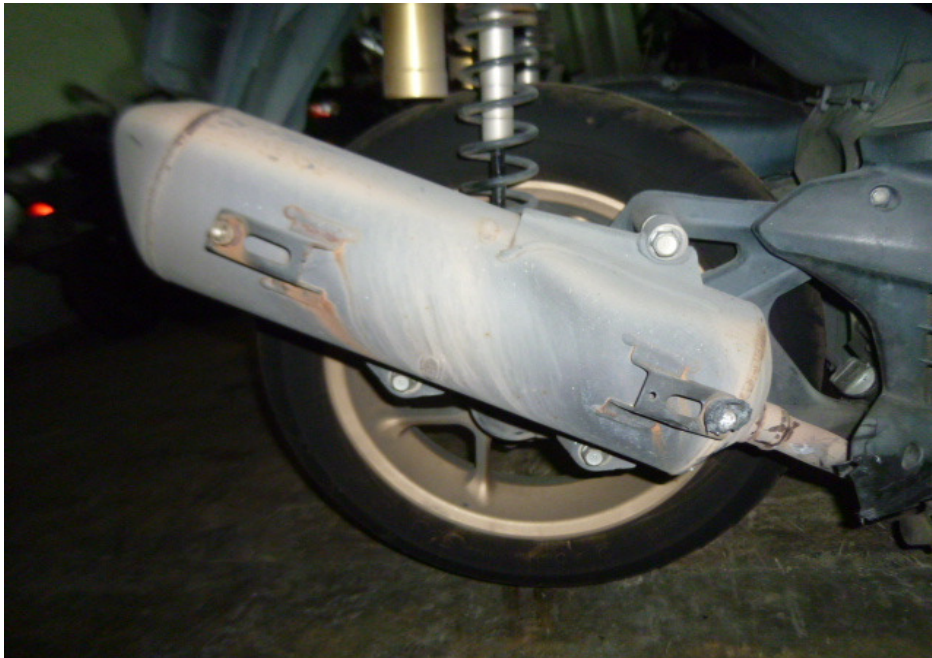
Photo 15 shows a closer view of the deformed exhaust muffler of the Motorcycle as a result of the accident.
