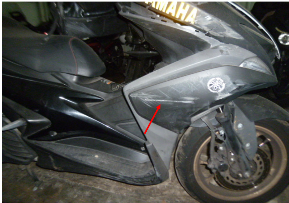
Photo 10 shows the grazed right cowling of the Motorcycle as a result of the accident (arrowed).
