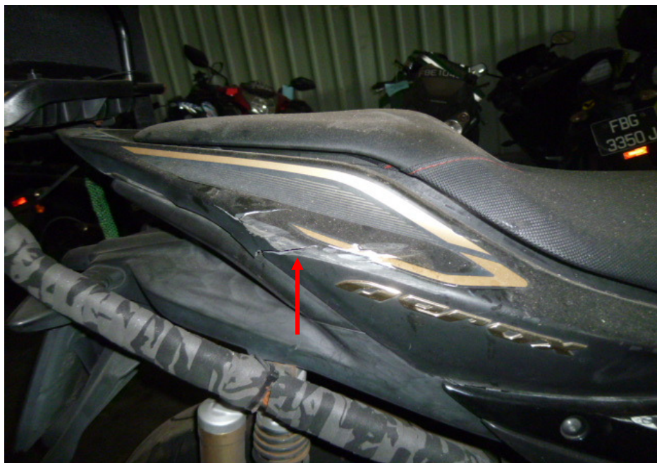
Photo 7 shows a closer view of the cracked right rear side cover of the Motorcycle as a result of the accident (arrowed).
