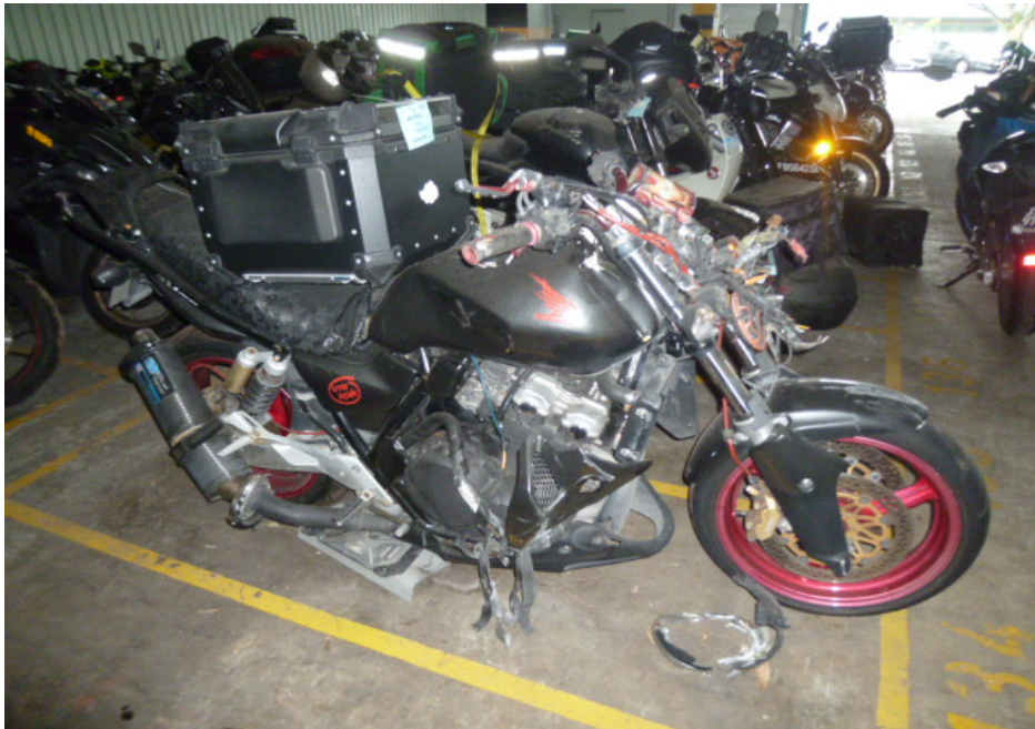
Photo 3 shows a general view of the right body of the Motorcycle at the time of our inspection. The Motorcycle was observed to have sustained damages all around. The body parts that were found to have been damaged include its speedometer gauge, headlight assembly, front forks, front mudguard, handlebar, radiator covers, petrol tank, top box rack, rear number plate and exhaust muffler, amongst others.
