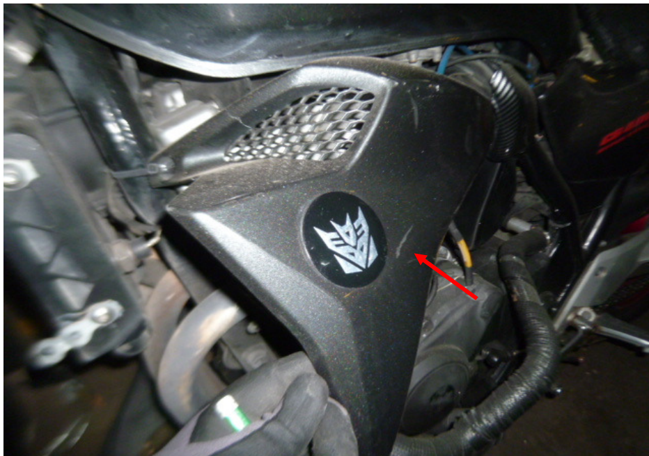
Photo 8 shows the left radiator cover of the Motorcycle that had sustained damages of grazing nature as a result of the accident (arrowed).
