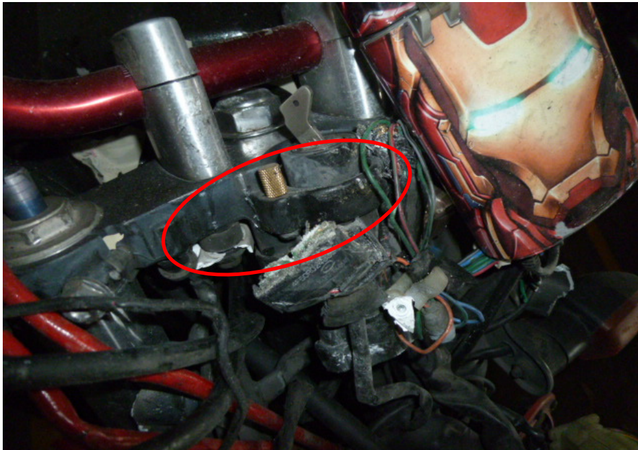
Photo 1 shows the mileage of the Motorcycle could not be recorded at the time of our inspection due to a missing speedometer gauge as a result of the accident (circled).
