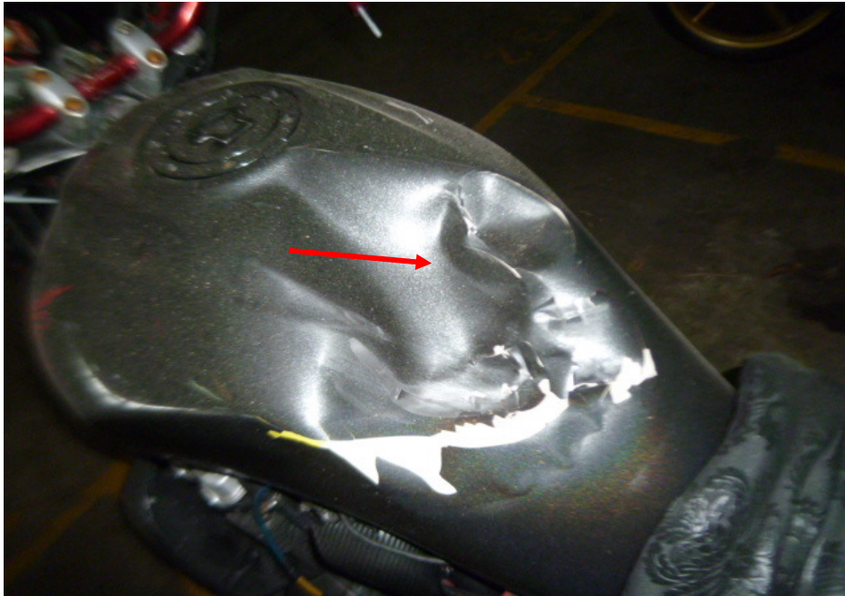
Photo 9 shows a closer view of the petrol tank, which was amongst the body parts of the Motorcycle that had sustained damage as a result of the accident (arrowed).
