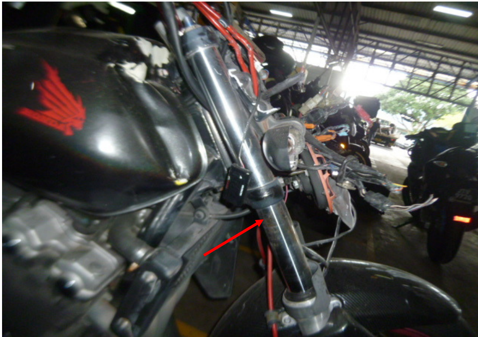
Photo 20 shows the front forks of the Motorcycle. The right front fork was observed to be bent as a result of the accident (arrowed). We were hence not able to conduct any tests on the steering system of the Motorcycle.
