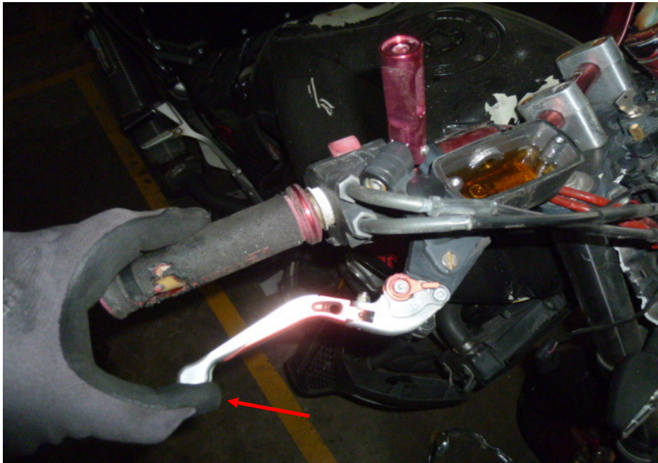
Photo 24 shows the front brake lever being depressed. There was some resistance felt (spongy like feel) upon pressing the front brake lever (arrowed). This would indicate that there is no leakage of pressure/vacuum in the front brake system.
