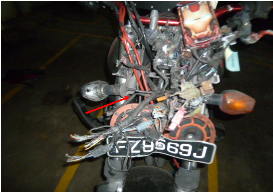
Photo 4 shows a closer view of the missing headlight assembly (arrowed) of the Motorcycle as a result of the accident.
