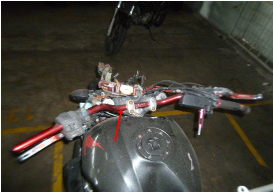
Photo 6 shows a closer view of the bent handlebar (arrowed) which was amongst the body parts at the front body of the Motorcycle that had sustained damage as a result of the accident.
