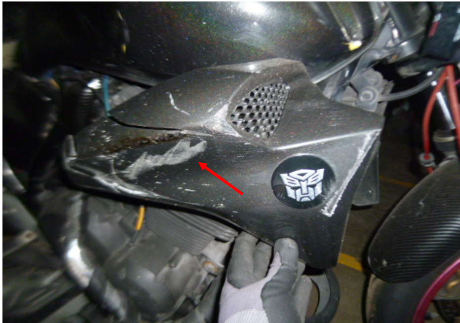
Photo 7 shows the right radiator cover of the Motorcycle that had sustained damages of grazing nature as a result of the accident (arrowed).
