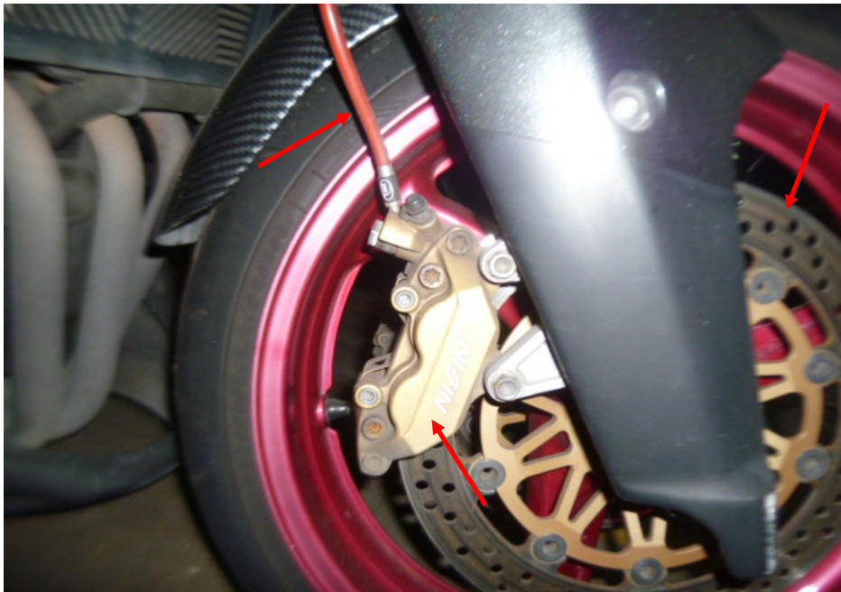
Photo 21 shows a close up view of the front brake caliper, front brake disc and front brake hose (arrowed) at the right side of the Motorcycle's front wheel, which are all part of the components in the hydraulic front brake system of the Motorcycle. Our visual checks of these various components had revealed all to be intact with no visible damage. No leakage of brake fluid was also observed.
