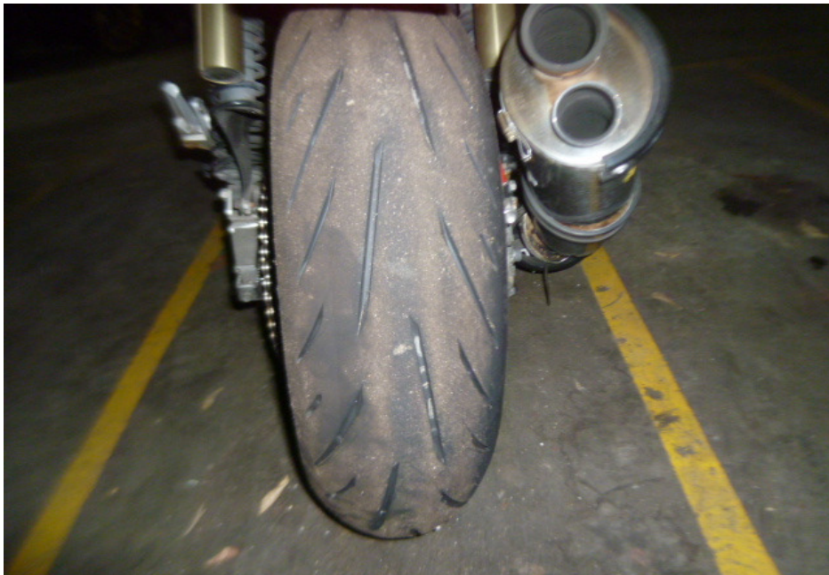
Photo 14 shows the condition of the Motorcycle's rear tyre. The rear tyre was observed to be in serviceable condition with remaining tread depth of approximately 6mm. We did not observe any tear, burst mark(s) and/or punctured hole(s) on the sidewalls as well as across the tread of the rear tyre. However the rear tyre was also observed to be deflated.
