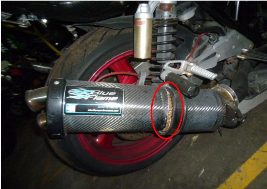
Photo 11 shows the exhaust muffler (circled) which was amongst the body parts of the Motorcycle that had sustained damage as a result of the accident.
