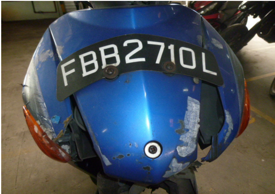
Photo 5 shows a closer view of the front cowl which was amongst the body parts of the Motorcycle that had sustained damage as a result of the accident.
