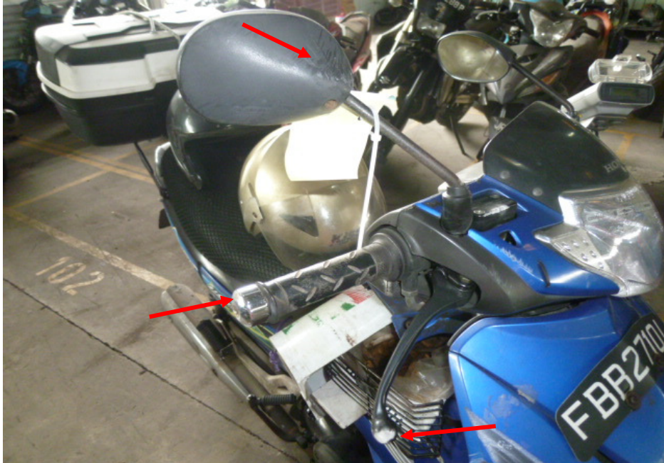
Photo 7 shows the right handlebar end, front brake lever and right side mirror (arrowed), which were amongst the body parts of the Motorcycle that had sustained damage as a result of the accident.
