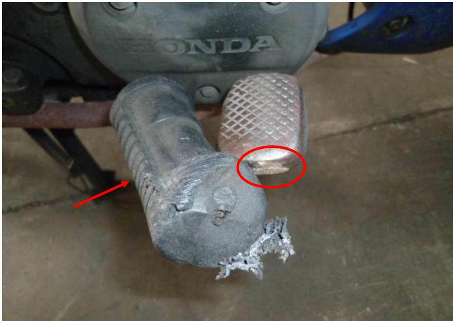
Photo 10 shows the grazed rear brake pedal (circled) and bent left front footrest (arrowed) of the Motorcycle as a result of the accident
