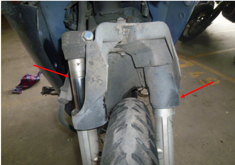
Photo 19 shows the front fork assembly of the Motorcycle. The front forks were observed to be bent (arrowed) as a result of the accident. We were hence not able to conduct any tests on the steering system of the Motorcycle.
