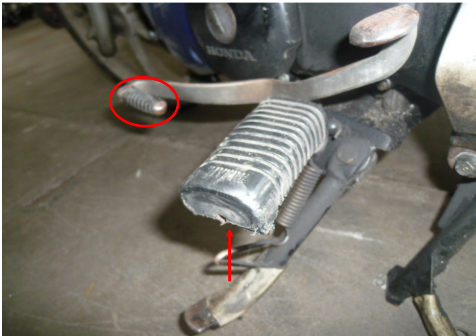
Photo 11 shows the grazed left front footrest (arrowed) and bent gear shift pedal (circled) of the Motorcycle as a result of the accident
