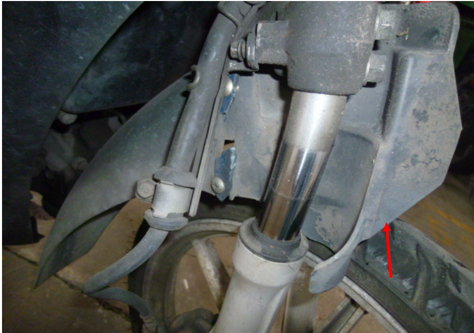
Photo 6 shows the cracked front mudguard (arrowed) of the Motorcycle as a result of the accident.
