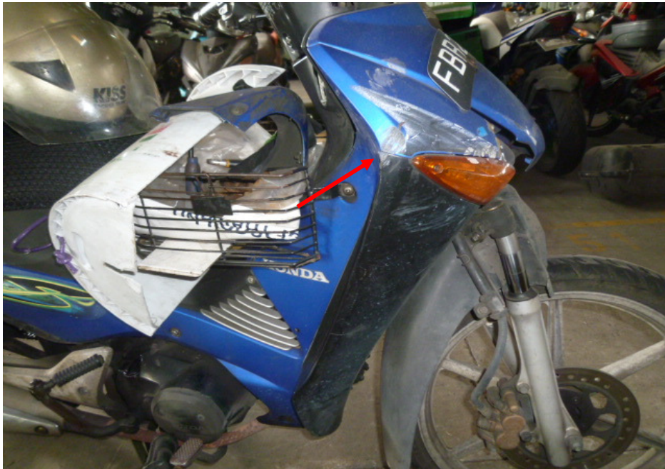
Photo 8 shows a closer view of the right cowling (arrowed) which was amongst the body parts of the Motorcycle that had sustained damage as a result of the accident.
