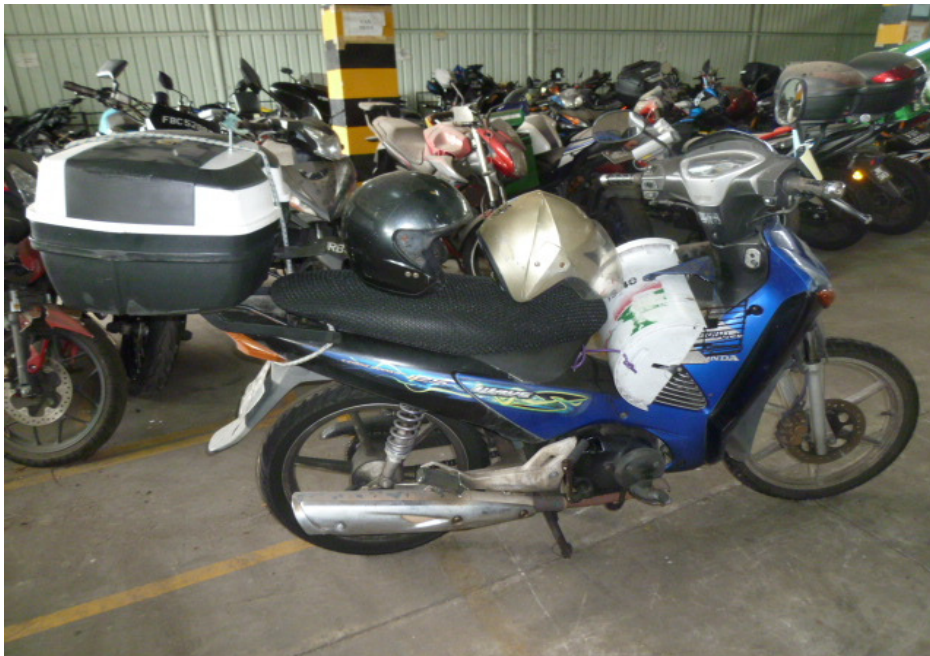
Photo 3 shows a general view of the right body of the Motorcycle at the time of our inspection. The Motorcycle was observed to have sustained damages all around. The body parts that were found to have been damaged include its headlight, head cowl, front cowl, side cowlings, right side mirror, right handlebar end, front brake lever, left front footrest and top box, amongst others.
