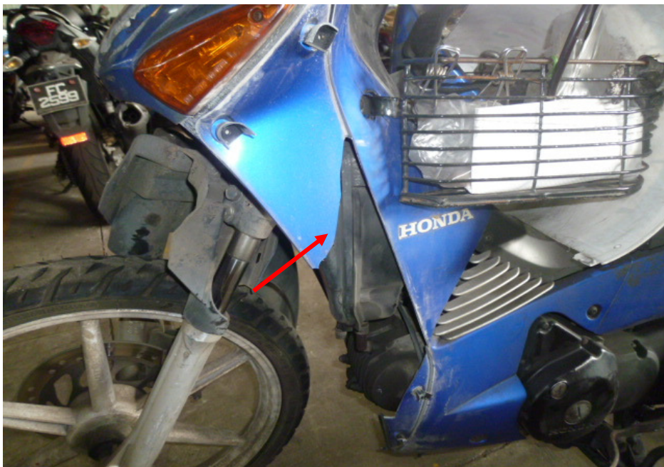
Photo 9 shows the left cowling (arrowed), which were amongst the body parts of the Motorcycle that had sustained damage as a result of the accident.
