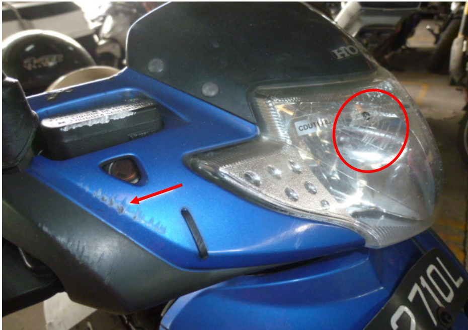
Photo 4 shows a closer view of headlight (circled) and head cowl (arrowed) which were amongst the body parts of the Motorcycle that had sustained damages of grazing nature as a result of the accident (circled).
