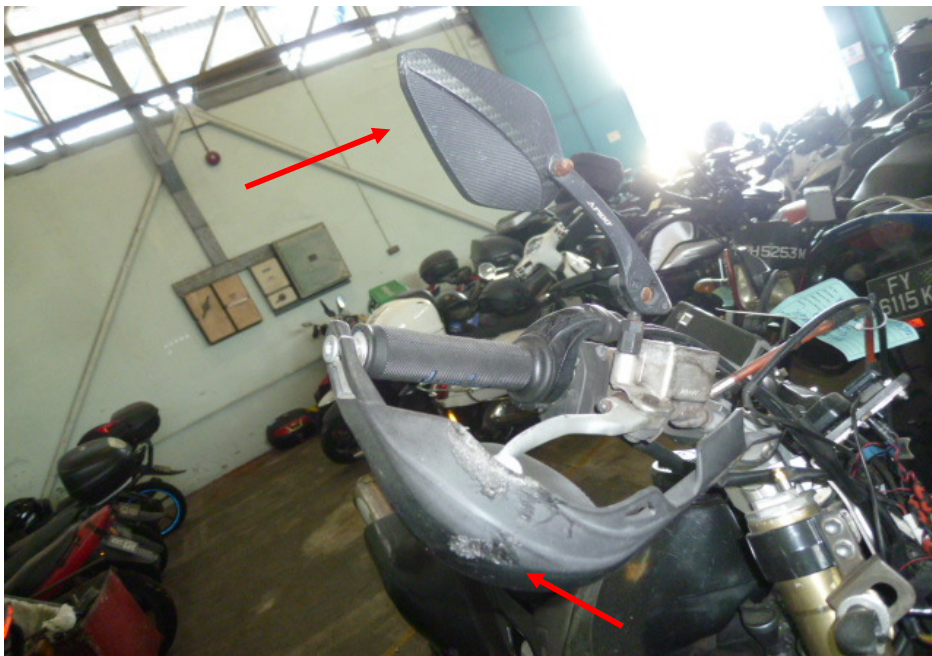
Photo 9 shows the right side mirror and front brake lever guard (arrowed), which were amongst the body parts of the Motorcycle that had sustained damage as a result of the accident.
