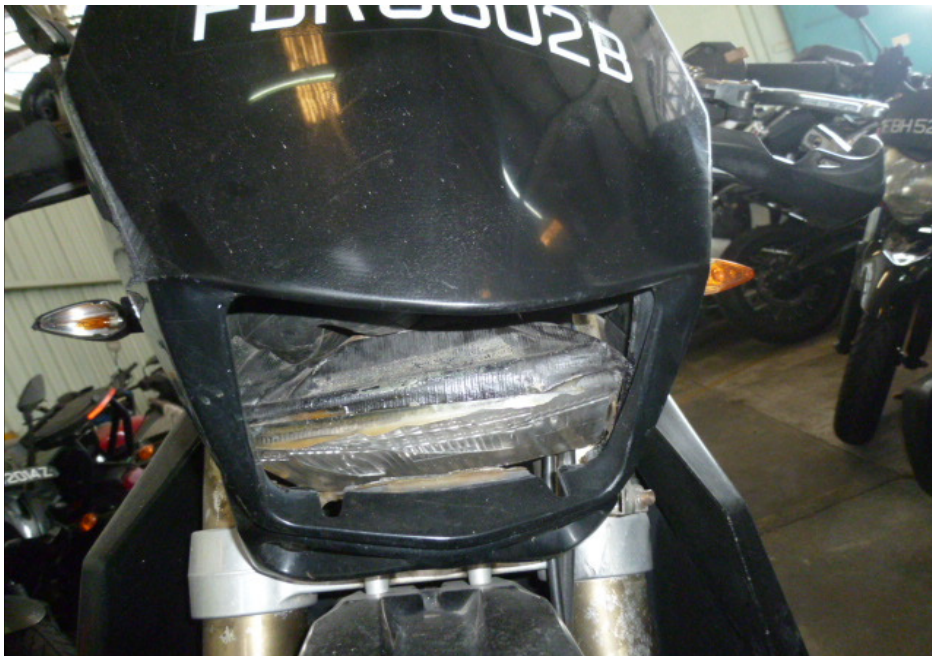
Photo 5 shows a close up view of the headlight assembly which was amongst the body parts of the Motorcycle that had sustained damage as a result of the accident.
