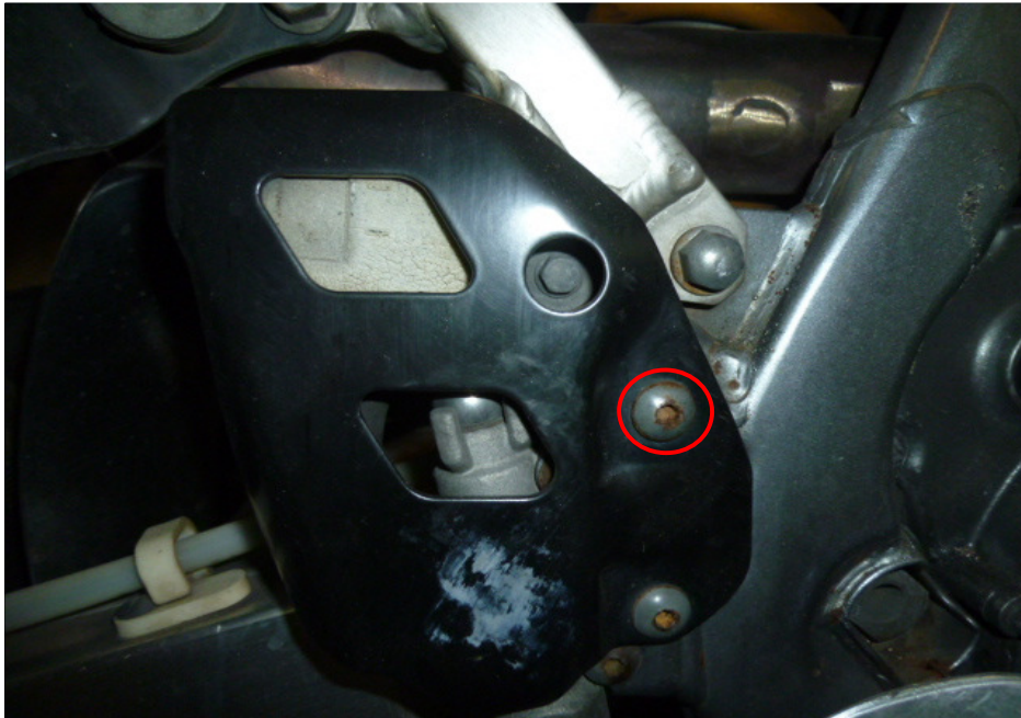
Photo 26 shows the brake fluid reservoir cover for the rear brake of the Motorcycle. We were unable to remove the right heel guard to examine whether the rear brake fluid was of sufficient level for operational purposes and without contamination due to a worn out screw (circled).
