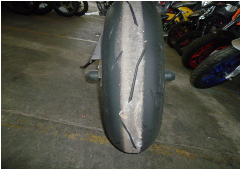
Photo 14 shows the condition of the Motorcycle's rear tyre. The rear tyre was observed to be in serviceable condition with remaining tread depth of approximately 5mm. The tyre was also observed to be sufficiently inflated for vehicular operation. We did not observe any tear, burst mark(s) and/or punctured hole(s) on the sidewalls as well as across the tread of the rear tyre.
