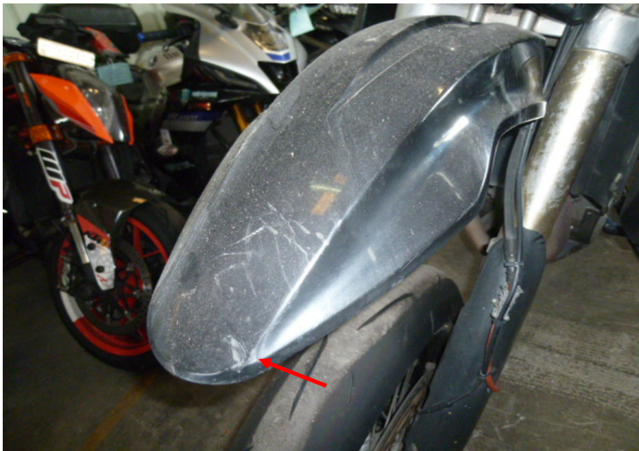
Photo 7 shows a closer view of the front mudguard (arrowed) which was amongst the body parts at the front body of the Motorcycle that had sustained damage as a result of the accident.
