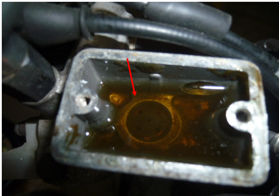
Photo 22 shows a close up view of the brake fluid reservoir for the front brake of the Motorcycle. The front brake fluid was observed to be of sufficient level for operational purposes. However it was found to be slightly contaminated (arrowed).
