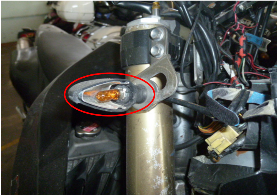
Photo 6 shows the broken left front signal lamp (circled) of the Motorcycle as a result of the accident.
