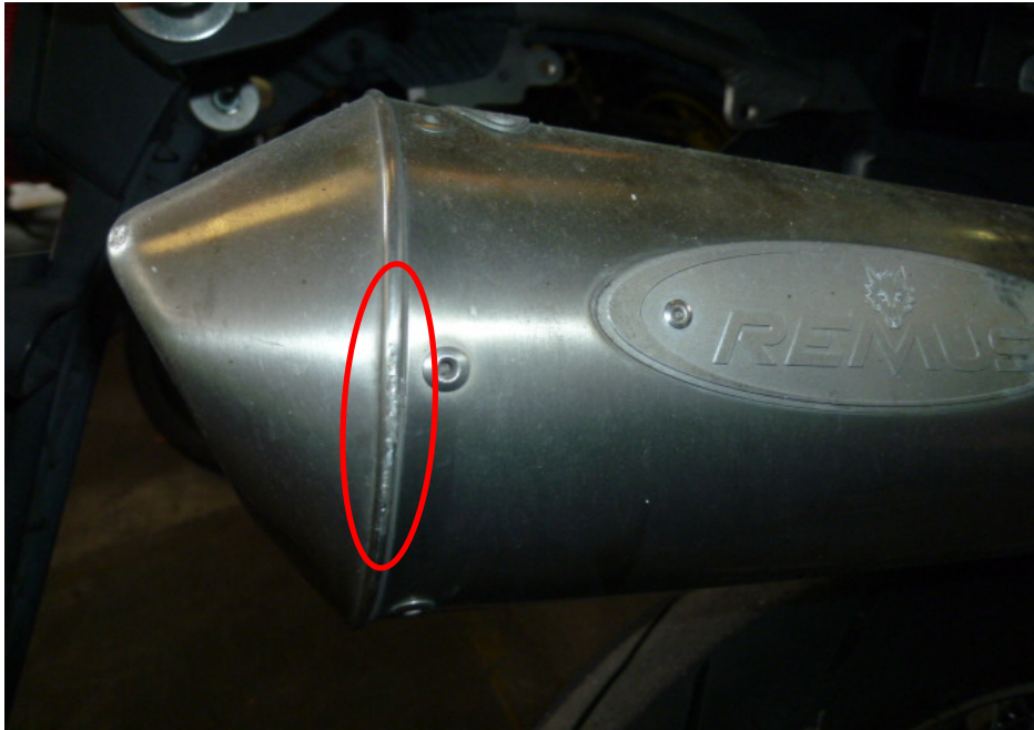
Photo 12 shows the exhaust muffler which was amongst the body parts of the Motorcycle that had sustained damage as a result of the accident (circled).
