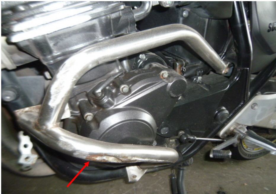
Photo 7 shows the grazed left engine crashbar of the Motorcycle as a result of the accident (arrowed).
