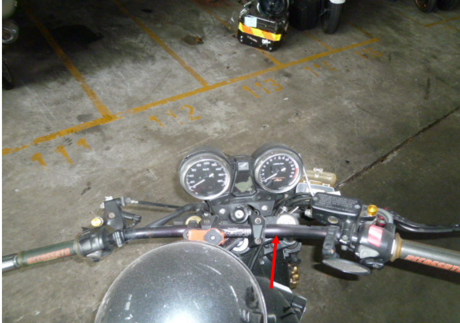
Photo 8 shows the bent handlebar of the Motorcycle as a result of the accident (arrowed).
