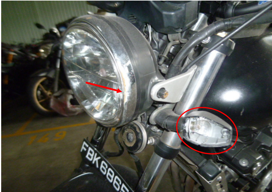
Photo 4 shows a closer view of the grazed headlight cover (arrowed) and broken left front signal lamp (circled) of the Motorcycle as a result of the accident.
