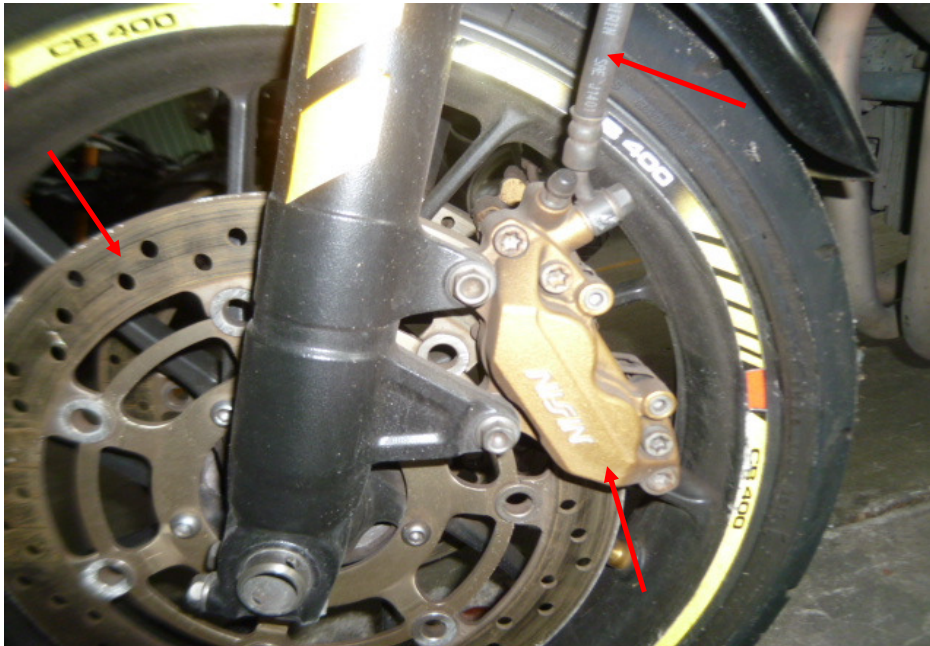
Photo 24 shows a close up view of the front brake caliper, front brake disc and front brake hose (arrowed) at the left side of the Motorcycle's front wheel, which are all part of the components in the hydraulic front brake system of the Motorcycle. Our visual checks of these various components had revealed all to be intact with no visible damage. No leakage of brake fluid was also observed.
