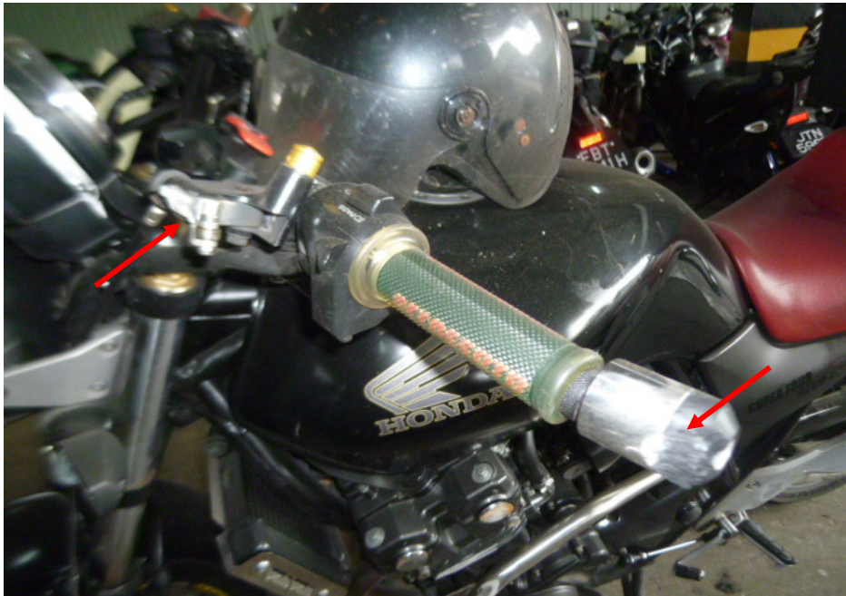
Photo 6 shows a closer view of the clutch lever and left handlebar end (arrowed) which were amongst the body parts at the front body of the Motorcycle that had sustained damage as a result of the accident.
