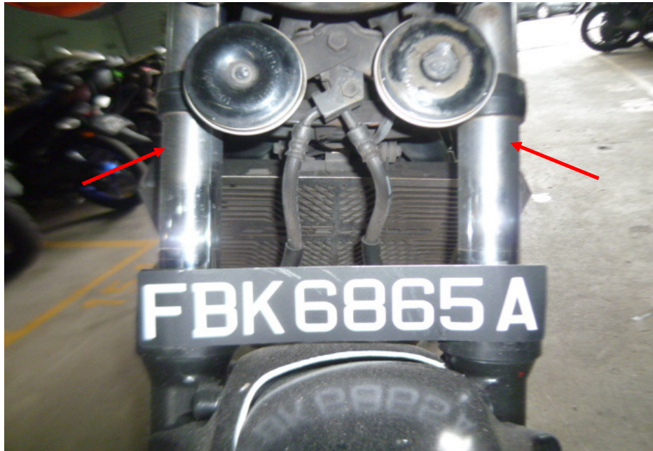
Photo 20 shows the front forks (arrowed) of the Motorcycle. The front forks and fork bracket of the Motorcycle were both found to be intact and undamaged. Turning the Motorcycle's handle bar towards the left and right did not produce any abnormal free play and/or resistance. The steering system of the Motorcycle was in serviceable condition at the time of our inspection.
