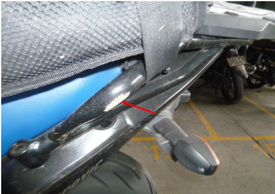
Photo 12 shows a closer view of the left pillion grab rail (arrowed) which was amongst the body parts at the rear body of the Motorcycle that had sustained damage as a result of the accident.
