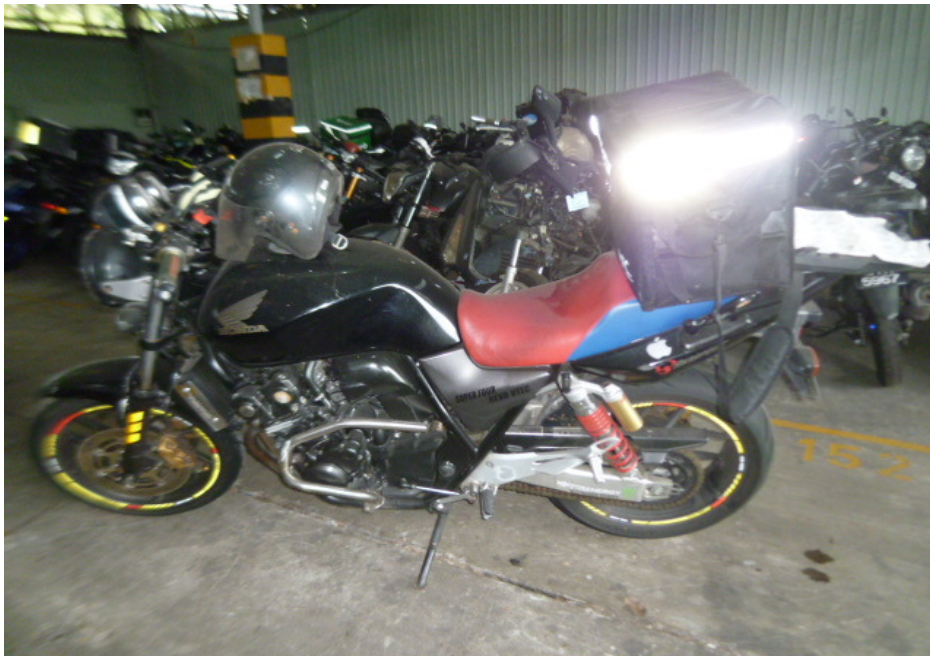
Photo 3 shows a general view of the left body of the Motorcycle at the time of our inspection. The Motorcycle was observed to have sustained damages at its frontal portion and left body. The body parts that were found to have been damaged include its headlight cover, handlebar and gear shift pedal, amongst others.
