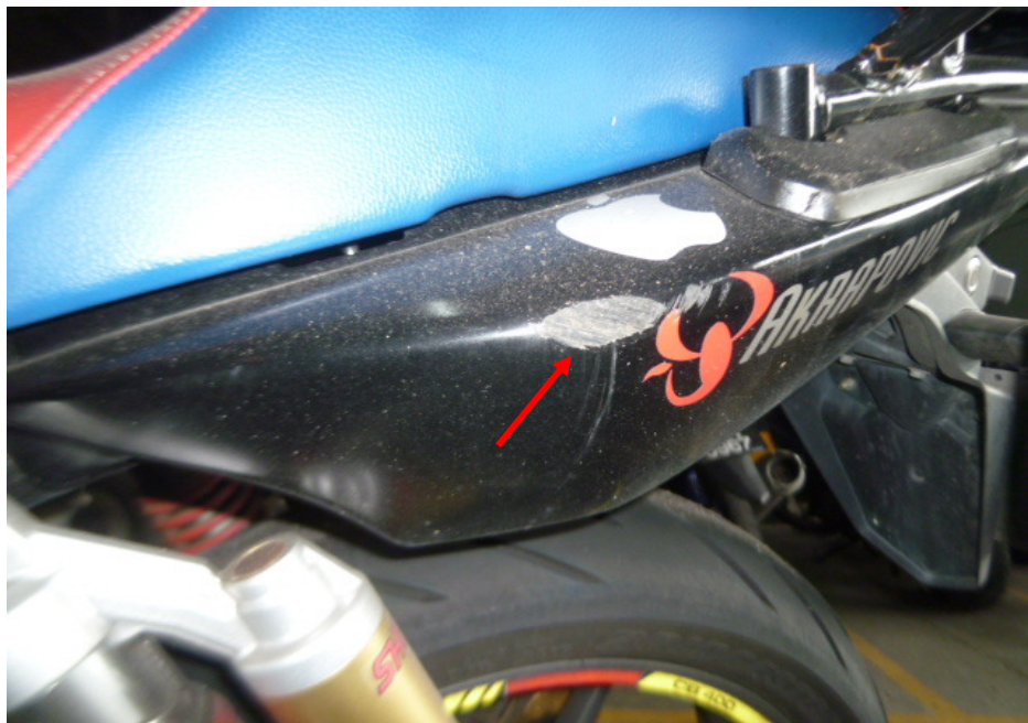
Photo 11 shows the grazed left rear side cover (arrowed) of the Motorcycle as a result of the accident.
