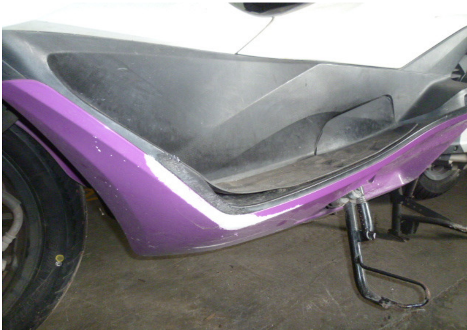
Photo 8 shows a close-up view of the left lower side cowling of the Motorcycle at the time of our inspection. The damage sustained was mainly of grazing nature.
