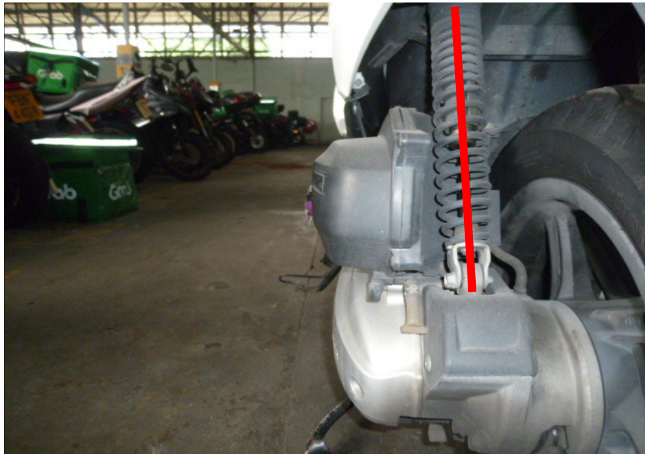
Photo 16 shows the left shock absorber of the Motorcycle which was found to be intact without any misalignment.
