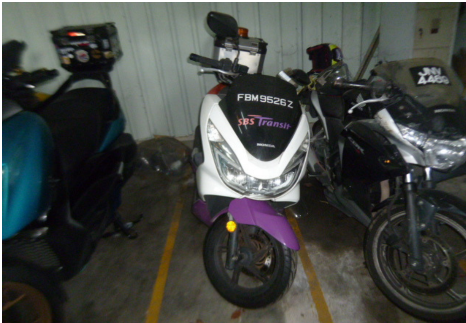
Photo 19 shows the front wheel of the Motorcycle turned towards its full left. Turning the Motorcycle's handle bar towards the left and right did not produce any abnormal free play and/or resistance. This would indicate that the steering system of the Motorcycle was in serviceable condition at the time of our inspection.
