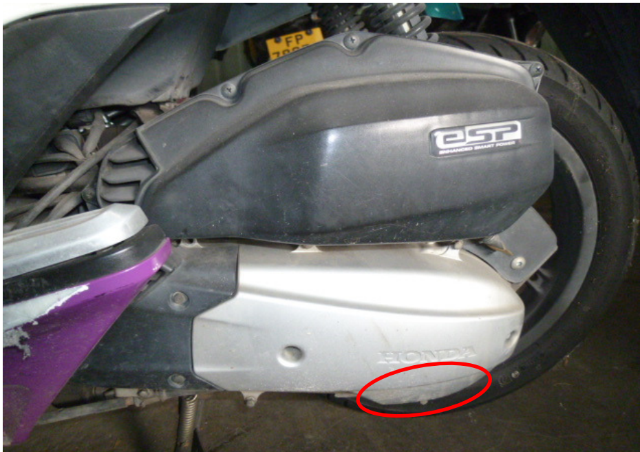
Photo 15 shows the drive train of the Motorcycle which was found to be intact without any misalignment. However the drive train cover had sustained damages of grazing nature as a result of the accident (circled). Upon examination of the Motorcycle's engine area, we had observed that the various engine related parts and components were intact with no visible damage. There was also no sign(s) or indication(s) of fluid leak observed around the engine area of the Motorcycle.
