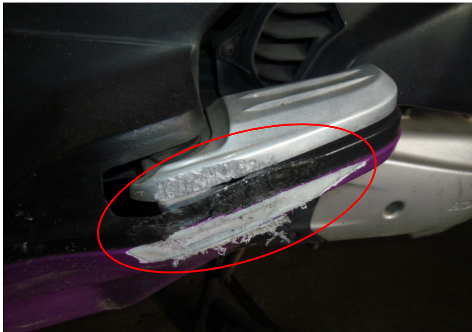
Photo 10 shows a closer view of the damaged left pillion footpeg and left rear bottom cowling of the Motorcycle at the time of our inspection (circled).
