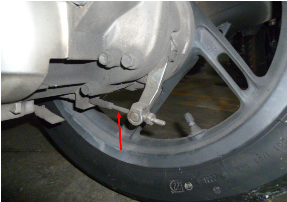
Photo 24 shows the rear wheel of the Motorcycle. The type of brake system for the rear wheel was of a mechanical type, controlled by the brake foot pedal of the Motorcycle. Our checks of the cable (arrowed), spring and drum which are all part of the components in the rear brake system of the Motorcycle reveal all to be intact and without damage.
