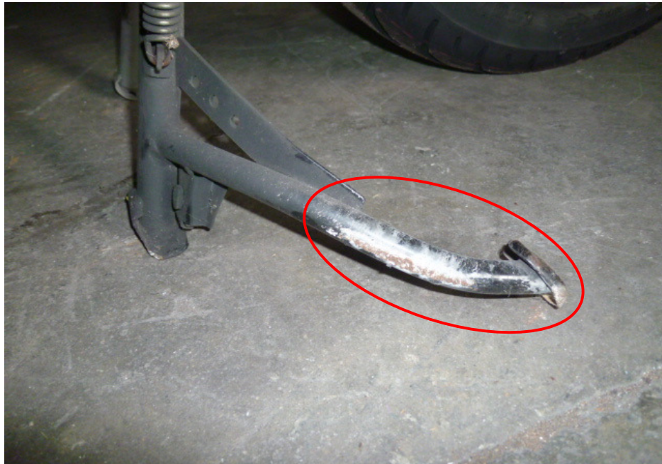
Photo 9 shows a closer view of the grazed main stand of the Motorcycle at the time of our inspection (circled).
