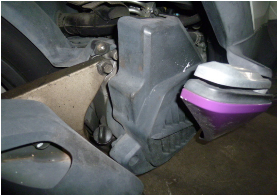
Photo 14 shows the radiator of the Motorcycle at the time of our inspection. The radiator was found to be intact with no visible damage. There was also no sign(s) or indication(s) of fluid leak observed around the radiator of the Motorcycle.
