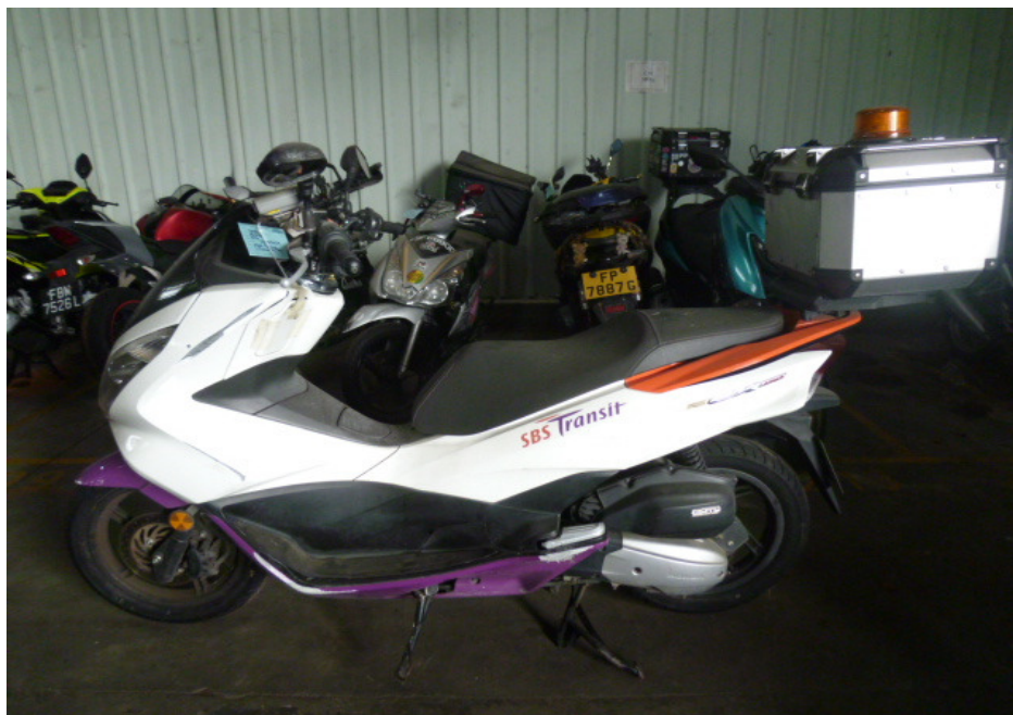
Photo 4 shows a general view of the left body of the Motorcycle at the time of our inspection. The body parts that were found to have been damaged include its front mudguard, rear brake lever, left side mirror, left handlebar end, left side cowl, left rear bottom cowl, main stand, left pillion footpeg and top box, amongst others as a result of the accident.
