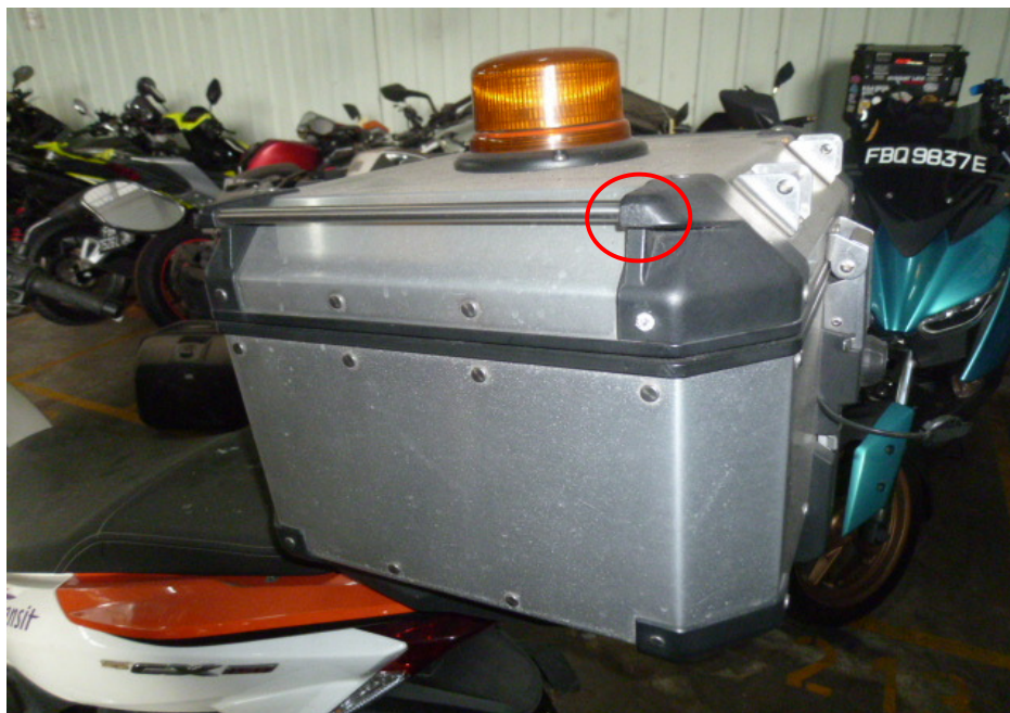
Photo 11 shows a closer view of the top box of the Motorcycle which had sustained damages of grazing nature due to the accident (circled).
