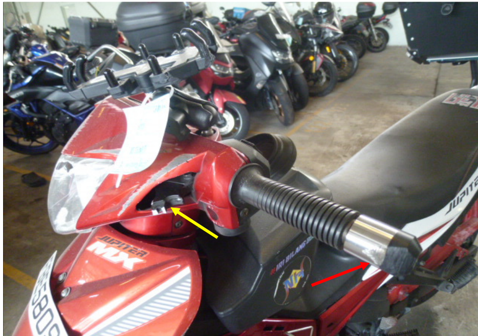
Photo 9 shows a closer view of the clutch lever and left handlebar end of the Motorcycle (arrowed). These parts were amongst the body parts of the Motorcycle which were damaged as a result of the accident.
