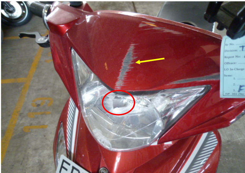
Photo 6 shows a closer view of the cracked headlight assembly (circled) and grazed head cowl (arrowed) of the Motorcycle as a result of the accident.
