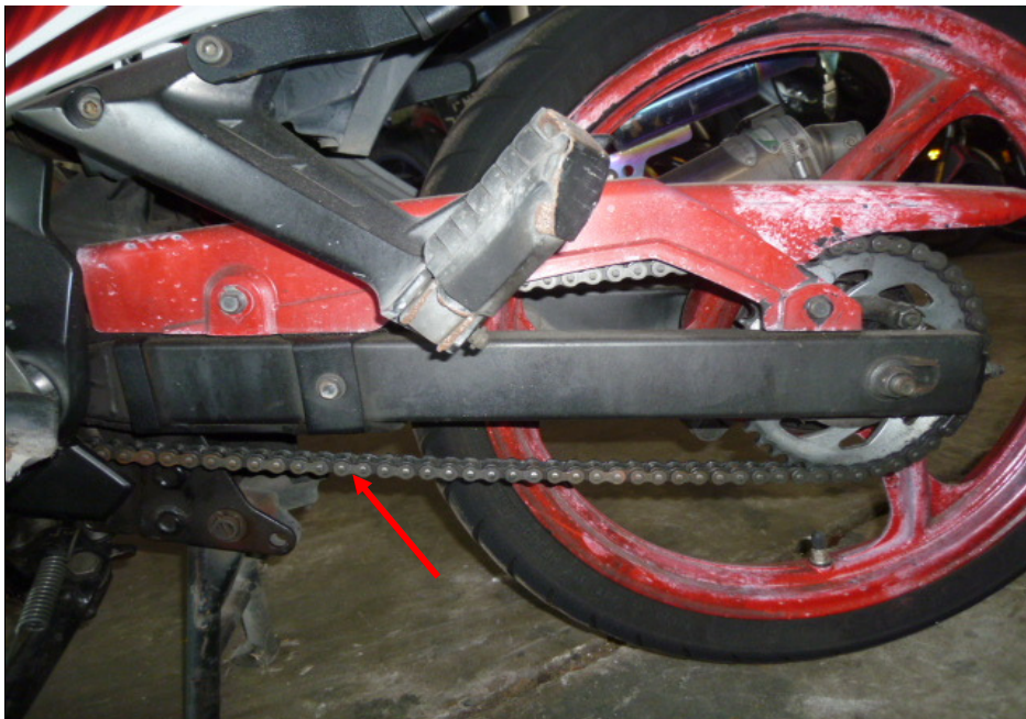
Photo 19 shows the gear train (arrowed) of the Motorcycle, which was observed to be intact with no misalignment. It was also adequately lubricated for operating purposes. The gear train rotates the rear wheel of the Motorcycle.
