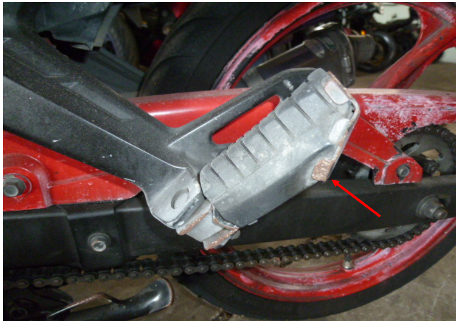
Photo 12 shows a closer view of the left pillion foot peg which was amongst the body parts of the Motorcycle that had sustained damage as a result of the accident (arrowed).
