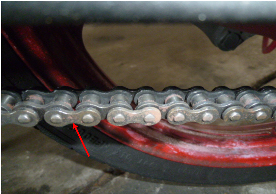
Photo 20 shows the closer view of the gear train (arrowed) of the Motorcycle, which was observed to be intact with no misalignment. It was also adequately lubricated for operating purposes.
