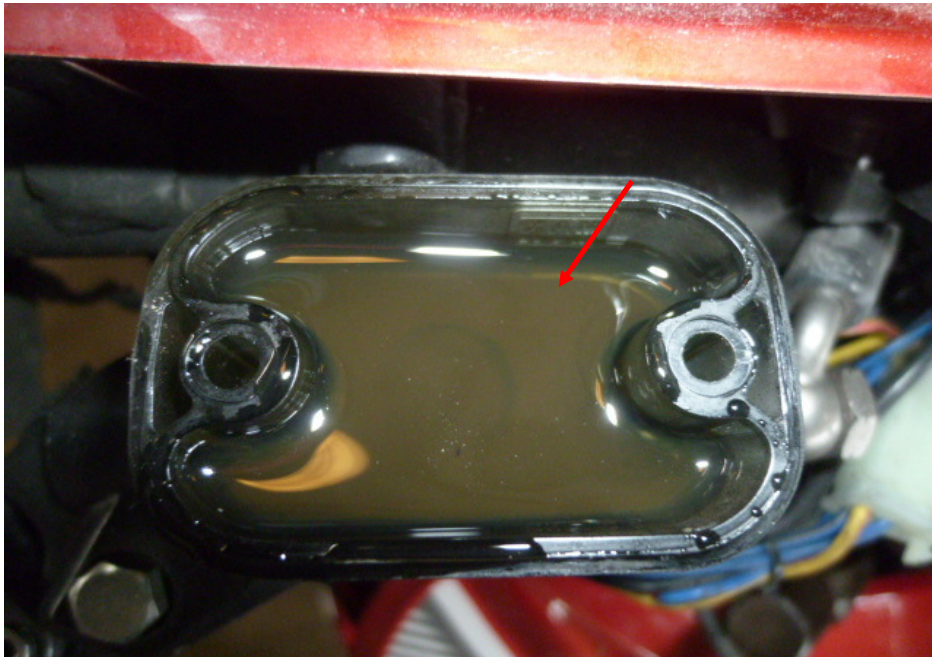
Photo 23 shows the brake fluid reservoir for the front brake of the Motorcycle. The brake fluid was found to be of sufficient level for operating purposes. However the brake fluid was found to be contaminated (arrowed).
