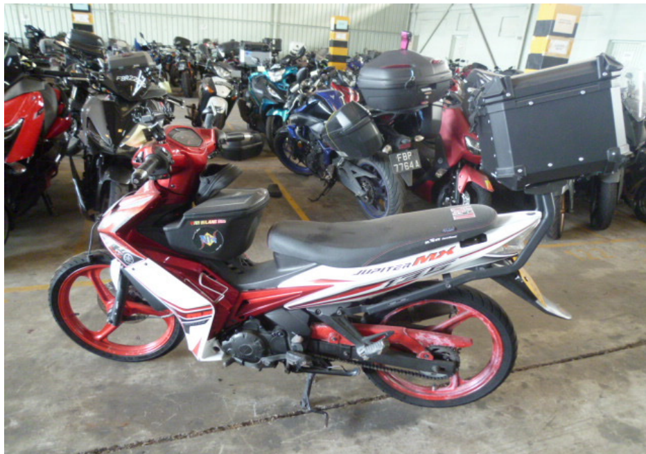
Photo 4 shows a general view of the left body of the Motorcycle at the time of our inspection. The Motorcycle had sustained damages all around. Body parts that were found to have been damaged include its head cowl, headlight assembly, speedometer gauge, front fork assembly, front mudguard, handlebar ends, right side mirror, clutch lever, front brake lever, side cowlings, gear shift pedal, left front footrest, left pillion foot peg, top box rack, top box and rear number plate, amongst others.
