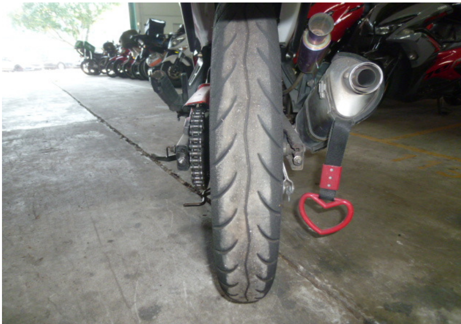
Photo 16 shows the condition of the Motorcycle's rear tyre. The pattern of the tread was clearly visible with remaining tread depth of approximately 1mm. We did not observe any tear, burst mark(s) and/or punctured hole(s) on the sidewalls as well as across the tread of the rear tyre.
