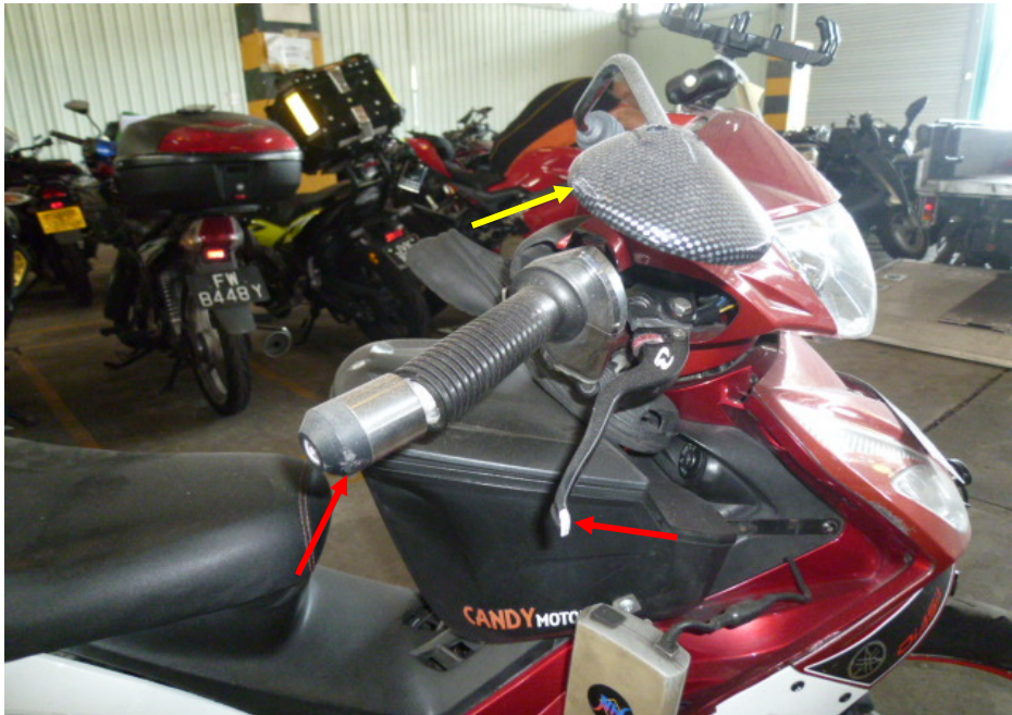
Photo 7 shows a closer view of the right side mirror, front brake lever and right handlebar end of the Motorcycle (arrowed). These parts were amongst the body parts of the Motorcycle which were damaged as a result of the accident.
