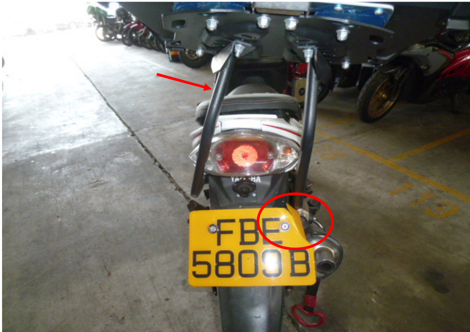
Photo 13 shows the cracked rear number plate (circled) and bent top box rack (arrowed) of the Motorcycle as a result of the accident.
