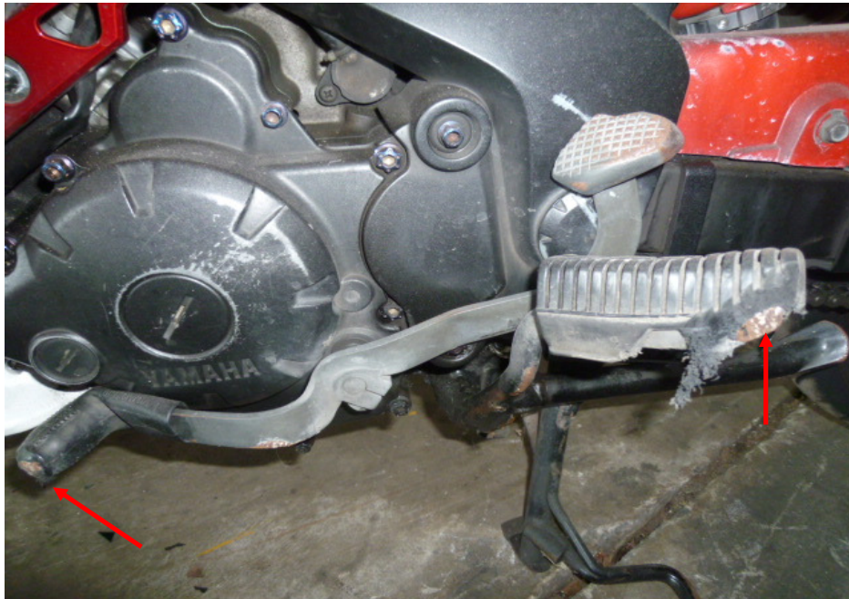
Photo 11 shows the gear shift pedal and left front footrest of the Motorcycle which had sustained damage as a result of the accident (arrowed).
