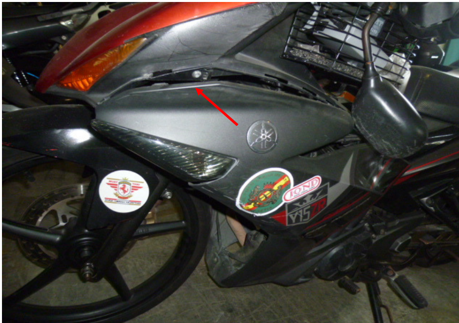
Photo 11 shows a closer view of the cracked left cowling of the Motorcycle as a result of the accident (arrowed).
