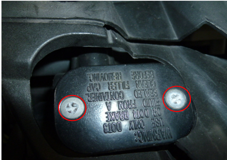
Photo 24 shows the brake fluid reservoir cover for the front brake of the Motorcycle. We were unable to examine whether the front brake fluid was without contamination due to the worn out screws (circled).
