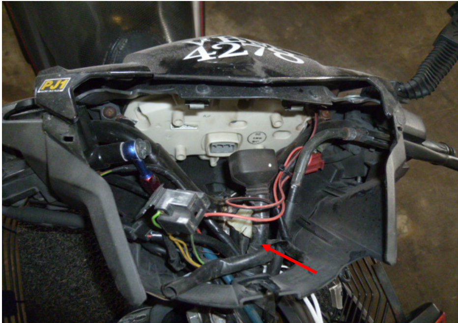
Photo 6 shows the missing headlight assembly (arrowed) of the Motorcycle as a result of the accident.
