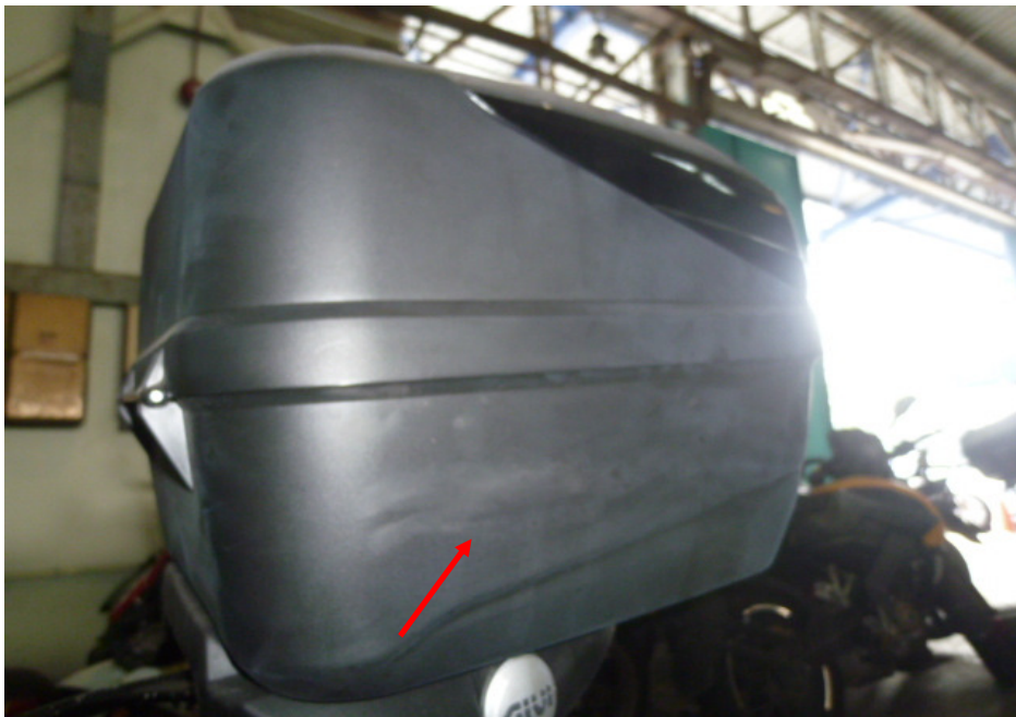
Photo 13 shows grazed top box (arrowed) of the Motorcycle a result of the accident.
