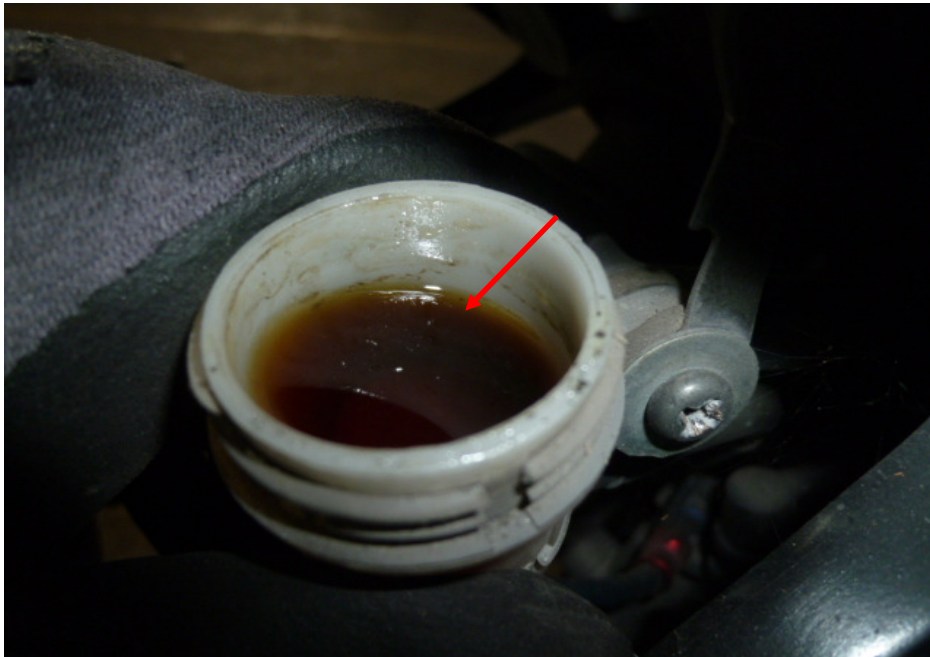
Photo 28 shows the brake fluid reservoir for the rear brake of the Motorcycle. The brake fluid was observed to be of sufficient level for operating purposes. However it was found to be slightly contaminated (arrowed).
