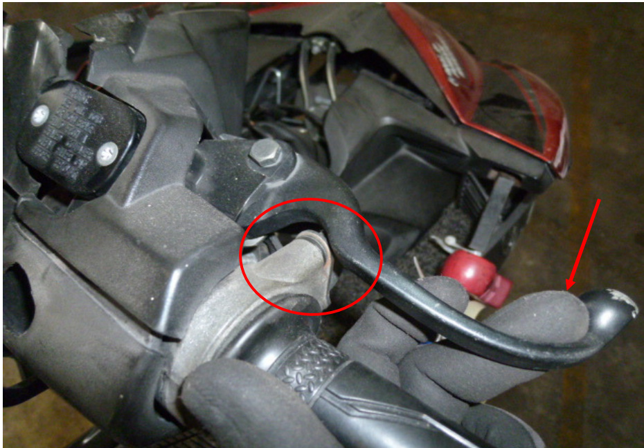
Photo 26 shows the front brake lever being depressed. There was some resistance felt (spongy like feel) upon pressing the front brake lever (arrowed). However the accident had caused the throttle cable housing of the Motorcycle to rotate (circled). Hence we were unable to fully depress the front brake lever to determine if there is a leakage of pressure/vacuum in the front brake system.
