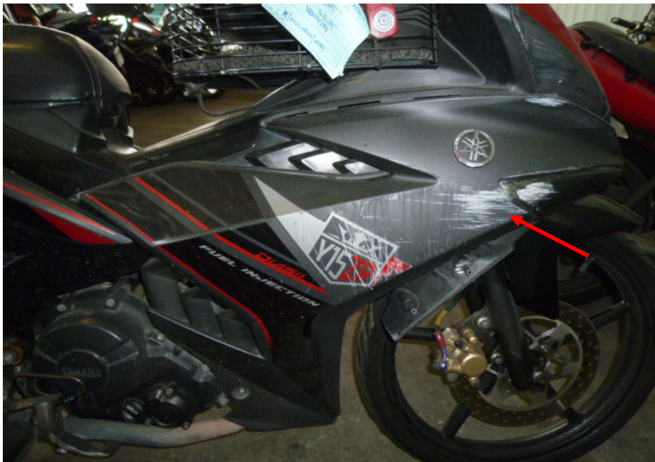
Photo 7 shows a closer view of the grazed right cowling of the Motorcycle as a result of the accident.
