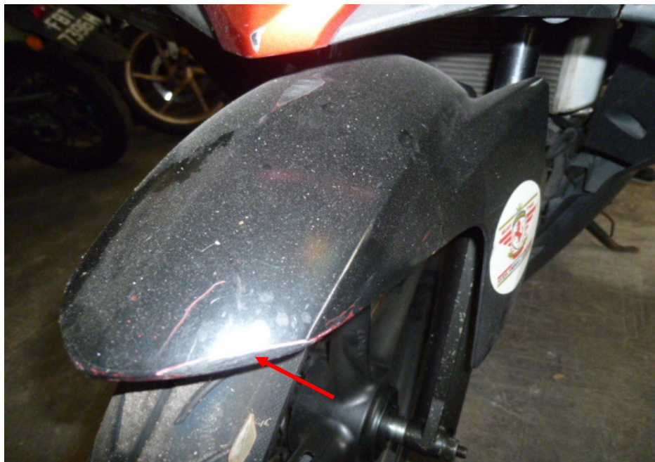
Photo 5 shows a closer view of the grazed front mudguard of the Motorcycle that as a result of the accident (arrowed).
