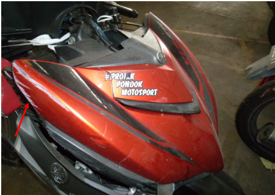
Photo 8 shows a closer view of the grazed front cowling of the Motorcycle as a result of the accident (arrowed).
