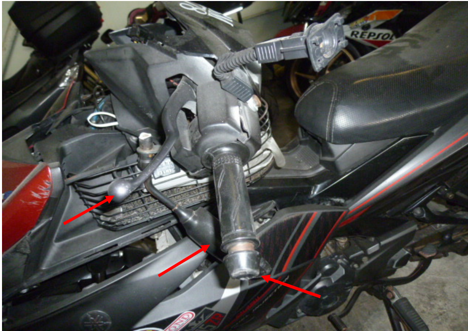
Photo 10 shows the left handlebar end, clutch brake lever and left side mirror (arrowed), which were amongst the body parts of the Motorcycle that had sustained damage as a result of the accident.
