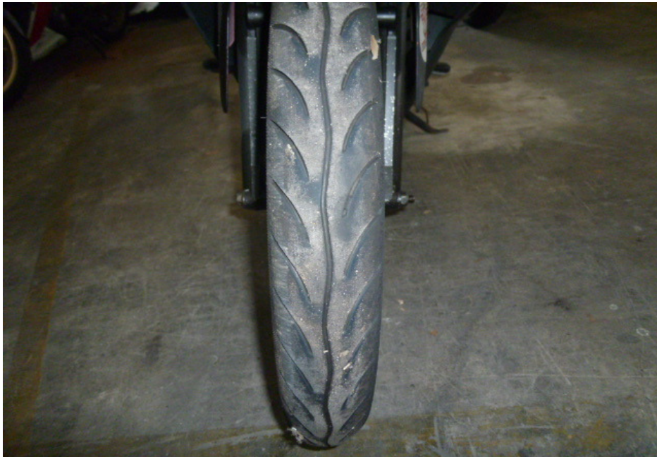
Photo 16 shows the condition of the Motorcycle's front tyre. The front tyre was observed to be in serviceable condition with remaining tread depth of approximately 2mm. The tyre was also observed to be sufficiently inflated for vehicular operation. We did not observe any tear, burst mark(s) and/or punctured hole(s) on the sidewalls as well as across the tread of the front tyre.
