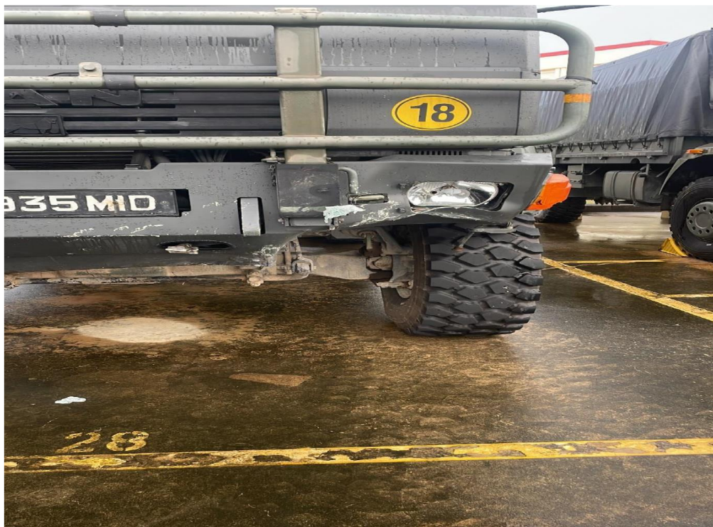
Figure 2E: Zoom in damage on LHS Front Bumper of (5TON) MID20935
