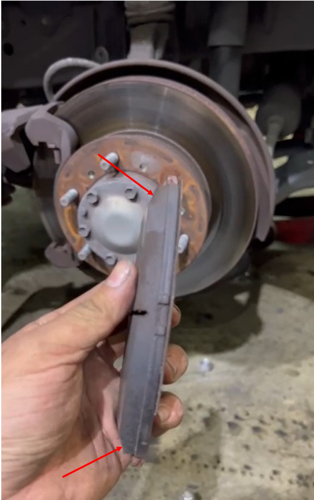
Photo 21 shows the Motor Lorry's front right brake pad after it was removed. The front right brake pad was found to be with sufficient frictional material (arrowed) for operational purposes.
