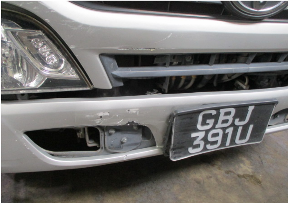
Photo 2 shows a closer view of the damaged front bumper, front number plate and front grille of the Motor Lorry.
