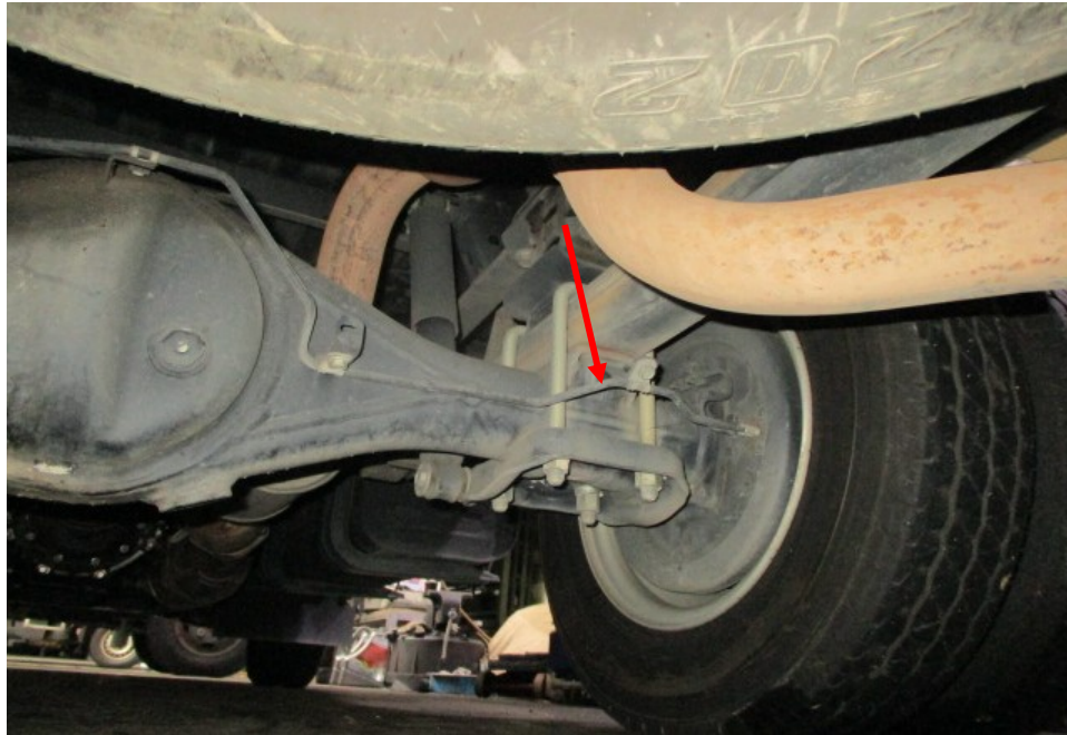
Photo 16 shows the brake fluid pipe (arrowed) at the rear right wheel of the Motor Lorry. I did not observe any leakage of brake fluid at the time of my inspection of the Motor Lorry. My static tests of the Motor Lorry's braking system, along with my visual examination of the various mechanical components in the braking system, had indicated that there was no internal leakage of pressure/vacuum. The braking system of the Motor Lorry was likely to be in serviceable condition at the material time of accident.
