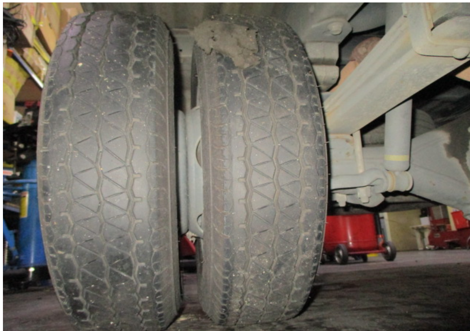
Photo 9 shows the rear right tyres of the Motor Lorry, which were observed to be in serviceable condition with remaining tread depth of approximately 5mm. Overall, there was no tear, cut or burst mark(s) on the outer and the inner sidewalls as well as across the tread of the 6 tyres that were fitted on the Motor Lorry.
