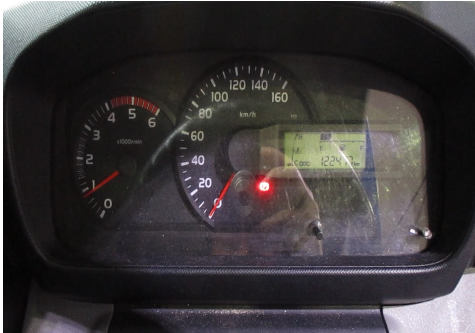
Photo 24 shows the warning lights no longer illuminated, indicating that there is no fault detected to the electronic safety features and warning features of the Motor Lorry during the self-test. These electronic safety systems and warning features of the Motor Lorry like the Supplemental Restraint System (SRS), warning lights for engine oil level and engine oil pressure, charging system, check engine light etc were all hence in working condition.
