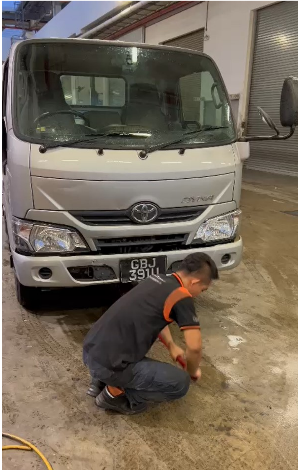
Photo 20 shows the Motor Lorry being jacked up at its frontal portion for removal and checks of its front brake pads.
