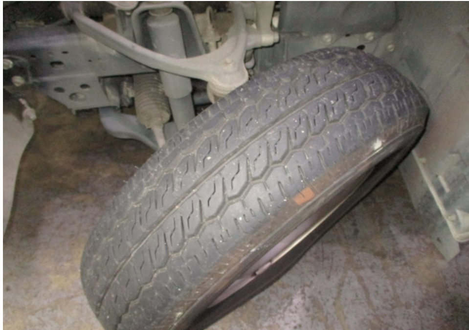
Photo 6 shows the front left tyre of the Motor Lorry, which was observed to be in serviceable condition with remaining tread depth of approximately 5mm. The tyre, which was wrapped around standard alloy wheel rim, was also observed to be sufficiently inflated for vehicular operation. Overall, there was no tear, cut or burst mark(s) on the outer and the inner sidewalls as well as across the tread of the 6 tyres that were fitted on the Motor Lorry.
