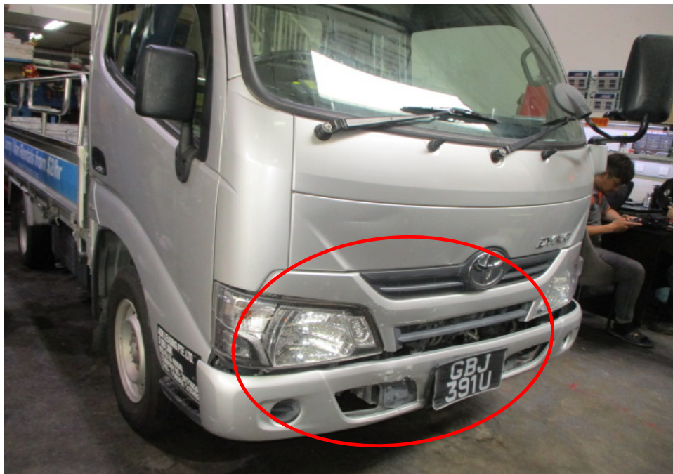
Photo 1 shows a general view of the front right body of the Motor Lorry at the time of my inspection. The Motor Lorry was observed to have sustained relatively minor impact damage at its frontal portion (circled). Body parts damaged include the front bumper, front number plate, front grille, front centre panel and front right headlamp amongst others
