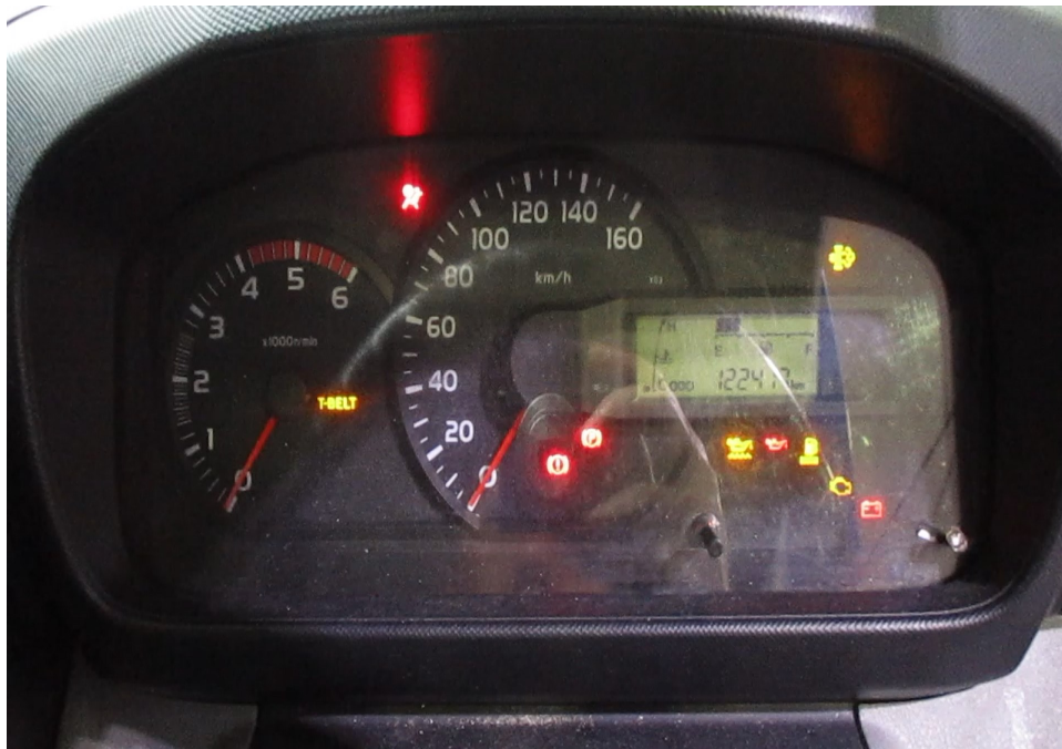
Photo 23 shows the warning lights for the various electronic safety features and warning features like the Supplemental Restraint System (SRS), warning lights for engine oil level and engine oil pressure, charging system, check engine light etc appearing on the instrument panel of the Motor Lorry during its self-test when the engine is cranked.
