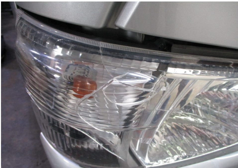
Photo 3 shows a closer view of the damaged front right headlamp of the Motor Lorry.
