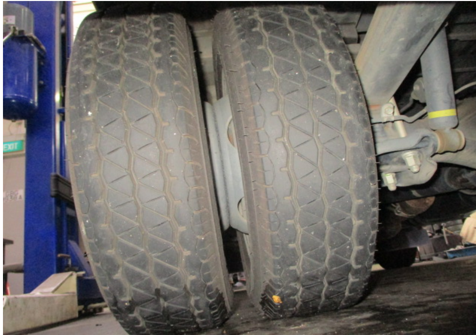
Photo 8 shows the rear left tyres of the Motor Lorry, which was observed to be in serviceable condition with remaining tread depth of approximately 5mm. The tyres, which were wrapped around standard alloy wheel rim, were also observed to be sufficiently inflated for vehicular operation. Overall, there was also no damage found on all 6 alloy wheel rims of the Motor Lorry.
