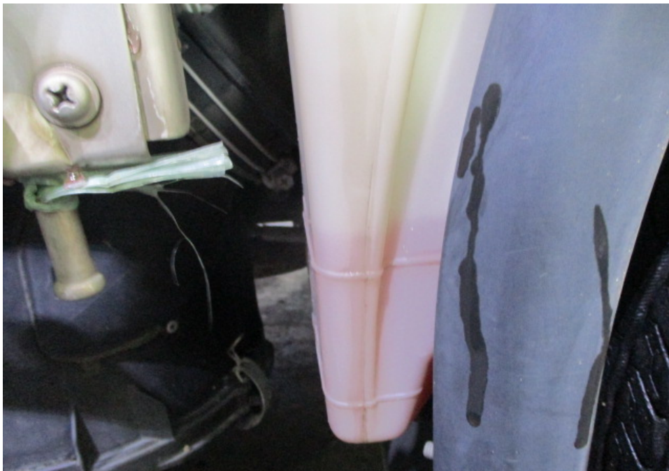
Photo 14 shows the engine coolant reservoir of the Motor Lorry at the time of my inspection. The engine coolant was observed to be of sufficient level and without any visible contamination.
