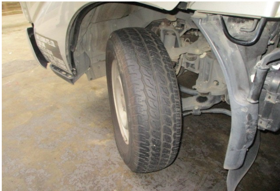
Photo 17 shows the front left wheel of the Motor Lorry turned to its full right. During my steering system test, I did not experience any abnormal free play and/or resistance when I had turned the steering wheel towards full left and full right. This would indicate that the steering system of the Motor Lorry was likely to be in serviceable condition at the material time of accident.
