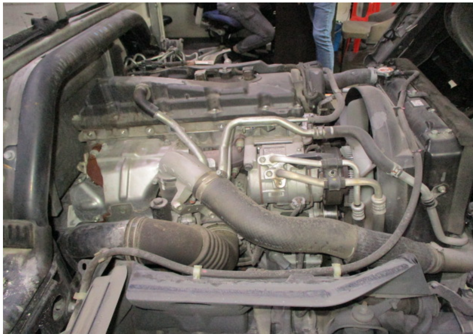
Photo 12 shows another view of the Motor Lorry's engine compartment. The various parts and components inside the engine compartment were unaffected by the accident. There was also no sign(s) or indication(s) of fluid leakage and/or fluid stain within the engine compartment (photograph shows the engine compartment as viewed from the right front side of the Motor Lorry).
