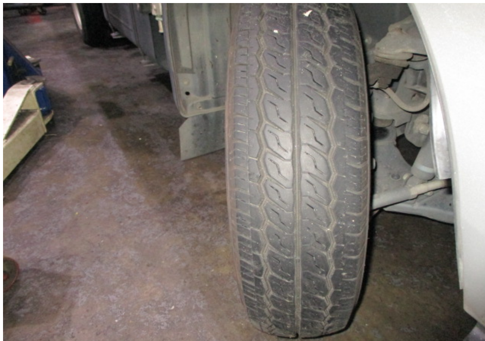
Photo 7 shows the front right tyre of the Motor Lorry, which was observed to be in serviceable condition with remaining tread depth of approximately 5mm. The tyre, which was wrapped around standard alloy wheel rim, was also observed to be sufficiently inflated for vehicular operation.
