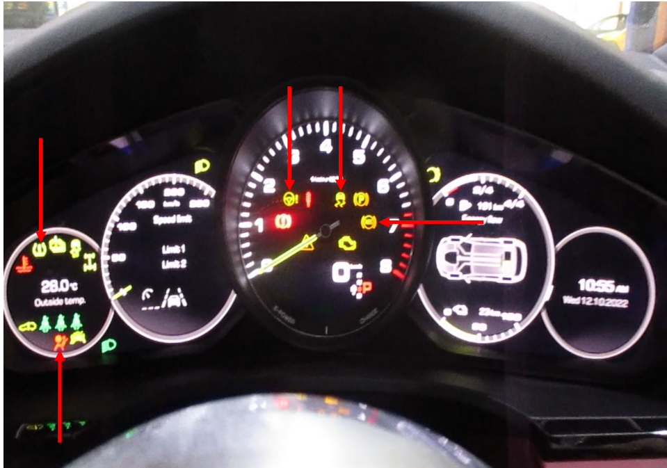
Photo 18 shows the warning lights for the various electronic safety features appearing on the instrument panel of the Motor Car during its self-test when the engine is cranked, in particular the ABS, SRS, TPM, EPS and TCS lights (arrowed).
