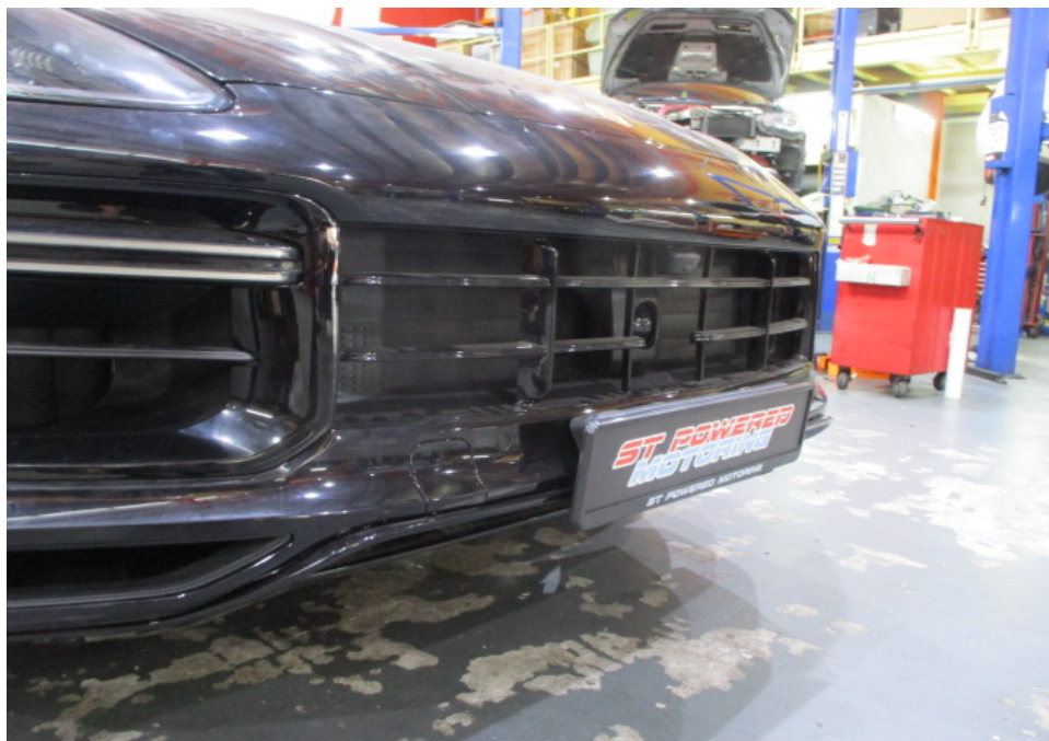
Photo 11 shows a closer view of the Motor Car's front bumper, front bumper lower cover, front bumper centre grille and front radar unit. The body parts at the frontal portion of the Motor Car were visually examined and it was observed that the repair/restoration works carried out to the damaged area of the Motor Car (refer to photograph 1 & 2 above) were reasonably adequate and in order.
