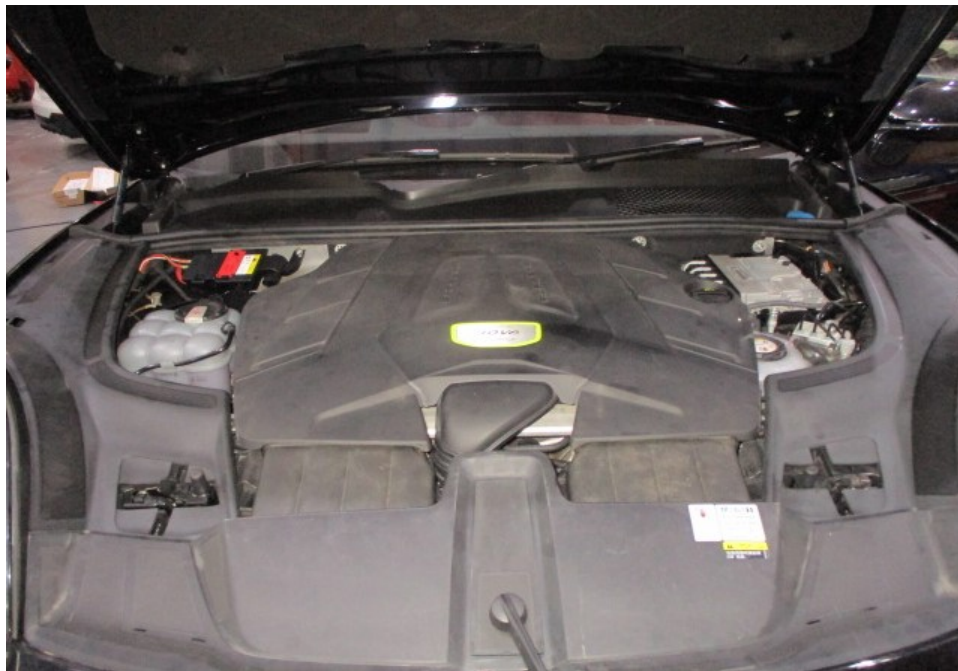
Photo 15 shows a general view of the engine compartment of the Motor Car at the time of my inspection. The various parts and components inside the engine compartment were all observed to be intact and properly fitted. There was also no sign(s) or indication(s) of fluid leak and/or fluid stain found inside the engine compartment. The repair/restoration works carried out to the various parts within the engine compartment like the front bonnet locks, front support panel, front support panel top garnish, aircon condenser and radiator amongst others were reasonably adequate and in order.
