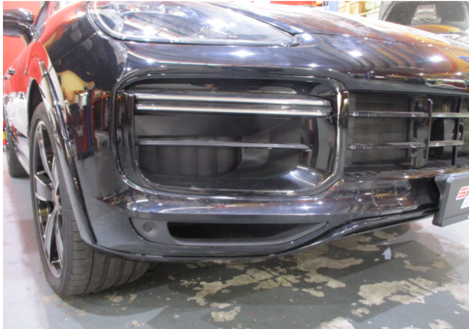
Photo 10 shows a closer view of the Motor Car's front bumper, front bumper right grille, front right day light and front right headlamp. The body parts at the frontal portion of the Motor Car were visually examined and it was observed that the repair/restoration works carried out to the damaged area of the Motor Car (refer to photograph 1 & 2 above) were reasonably adequate and in order.
