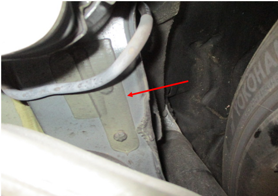
Photo 27 shows the chassis/structural body at the underside rear right of the Motor Car. I did not find any weld marks other than original spot weld marks on the chassis/structural body of the Motor Car. The original factory sealant (arrowed) at the joints along the chassis/structural body was untouched, indicating no work was done on the chassis/structural body of the Motor Car and that the chassis/structural body was originally fitted.
