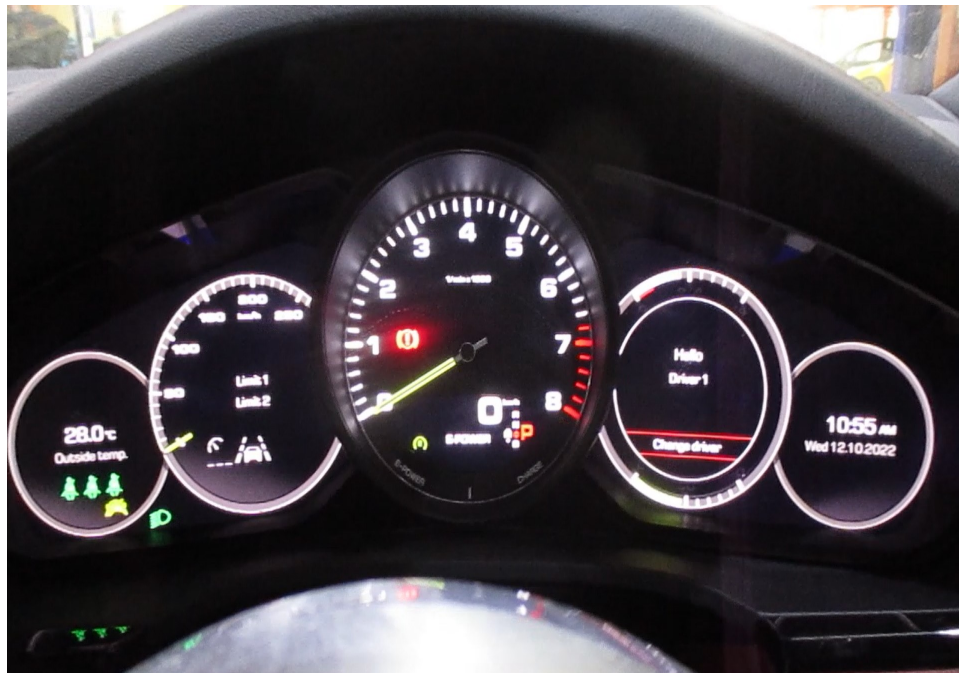
Photo 19 shows the respective warning lights no longer illuminated, indicating that there is no fault detected to the ABS, SRS, TPM, EPS and TCS systems of the Motor Car during the self-test. These electronic systems were hence in working condition at the time of my inspection.
