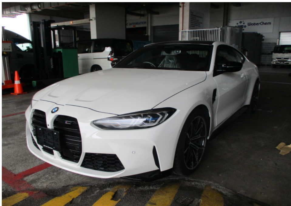
Photo 9 shows a general view of the front left body of the Motor Car at the time of my inspection. The Motor Car was observed to be in a relatively good general condition with no loose exterior fittings observed. The body parts at the front left portion of the Motor Car were visually examined and it was observed that the repair/restoration works carried out to the damaged area of the Motor Car (refer to photograph 4 above) were reasonably adequate and in order.
