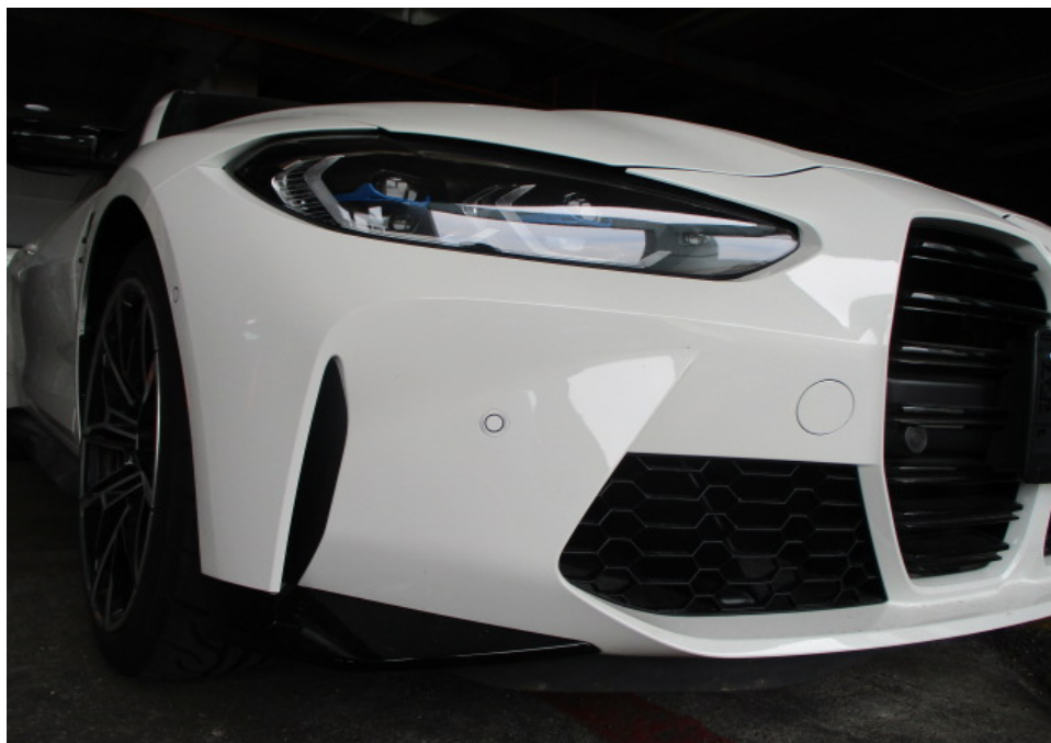
Photo 7 shows a closer view of the Motor Car's front bumper, front bumper right sensor, front bumper right lower grille, front bumper right lower garnish and front bumper right air guide. The body parts at the right front portion of the Motor Car were visually examined and it was observed that the repair/restoration works carried out to the damaged area of the Motor Car (refer to photograph 1 above) were reasonably adequate and in order.
