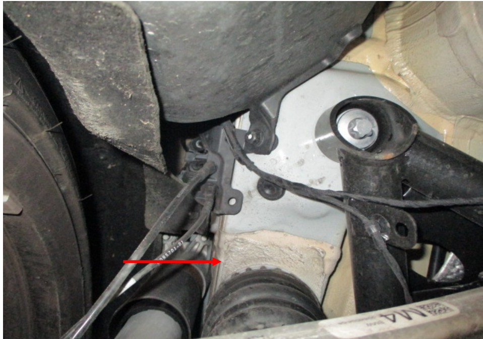
Photo 26 shows the chassis/structural body at the underside rear left of the Motor Car. The original factory sealant (arrowed) at the joints along the chassis/structural body was observed to be untouched. In general, I had found no work was carried out on the chassis/structural body of the Motor Car. The chassis/structural body of the Motor Car was originally fitted.
