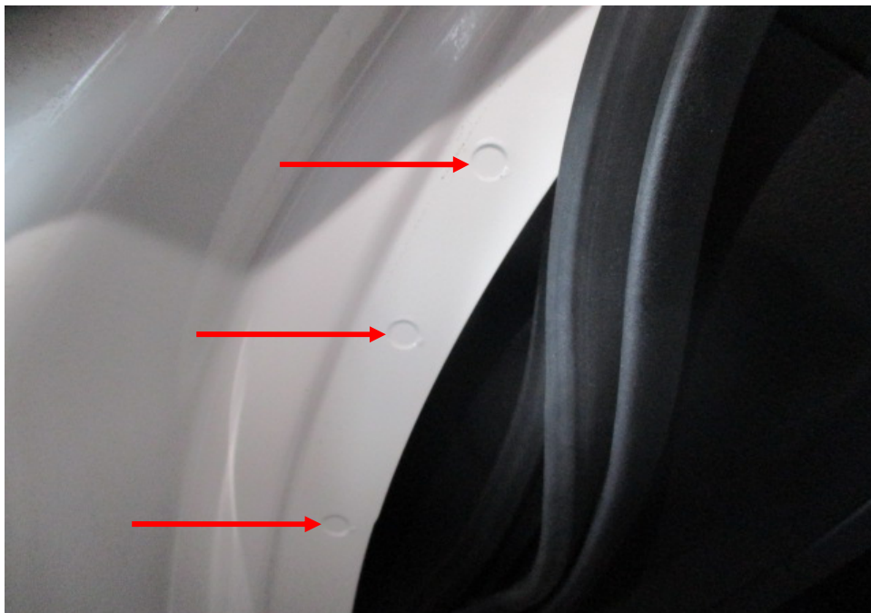
Photo 29 shows the left side "A" pillar of the Motor Car. I did not find any weld marks other than original spot weld marks (arrowed) on the left side "A" pillar of the Motor Car which, indicates that there was no re-welding works carried out. In general, I had found all the non-detachable body panels of the Motor Car to be originally fitted at the time of my inspection.
