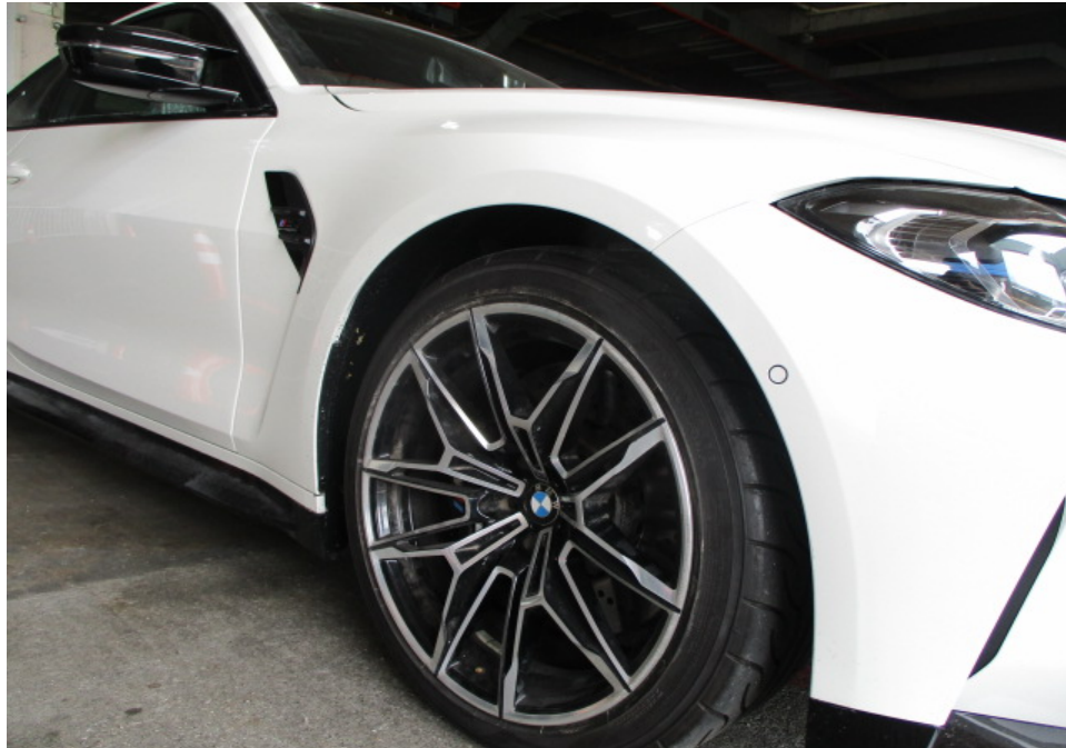
Photo 8 shows a closer view of the Motor Car's front bumper, front bumper right sensor, front right fender, front right wheel rim and front right door. The body parts at the right front portion of the Motor Car were visually examined and it was observed that the repair/restoration works carried out to the damaged area of the Motor Car (refer to photograph 1 above) were reasonably adequate and in order.
