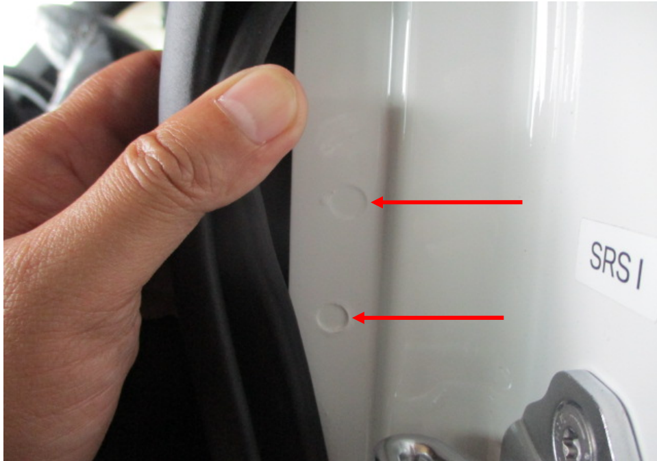
Photo 30 shows the left side rear body panel of the Motor Car. I did not find any weld marks other than original spot weld marks (arrowed) on the left side rear body panel of the Motor Car, which indicates that there was no re-welding works carried out. In general, I had found all the non-detachable body panels of the Motor Car to be originally fitted at the time of my inspection.
