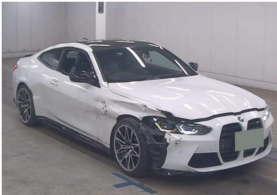
Photo 1 shows the front right body of the Motor Car (photograph provided to me). The Motor Car was observed to have sustained damage at its right front portion. The front bumper, front bumper right bracket, front bumper right lower garnish, front bumper right air guide, front bumper right sensor, front bonnet, front right headlamp, front right fender and front right door were amongst the body parts that were observed to have been damaged.
