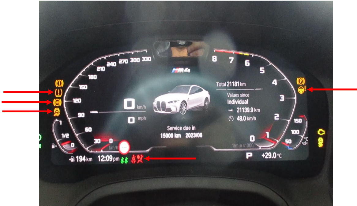
Photo 16 shows the warning lights for the various electronic safety features appearing on the instrument panel of the Motor Car during its self-test when the engine is cranked, in particular the ABS, SRS, IAS, TPM and DSC lights (arrowed).
