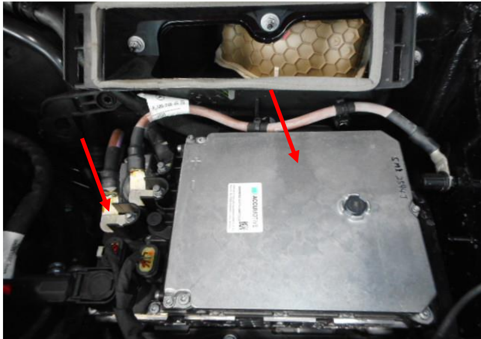
Photo 6 shows the close up view of the 48v battery and its components (arrowed) in the engine compartment portion of the Insured Vehicle at the time of our inspection. The 48v battery and its components is observed to be unaffected and by any signs of accident.
