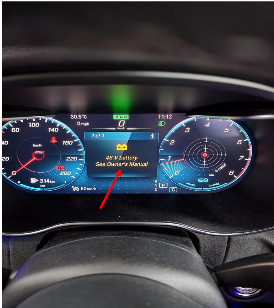
Photo 8 shows the conducted ECU diagnosis of the Insured Vehicle at the time of our inspection. There was an electronic error (arrowed) on the 48v battery integrated starter system (ISG) of the Insured Vehicle.
