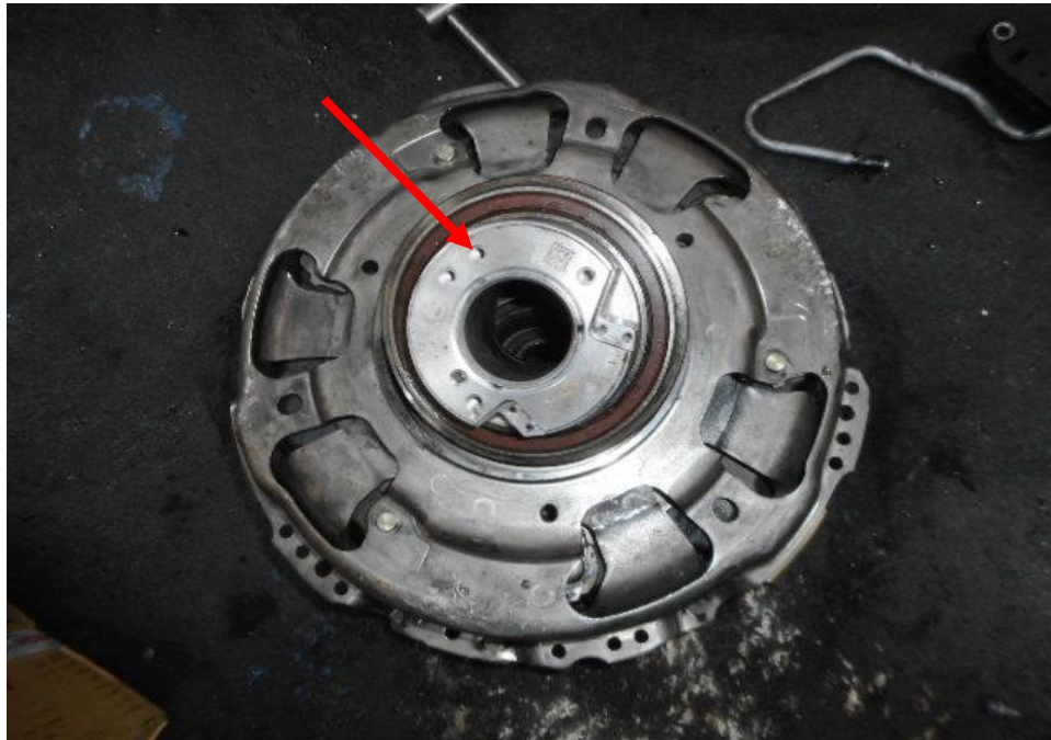
Photo 6 shows the general view of clutch unit of the gearbox unit of the Insured Vehicle at the time of our inspection. The clutch bearing (arrowed) component in the gearbox unit is observed to be unaffected and by any signs of accident. However, whining and grinding sound was heard when the clutch bearing was turned and upon closer inspection there was grease leaking out from the clutch bearing.
