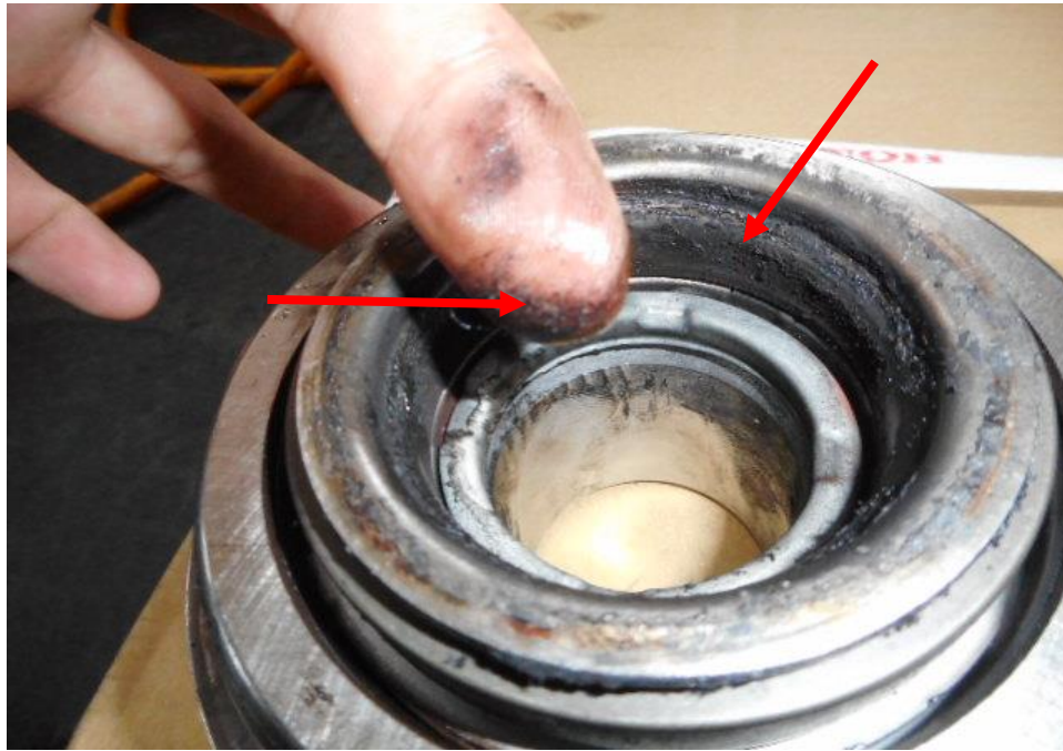
Photo 8 shows the close up view of clutch bearing of the clutch of the gearbox unit of the Insured Vehicle at the time of our inspection. The clutch bearing (yellow arrow) component in the gearbox unit is observed to be unaffected and by any signs of accident. However, whining and grinding sound was heard when the clutch bearing was turned and upon closer inspection there was grease leaking (red arrow) out from the clutch bearing.
