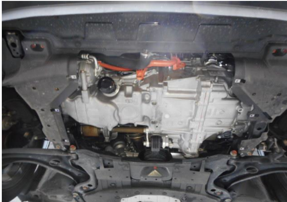
Photo 4 shows the general view of the undercarriage portion of the Insured Vehicle at the time of our inspection. The undercarriage compartment is observed to be unaffected by any signs of accident.
