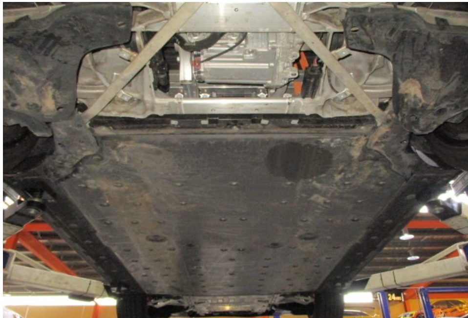
Photo 29 shows the underside centre of the Motor Car, at the location where the high voltage battery is fitted. The high voltage system of the Motor Car was visually checked, and it was observed that the various high voltage parts and components like the high voltage battery, inverter unit, converter unit, high voltage cables, electric motors and electric aircon compressor amongst others, were properly secured and without any physical damage.
