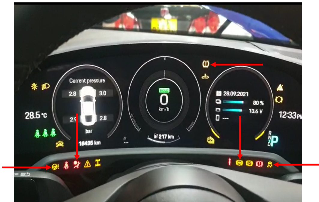
Photo 21 shows the warning lights for the various electronic safety features appearing on the instrument panel of the Motor Car during its self-test when the engine is cranked, in particular the ABS, SRS, EPS, TPM and SCS lights (arrowed).
