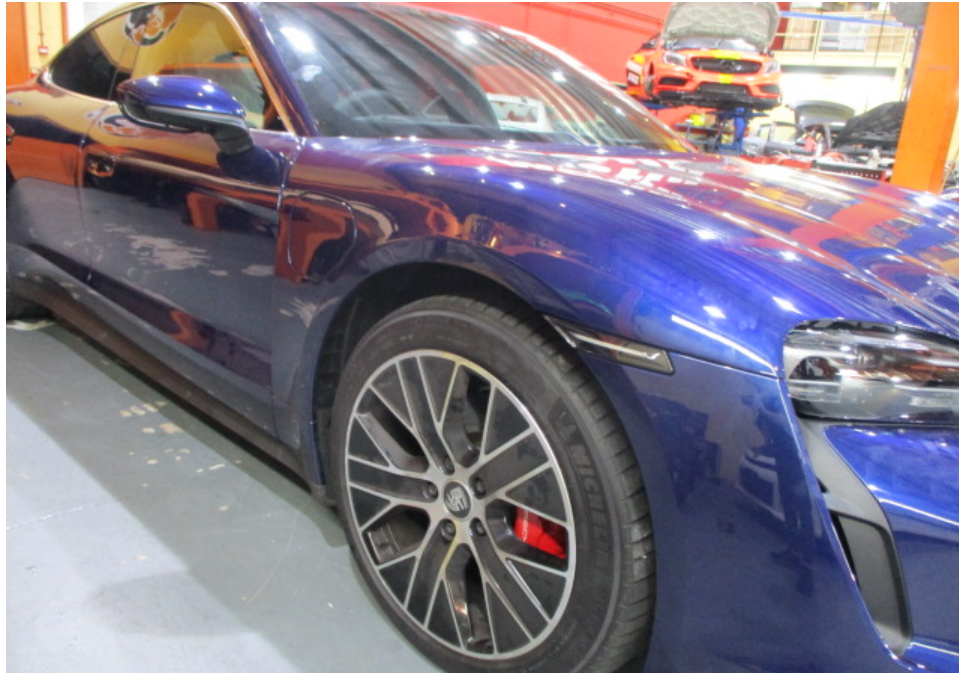
Photo 6 shows a closer view of the Motor Car's front bonnet, front right signal lamp, front right fender and front right wheel rim. The body parts at the frontal portion of the Motor Car were visually examined and it was observed that the repair/restoration works carried out to the damaged area of the Motor Car (refer to photograph 1 - 3 above) were reasonably adequate and in order.
