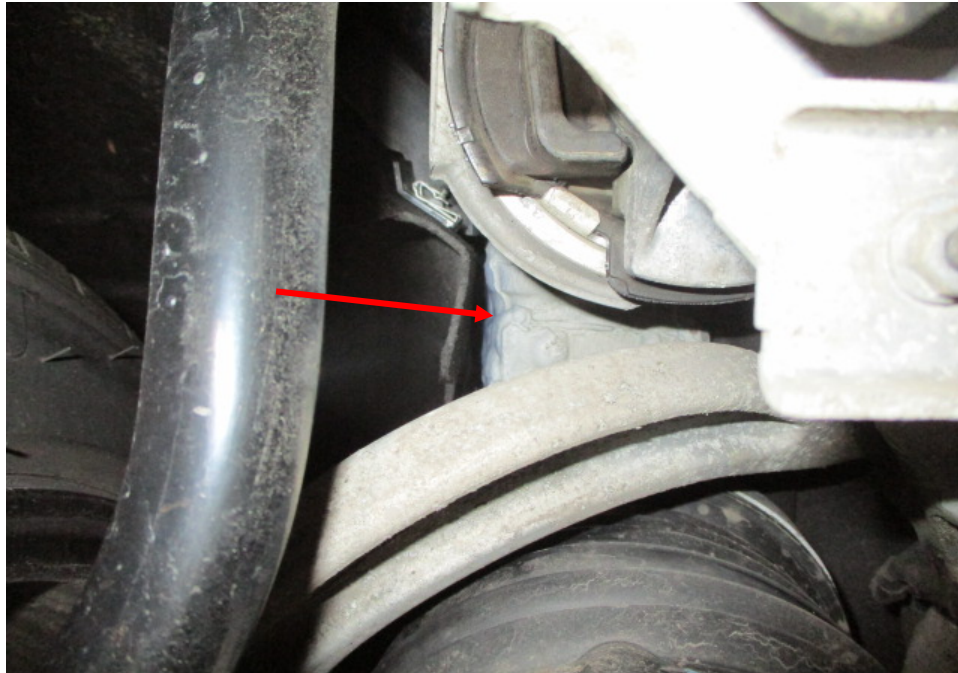
Photo 32 shows the chassis/structural body at the underside rear left of the Motor Car. The original factory sealant (arrowed) at the joints along the chassis/structural body was observed to be untouched. In general, I had found no work was carried out on the chassis/structural body of the Motor Car. The chassis/structural body of the Motor Car was originally fitted.
