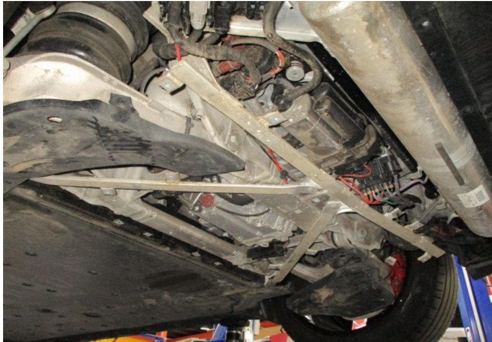
Photo 28 shows the underside rear of the Motor Car, at the location where the rear electric motor is fitted. The high voltage system of the Motor Car was visually checked, and it was observed that the various high voltage parts and components like the high voltage battery, inverter unit, converter unit, high voltage cables, electric motors and electric aircon compressor amongst others, were properly secured and without any physical damage..
