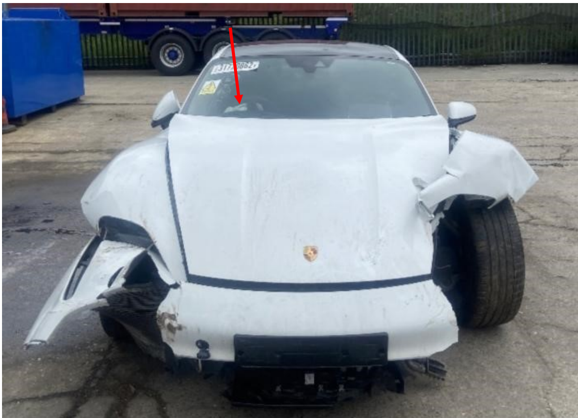
Photo 2 shows the frontal body of the Motor Car (photograph provided to me). The Motor Car was observed to have sustained damage at its frontal portion. The front bumper, front bumper lower lip, front bumper centre frame, front bumper right air guide, front bumper left air guide, front bumper right lower grille, front bumper left lower grille, front bumper sensors, front bonnet, front right headlamp and front left headlamp were amongst the body parts that were observed to have been damaged. The driver's airbag was deployed (arrowed).
