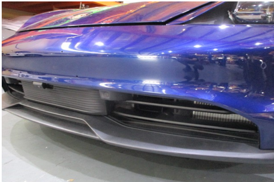
Photo 11 shows a closer view of the Motor Car's front bumper, front bumper lower lip, front bumper left lower grille, front bumper sensors, front bumper centre frame and front left radiator. The body parts at the frontal portion of the Motor Car were visually examined and it was observed that the repair/restoration works carried out to the damaged area of the Motor Car (refer to photograph 1 - 3 above) were reasonably adequate and in order.
