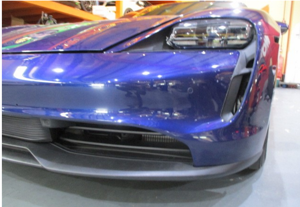
Photo 10 shows a closer view of the Motor Car's front bumper, front bumper lower lip, front bumper left air guide, front bumper left lower grille and front left headlamp. The body parts at the frontal portion of the Motor Car were visually examined and it was observed that the repair/restoration works carried out to the damaged area of the Motor Car (refer to photograph 1 - 3 above) were reasonably adequate and in order.
