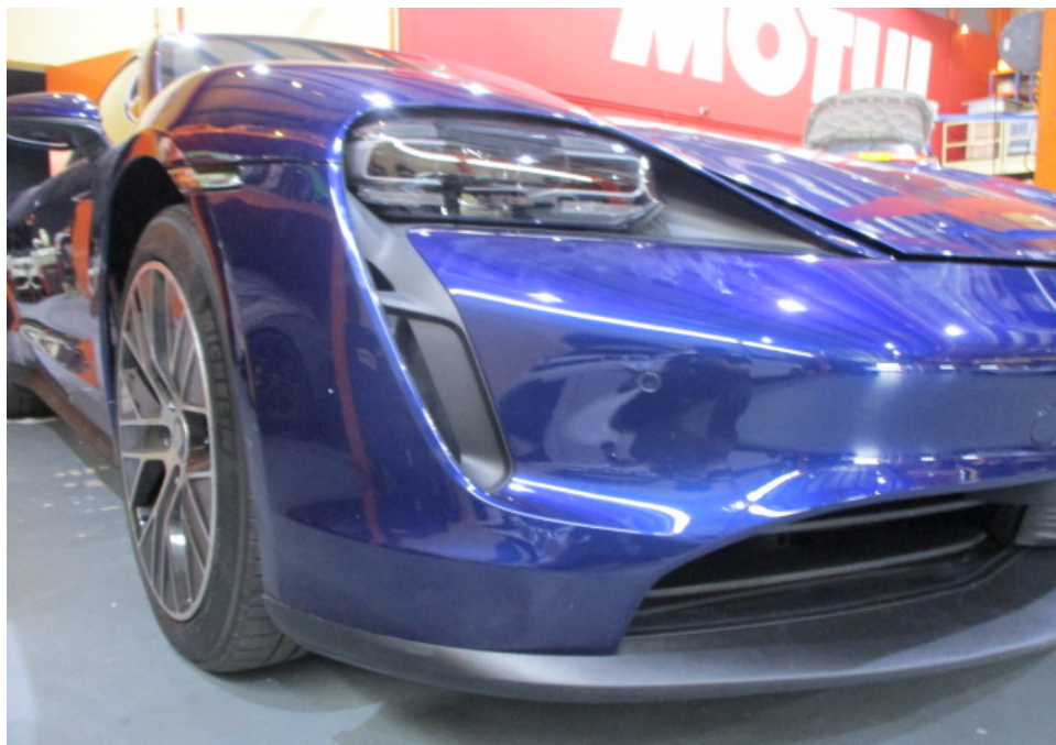
Photo 7 shows a closer view of the Motor Car's front bumper, front bumper lower lip, front bumper right air guide, front bumper right lower grille and front right headlamp. The body parts at the frontal portion of the Motor Car were visually examined and it was observed that the repair/restoration works carried out to the damaged area of the Motor Car (refer to photograph 1 - 3 above) were reasonably adequate and in order.
