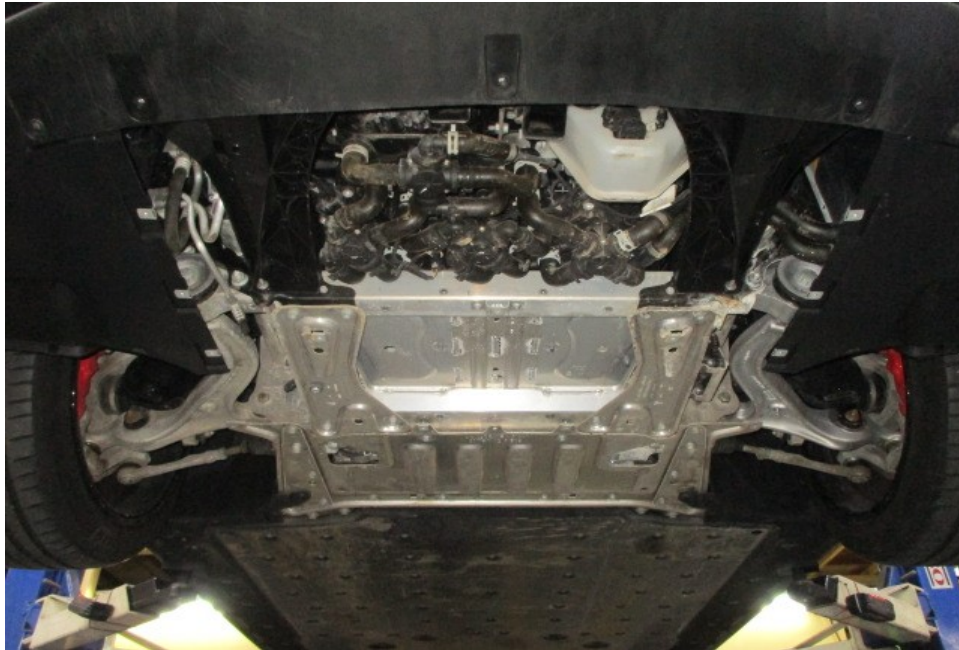
Photo 30 shows the underside front of the Motor Car, at the location where the front electric motor, is fitted. The high voltage system of the Motor Car was visually checked, and it was observed that the various high voltage parts and components like the high voltage battery, inverter unit, converter unit, high voltage cables, electric motors and electric aircon compressor amongst others, were properly secured and without any physical damage.
