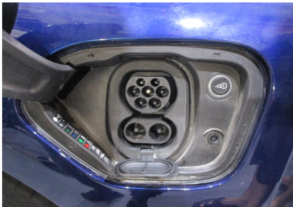
Photo 17 shows the high voltage charging port located at the front left fender of the Motor Car at the time of my inspection. A Combined Charging Standard 2 (CCS 2) for direct current (DC) charging was fitted on the front left fender of the Motor Car. No physical damage was observed to the charging head.
