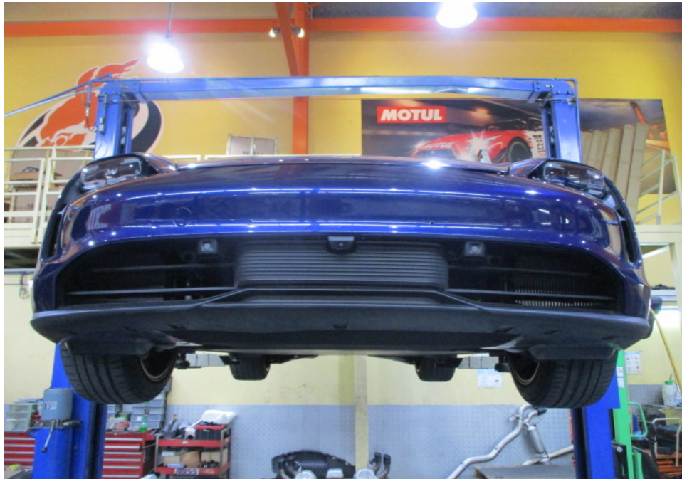
Photo 23 shows the Motor Car hoisted up for checks on its undercarriage. There was no sign(s) or indication(s) of fluid leakage and/or fluid stain(s) on the underside of the Motor Car. The undercarriage components of the Motor Car were also all observed to be intact and secured in an appropriate manner.
