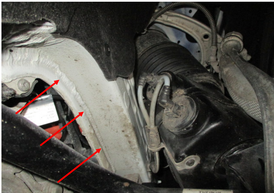
Photo 34 shows the chassis/structural body at the underside front right of the Motor Car. The original factory sealant (arrowed) at the joints along the chassis/structural body was observed to be untouched. In general, I had found no work was carried out on the chassis/structural body of the Motor Car. The chassis/structural body of the Motor Car was originally fitted.
