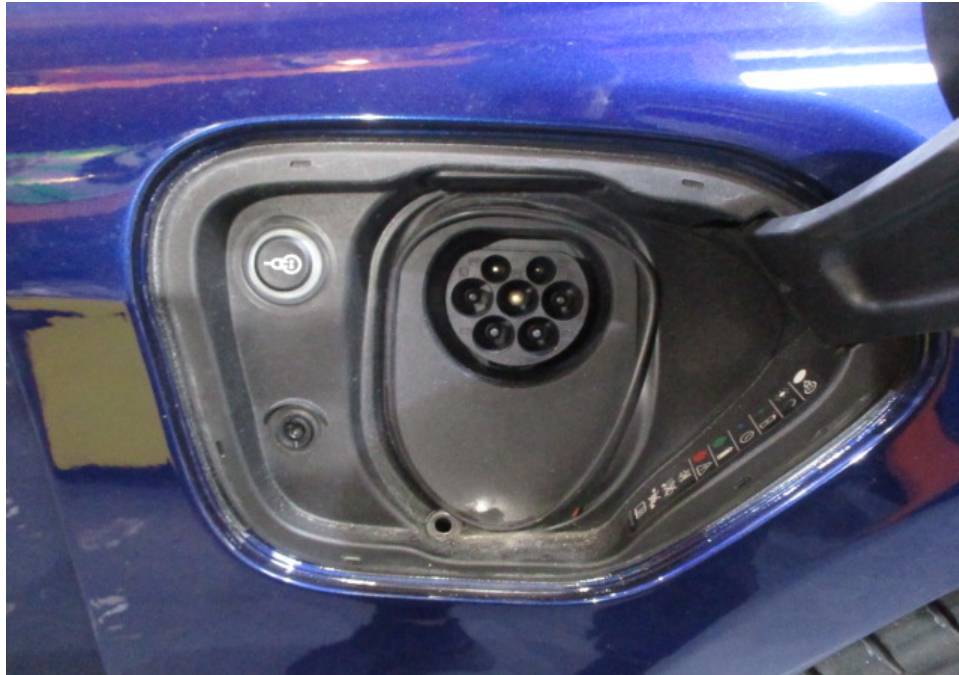
Photo 18 shows the high voltage charging port located at the front right fender of the Motor Car at the time of my inspection. A JS 1772 (Type 2) for alternating current (AC) charging was fitted on the front right fender of the Motor Car. No physical damage was observed to the charging head.
