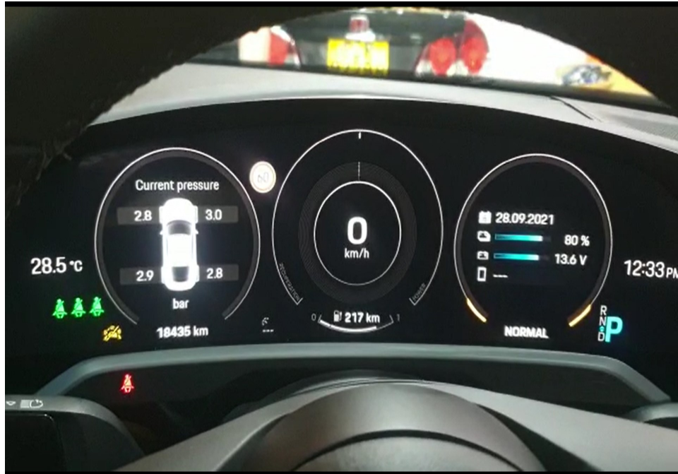
Photo 22 shows the respective warning lights no longer illuminated, indicating that there is no fault detected to the ABS, SRS, EPS, TPM and SCS systems of the Motor Car during the self-test. These electronic systems were hence in working condition at the time of my inspection.
