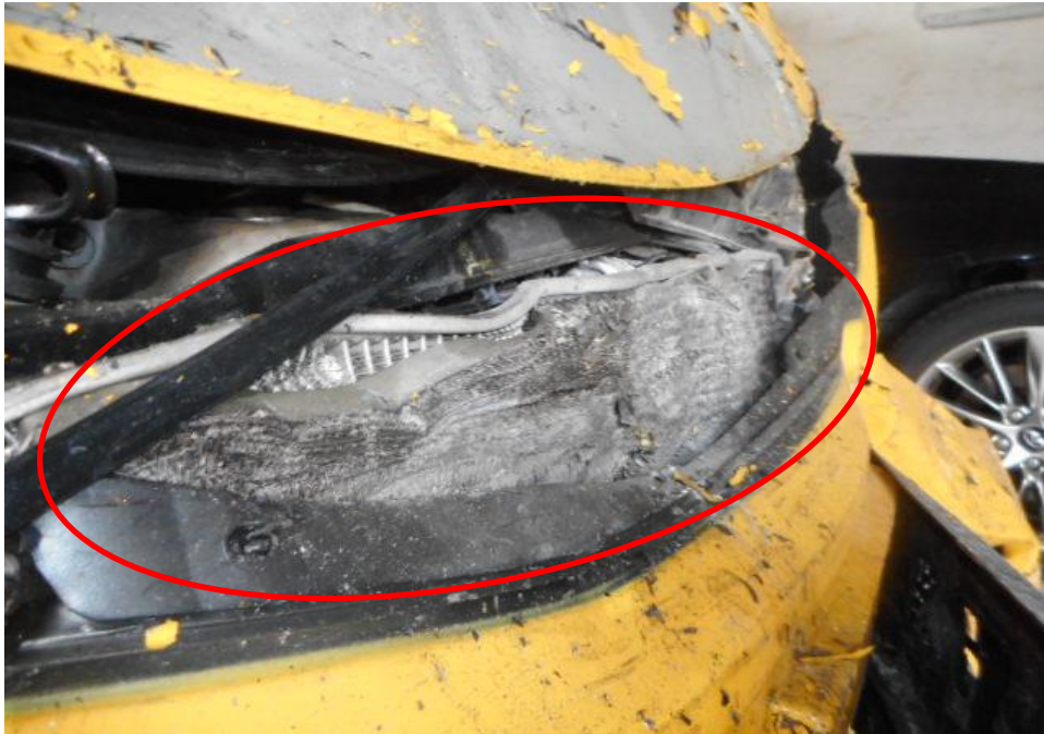
Photo 18 shows the close up view of the Motor Car's front body at the time of my inspection. The Motor car was observed to have sustained damage at its front portion. Its engine (circled) was amongst the various components in the engine compartments were also damaged as a result of the accident.
