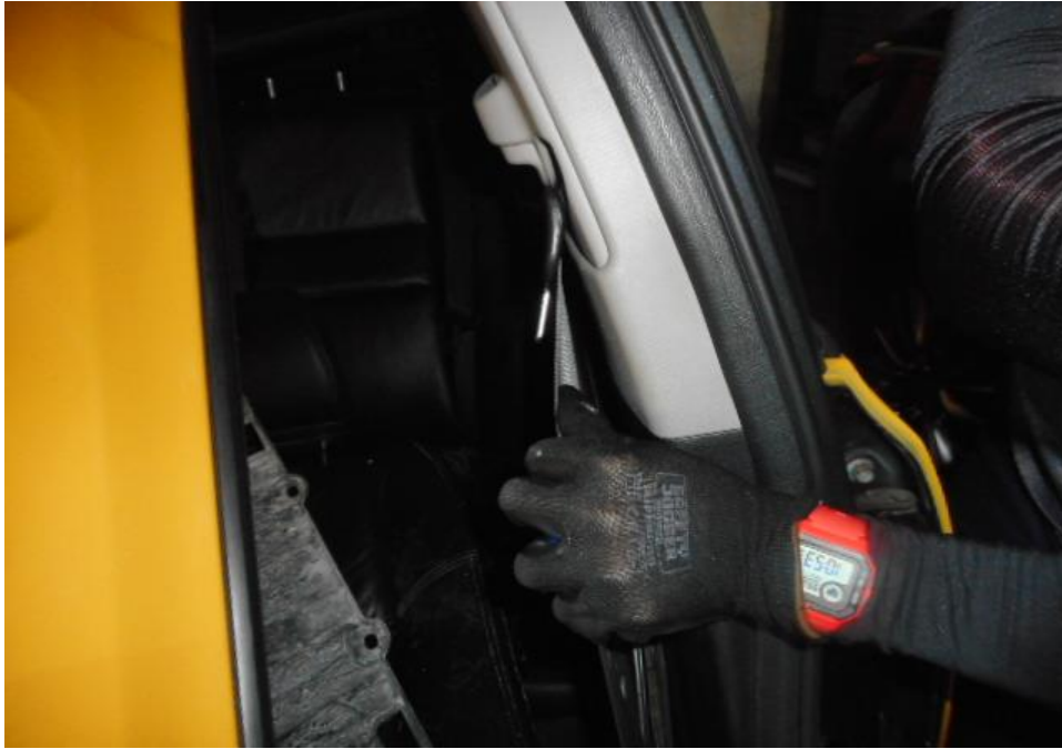
Photo 28 shows that the seat belt on the left seat was not worn at the material time of accident as the safety pre-tensioners was activated at the moment of impact and caused the seat belt to be locked into the last position.
