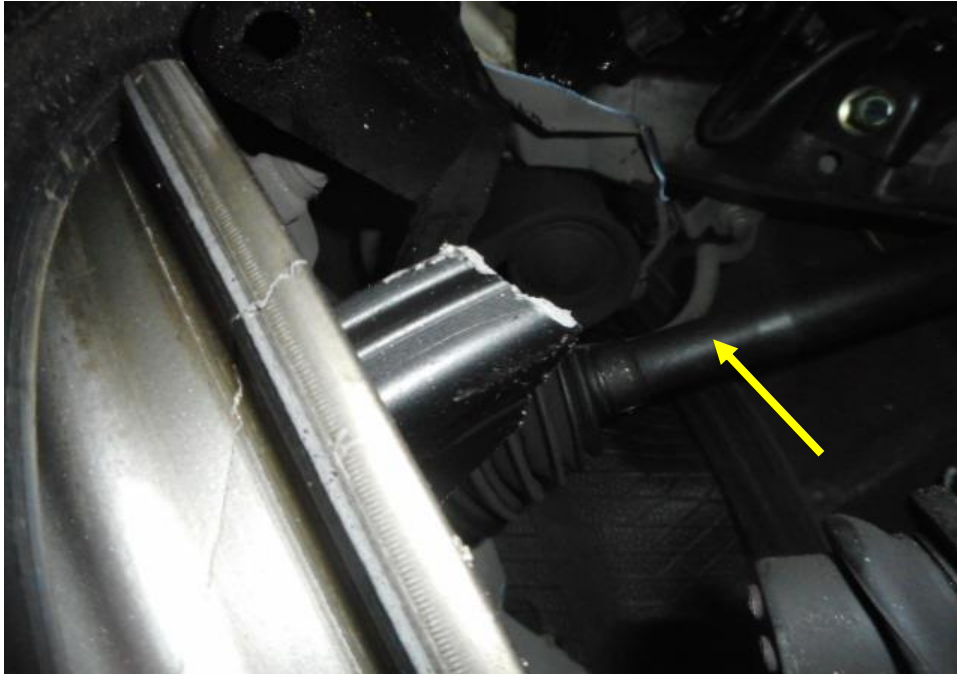
Photo 25 shows the various undercarriage components at the front right wheel of the Motor Car, in particular the driveshaft (arrowed) was observed to be intact and without visible damage.
