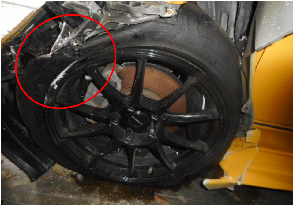
Photo 12 shows the general condition of the front left tyre of the Motor Car, which was observed to be deflated due to the damaged rim (circled) as a result of the accident. The tyre was also observed with cut mark(s) with remaining tread depth of approximately 6mm.
