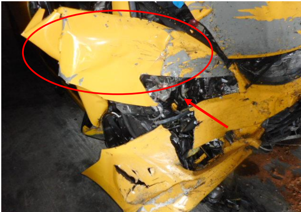
Photo 6 shows the close up view of the Motor Car's front body at the time of my inspection. The Motor car was observed to have sustained damage at its front portion. Its front right headlamp (circled) and front right fender (arrowed) was amongst the body parts and various components in the engine compartments were also damaged as a result of the accident.
