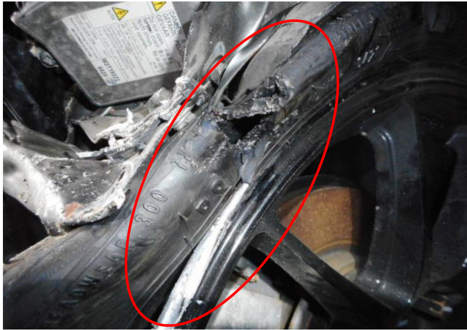
Photo 13 shows the close up condition of the front left tyre of the Motor Car, which was observed to be deflated due to the damaged rim (circled) as a result of the accident. The tyre was also observed with cut mark(s) with remaining tread depth of approximately 6mm.
