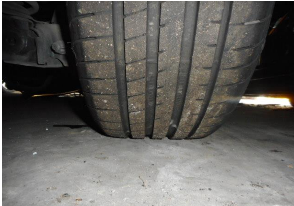
Photo 14 shows the condition of the rear right tyre of the Motor Car, which was observed to be in serviceable condition with remaining tread depth of approximately 5.8mm. The tyre was also observed to be sufficiently inflated for vehicular operation with no tear, cut or burst mark(s).
