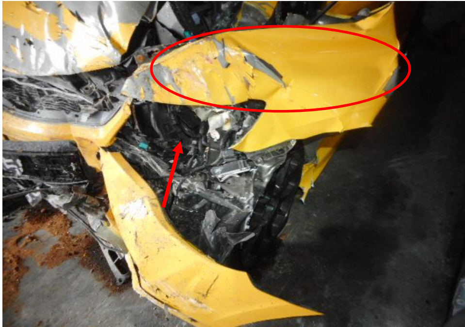
Photo 7 shows the close up view of the Motor Car's front body at the time of my inspection. The Motor car was observed to have sustained damage at its front portion. Its front left headlamp (circled) and front left fender (arrowed) was amongst the body parts and various components in the engine compartments were also damaged as a result of the accident.
