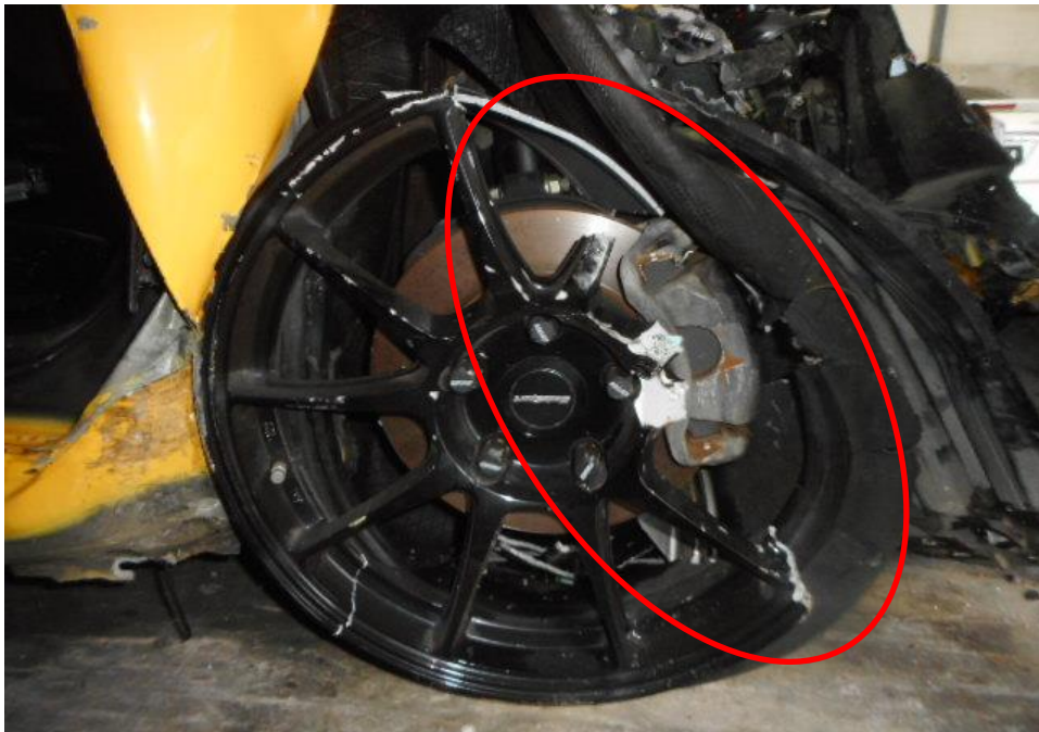
Photo 10 shows the general condition of the front right tyre of the Motor Car, which was observed to be deflated due to the damaged rim (circled) as a result of the accident. The tyre was also observed with cut mark(s) with remaining tread depth of approximately 6.1mm.
