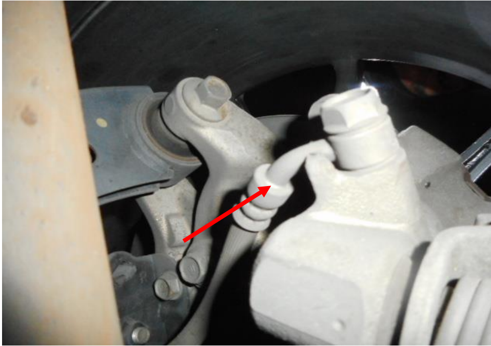
Photo 21 shows the brake hose/pipe (arrowed) at the rear right wheel of the Motor Car. No leakage of brake fluid was observed. Visual examination of the various components of the braking system like the brake caliper to be intact and without visible damage.
