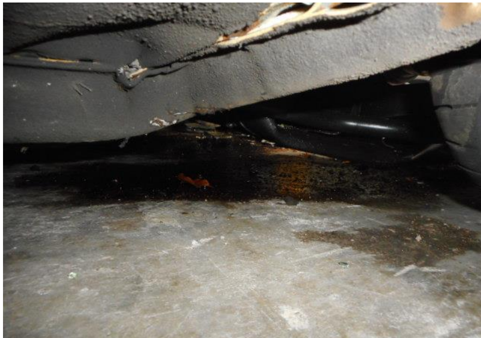
Photo 19 shows the undercarriage of the Motor Car, at the area where the engine housing and transmission housing are located. I found sign(s) or indication(s) of fluid leak and/or fluid stain(s) on the underside of the Motor Car due to the damaged engine as a result of the accident.
