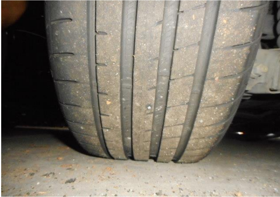
Photo 15 shows the condition of the rear left tyre of the Motor Car, which was observed to be in serviceable condition with remaining tread depth of approximately 6mm. The tyre was also observed to be sufficiently inflated for vehicular operation with no tear, cut or burst mark(s).
