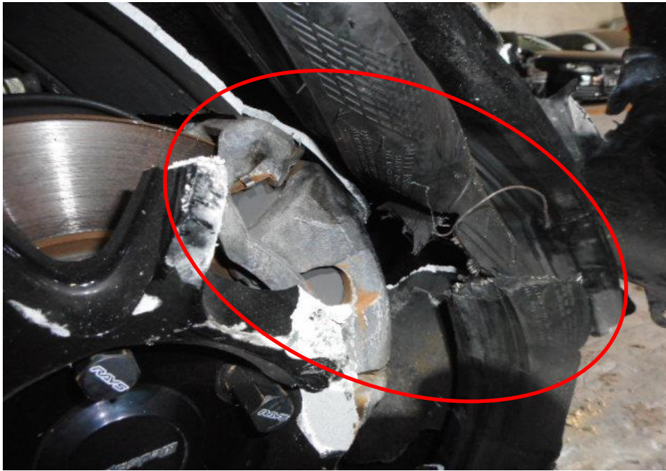
Photo 11 shows the close up condition of the front right tyre of the Motor Car, which was observed to be deflated due to the damaged rim (circled) as a result of the accident. The tyre was also observed with cut mark(s) with remaining tread depth of approximately 6.1mm.
