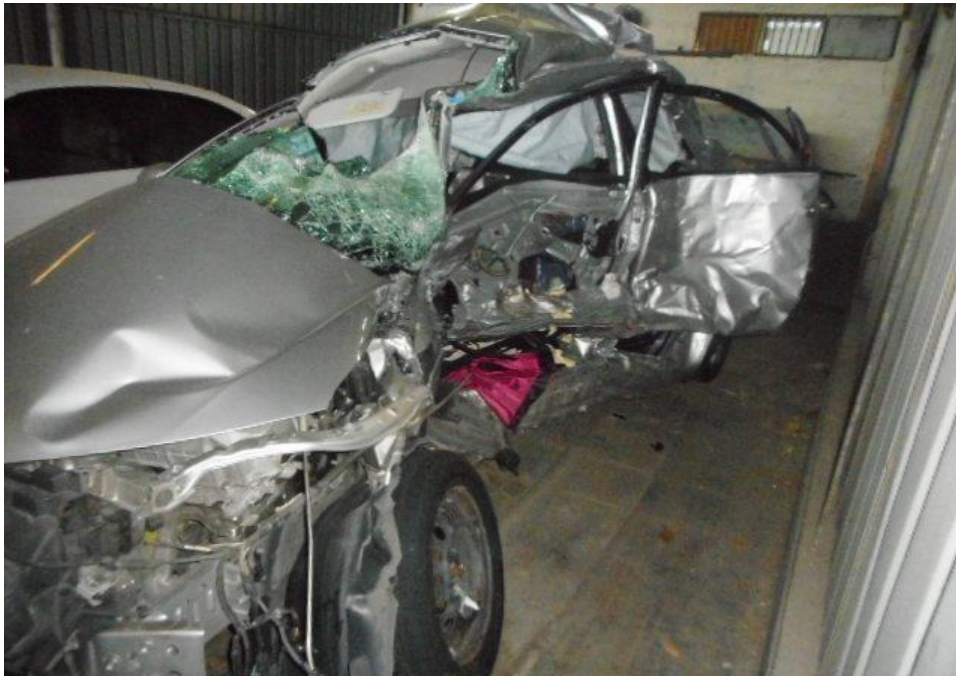
Photo 11 shows a general view of the Motor Car's left body at the time of my inspection. The Motor car was observed to have sustained damage at its left portion. Its left doors and left chassis was amongst the body parts damaged as a result of the accident.
