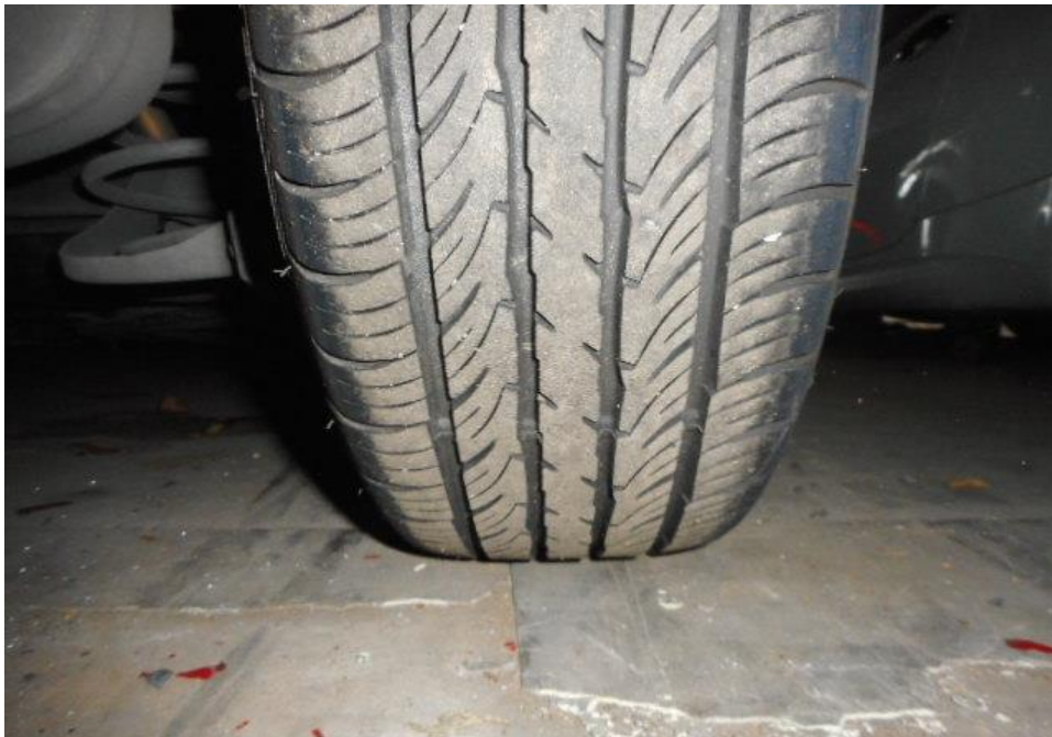
Photo 14 shows the condition of the rear right tyre of the Motor Car, which was observed to be in serviceable condition with remaining tread depth of approximately 6mm. The tyre was also observed to be sufficiently inflated for vehicular operation with no tear, cut or burst mark(s).
