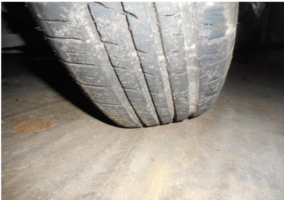
Photo 16 shows the condition of the front left tyre of the Motor Car, which was observed to be in serviceable condition with remaining tread depth of approximately 5.8mm. The tyre was also observed to be sufficiently inflated for vehicular operation with no tear, cut or burst mark(s).
