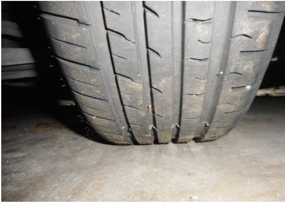
Photo 13 shows the condition of the front right tyre of the Motor Car, which was observed to be in serviceable condition with remaining tread depth of approximately 5.7mm. The tyre, which was wrapped around alloy wheel rim, was also observed to be sufficiently inflated for vehicular operation.
