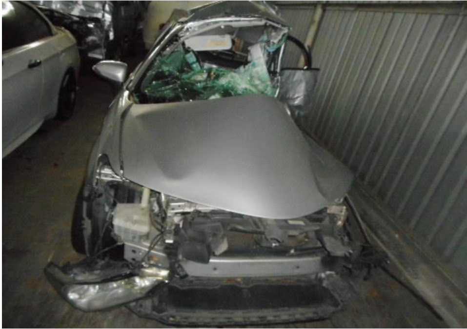
Photo 5 shows a general view of the Motor Car's front body at the time of my inspection. The Motor car was observed to have sustained damage at its front and roof portion. Its front windscreen, front bonnet, front bumper, front left fender, front left, right headlamp and roof panel was amongst the body parts that were damaged as a result of the accident. The Supplemental Restraint System (SRS) was activated as a result of the accident.
