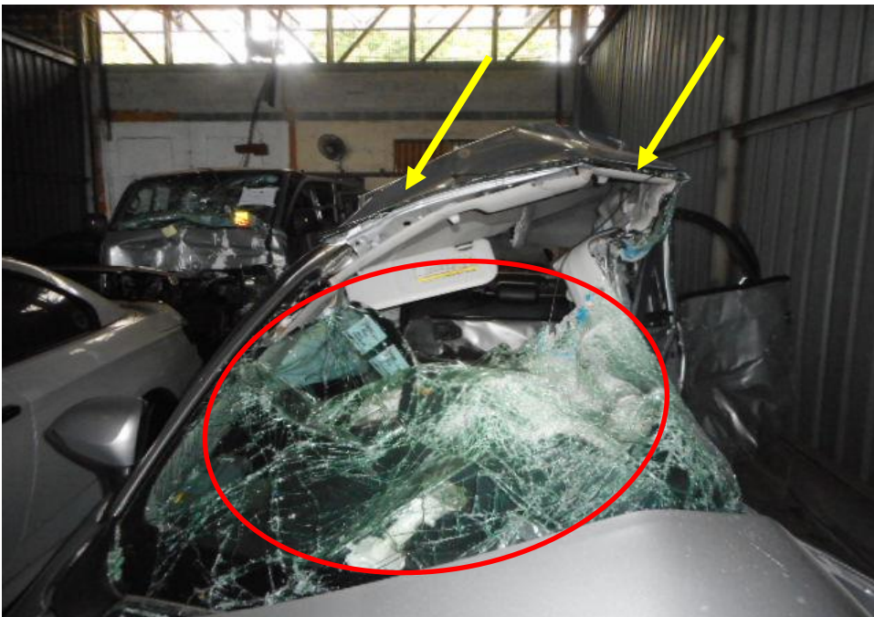
Photo 6 shows the close up view of the Motor Car's front body and roof panel at the time of my inspection. The Motor car was observed to have sustained damage at its front portion. Its front windscreen (circled) and front panel (arrowed) was damaged as a result of the accident.
