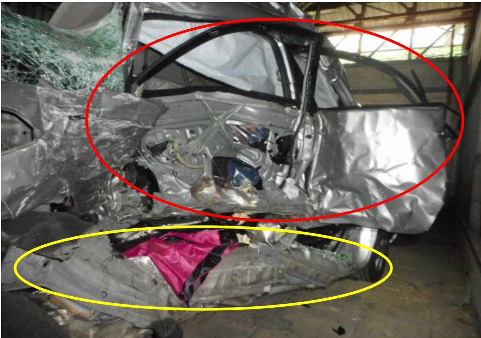
Photo 12 shows the close up view of the Motor Car's left body at the time of my inspection. The Motor car was observed to have sustained damage at its left portion. Its right doors (red circle) and left chassis (yellow circle) was amongst the body parts damaged as a result of the accident.
