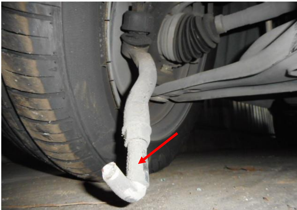
Photo 26 shows the various undercarriage components at the front left wheel of the Motor Car, in particular the steering tie rod end (arrowed) was observed to be damaged as a result of the accident.
