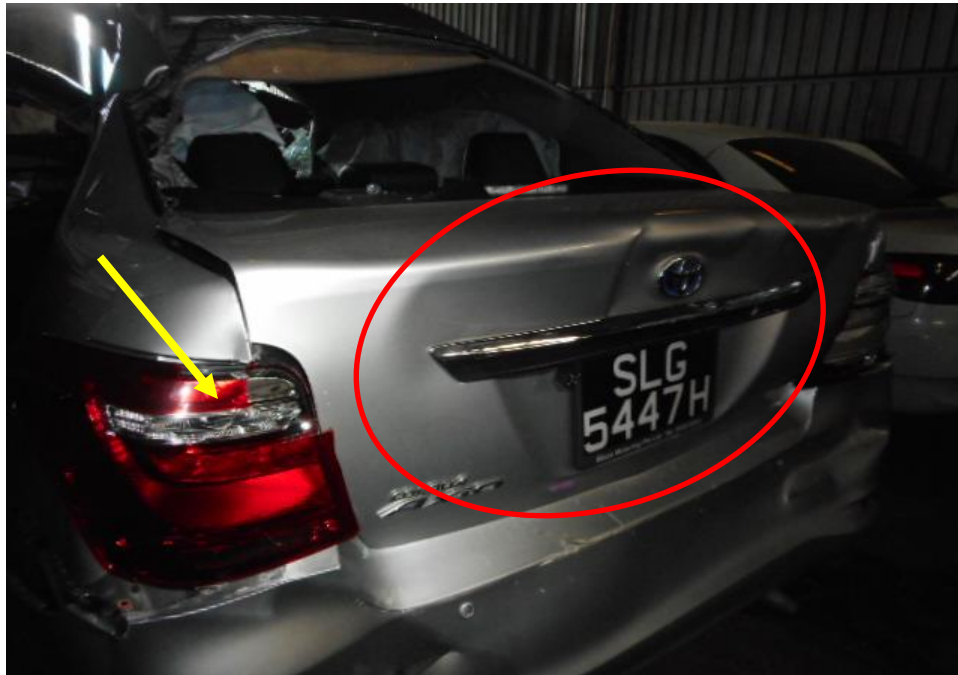
Photo 3 shows a close up view of the Motor Car's rear body at the time of my inspection. The rear portion of the Motor Car was observed to sustain damages as a result of the accident. Its rear boot (circled) and rear left brake lamp (arrowed) were damaged as a result of the accident.
