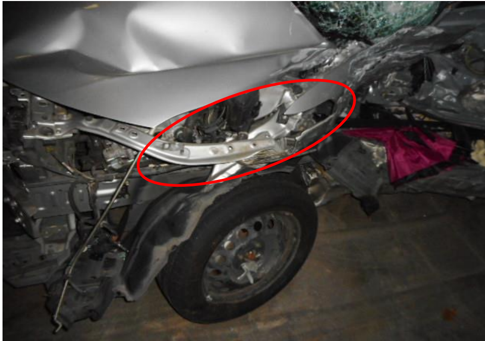
Photo 9 shows the close up view of the Motor Car's front body at the time of my inspection. The Motor car was observed to have sustained damage at its front portion. Its front right fender (circled) was amongst the body part damaged as a result of the accident.
