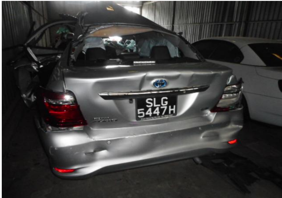
Photo 1 shows a general view of the Motor Car's rear body at the time of my inspection. The rear portion of the Motor Car was observed to sustain damages as a result of the accident. Its rear windscreen, rear boot, rear bumper, rear both brake lamps were damaged as a result of the accident.
