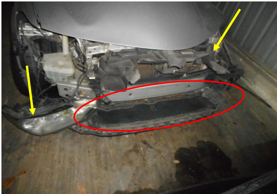
Photo 8 shows the close up view of the Motor Car's front body at the time of my inspection. The Motor car was observed to have sustained damage at its front portion. Its front bumper (circled) and its front left and right headlamps (arrowed) was damaged as a result of the accident.
