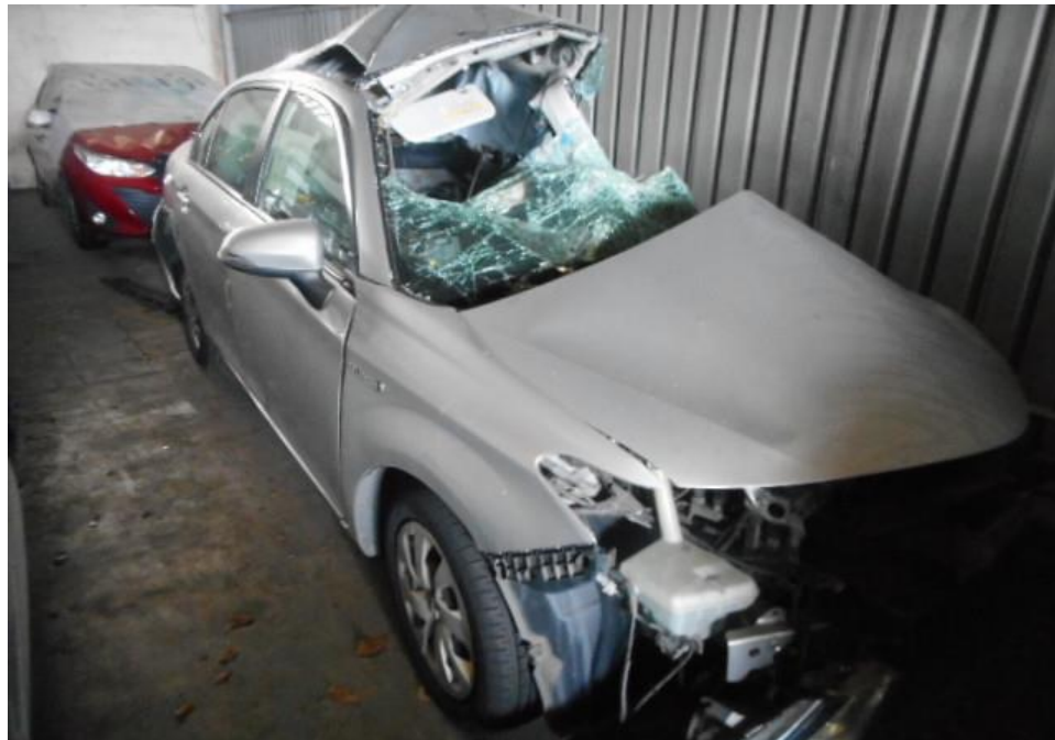
Photo 10 shows a general view of the Motor Car's right body at the time of my inspection. The right portion of the Motor Car was observed to have been removed due to the accident.
