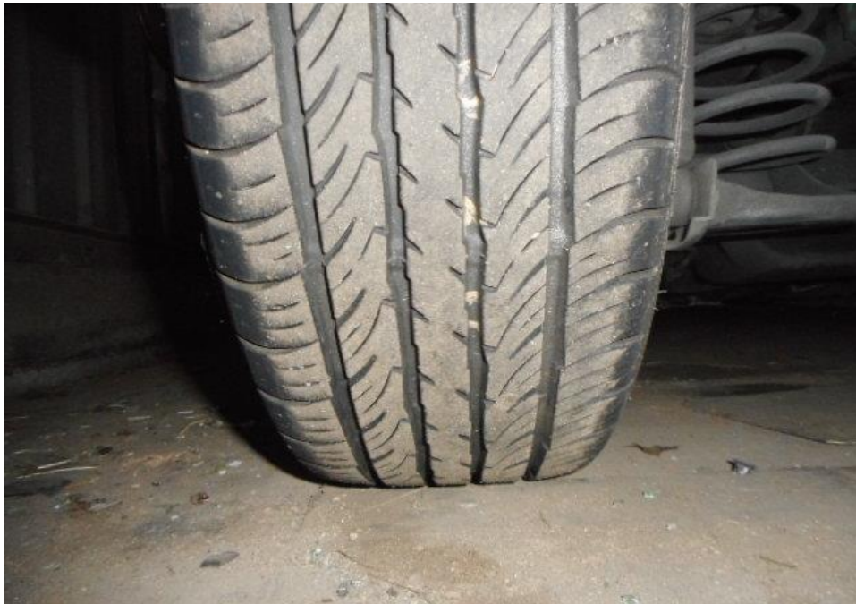
Photo 15 shows the condition of the rear left tyre of the Motor Car, which was observed to be in serviceable condition with remaining tread depth of approximately 5.7mm. The tyre was also observed to be sufficiently inflated for vehicular operation with no tear, cut or burst mark(s).
