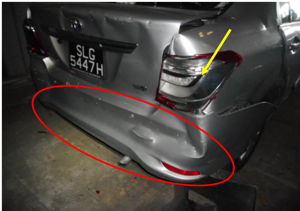
Photo 4 shows a close up view of the Motor Car's rear body at the time of my inspection. The rear portion of the Motor Car was observed to sustain damages as a result of the accident. Its rear bumper (circled) and rear right brake lamp (arrowed) were damaged as a result of the accident.
