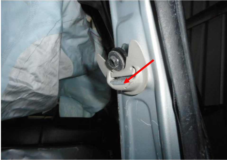
Photo 28 shows that the seat belt on the left seat was observed to be missing at the time of our inspection.
