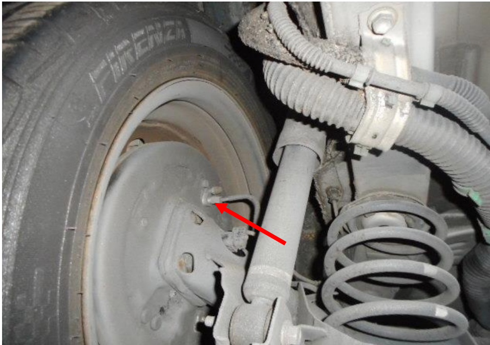
Photo 21 shows the brake hose/pipe (arrowed) at the rear left wheel of the Motor Car. No leakage of brake fluid was observed. Visual examination of the various components of the braking system like the brake drum to be intact and without visible damage.
