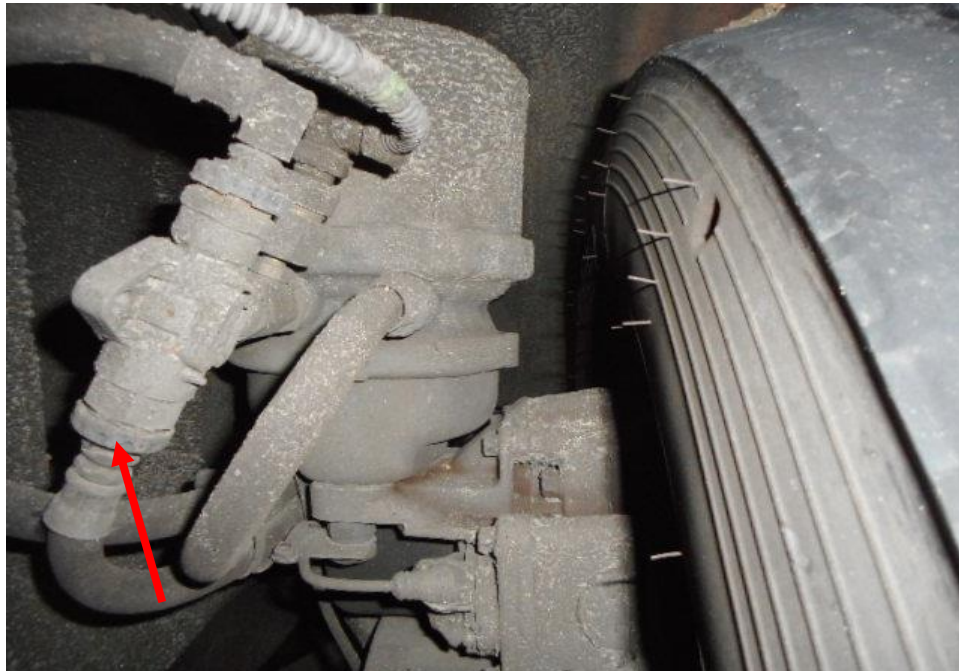
Photo 21 shows the brake pipe (arrowed) at the rear left wheel of the Motor Bus. I did not observe any leakage of brake fluid at the time of my inspection of the Motor Bus. My visual examination of the various mechanical components of the braking system where generally intact and unaffected by the accident.
