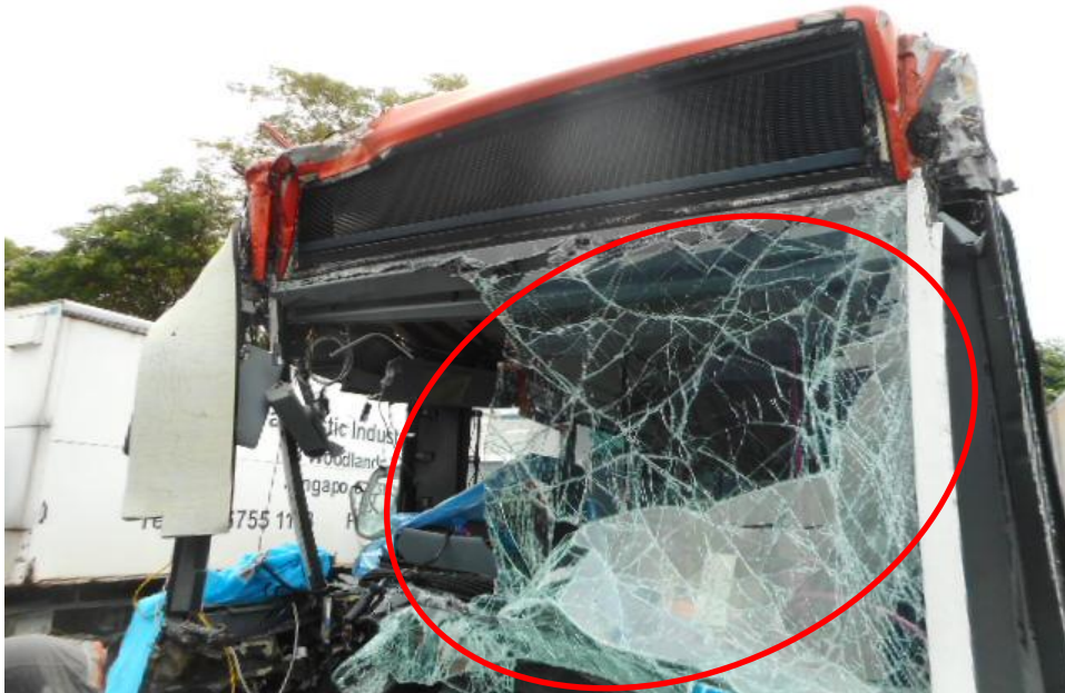
Photo 5 shows a close up view of the front body of the Motor Bus at the time of my inspection. The Motor Bus was observed to sustained damage at its front portion. Its front windscreen (circled) were damage at the time of my inspection as a result of the accident.
