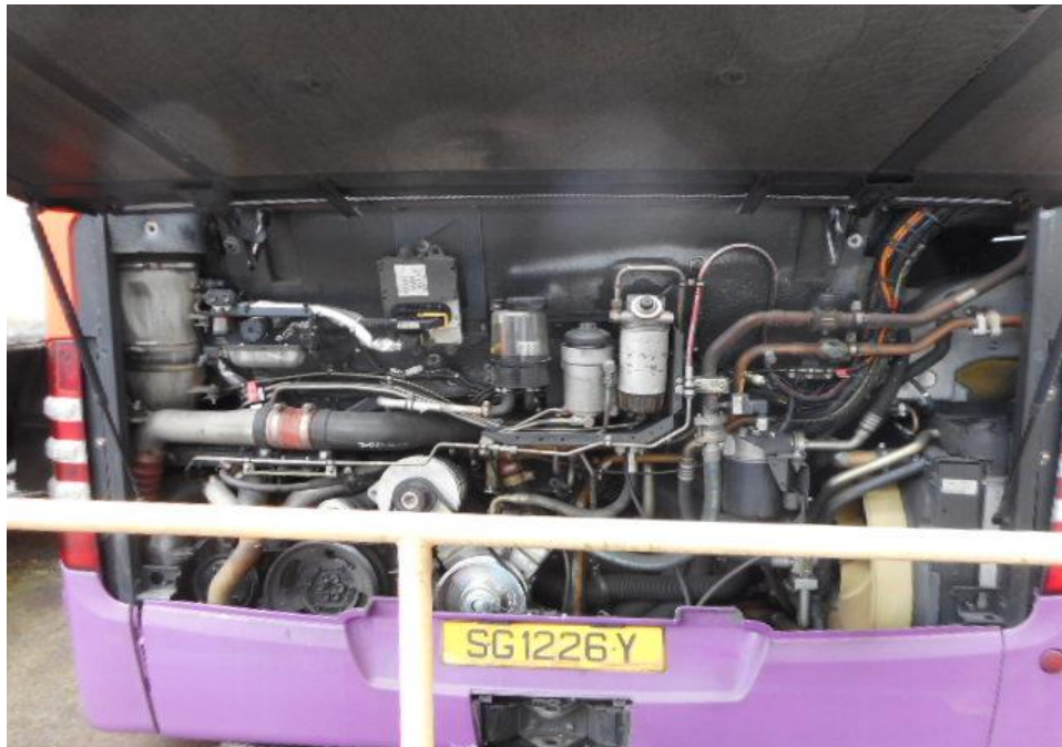
Photo 14 shows a general view of the Motor Bus's engine compartment, which was accessed by lifting the rear of the Motor Bus. The various parts and components inside the engine compartment were unaffected by the accident. There was also no sign(s) or indication(s) of fresh fluid leakage and/or fluid stain within the engine compartment
