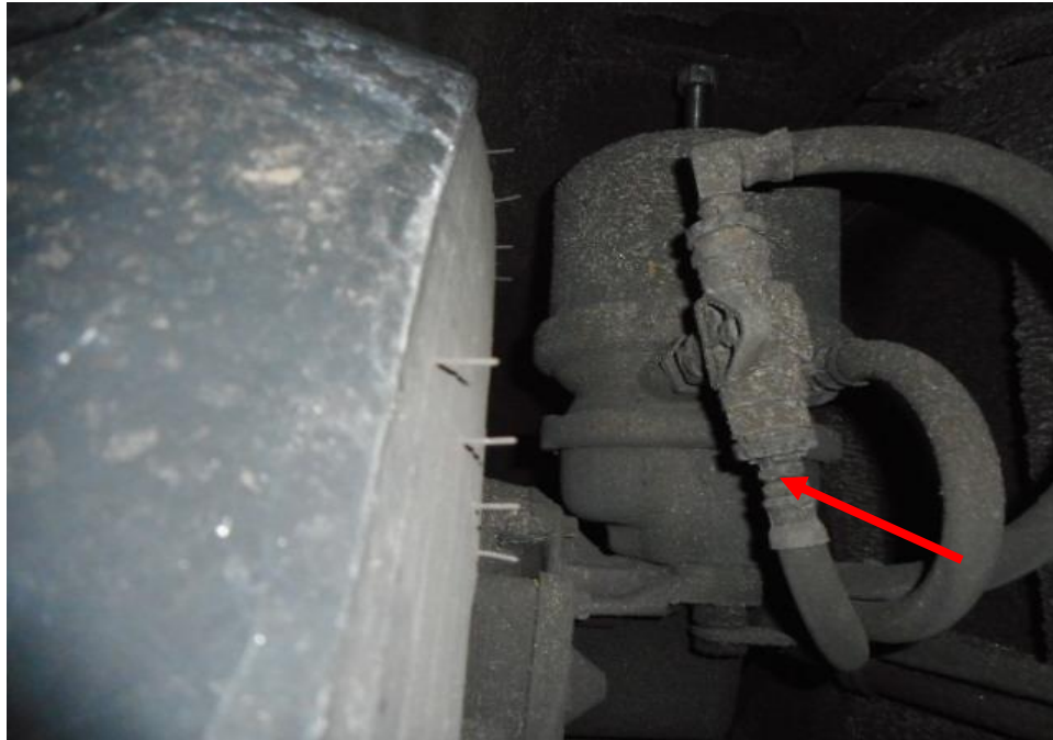
Photo 20 shows the brake pipe (arrowed) at the rear right wheel of the Motor Bus. I did not observe any leakage of brake fluid at the time of my inspection of the Motor Bus. My visual examination of the various mechanical components of the braking system where generally intact and unaffected by the accident.
