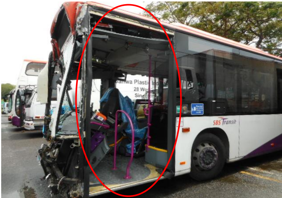
Photo 7 shows a close up of the left body of the Motor Bus at the time of my inspection. The Motor Bus was observed to sustained damage at its front portion. Its front door (circled) were damage at the time of my inspection as a result of the accident.
