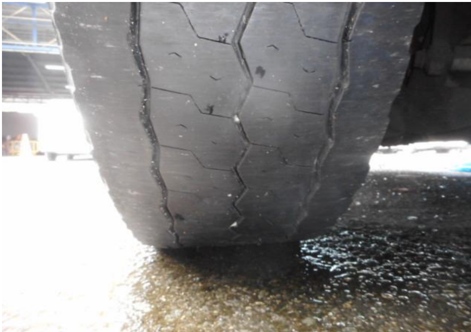
Photo 13 shows the condition of the front left tyres of the Motor Bus, which were observed to be in serviceable condition with remaining tread depth of approximately 7.5mm. There was also no tear, cut or burst mark(s) on the outer and the inner sidewalls as well as across the tread of the 6 tyres that were fitted on the Motor Bus.
