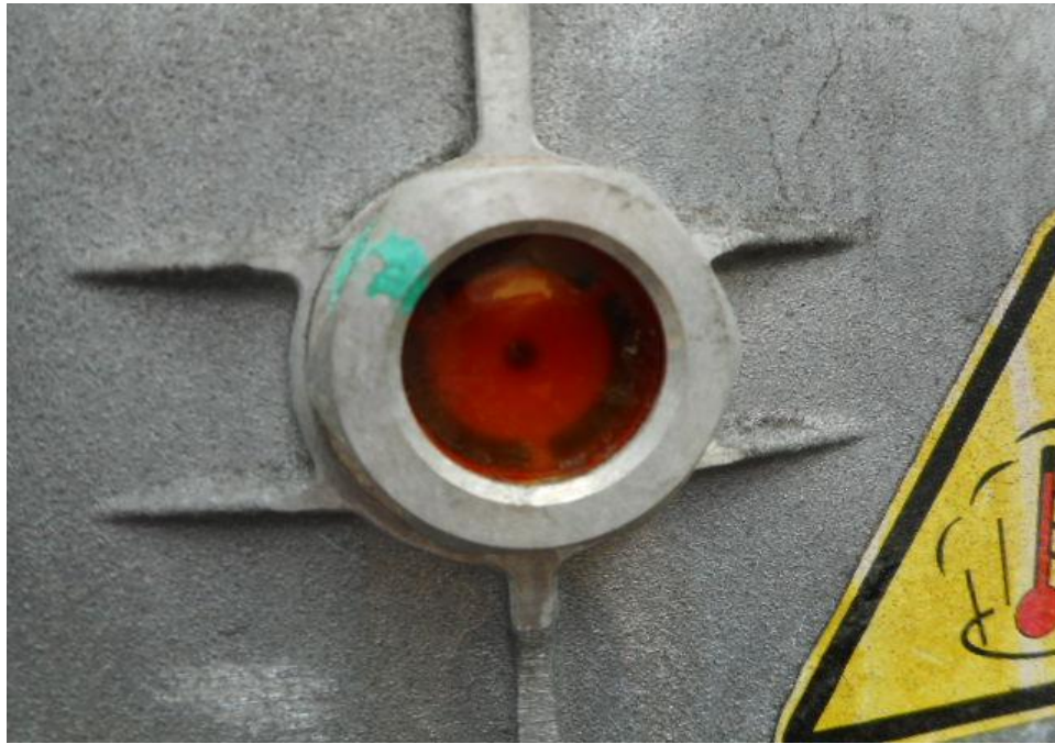
Photo 15 shows the engine coolant reservoir of the Motor Bus at the time of my inspection. The engine coolant was observed to be sufficient for operation and without any visible contamination.
