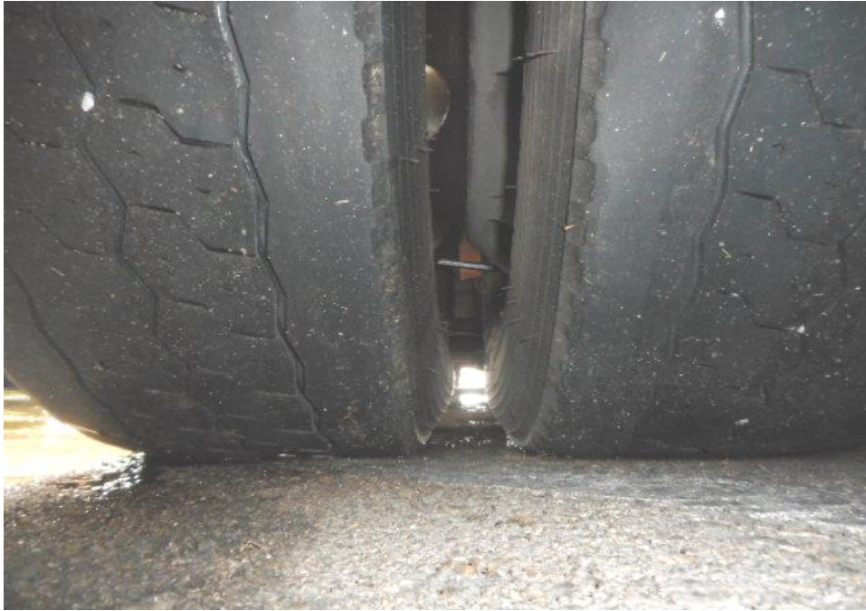
Photo 12 shows the condition of the rear left tyres of the Motor Bus, which was observed to be in serviceable condition with remaining tread depth of approximately 6.1mm. The tyres, which were wrapped around standard steel wheel rim, were also observed to be sufficiently inflated for vehicular operation. There was also no damage found on all 6 steel wheel rims of the Motor Bus.
