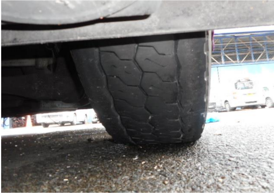
Photo 10 shows the condition of the front right tyre of the Motor Bus, which was observed to be in serviceable condition with remaining tread depth of approximately 11.5mm. The tyre, which was wrapped around standard steel wheel rim, was also observed to be sufficiently inflated for vehicular operation. There was no tear, cut or burst mark(s) on the outer and the inner sidewalls as well as across the tread of the 6 tyres that were fitted on the Motor Bus.
