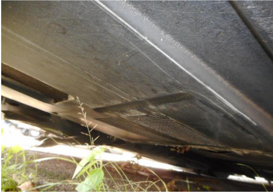
Photo 19 shows the undercarriage of the Motor Bus, at the area where the engine housing and transmission housing are located. I did not find any sign(s) or indication(s) of fluid leak and/or fluid stain(s) on the underside of the Motor Bus.
