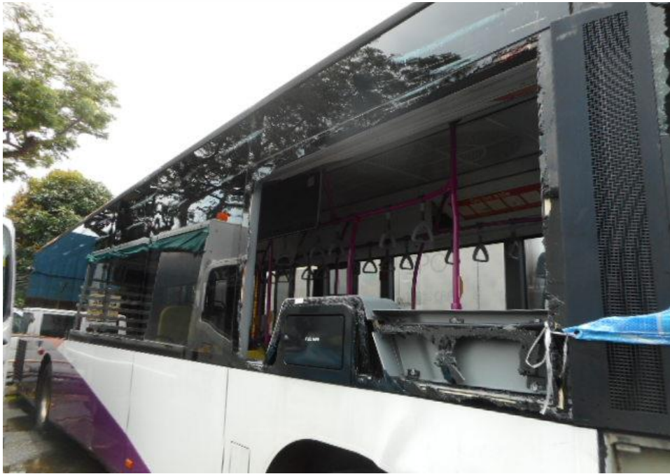
Photo 8 shows a close up view of the right portion of the Motor Bus at the time of our inspection. The right portion of the Motor Bus was observed to have been unaffected by the accident. However, the windscreen was removed by the SCDF officers for rescue procedures.
