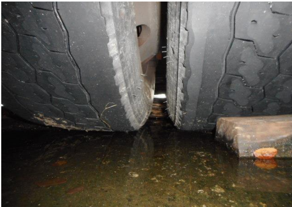
Photo 11 shows the condition of the rear right tyre of the Motor Bus, which was observed to be in serviceable condition with remaining tread depth of approximately 5.7mm. The tyre, which was wrapped around standard steel wheel rim, was also observed to be sufficiently inflated for vehicular operation.
