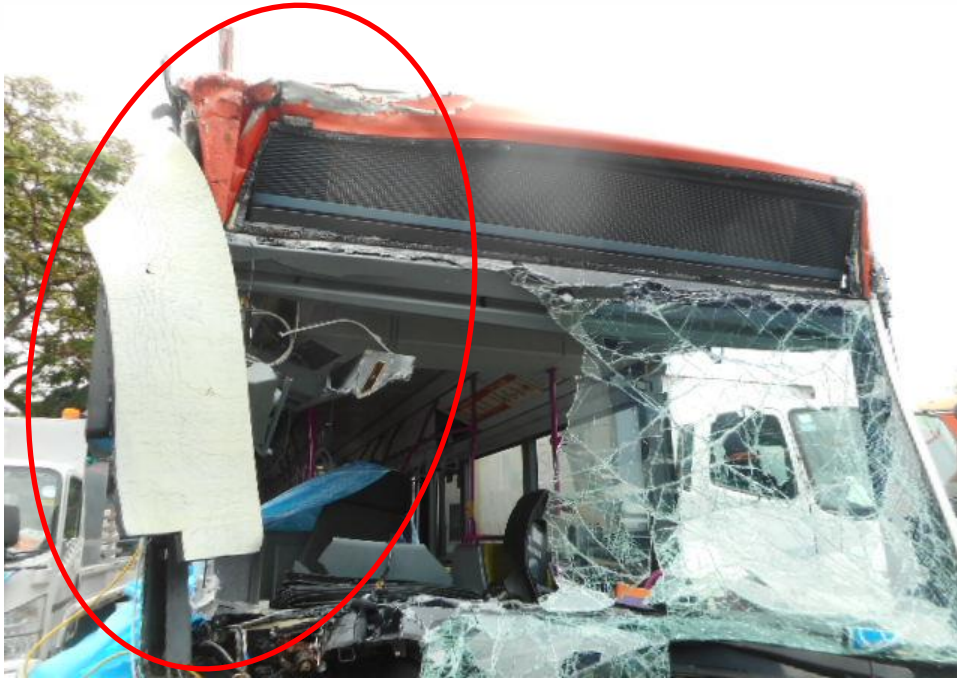
Photo 4 shows a close up view of the front body of the Motor Bus at the time of my inspection. The Motor Bus was observed to sustained damage at its front portion. Its front cabin structure (circled) were damage at the time of my inspection as a result of the accident.
