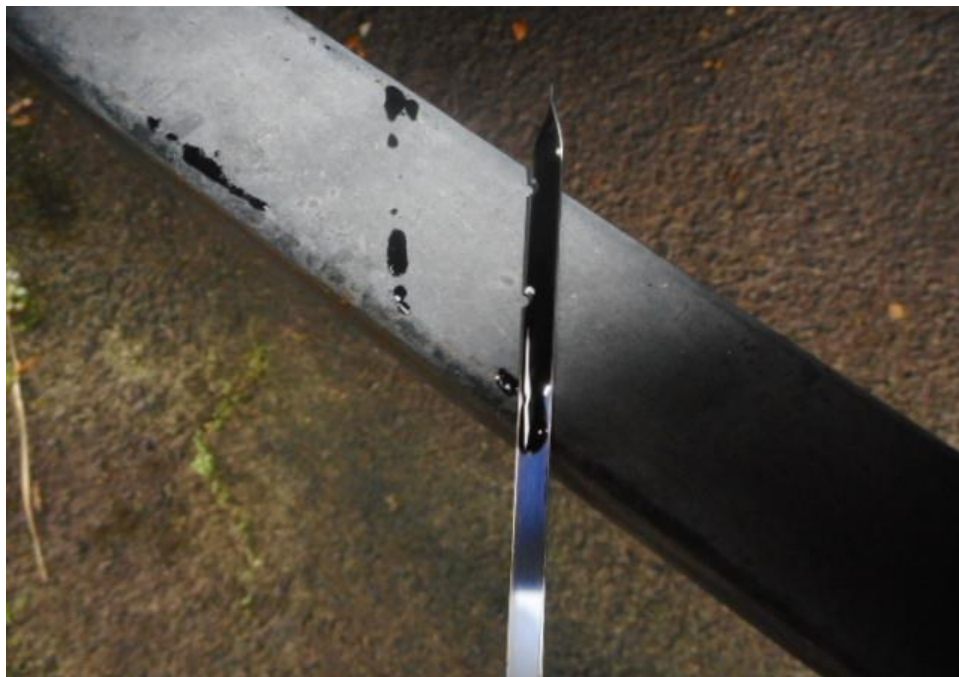
Photo 16 shows the engine oil dip stick system of the Motor Bus at the time of my inspection. The engine oil was observed to be sufficient for operation and without any visible contamination.
