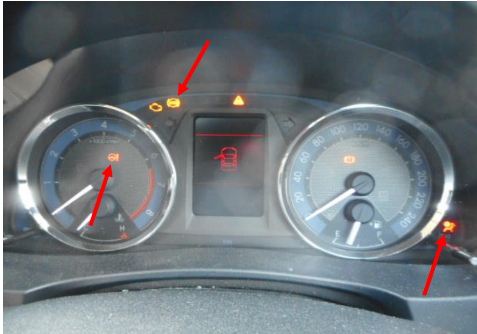
Photo 25 shows the warning light for Anti-Lock Brake System (ABS), Electric Power Steering System (EPS) and Supplemental Restraint System (SRS) (arrowed) appearing on the instrument panel of the Motor Car during the self-test of its various electronic operating systems when its engine was cranked.
