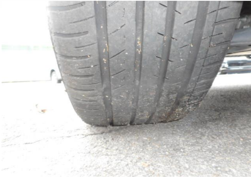
Photo 12 shows the condition of the front left tyre of the Motor Car, which was observed to be in serviceable condition with remaining tread depth of approximately 5.5mm. There was also no tear, cut or burst mark(s) on the outer and the inner sidewalls as well as across the tread of the Motor Car's 4 tyres.
