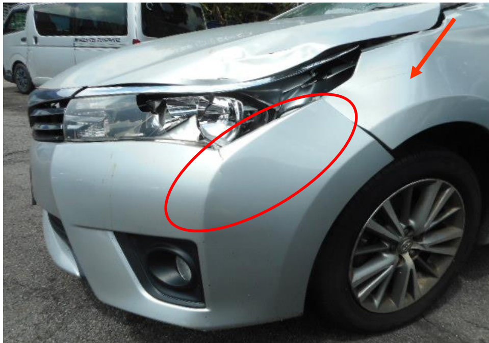
Photo 5 shows a close up view of the Motor Car's front body at the time of my inspection. The front portion of the Motor Car was observed to have sustained damage. Its front bumper (circled) and front left fender (arrowed) was the body parts that were damaged as a result of the accident.
