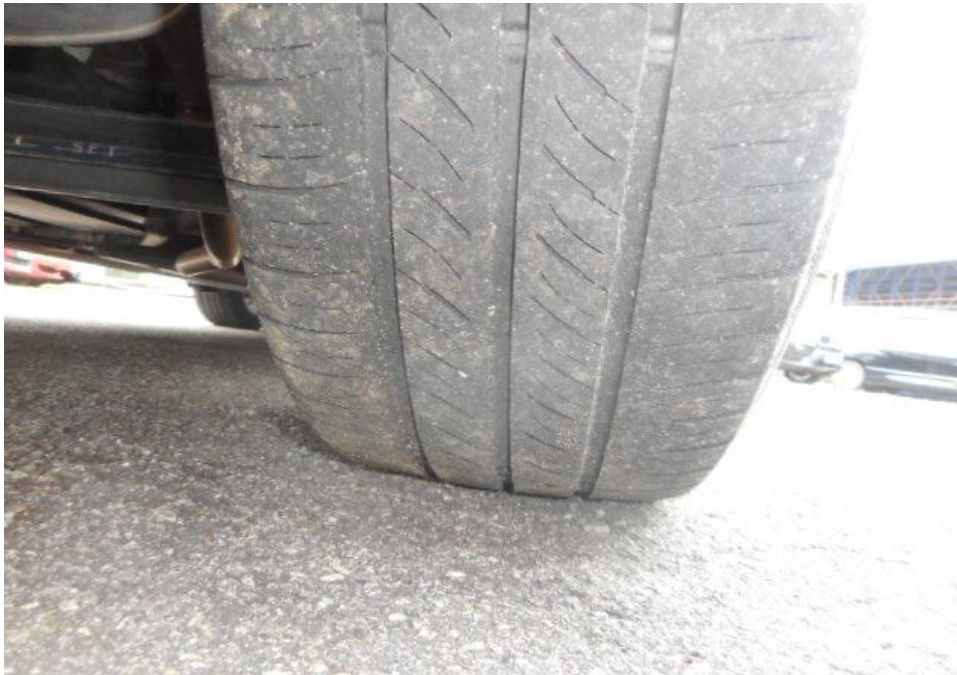
Photo 10 shows the condition of the rear right tyre of the Motor Car, which was observed to be in serviceable condition with remaining tread depth of approximately 4mm. The tyre was also observed to be sufficiently inflated for vehicular operation with no tear, cut or burst mark(s).
