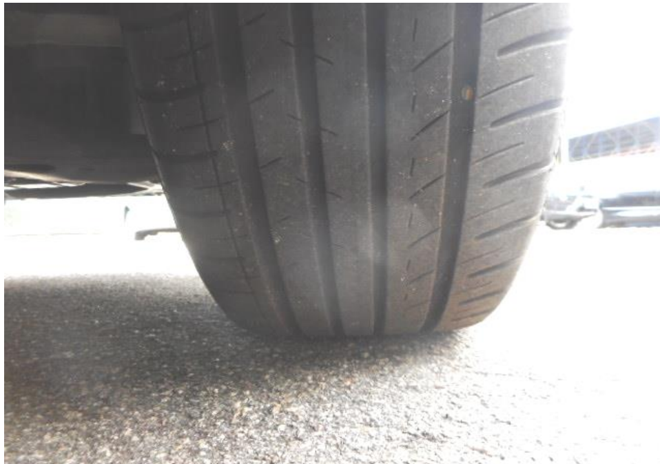
Photo 9 shows the condition of the front right tyre of the Motor Car, which was observed to be in serviceable condition with remaining tread depth of approximately 4.8mm. The tyre was sufficiently inflated for vehicular operation with no tear, cut or burst mark(s) on the outer and the inner sidewalls as well as across the tread. The 4 tyres of the Motor Car were wrapped around standard steel wheel rims without any damage.
