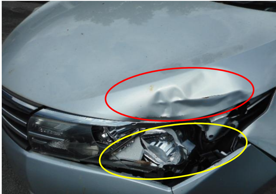
Photo 4 shows a close up view of the Motor Car's front body at the time of my inspection. The front portion of the Motor Car was observed to have sustained damage. Its front bonnet (red circle) and front left headlamp (yellow circle) was the body parts that were damaged as a result of the accident.
