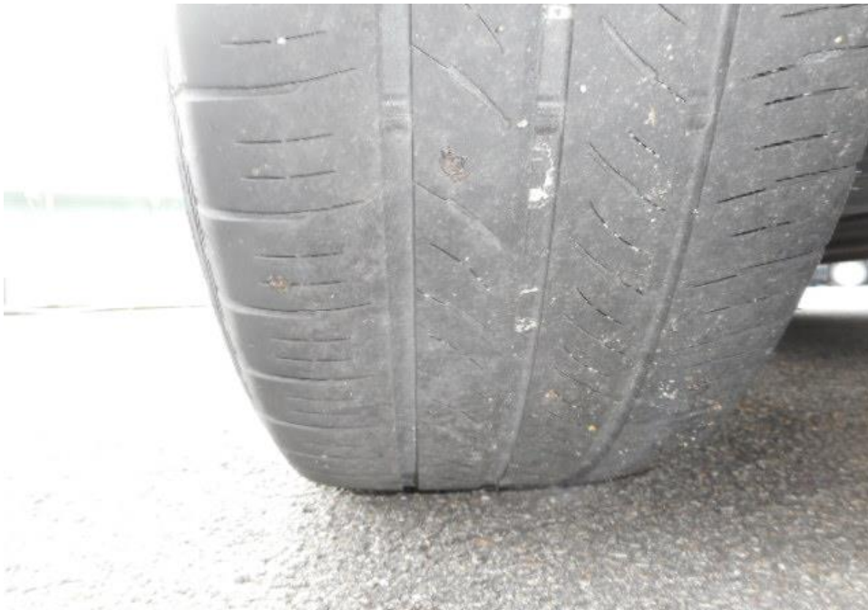
Photo 11 shows the condition of the rear left tyre of the Motor Car, which was observed to be in serviceable condition with remaining tread depth of approximately 2.6mm. The tyre, which was wrapped around steel wheel rim, was also observed to be sufficiently inflated for vehicular operation. The 4 tyres of the Motor Car were wrapped around standard steel wheel rims.
