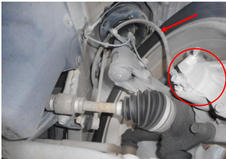
Photo 21 shows the brake hose/pipe (arrowed) at the front left wheel of the Motor Car. No leakage of brake fluid was observed. Visual examination of the various components of the braking system like the brake caliper (circled), brake booster, brake pedal etc had revealed all to be intact and without visible damage.
