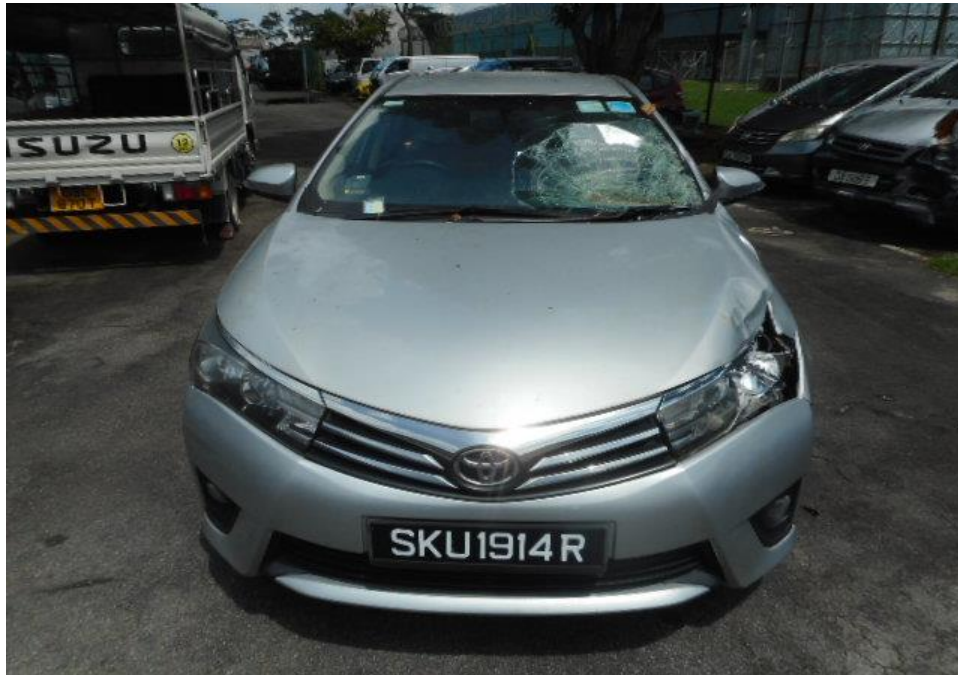
Photo 2 shows a general view of the Motor Car's front body at the time of my inspection. The front portion of the Motor Car was observed to have sustained damage. Its front windscreen, front bonnet, front bumper, front left fender and front left headlamp plate was amongst the body parts that were damaged as a result of the accident.
