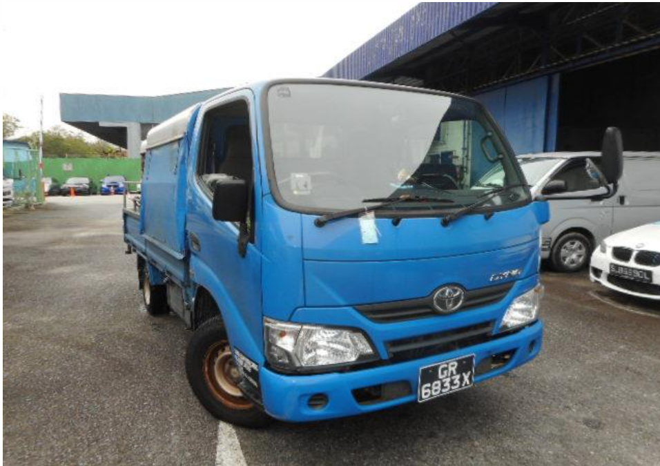
Photo 20 shows the front right wheel of the Motor Lorry turned to its full left. During my steering system test, I did not experience any abnormal free play and/or resistance when I had turned the steering wheel towards the left and right. This would suggest that the steering system of the Motor Lorry was likely to be in serviceable condition at the material time of accident.
