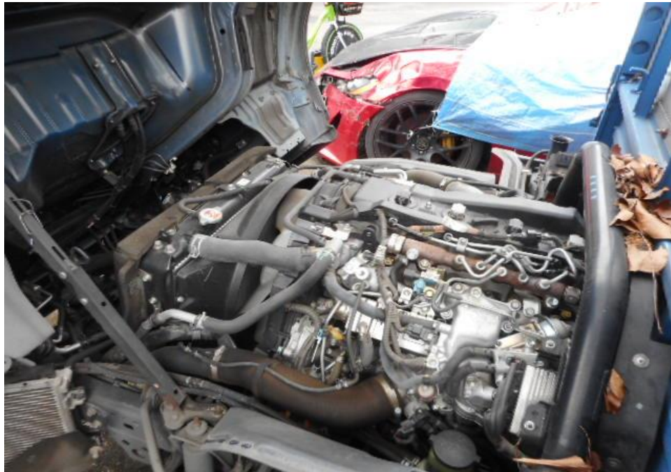
Photo 10 shows a general view of the Motor Lorry's engine compartment. The various parts and components inside the engine compartment were unaffected by the accident. There was also no sign(s) or indication(s) of fluid leakage and/or fluid stain within the engine compartment.
