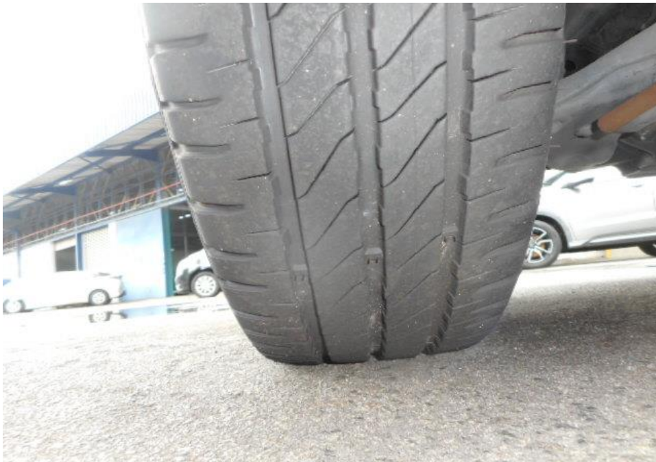
Photo 9 shows the condition of the front left tyre of the Motor Lorry, which was observed to be in serviceable condition with remaining tread depth of approximately 5.8mm. There was also no tear, cut or burst mark(s) on the outer and the inner sidewalls as well as across the tread of the Motor Lorry's 6 tyres.
