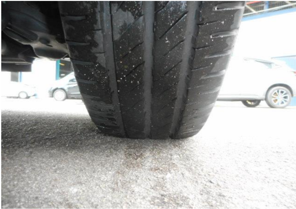
Photo 6 shows the condition of the front right tyre of the Motor Lorry, which was observed to be in serviceable condition with remaining tread depth of approximately 6.3mm. The tyre was sufficiently inflated for vehicular operation with no tear, cut or burst mark(s) on the outer and the inner sidewalls as well as across the tread. The 6 tyres of the Motor Lorry were wrapped around standard steel wheel rims without any damage.
