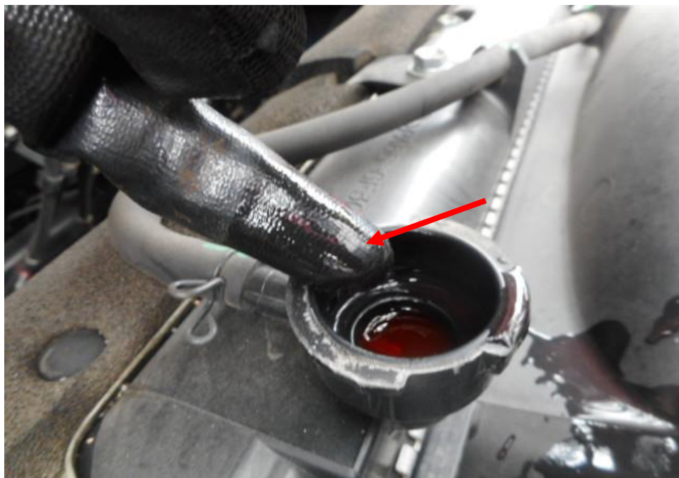
Photo 12 shows checks being carried out to the engine coolant of the Motor Lorry at the time of my inspection. The engine coolant was observed to be of sufficient level (arrowed) and without any visible contamination.
