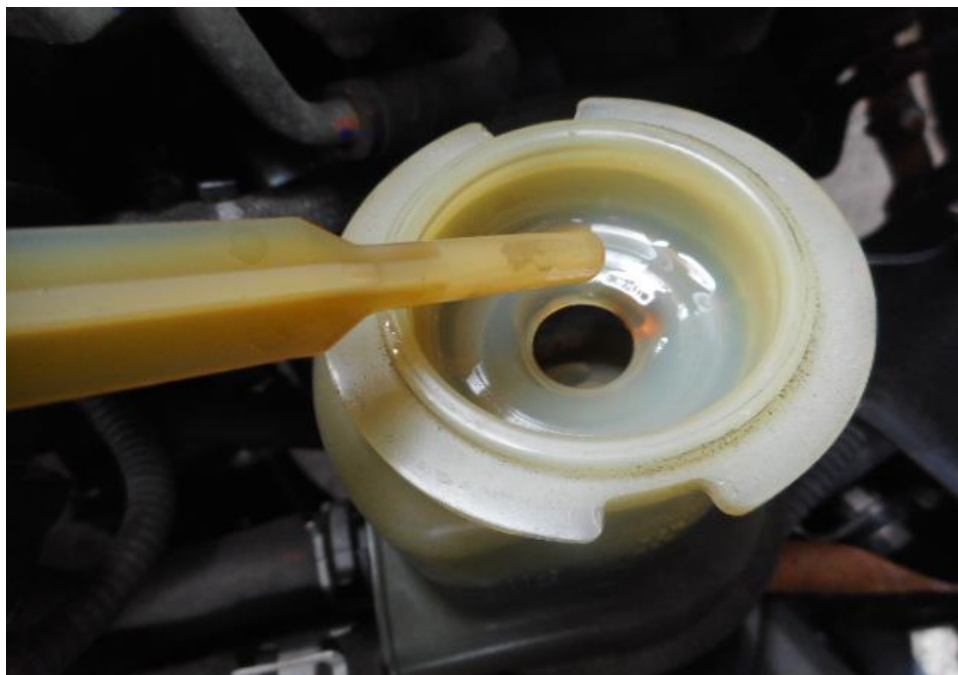
Photo 14 shows the power steering fluid dip stick of the Motor Lorry at the time of my inspection. The power steering fluid was observed to be of sufficient level and without any visible contamination.
