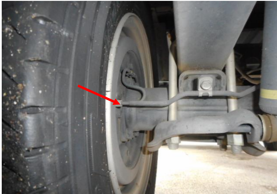
Photo 17 shows the brake hose/pipe (arrowed) at the rear left wheel of the Motor Lorry. I did not observe any leakage of brake fluid at the time of my inspection of the Motor Lorry. Static tests of the Motor Lorry's braking system had indicated that there was no internal leakage of pressure/vacuum. The undercarriage components of the Motor Lorry were also all found to be intact and without any visible damage.
