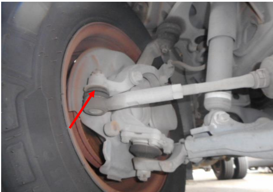
Photo 21 shows the various undercarriage components at the front right wheel of the Motor Lorry, in particular the steering tie rod (arrowed). The various steering components were all found to be intact, suggesting that the steering system of the Motor Lorry was likely to be in serviceable condition at the material time of accident. There was also no sign of fluid stain observed on the various undercarriage components at the front right wheel of the Motor Lorry.
