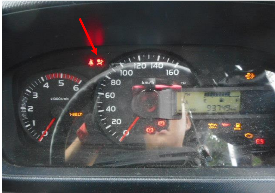
Photo 23 shows the warning light for Supplemental Restraint System (SRS) (arrowed) appearing on the instrument panel of the Motor Lorry during the self-test of its various electronic operating systems when its engine was cranked.
