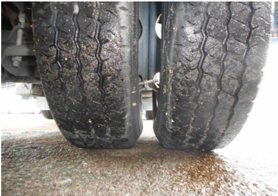
Photo 7 shows the condition of the rear right tyre of the Motor Lorry, which was observed to be in serviceable condition with remaining tread depth of approximately 3.5mm. The tyre was also observed to be sufficiently inflated for vehicular operation with no tear, cut or burst mark(s).
