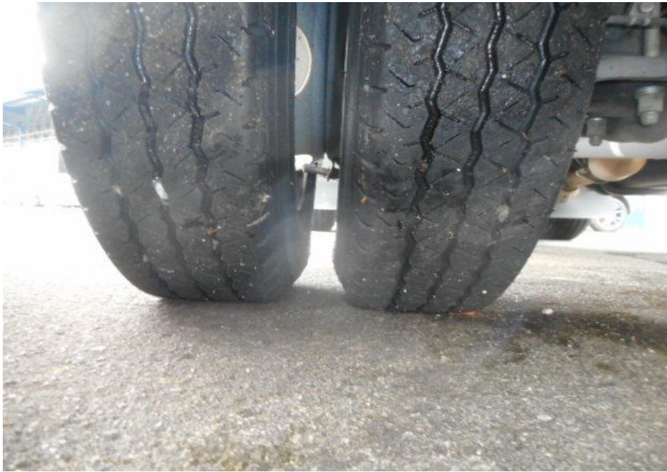
Photo 8 shows the condition of the rear left tyre of the Motor Lorry, which was observed to be in serviceable condition with remaining tread depth of approximately 3.1mm. The tyre, which was wrapped around steel wheel rim, was also observed to be sufficiently inflated for vehicular operation. The 6 tyres of the Motor Lorry were wrapped around standard steel wheel rims.
