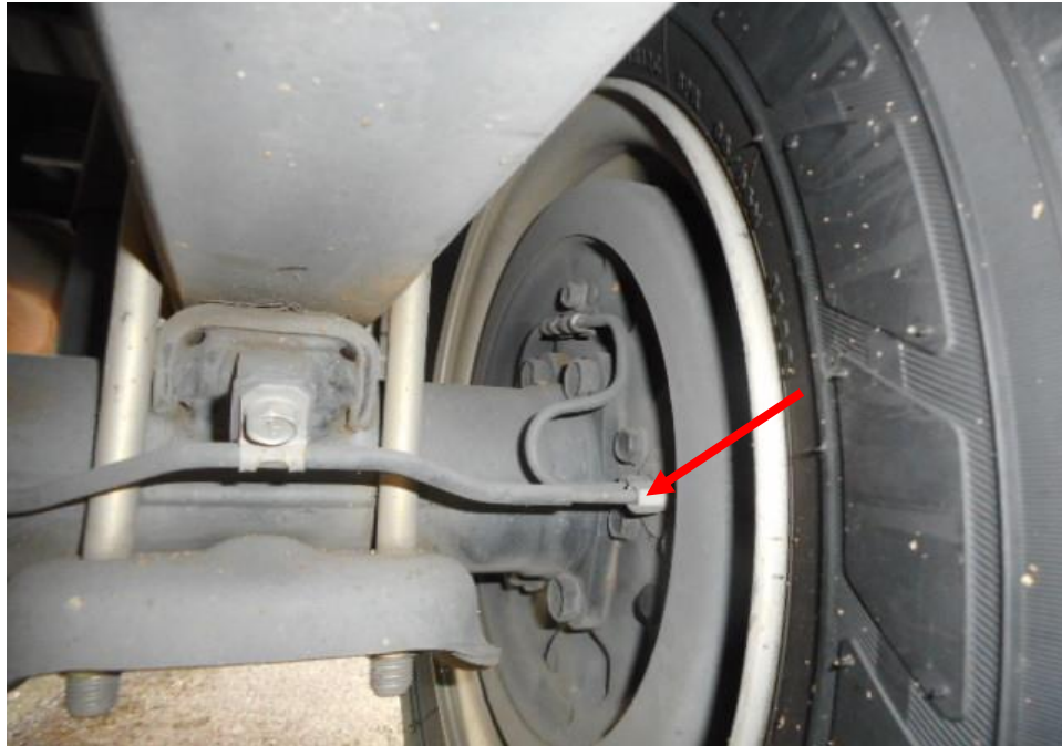
Photo 16 shows the brake hose/pipe (arrowed) at the rear right wheel of the Motor Lorry. No leakage of brake fluid was observed. Visual examination of the various components of the braking system like the drum brake, brake booster, brake pedal etc. had revealed all to be intact and without visible damage.
