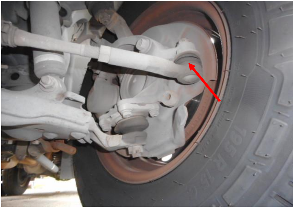
Photo 22 shows the various undercarriage components at the front left wheel of the Motor Lorry, which had included the steering tie rod (arrowed). The various undercarriage components of the Motor Lorry were all found to be intact without any visible damage.
