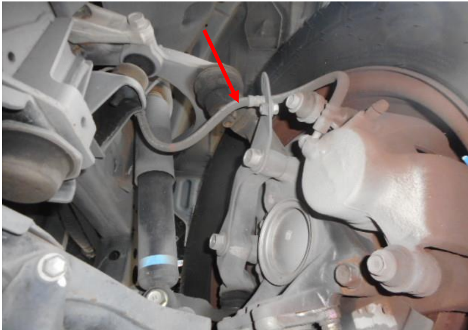
Photo 18 shows the brake hose/pipe (arrowed) at the front right wheel of the Motor Lorry. I did not observe any leakage of brake fluid at the time of my inspection of the Motor Lorry. Static tests of the Motor Lorry's braking system had indicated that there was no internal leakage of pressure/vacuum. The undercarriage components of the Motor Lorry were also all found to be intact and without any visible damage.
