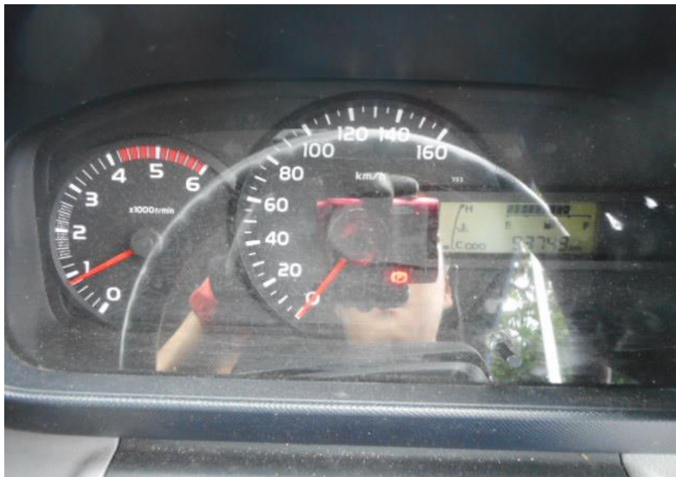
Photo 24 shows no warning lights illuminated on the instrument panel of the Motor Lorry after the engine was cranked. This would suggest that there was no abnormality to the electronic operating system of the Motor Lorry, like the SRS and etc.
