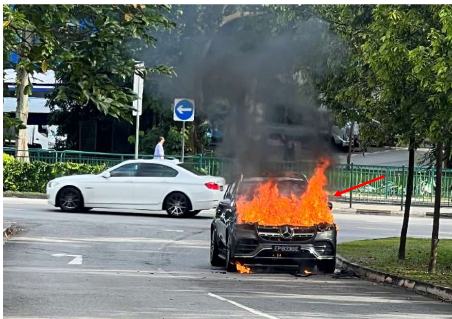
Photo 12 shows the Insured Vehicle on fire before the arrival of the SCDF. In general, the information that could be gathered from this photograph had corresponded to the events that were related to us by Mr Lee which is the fire had started from the engine compartment of the Insured Vehicle (arrowed).
