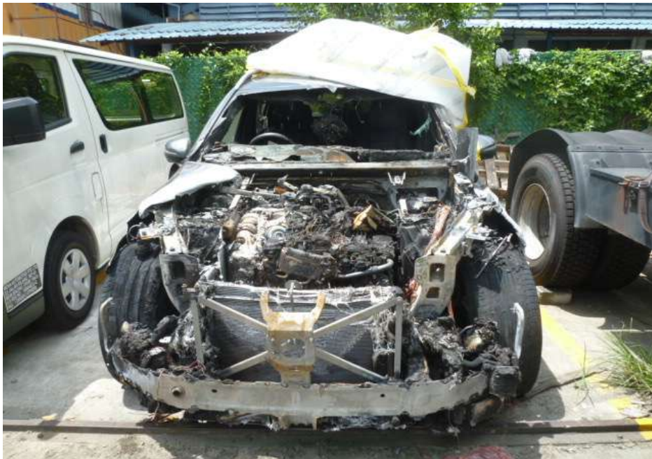
Photo 2 shows the general view of the frontal portion of the Insured Vehicle at the time of our inspection. The fire damage to the Insured Vehicle was confined to its frontal portion. The entire engine compartment of the Insured Vehicle was observed to be severely burnt while the interior compartment was observed to be seriously affected by the fire.
