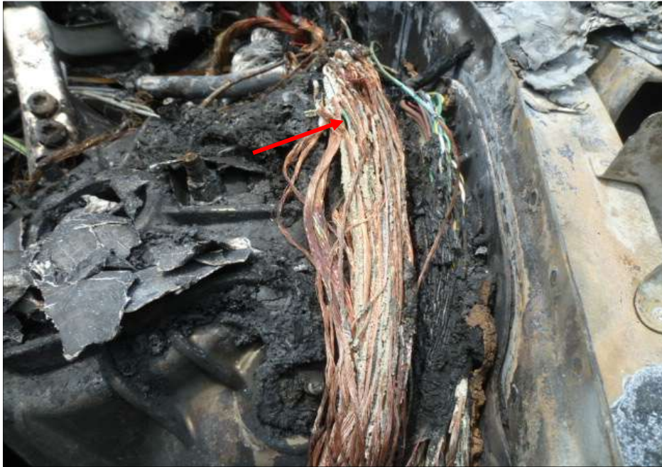
Photo 8 shows a closer view of the greenish residue on some of the burnt wirings of the Insured Vehicle (arrowed). The presence of greenish residue indicates internal heating of copper wires, a sign of an electrical short circuit occurring. The greenish residue is normally left behind from oxidation as a result of chemical reaction involving the copper wires.
