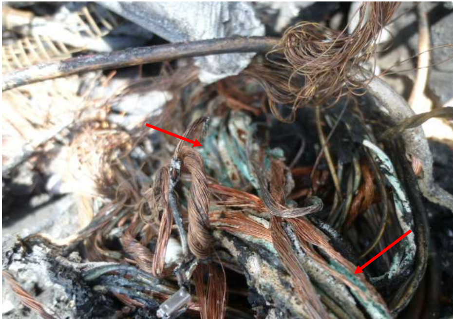
Photo 10 shows a close up view of the greenish residue on the wirings of the Insured Vehicle (red arrows). The presence of such greenish residue suggests occurrence of an electrical short circuit.
