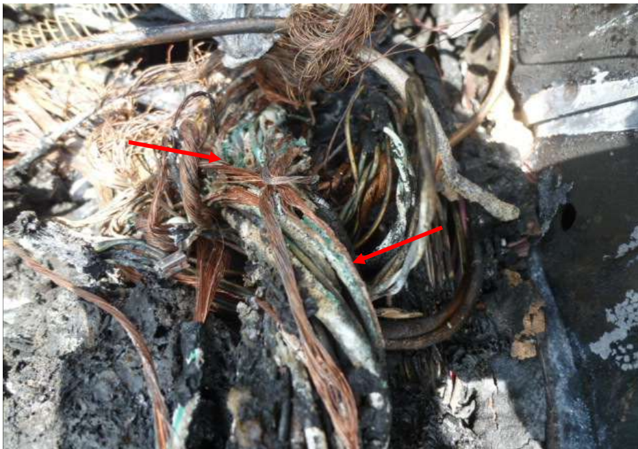
Photo 9 shows a closer view of the greenish residue on the wirings of the Insured Vehicle (red arrows). The presence of such greenish residue suggests occurrence of an electrical short circuit.
