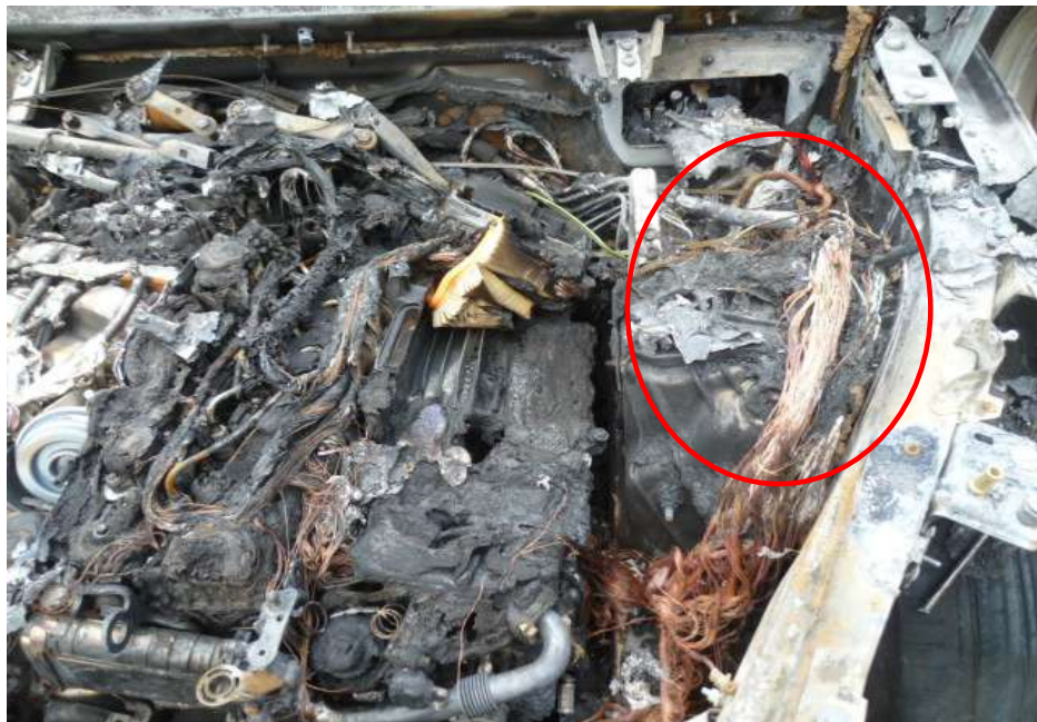
Photo 7 shows the wirings around the rear left portion of the engine compartment which is near to the vicinity where the fire to the Insured Vehicle had likely started. We observed greenish residue on some of the burnt wirings of the Insured Vehicle (circled). The presence of greenish residue indicates internal heating of copper wires, a sign of an electrical short circuit occurring.
