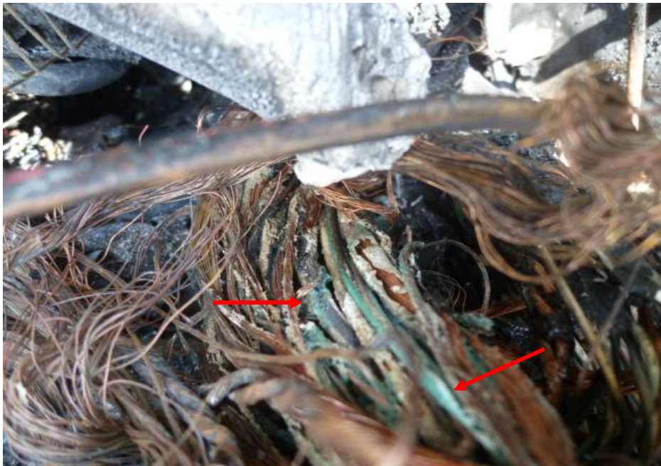
Photo 11 shows a close up view of the greenish residue on the wirings of the Insured Vehicle (red arrows). The presence of such greenish residue suggests occurrence of an electrical short circuit.
