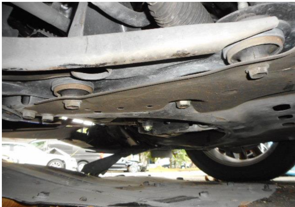
Photo 19 shows the undercarriage of the Motor Taxi, at the area where the engine housing and transmission housing are located. I did not find any sign(s) or indication(s) of fluid leak and/or fluid stain(s) on the underside of the Motor Taxi.
