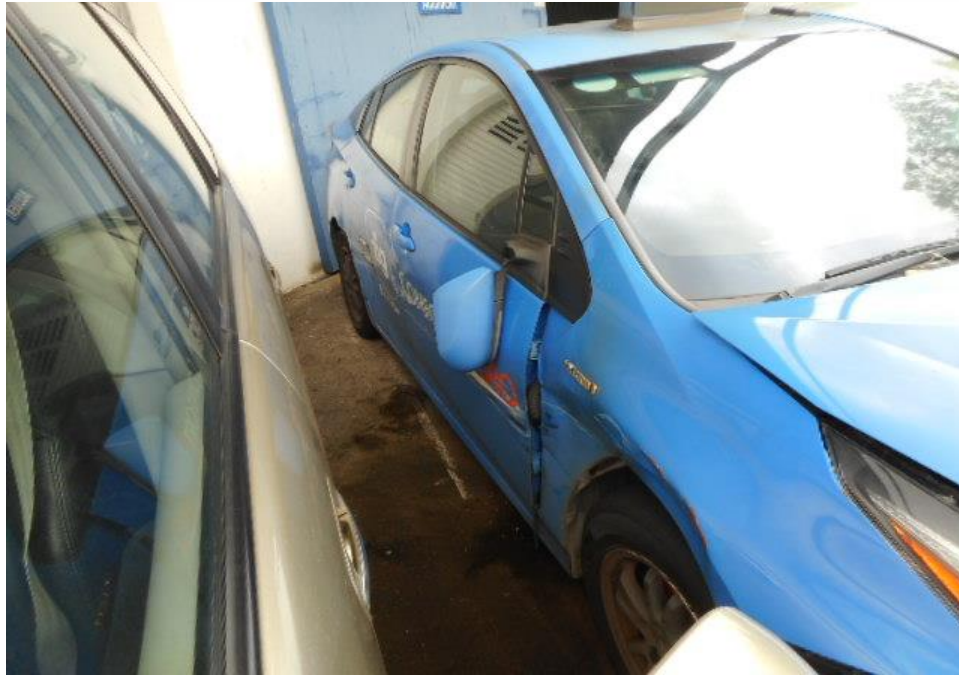
Photo 5 shows a general view of the Motor Taxi's right body at the time of my inspection. The right portion of the Motor Taxi was observed to have sustained damages as a result of the accident. Its right door panel and its right rear view mirror was damaged as a result of the accident.
