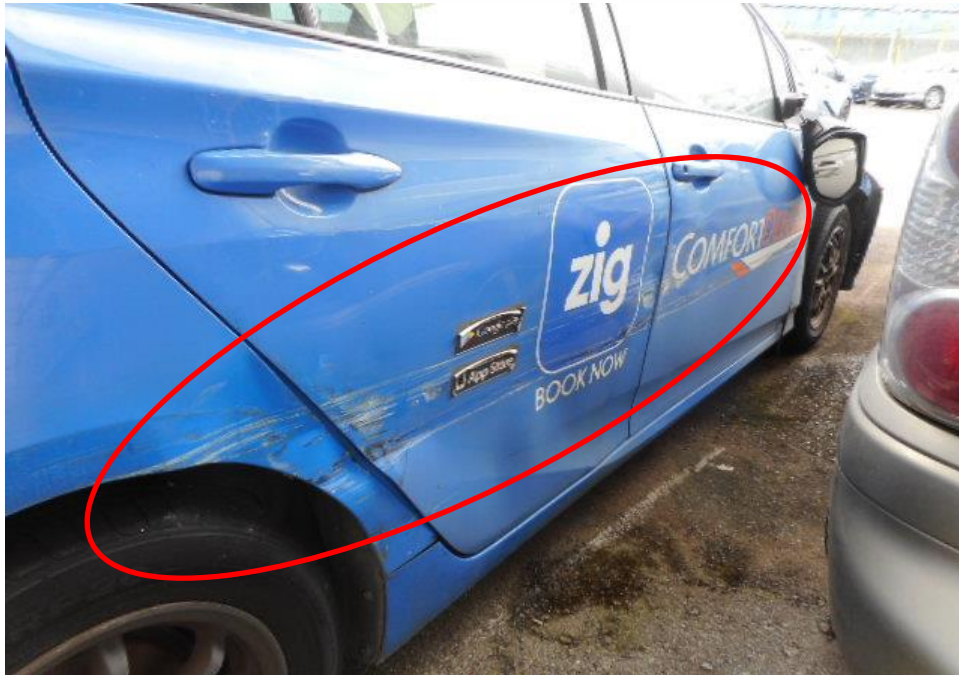
Photo 7 shows the close up view of the Motor Taxi's right body at the time of my inspection. The Motor Taxi was observed to have sustained damage at its right portion. Its right body panel (circled) was damaged as a result of the accident.
