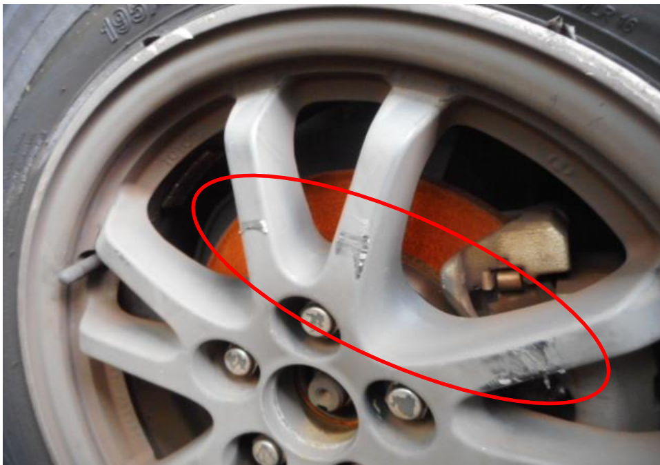
Photo 10 shows the close up condition of the front wheel rim of the Motor Taxi. The wheel rim (circled) was observed to sustained minor damages as a result of the accident.
