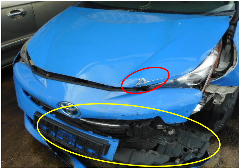
Photo 3 shows the close up view of the Motor Taxi's front body at the time of my inspection. The Motor Taxi was observed to have sustained damage at its front portion. Its front bonnet (red circle) and front bumper (yellow circle) was damaged as a result of the accident.
