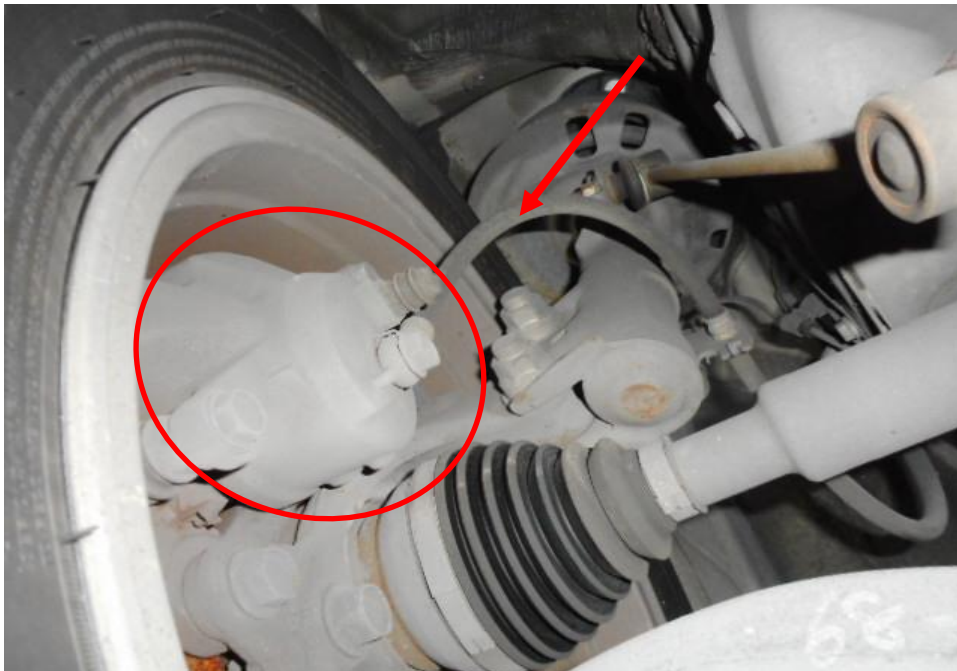
Photo 22 shows the brake hose/pipe (arrowed) at the front right wheel of the Motor Taxi. I did not observe any leakage of brake fluid at the time of my inspection of the Motor Taxi. Static tests of the Motor Taxi's braking system had indicated that there was no internal leakage of pressure/vacuum.
