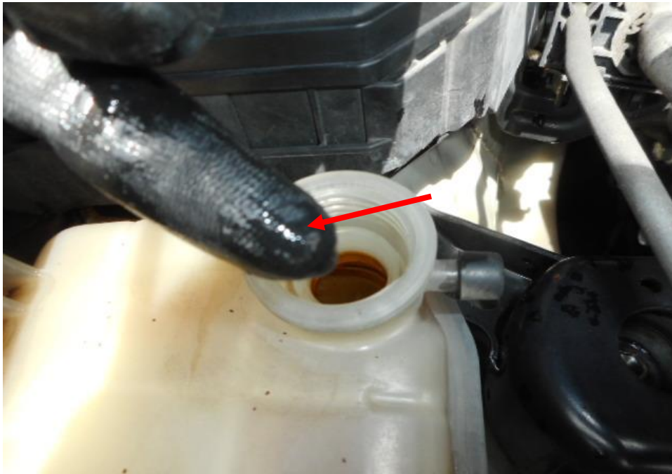
Photo 16 shows the coolant reservoir of the Motor Taxi at the time of my inspection. The coolant fluid was observed to be of sufficient level (arrowed) and without any visible contamination.
