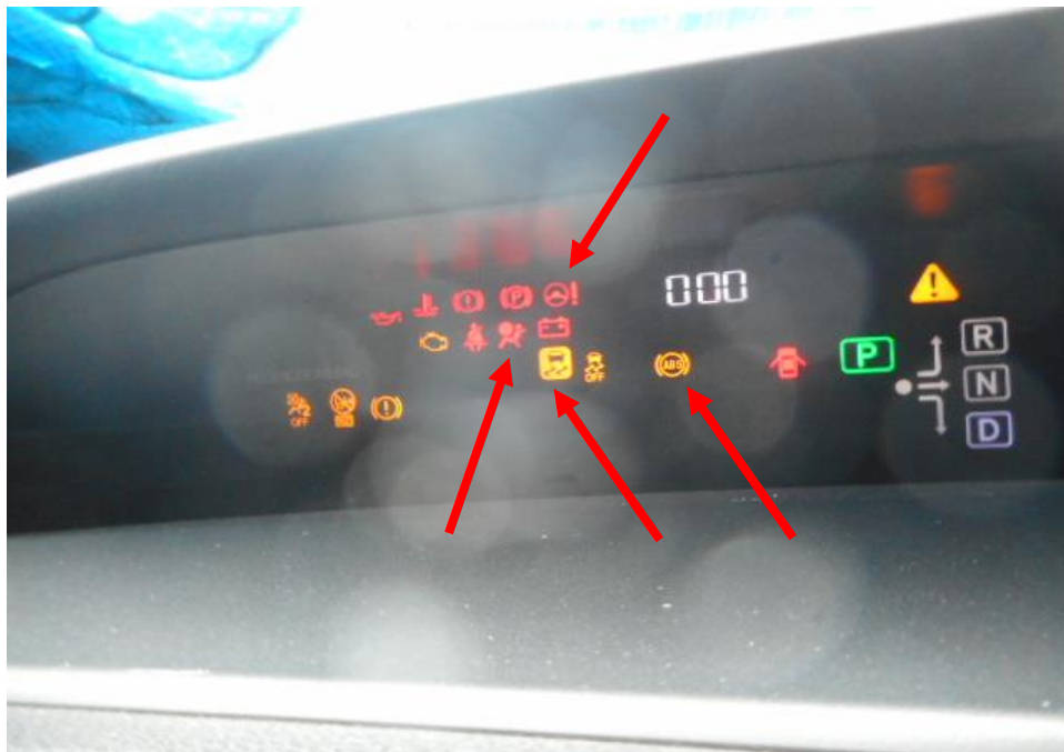
Photo 27 shows the warning light for Anti-Lock Brake System (ABS), Electric Power Steering System (EPS), Traction Control System (TCS) and Supplemental Restraint System (SRS) (arrowed) appearing on the instrument panel of the Motor Taxi during the self-test of its various electronic operating systems when its engine was cranked.
