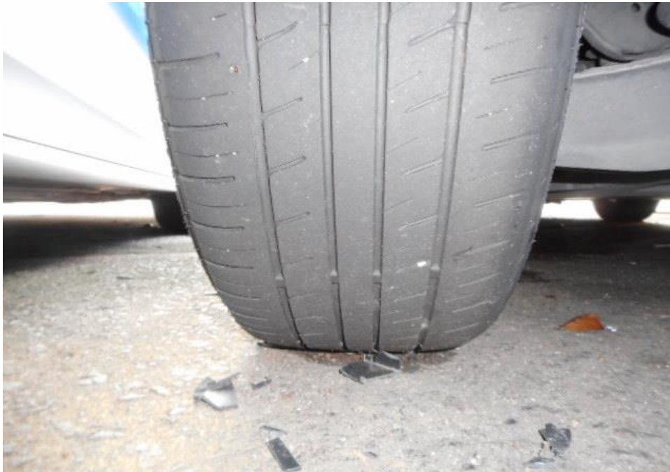
Photo 13 shows the condition of the rear left tyre of the Motor Taxi, which was observed to be in serviceable condition with remaining tread depth of approximately 3.3mm. The tyre was also observed to be sufficiently inflated for vehicular operation with no tear, cut or burst mark(s).
