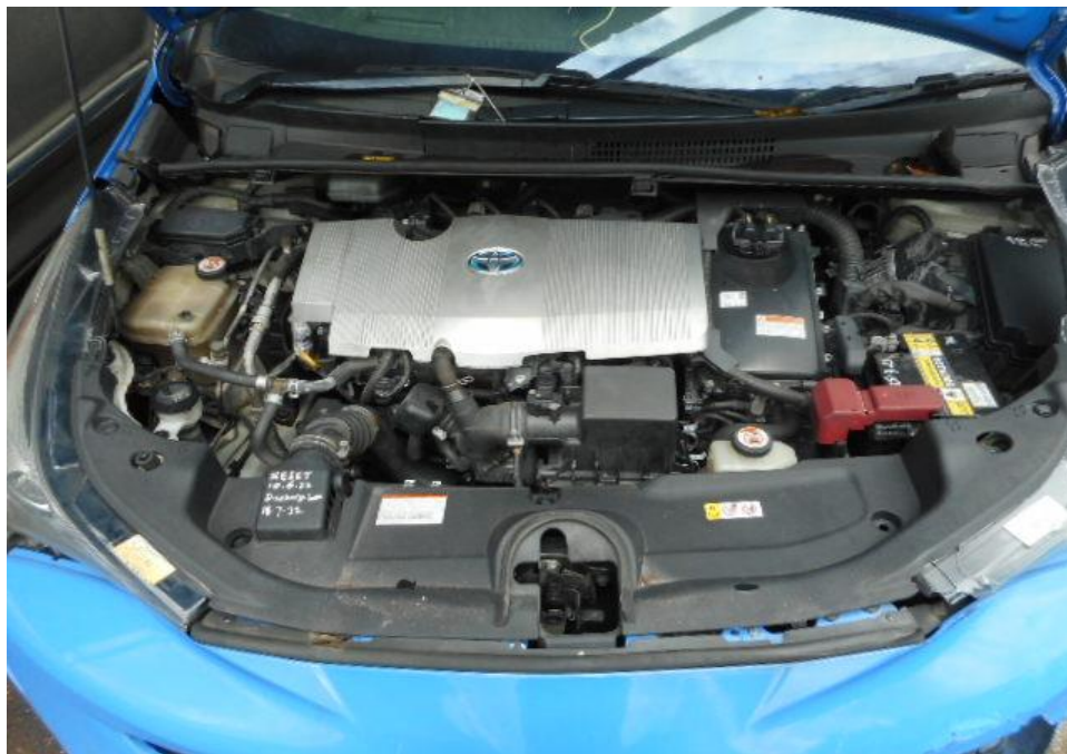
Photo 15 shows a general view of the Motor Taxi's engine compartment. The various parts and components inside the engine compartment were unaffected by the accident. There was also no sign(s) or indication(s) of fluid leakage and/or fluid stain within the engine compartment.
