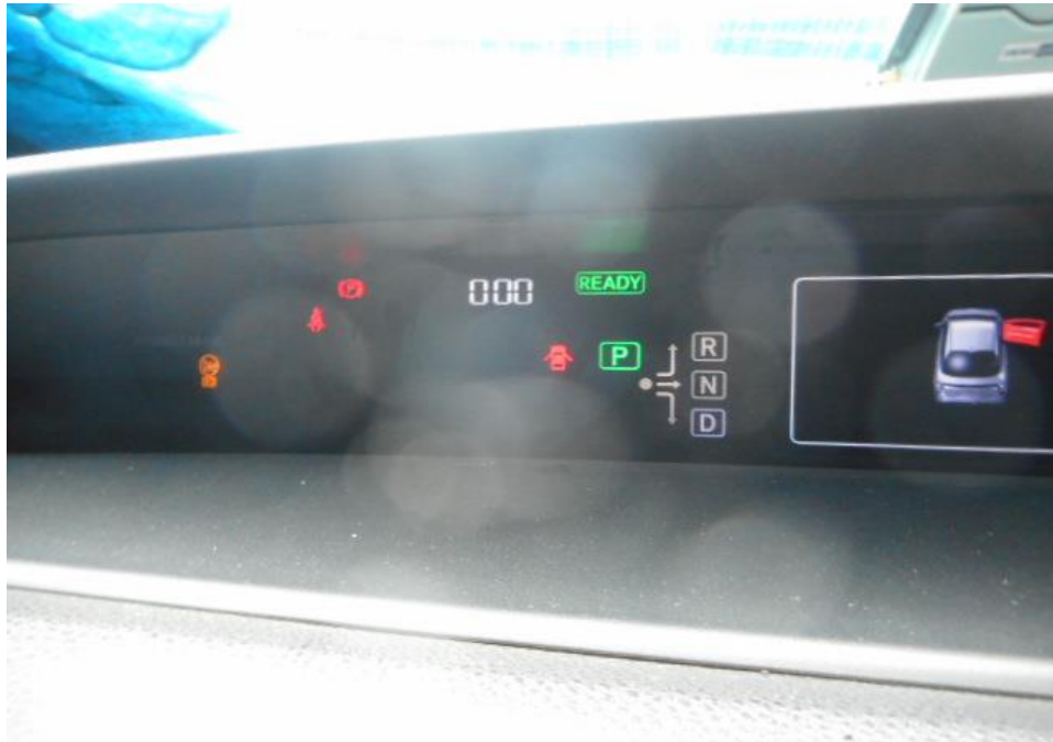
Photo 28 shows no warning lights illuminated on the instrument panel of the Motor Taxi after the engine was cranked. This would suggest that there was no abnormality to the electronic operating system of the Motor Taxi, like the ABS, EPS, TCS and SRS etc.
