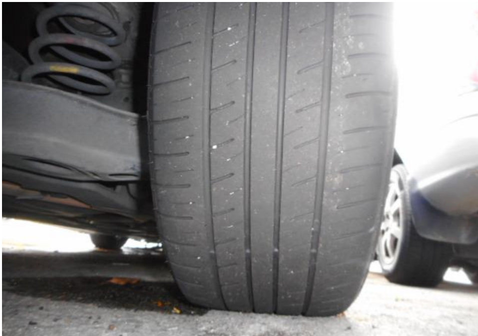
Photo 12 shows the condition of the rear right tyre of the Motor Taxi, which was observed to be in serviceable condition with remaining tread depth of approximately 2.9mm. The tyre was also observed to be sufficiently inflated for vehicular operation with no tear, cut or burst mark(s).
