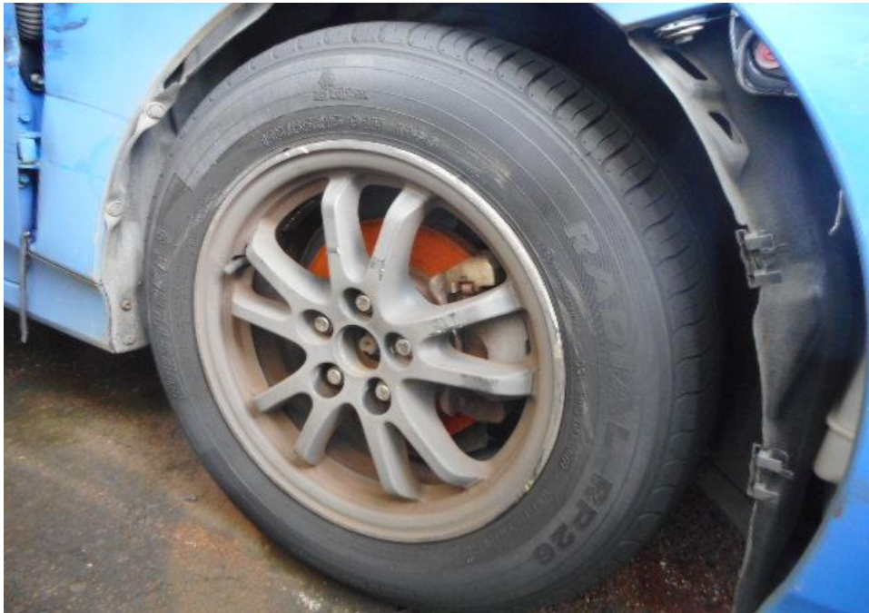
Photo 9 shows the condition of the front right tyre of the Motor Taxi, which was observed to be in serviceable condition with remaining tread depth of approximately 4.2mm. The tyre, which was wrapped around alloy wheel rim, was also observed to be sufficiently inflated for vehicular operation. The right wheel rim was observed to sustained minor damages as a result of the accident.
