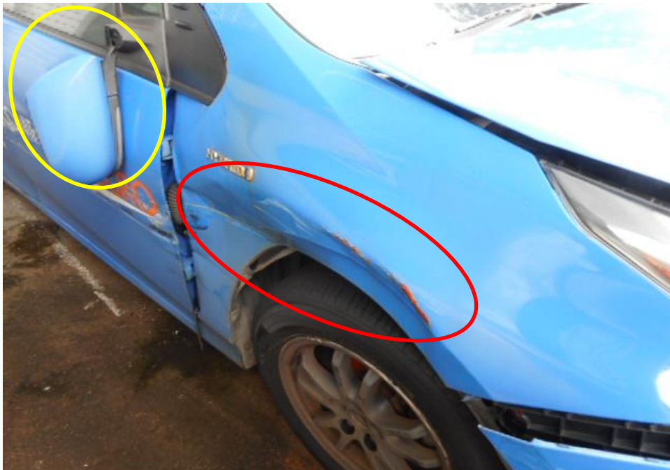
Photo 6 shows the close up view of the Motor Taxi's right body at the time of my inspection. The Motor Taxi was observed to have sustained damage at its right portion. Its right fender (red circle) and its right rear view mirror (yellow circle) was damaged as a result of the accident.
