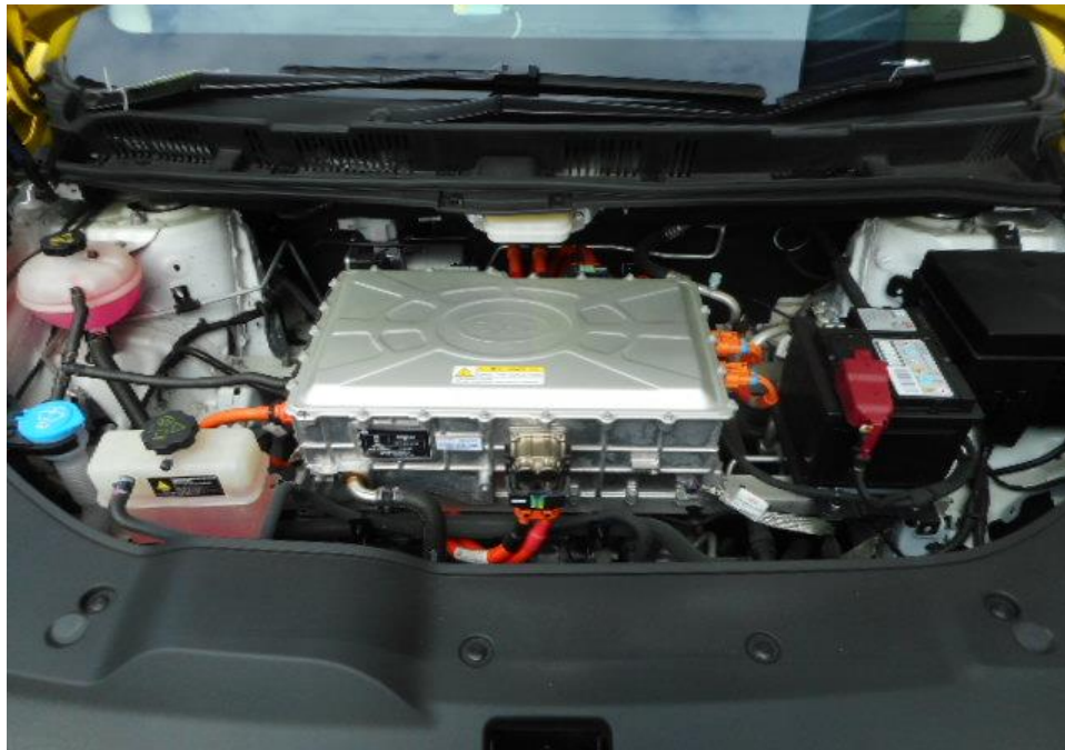
Photo 10 shows a general view of the Electric Taxi's engine compartment. The various parts and components inside the engine compartment were unaffected by the accident. There was also no sign(s) or indication(s) of fluid leakage and/or fluid stain within the engine compartment.
