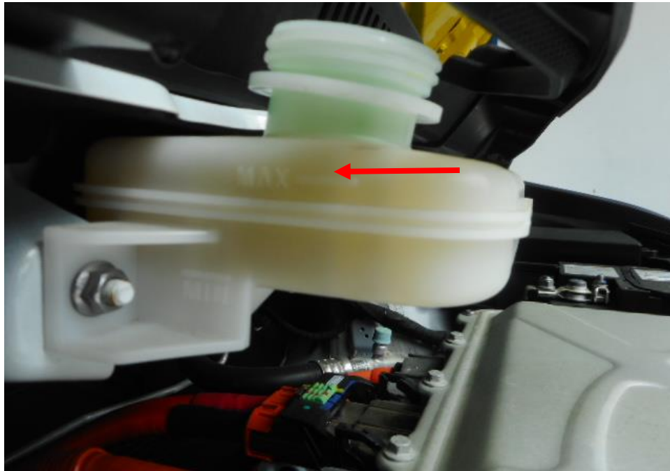
Photo 11 shows the brake fluid reservoir of the Electric Taxi at the time of my inspection. The brake fluid was observed to be of sufficient level (arrowed) and without any visible contamination.
