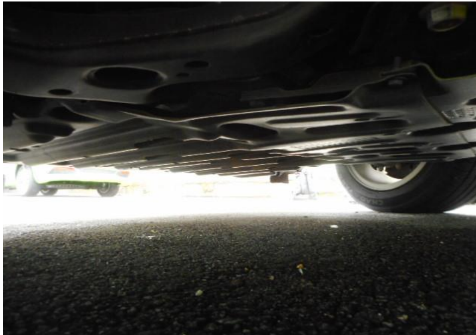
Photo 13 shows the undercarriage of the Electric Taxi, at the area where the electric motor housing are located. I did not find any sign(s) or indication(s) of fluid leak and/or fluid stain(s) on the underside of the Electric Taxi.
