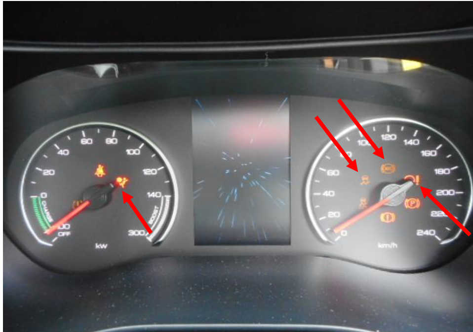
Photo 21 shows the warning light for Anti-Lock Brake System (ABS) and Power Steering System (EPS), Supplemental Restraint System (SRS) and Traction Control (TC) (arrowed) appearing on the instrument panel of the Electric Taxi during the self-test of its various electronic operating systems when its engine was cranked.
