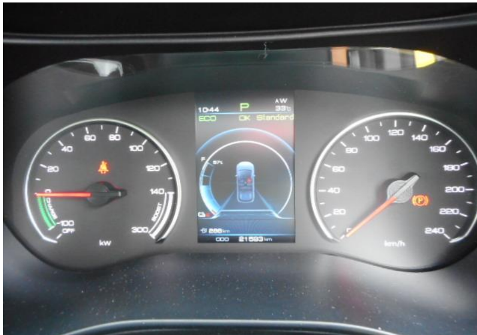
Photo 22 shows no warning lights illuminated on the instrument panel of the Electric Taxi after the engine was cranked. This would suggest that there was no abnormality to the electronic operating system of the Electric Taxi, like the ABS, EPS, SRS, and TC etc.
