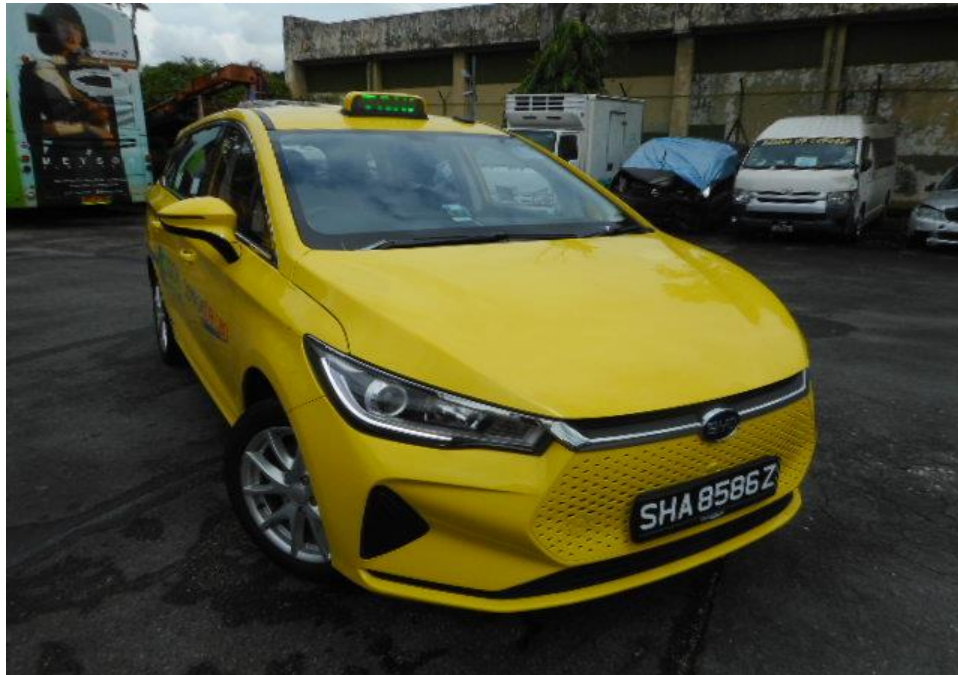
Photo 18 shows the front right wheel of the Electric Taxi turned to its full left. During my steering system test, I did not experience any abnormal free play and/or resistance when I had turned the steering wheel towards the left and right. This would suggest that the steering system of the Electric Taxi was likely to be in serviceable condition at the material time of accident.
