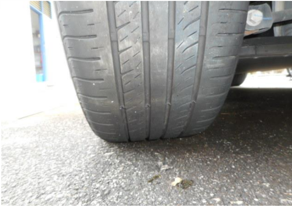
Photo 8 shows the condition of the rear left tyre of the Electric Taxi, which was observed to be in serviceable condition with remaining tread depth of approximately 3.8mm. The tyre, which was wrapped around steel wheel rim, was also observed to be sufficiently inflated for vehicular operation. The 4 tyres of the Electric Taxi were wrapped around standard steel wheel rims.
