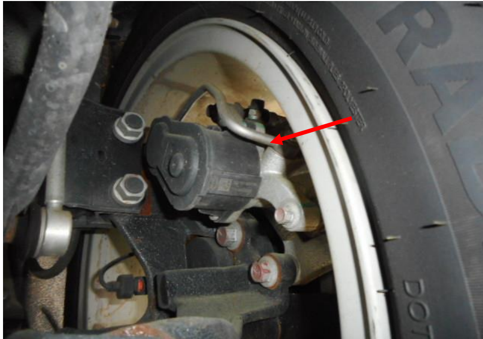
Photo 14 shows the brake hose/pipe (arrowed) at the rear right wheel of the Electric Taxi. No leakage of brake fluid was observed. Visual examination of the various components of the braking system like the drum brake, brake booster, brake pedal etc. had revealed all to be intact and without visible damage.
