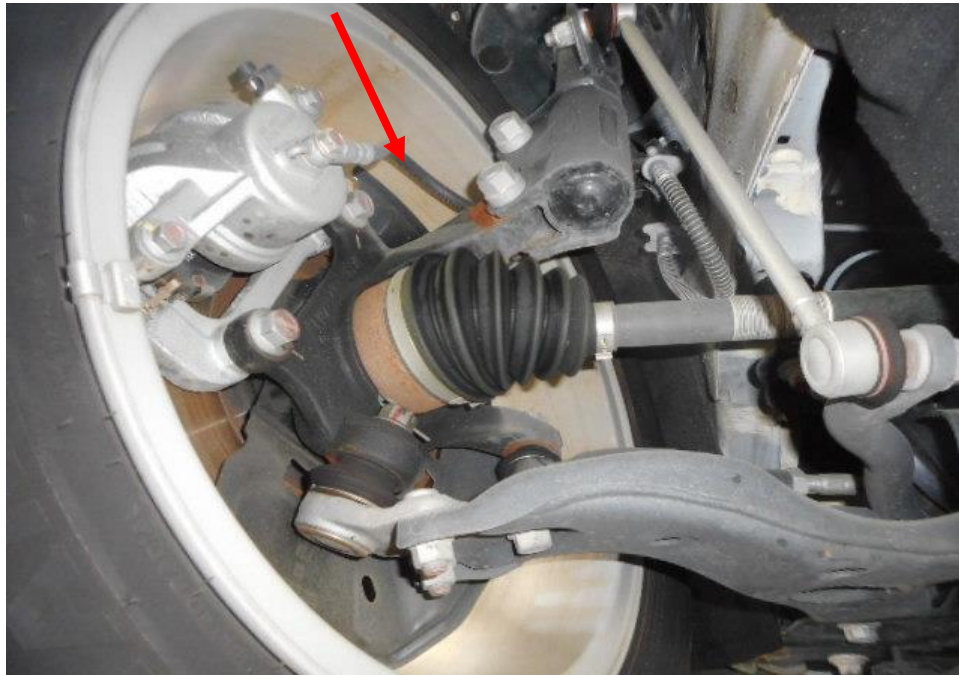
Photo 16 shows the brake hose/pipe (arrowed) at the front right wheel of the Electric Taxi. I did not observe any leakage of brake fluid at the time of my inspection of the Electric Taxi. Static tests of the Electric Taxi's braking system had indicated that there was no internal leakage of pressure/vacuum. The undercarriage components of the Electric Taxi were also all found to be intact and without any visible damage.
