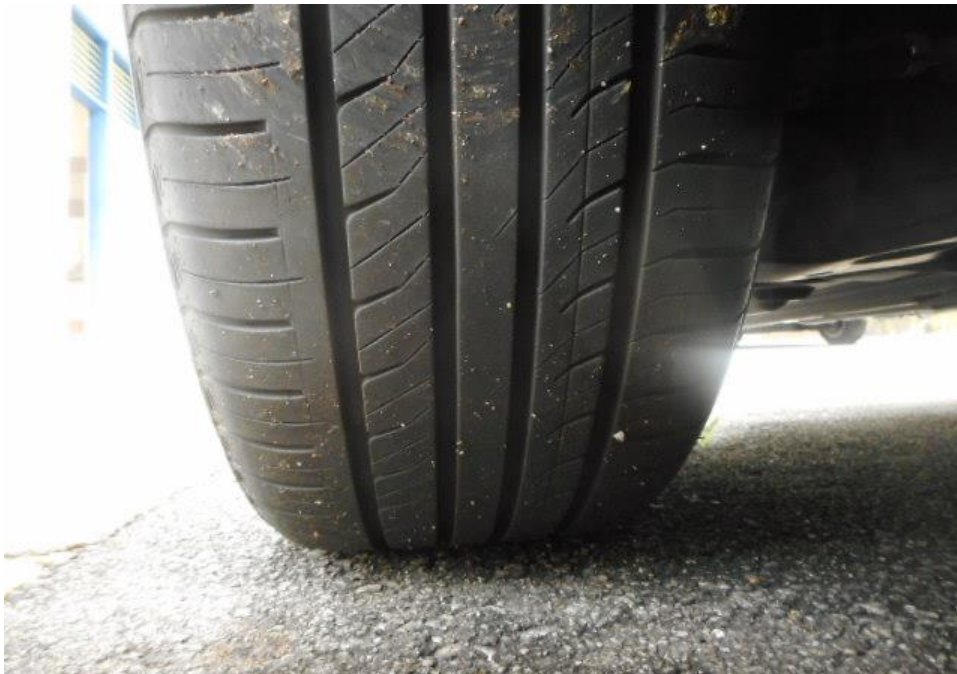
Photo 9 shows the condition of the front left tyre of the Electric Taxi, which was observed to be in serviceable condition with remaining tread depth of approximately 6.1mm. There was also no tear, cut or burst mark(s) on the outer and the inner sidewalls as well as across the tread of the Electric Taxi's 4 tyres.
