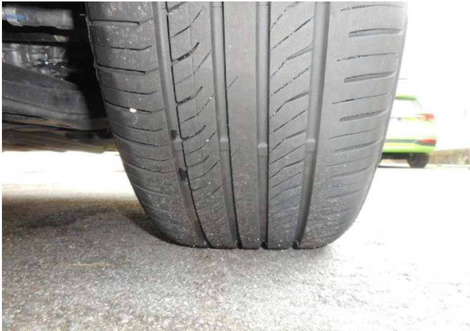
Photo 6 shows the condition of the front right tyre of the Electric Taxi, which was observed to be in serviceable condition with remaining tread depth of approximately 6.2mm. The tyre was sufficiently inflated for vehicular operation with no tear, cut or burst mark(s) on the outer and the inner sidewalls as well as across the tread. The 4 tyres of the Electric Taxi were wrapped around standard steel wheel rims without any damage.
