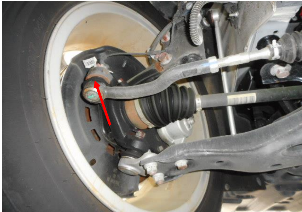
Photo 20 shows the various undercarriage components at the front left wheel of the Electric Taxi, which had included the steering tie rod (arrowed). The various undercarriage components of the Electric Taxi were all found to be intact without any visible damage.
