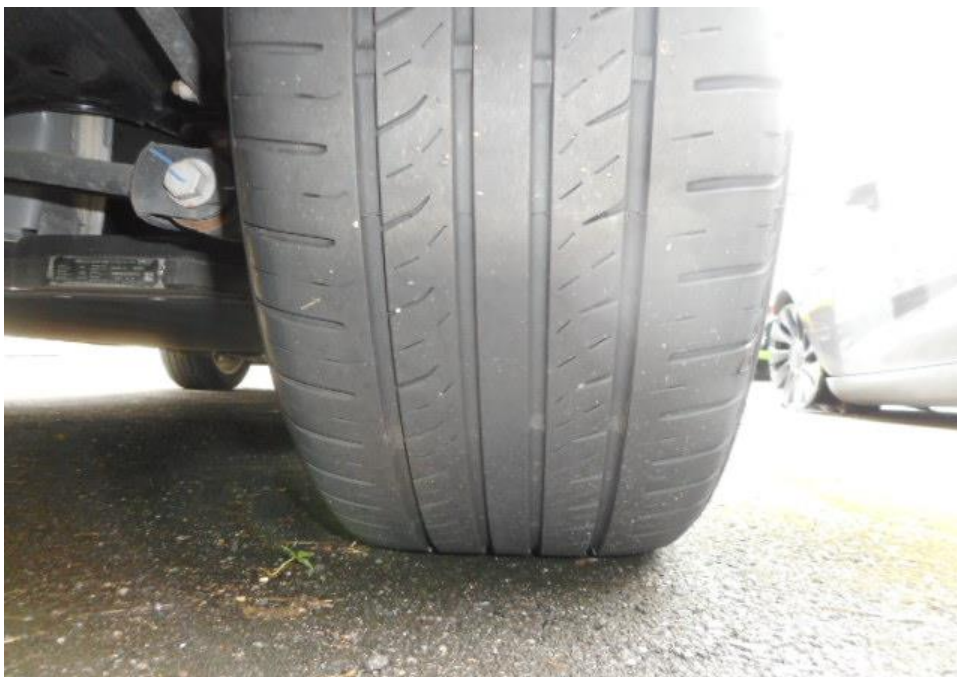
Photo 7 shows the condition of the rear right tyre of the Electric Taxi, which was observed to be in serviceable condition with remaining tread depth of approximately 4.3mm. The tyre was also observed to be sufficiently inflated for vehicular operation with no tear, cut or burst mark(s).
