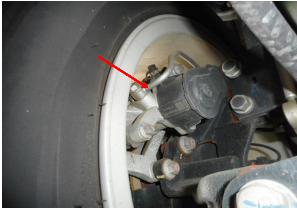
Photo 15 shows the brake hose/pipe (arrowed) at the rear left wheel of the Electric Taxi. I did not observe any leakage of brake fluid at the time of my inspection of the Electric Taxi. Static tests of the Electric Taxi's braking system had indicated that there was no internal leakage of pressure/vacuum. The undercarriage components of the Electric Taxi were also all found to be intact and without any visible damage.
