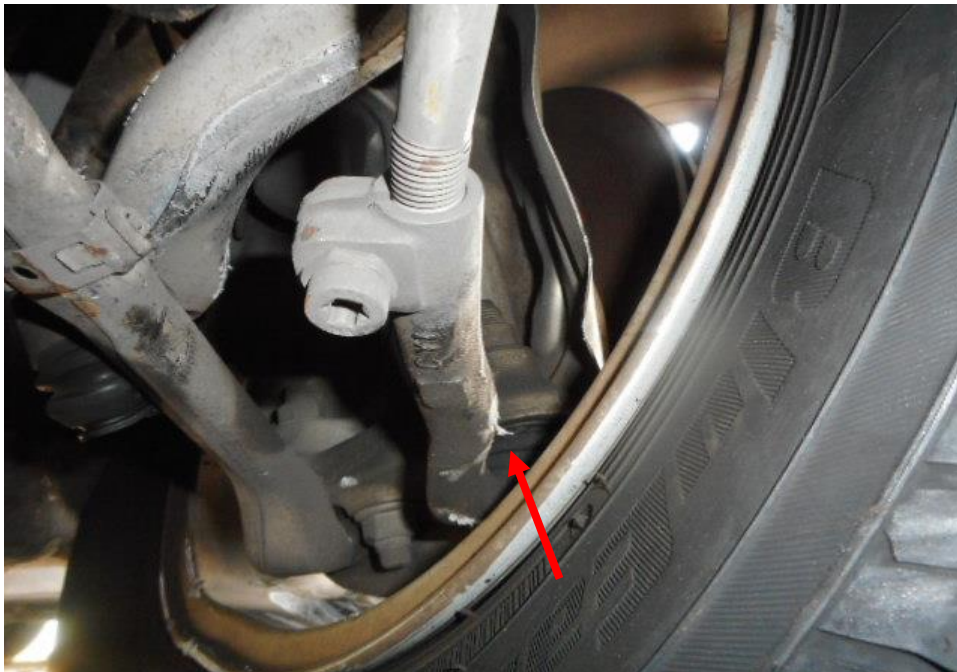
Photo 28 shows the various undercarriage components the front left wheel of the Motor Car, in particular the steering tie rod (arrowed) was found to be intact. However, the lower control arm was observed to be damaged as result of the accident. There was also no sign of fluid stain observed on the various undercarriage components at the front right wheel of the Motor Car.
