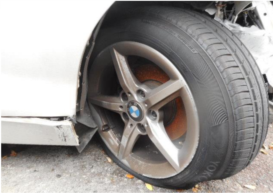
Photo 11 shows the general condition of the front right tyre of the Motor Car, which was observed to be deflated due to the damaged rim as a result of the accident. The tyre was also observed with cut mark(s) with remaining tread depth of approximately 5.6mm.
