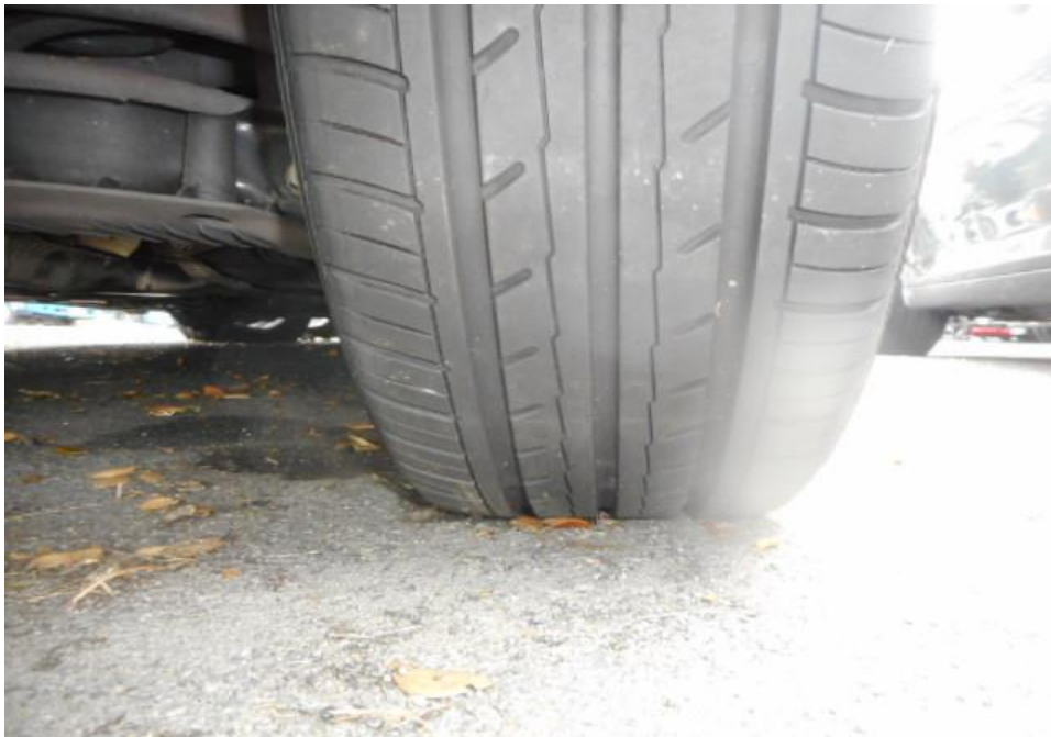
Photo 16 shows the condition of the rear right tyre of the Motor Car, which was observed to be in serviceable condition with remaining tread depth of approximately 5.2mm. The tyre was also observed to be sufficiently inflated for vehicular operation with no tear, cut or burst mark(s).
