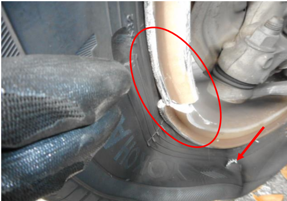
Photo 12 shows the close up condition of the front right tyre of the Motor Car, which was observed to be deflated due to the damaged rim (circled) as a result of the accident. The tyre was also observed with cut mark (arrowed) with remaining tread depth of approximately 5.6mm.
