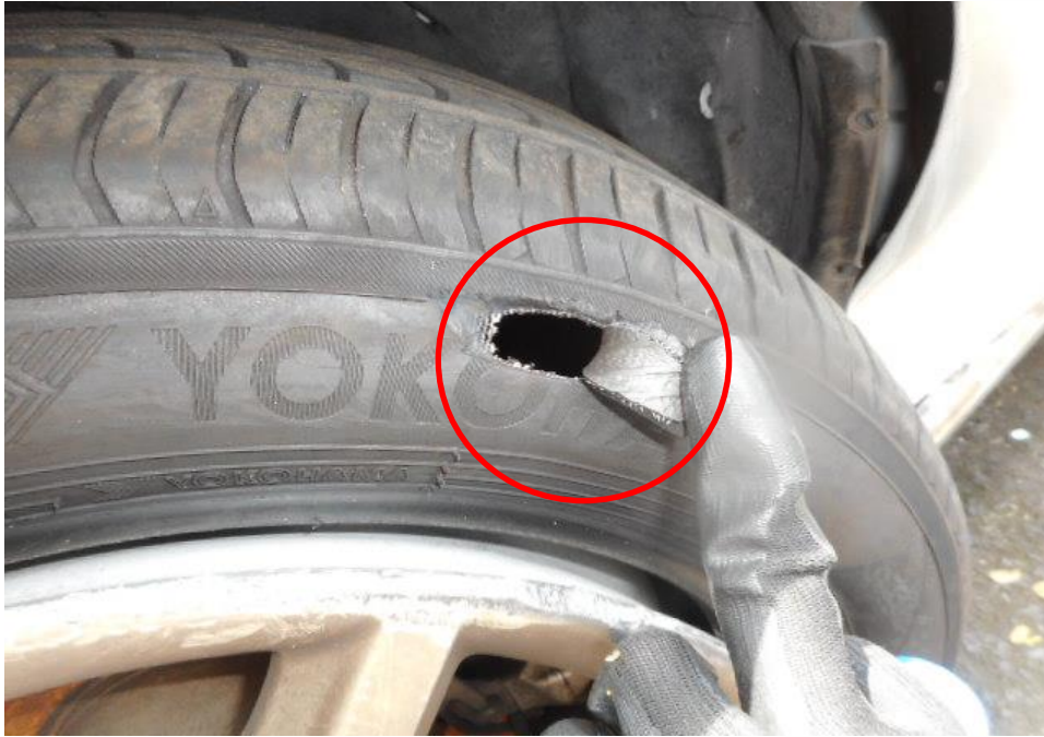
Photo 15 shows the close up condition of the front left tyre of the Motor Car, which was observed to be deflated due to the damaged rim as a result of the accident. The tyre was also observed with cut mark (circled) with remaining tread depth of approximately 5.7mm.
