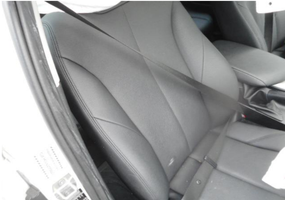
Photo 31 shows that the seat belt on the right seat were able to be fastened securely into the respective pre-tensioners that were fitted at the sides of each seat.
