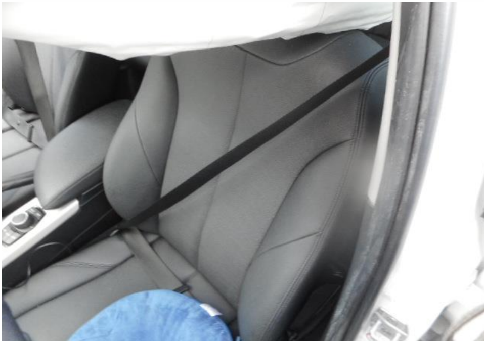
Photo 32 shows that the seat belt on the left seat were able to be fastened securely into the respective pre-tensioners that were fitted at the sides of each seat.
