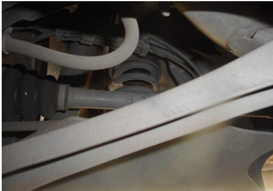
Photo 30 shows the various undercarriage components at the front right wheel of the Motor Car, the driveshaft (arrowed) was observed to be intact. There was also no sign of fluid stain observed on the various undercarriage components at the rear left wheel of the Motor Car.
