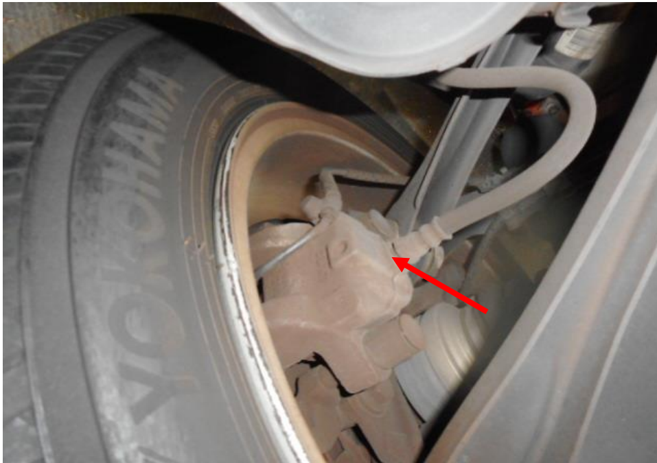
Photo 23 shows the brake hose/pipe (arrowed) at the rear left wheel of the Motor Car. No leakage of brake fluid was observed. Visual examination of the various components of the braking system like the brake caliper to be intact and without visible damage.
