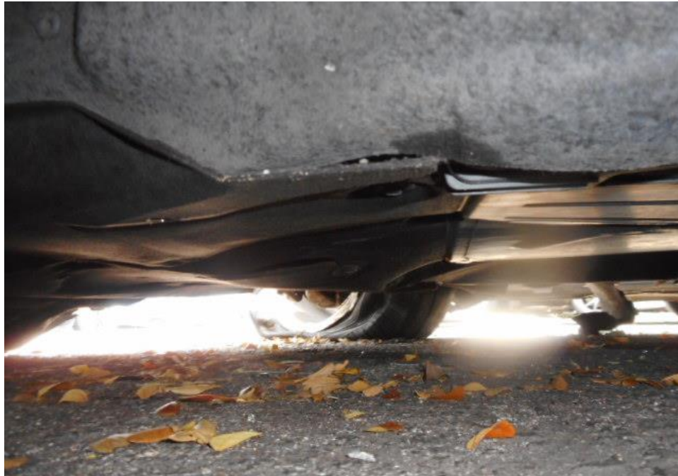
Photo 22 shows the undercarriage of the Motor Car, at the area where the engine housing and transmission housing are located. I did not find any sign(s) or indication(s) of fluid leak and/or fluid stain(s) on the underside of the Motor Car.
