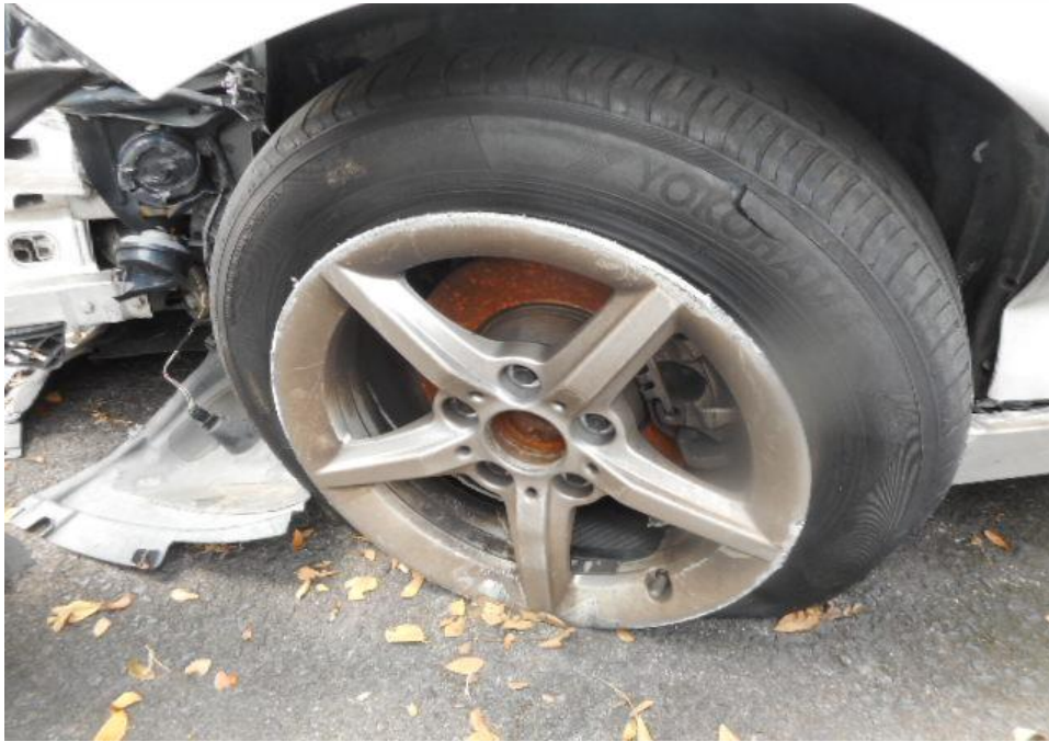
Photo 13 shows the general condition of the front left tyre of the Motor Car, which was observed to be deflated due to the damaged rim as a result of the accident. The tyre was also observed with cut mark(s) with remaining tread depth of approximately 5.7mm.
