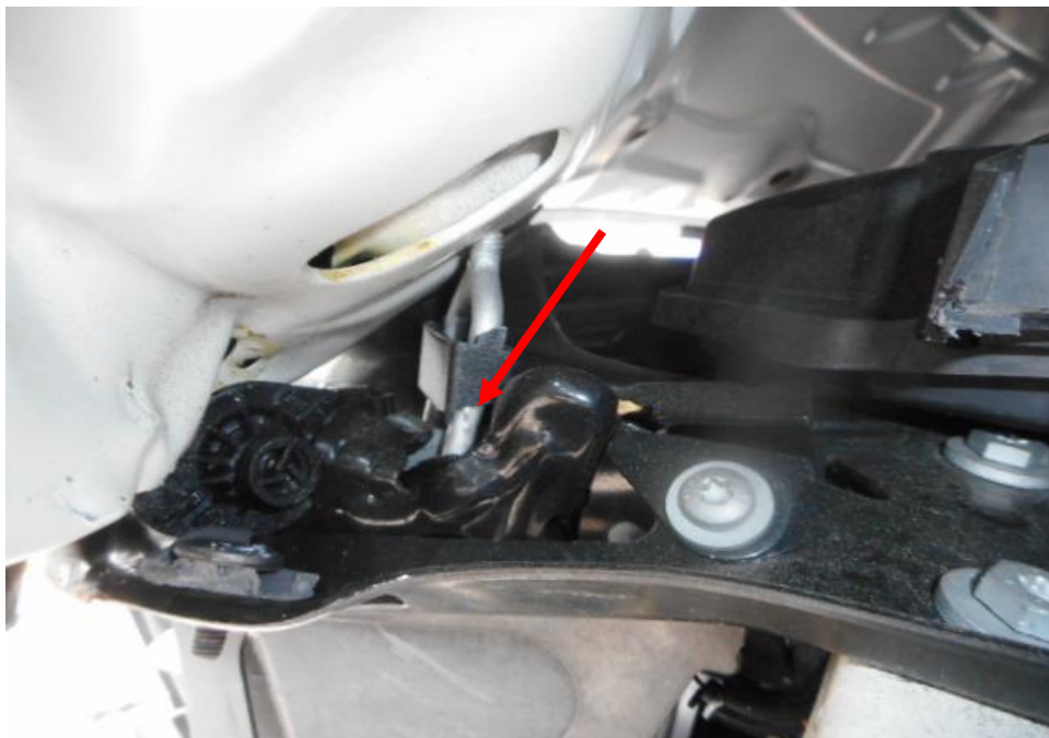
Photo 19 shows the close up view of the damaged front bonnet lock mechanism (arrowed) and the structure of the engine compartment of the Motor Car at the time of my inspection resulting it unable to open a result of the accident. (Unable to open)
