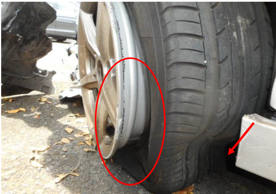
Photo 14 shows the close up condition of the front left tyre of the Motor Car, which was observed to be deflated due to the damaged rim (circled) as a result of the accident. The tyre was also observed with cut mark (arrowed) with remaining tread depth of approximately 5.7mm.
