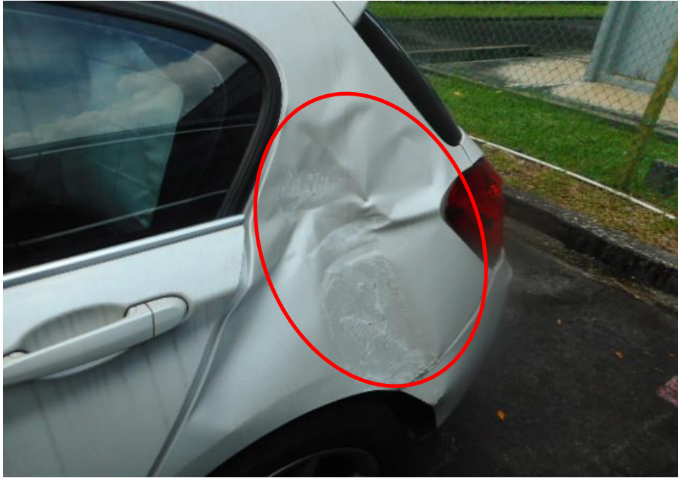
Photo 9 shows a general view of the Motor Car's left body at the time of my inspection. The Motor car was observed to have sustained damage at its left portion. Its left body panel (circled) was damaged as a result of the accident.
