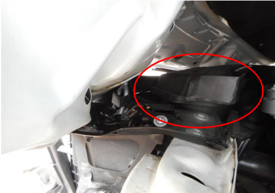
Photo 20 shows the close up view of the Motor Car's front body at the time of my inspection. The Motor car was observed to have sustained damage at its front portion. Its engine (circled) was amongst the various components in the engine compartments were also damaged as a result of the accident.
