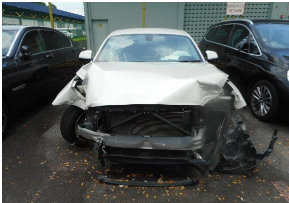
Photo 2 shows a general view of the Motor Car's front body at the time of my inspection. The Motor car was observed to have sustained damage at its front and left portion. Its front windscreen, front bonnet, front bumper, front left and right fender, front left and right headlamp was amongst the body parts and various engine components were also damaged as a result of the accident. The Supplemental Restraint System (SRS) was activated as a result of the accident.
