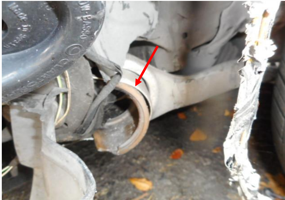
Photo 29 shows the various undercarriage components the front left wheel of the Motor Car, the lower control arm (arrowed) was observed to be damaged as result of the accident.
