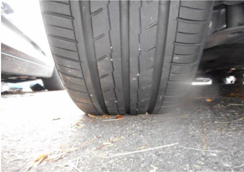
Photo 17 shows the condition of the rear left tyre of the Motor Car, which was observed to be in serviceable condition with remaining tread depth of approximately 4.1mm. The tyre was also observed to be sufficiently inflated for vehicular operation with no tear, cut or burst mark(s).
