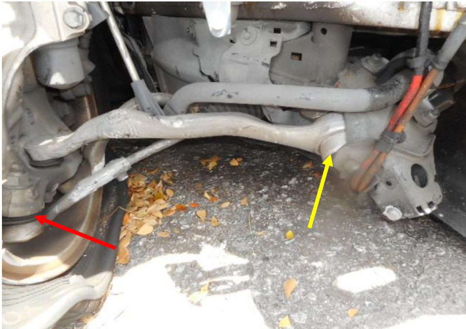
Photo 27 shows the various undercarriage components at the front right wheel of the Motor Car, in particular the steering tie rod (red arrow) was found to be intact. However, the lower control arm was observed to be damaged as result of the accident (yellow arrow). There was also no sign of fluid stain observed on the various undercarriage components at the front right wheel of the Motor Car.
