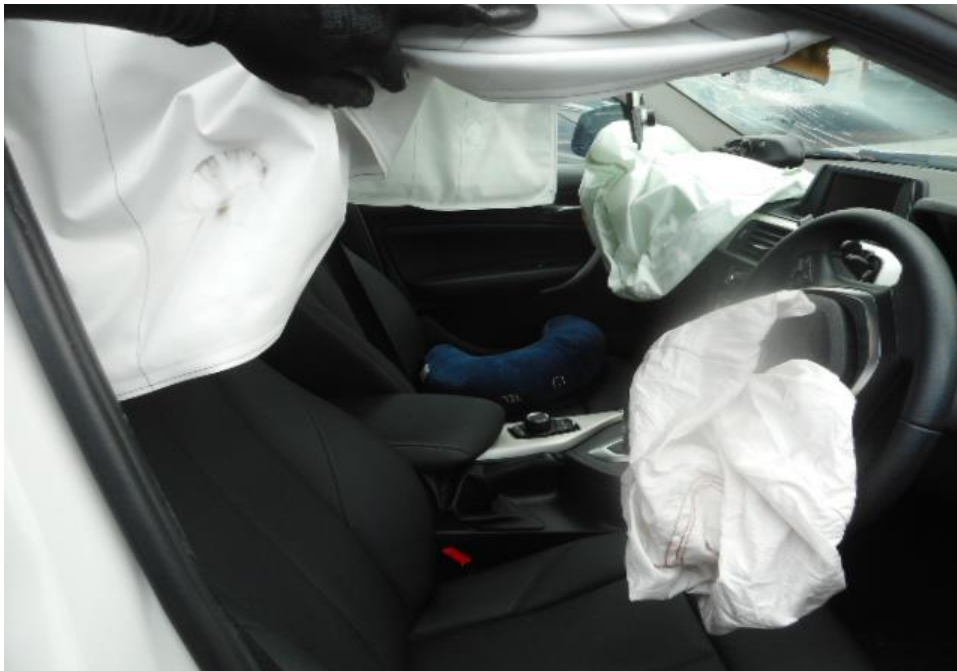
Photo 18 shows the deployment of the Supplemental Restraint System (SRS) airbag in the Motor Car as a result of the accident.
