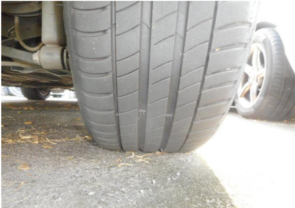
Photo 8 shows the condition of the rear right tyre of the Motor Car, which was observed to be in serviceable condition with remaining tread depth of approximately 6.3mm. The tyre was also observed to be sufficiently inflated for vehicular operation with no tear, cut or burst mark(s).
