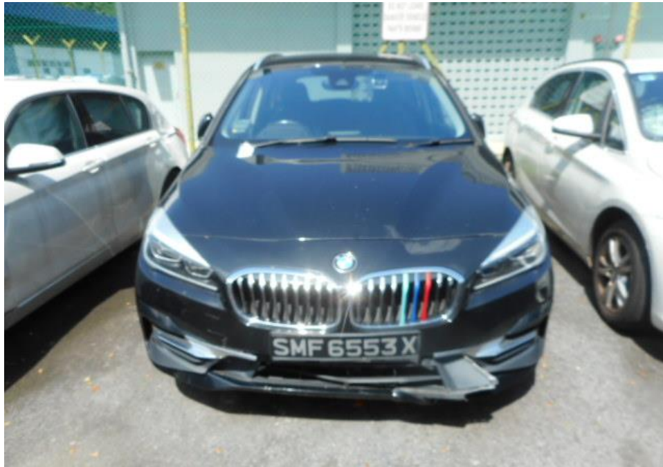
Photo 2 shows a general view of the Motor Car's front body at the time of my inspection. The front portion of the Motor Car was observed to have sustained damage. Its front bumper and was amongst the body part and engine coolant radiator component that were damaged as a result of the accident.
