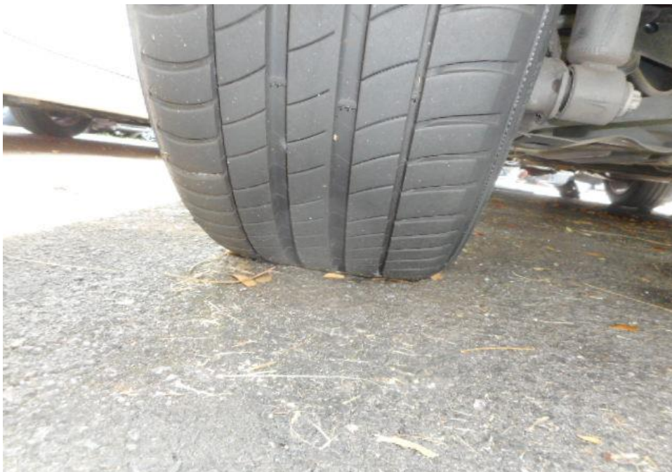
Photo 9 shows the condition of the rear left tyre of the Motor Car, which was observed to be in serviceable condition with remaining tread depth of approximately 6.2mm. The tyre, which was wrapped around steel wheel rim, was also observed to be sufficiently inflated for vehicular operation. The 4 tyres of the Motor Car were wrapped around standard steel wheel rims.
