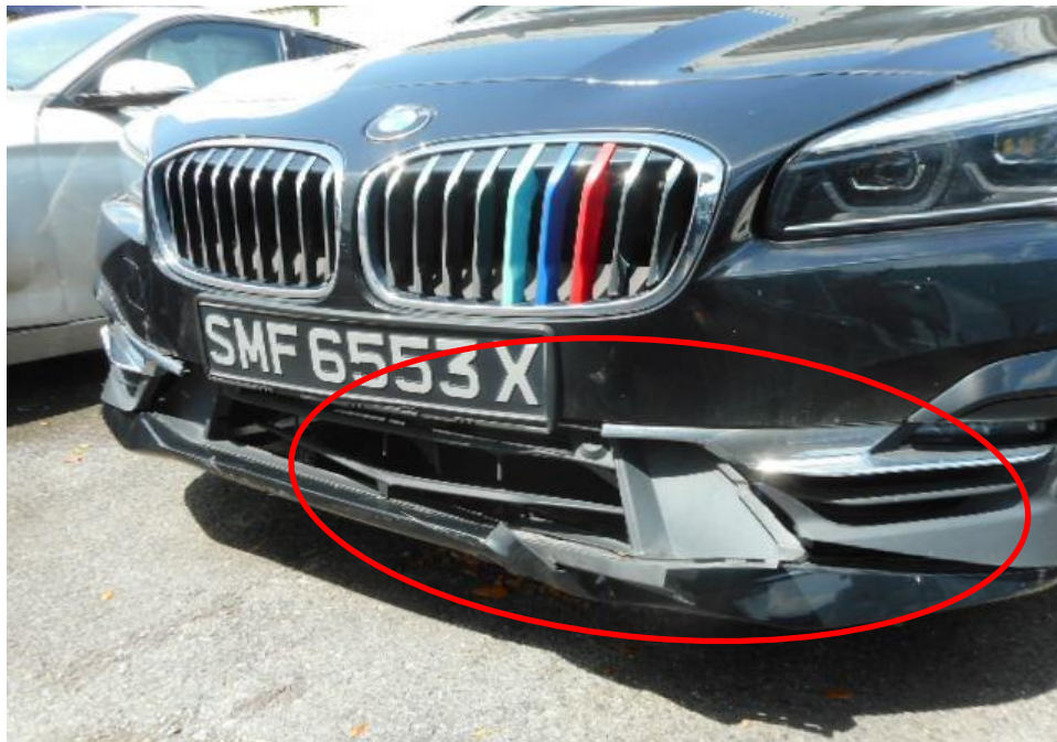
Photo 3 shows a close up view of the Motor Car's front body at the time of my inspection. The front portion of the Motor Car was observed to have sustained damage. Its front bumper (circled) was the body part that were damaged as a result of the accident.
