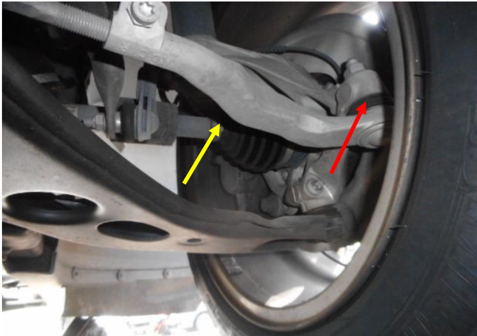
Photo 22 shows the various undercarriage components at the front right wheel of the Motor Car, in particular the steering tie rod (red arrow) and drive shaft (yellow arrow). The various steering components were all found to be intact, suggesting that the steering system of the Motor Car was likely to be in serviceable condition at the material time of accident. There was also no sign of fluid stain observed on the various undercarriage components at the front right wheel of the Motor Car.
