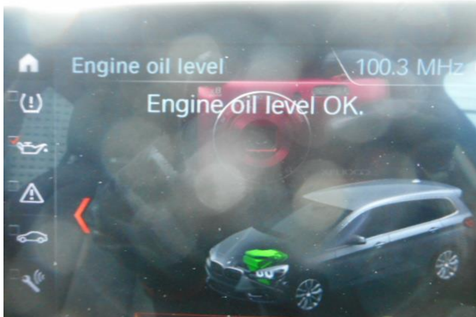
Photo 15 shows the engine oil display of the Motor Car at the time of my inspection. The engine oil was observed to be of sufficient level.
