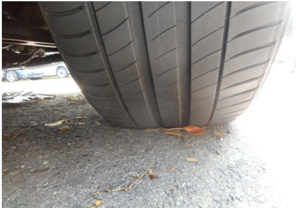
Photo 7 shows the condition of the front right tyre of the Motor Car, which was observed to be in serviceable condition with remaining tread depth of approximately 5.3mm. The tyre was sufficiently inflated for vehicular operation with no tear, cut or burst mark(s) on the outer and the inner sidewalls as well as across the tread. The 4 tyres of the Motor Car were wrapped around standard steel wheel rims without any damage.
