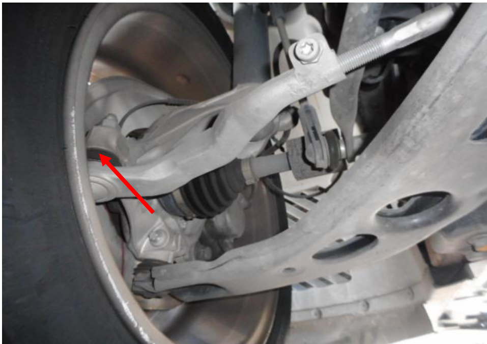
Photo 23 shows the various undercarriage components at the front left wheel of the Motor Car, which had included the steering tie rod (red arrow). The various undercarriage components of the Motor Car were all found to be intact without any visible damage.
