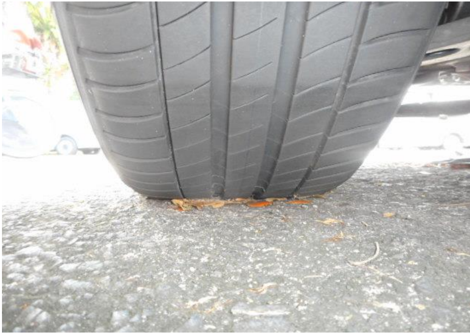
Photo 10 shows the condition of the front left tyre of the Motor Car, which was observed to be in serviceable condition with remaining tread depth of approximately 5.2mm. There was also no tear, cut or burst mark(s) on the outer and the inner sidewalls as well as across the tread of the Motor Car's 4 tyres.
