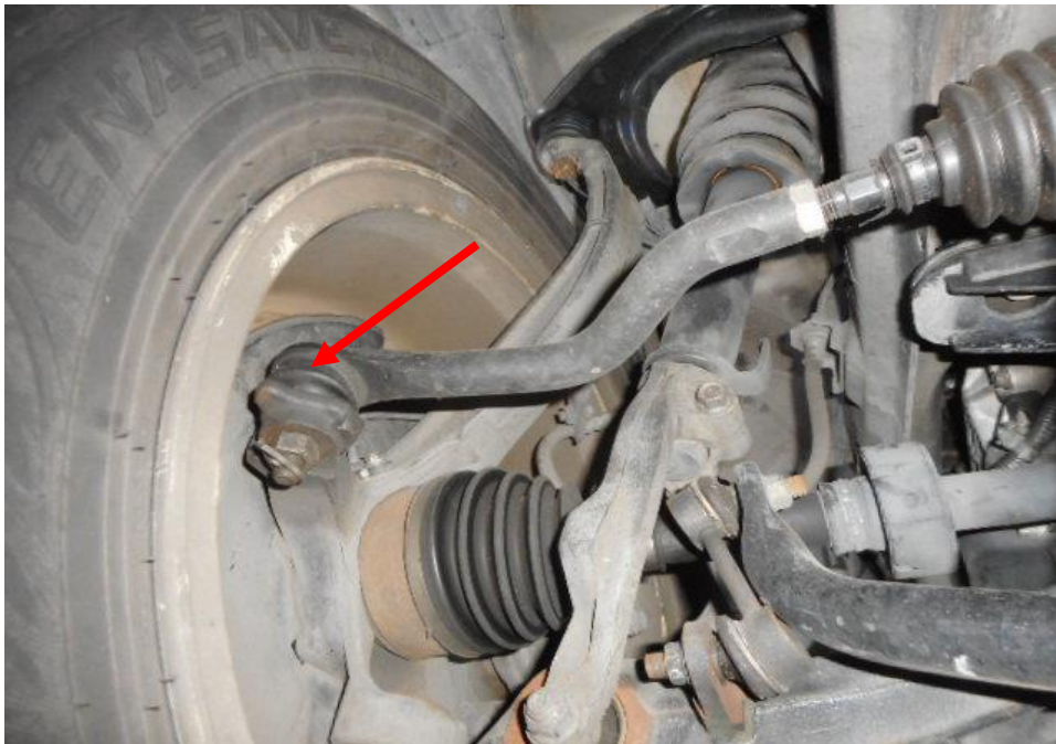
Photo 26 shows the various undercarriage components at the front left wheel of the Motor Car, which had included the steering tie rod (arrowed). The various undercarriage components of the Motor Car were all found to be intact without any visible damage.
