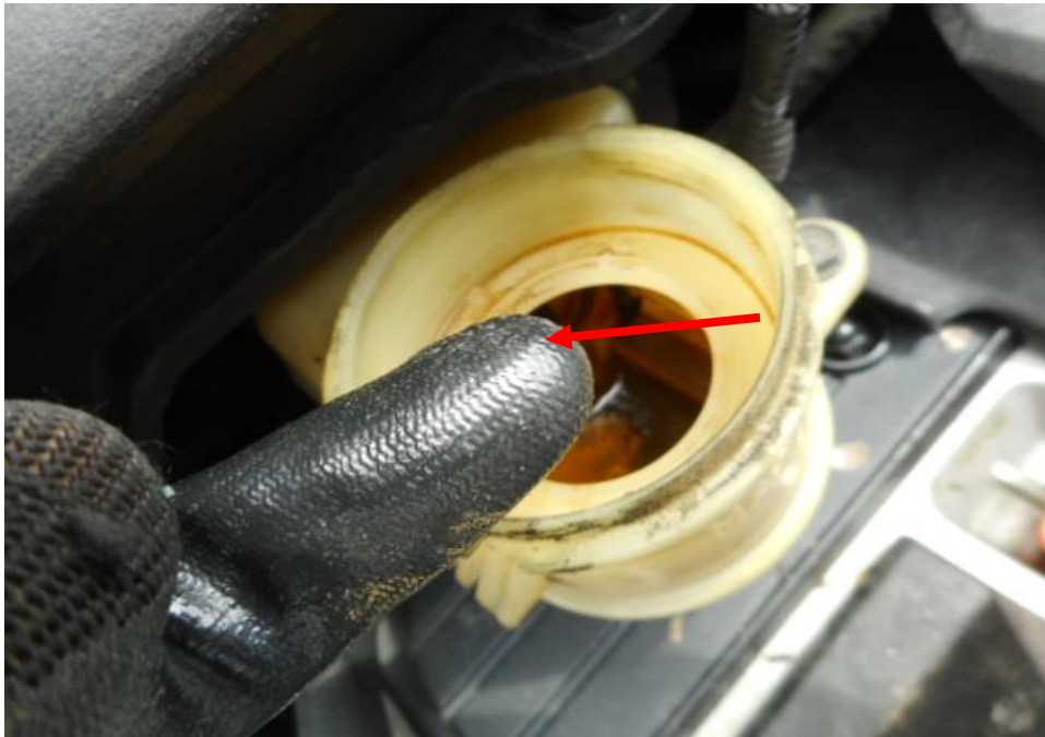
Photo 14 shows the brake fluid reservoir of the Motor Car at the time of my inspection. The brake fluid was observed to be of insufficient level (arrowed) however, we did not observed any leakage to the braking components
