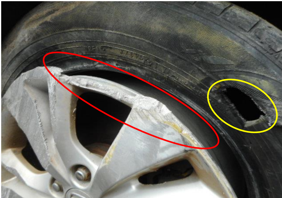
Photo 9 shows the close up condition of the front right tyre of the Motor Car, which was observed to be in unserviceable condition with remaining tread depth of approximately 3.8mm. The tyre was also observed to be deflated with cut marks (yellow circle) and the wheel rim (red circle) was also damaged as a result of the accident.
