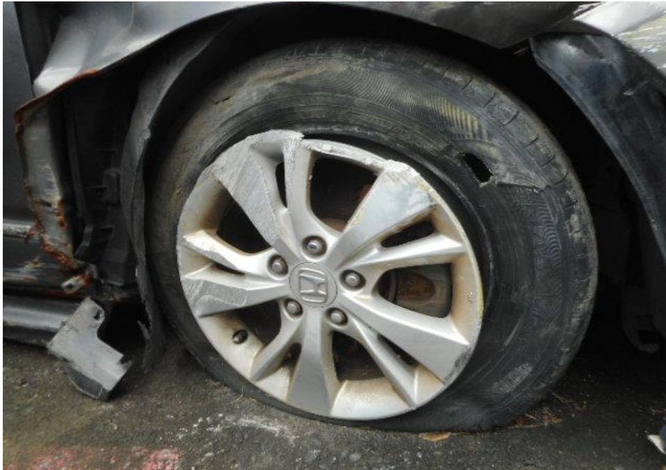
Photo 8 shows the condition of the front right tyre of the Motor Car, which was observed to be in unserviceable condition with remaining tread depth of approximately 3.8mm. The tyre was also observed to be deflated with cut marks and the wheel rim was also damaged as a result of the accident.
