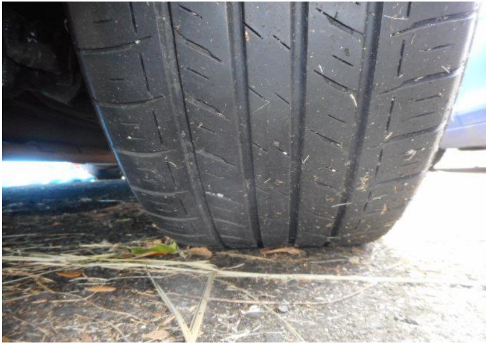
Photo 10 shows the condition of the rear right tyre of the Motor Car, which was observed to be in serviceable condition with remaining tread depth of approximately 4.6mm. The tyre was also observed to be sufficiently inflated for vehicular operation with no tear, cut or burst mark(s).
