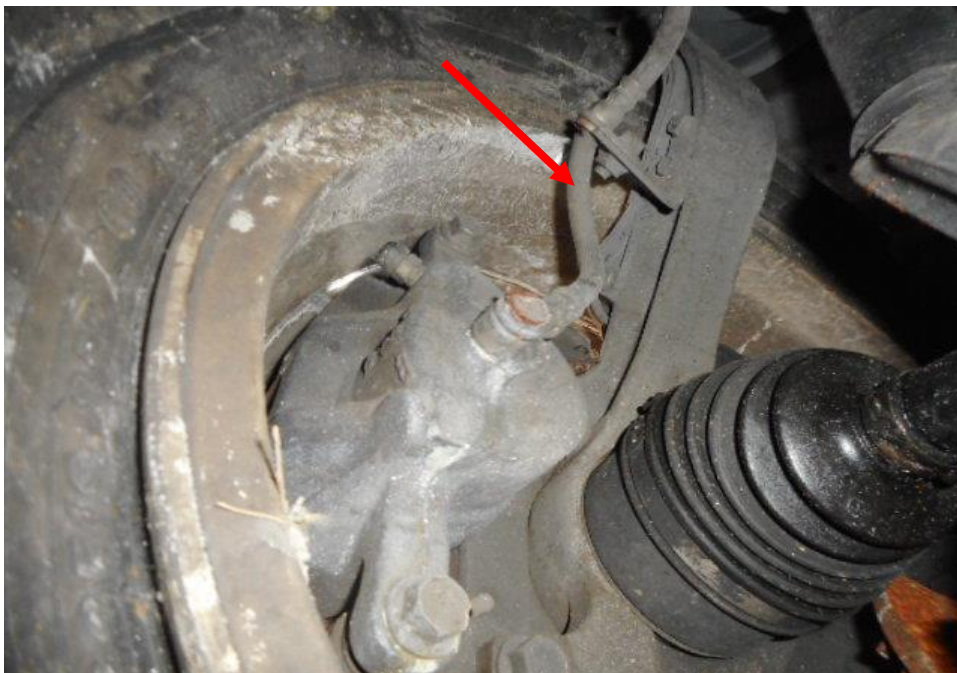
Photo 22 shows the brake hose/pipe (arrowed) at the front right wheel of the Motor Car. I did not observe any leakage of brake fluid at the time of my inspection of the Motor Car. The undercarriage components of the Motor Car were also all found to be intact and without any visible damage.
