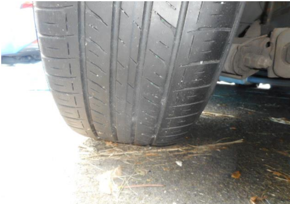
Photo 11 shows the condition of the rear left tyre of the Motor Car, which was observed to be in serviceable condition with remaining tread depth of approximately 4.9mm. The tyre, which was wrapped around alloy wheel rim, was also observed to be sufficiently inflated for vehicular operation. The 4 tyres of the Motor Car were wrapped around standard alloy wheel rims.
