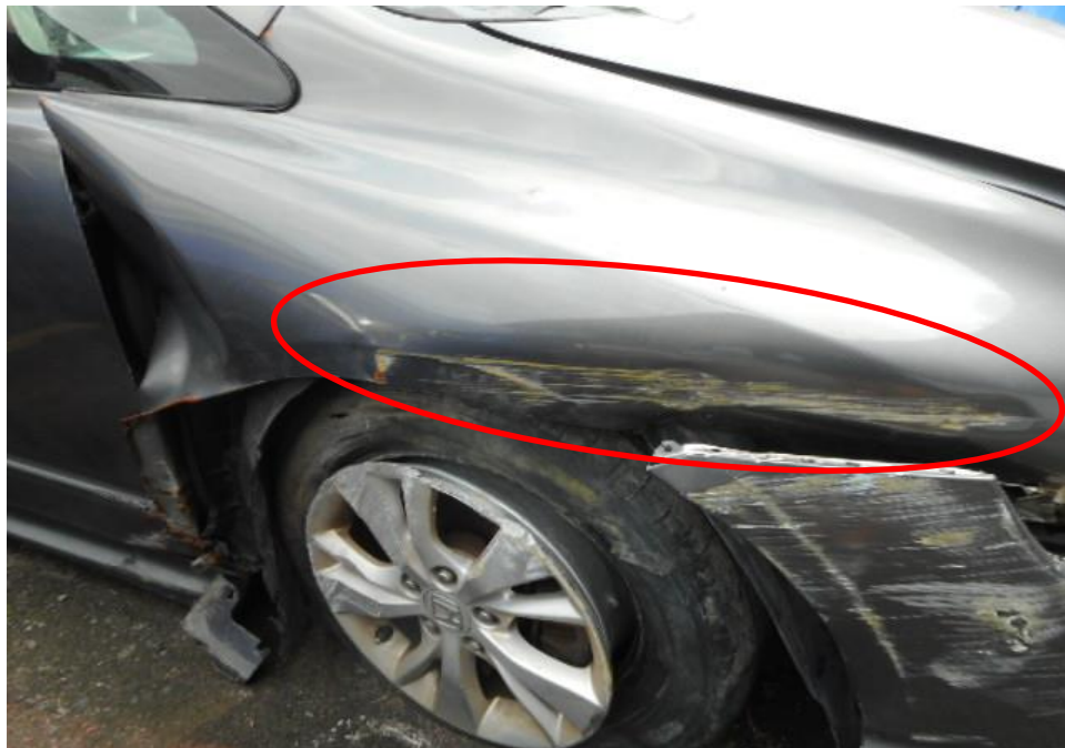
Photo 3 shows a close up view of the Motor Car's front body at the time of my inspection. The front portion of the Motor Car was observed to have sustained damage. Its front right fender (circled) was amongst the body parts that were damaged as a result of the accident.
