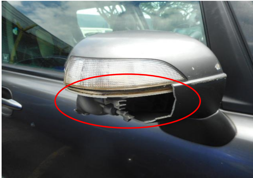
Photo 4 shows a close up view of the Motor Car's front body at the time of my inspection. The front portion of the Motor Car was observed to have sustained damage. Its front right rear view mirror (circled) was amongst the body parts that were damaged as a result of the accident.
