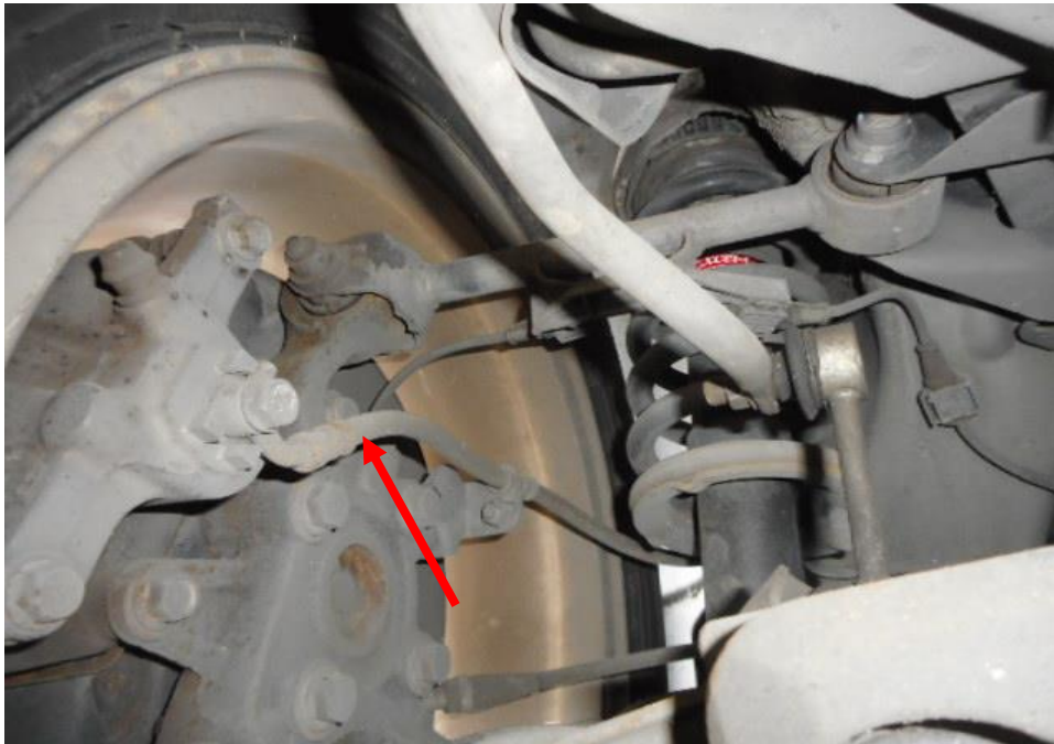
Photo 21 shows the brake hose/pipe (arrowed) at the rear left wheel of the Motor Car. I did not observe any leakage of brake fluid at the time of my inspection of the Motor Car. The undercarriage components of the Motor Car were also all found to be intact and without any visible damage.
