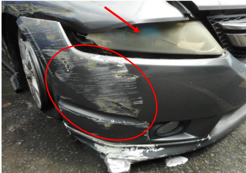
Photo 2 shows a close up view of the Motor Car's front body at the time of my inspection. The front portion of the Motor Car was observed to have sustained damage. Its front bumper (circled) and front right headlamp (arrowed) was amongst the body parts that were damaged as a result of the accident.
