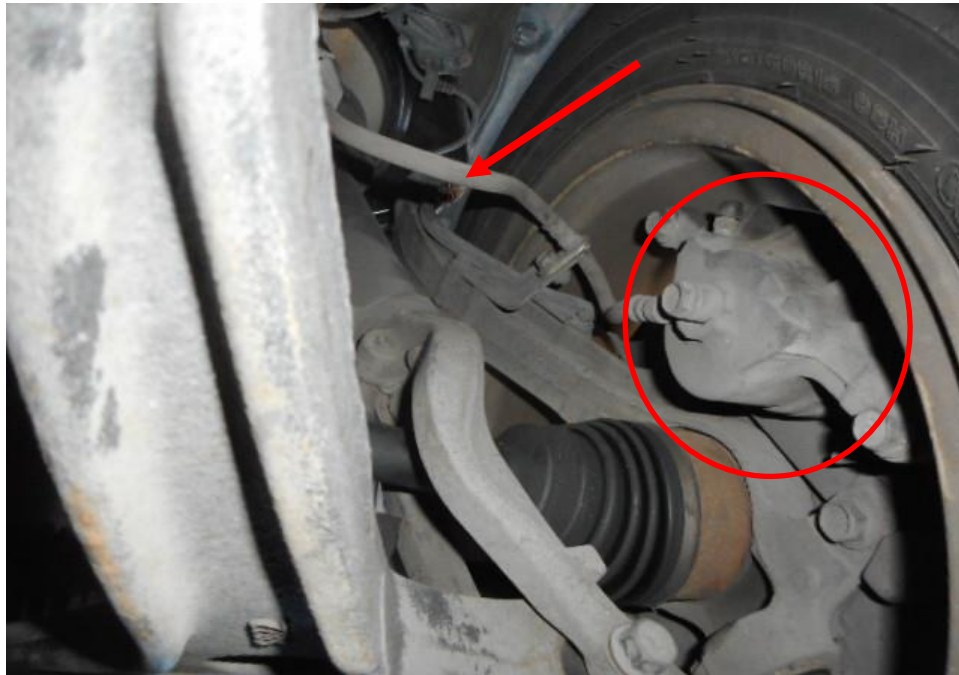
Photo 23 shows the brake hose/pipe (arrowed) at the front left wheel of the Motor Car. No leakage of brake fluid was observed. Visual examination of the various components of the braking system like the brake caliper (circled), brake booster, brake pedal etc had revealed all to be intact and without visible damage.
