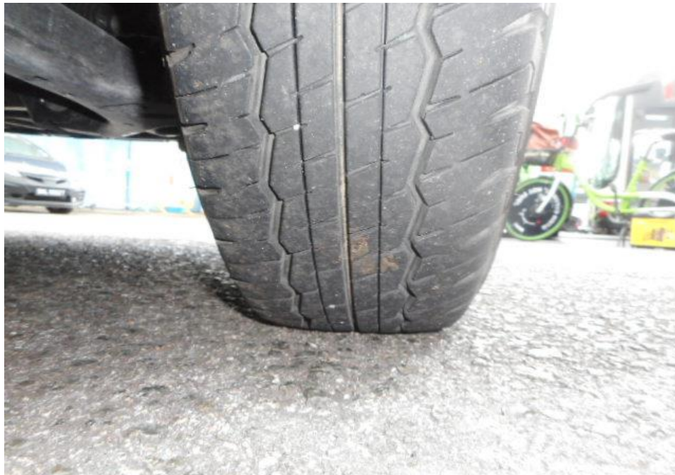
Photo 7 shows the condition of the front right tyre of the Motor Van, which was observed to be in serviceable condition with remaining tread depth of approximately 5.4mm. The tyre, which was wrapped around standard steel wheel rim, was also observed to be sufficiently inflated for vehicular operation. There was no tear, cut or burst mark(s) on the outer and the inner sidewalls as well as across the tread of the 4 tyres that were fitted on the Motor Van.
