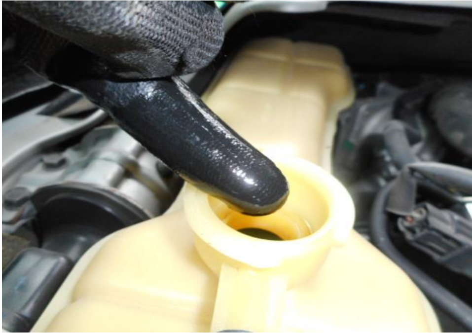
Photo 13 shows the engine coolant of the Motor Van at the time of my inspection. The engine coolant was observed to be of sufficient level and without any visible contamination.
