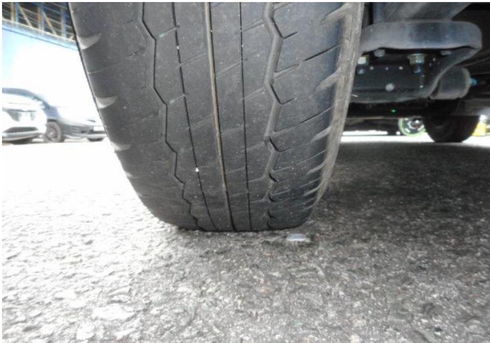
Photo 9 shows the condition of the rear left tyres of the Motor Van, which was observed to be in serviceable condition with remaining tread depth of approximately 4.7mm. The tyres, which were wrapped around standard steel wheel rim, were also observed to be sufficiently inflated for vehicular operation. There was also no damage found on all 4 steel wheel rims of the Motor Van.
