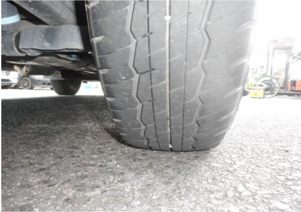
Photo 8 shows the condition of the rear right tyre of the Motor Van, which was observed to be in serviceable condition with remaining tread depth of approximately 5mm. The tyre, which was wrapped around standard steel wheel rim, it was observed to be sufficiently inflated for vehicular operation.
