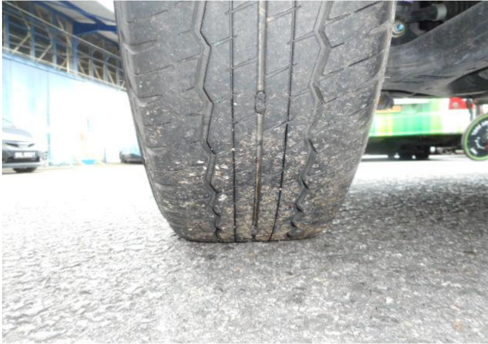
Photo 10 shows the condition of the rear right tyres of the Motor Van, which were observed to be in serviceable condition with remaining, tread depth of approximately 4.8mm. There was also no tear, cut or burst mark(s) on the outer and the inner sidewalls as well as across the tread of the 4 tyres that were fitted on the Motor Van.
