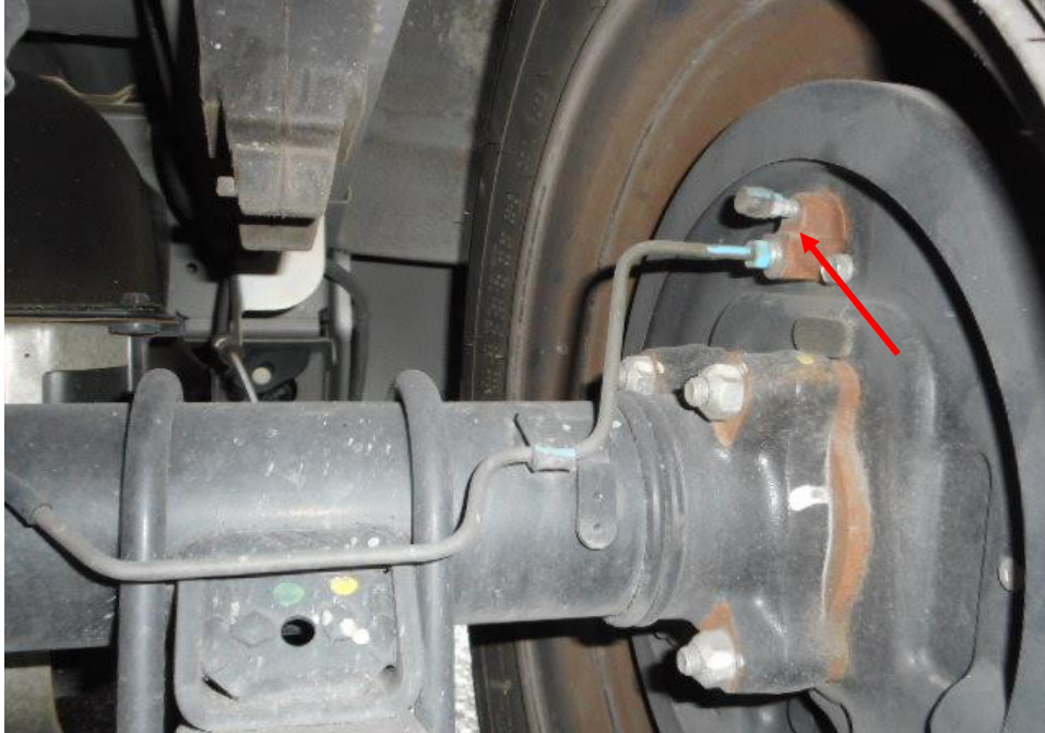
Photo 18 shows the brake pipe (arrowed) at the rear right wheel of the Motor Van. I did not observe any leakage of brake fluid at the time of my inspection of the Motor Van. My static tests of the Motor Van's braking system, along with my visual examination of the various mechanical components in the braking system, had indicated that there was no internal leakage of pressure/vacuum. Hence the braking system of the Motor Van was likely to be in serviceable condition at the material time of accident.
