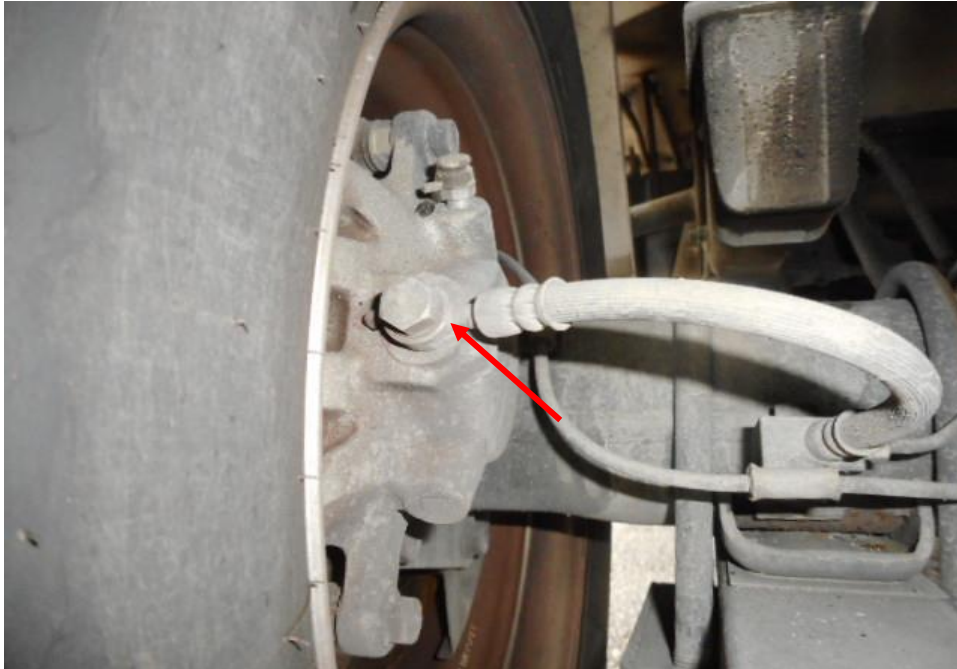
Photo 19 shows the brake pipe (arrowed) at the rear left wheel of the Motor Lorry. I did not observe any leakage of brake fluid at the time of my inspection of the Motor Lorry. My static tests of the Motor Lorry's braking system, along with my visual examination of the various mechanical components in the braking system had indicated that there was no internal leakage of pressure/vacuum. Hence the braking system of the Motor Lorry was likely to be in serviceable condition at the material time of accident.
