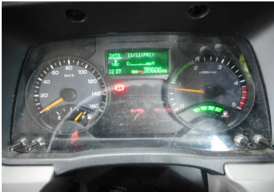
Photo 24 shows no warning lights illuminated on the instrument panel of the Motor Lorry after the engine was cranked. This would suggest that there was no abnormality to the electronic operating system of the Motor Van, like the ABS, SRS and etc.
