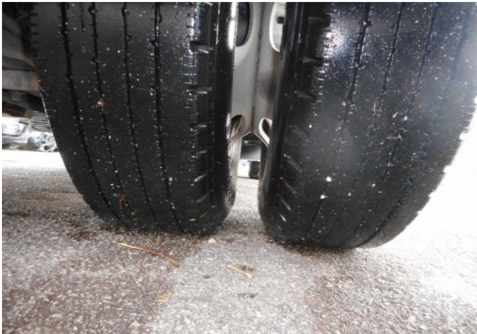
Photo 7 shows the condition of the rear right tyre of the Motor Lorry, which was observed to be in serviceable condition with remaining tread depth of approximately 3.7mm. The tyre, which was wrapped around standard steel wheel rim, it was observed to be sufficiently inflated for vehicular operation.
