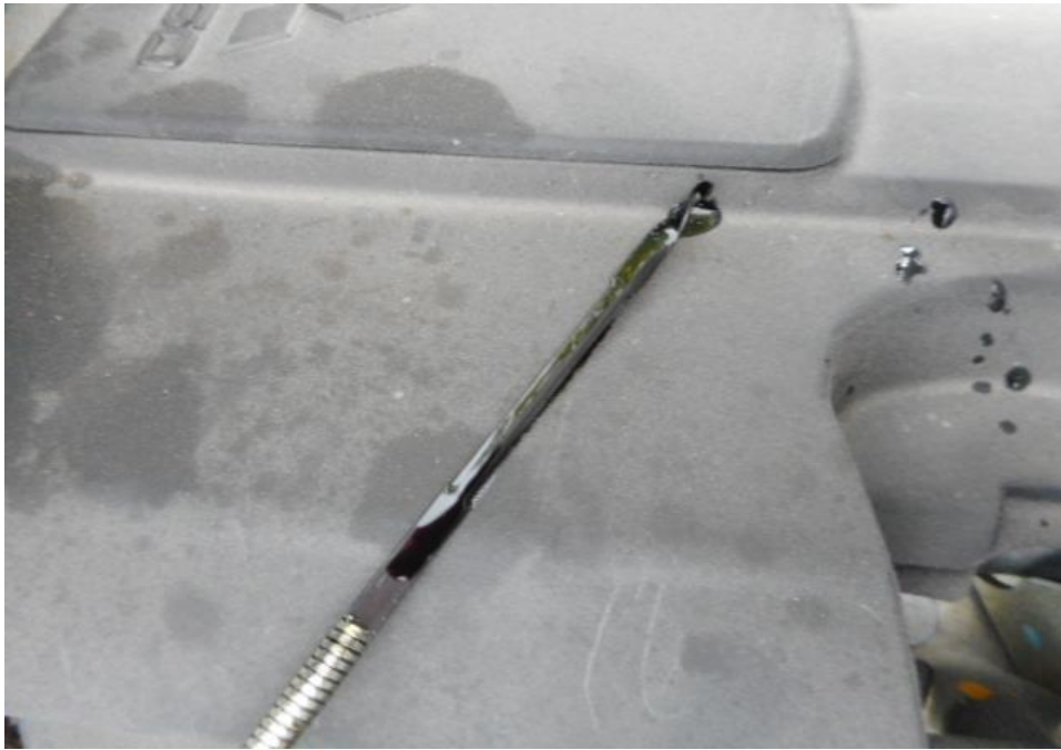
Photo 13 shows the engine oil dip stick of the Motor Lorry at the time of my inspection. The engine oil was observed to be of sufficient level and without any visible contamination.
