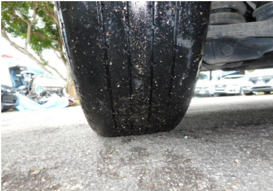
Photo 9 shows the condition of the front right tyre of the Motor Lorry, which was observed to be in serviceable condition with remaining tread depth of approximately 4.2mm. The tyres, which were wrapped around standard steel wheel rim, were also observed to be sufficiently inflated for vehicular operation.
