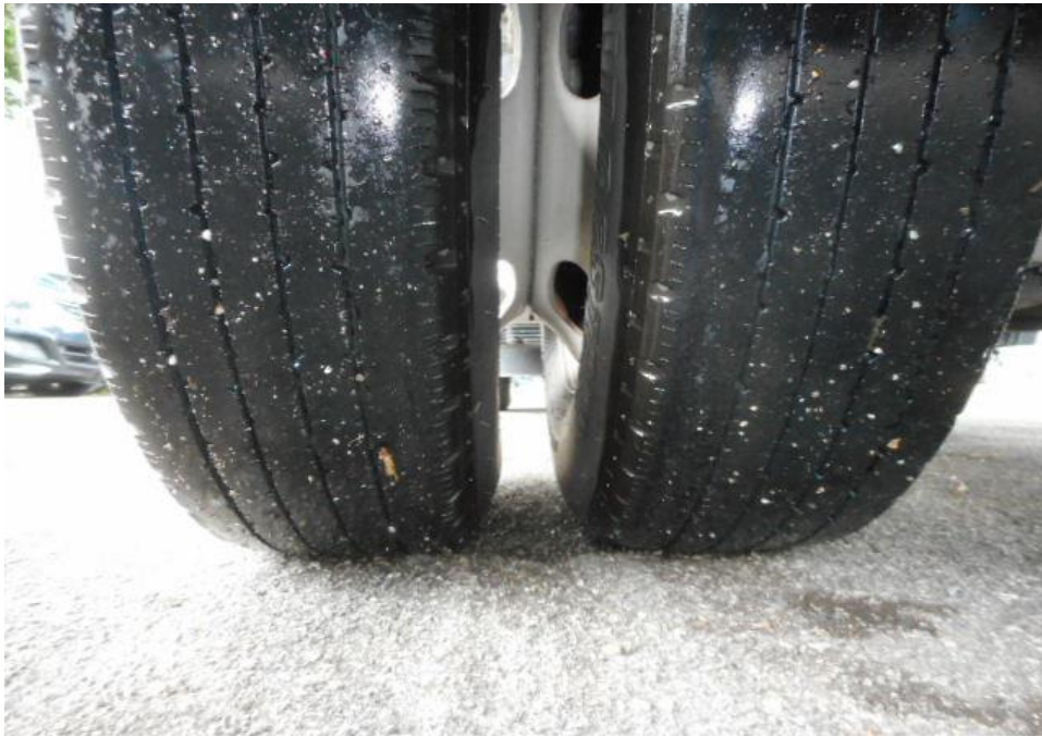
Photo 8 shows the condition of the rear left tyres of the Motor Lorry, which was observed to be in serviceable condition with remaining tread depth of approximately 4.2mm. The tyres, which were wrapped around standard steel wheel rim, were also observed to be sufficiently inflated for vehicular operation.
