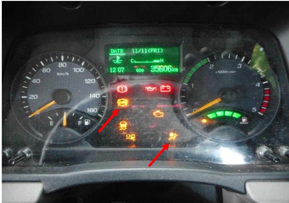
Photo 23 shows the warning light for Anti-Lock Brake System (ABS) and Supplemental Restraint System (SRS) (arrowed) appearing on the instrument panel of the Motor Lorry during the self-test of its various electronic operating systems when its engine was cranked.
