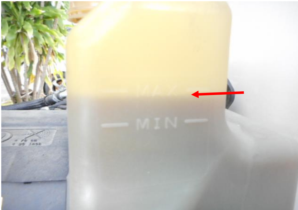
Photo 14 shows the power steering fluid reservoir of the Motor Lorry at the time of my inspection. The power steering fluid (arrowed) was observed to be of sufficient level and without any visible contamination.
