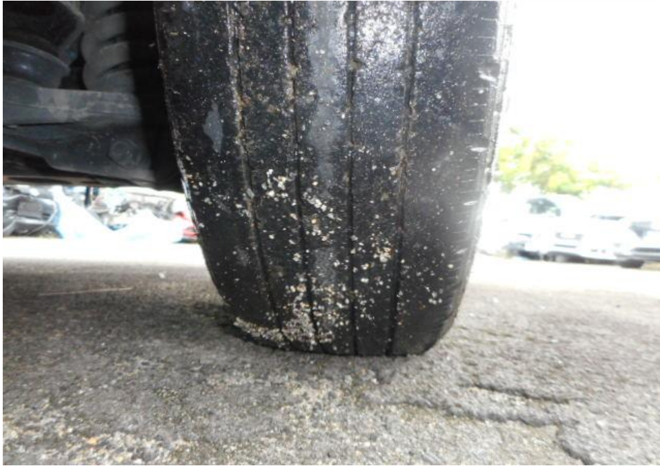
Photo 6 shows the condition of the front right tyre of the Motor Lorry, which was observed to be in serviceable condition with remaining tread depth of approximately 4.6mm. The tyre, which was wrapped around standard steel wheel rim, it was observed to be sufficiently inflated for vehicular operation.
