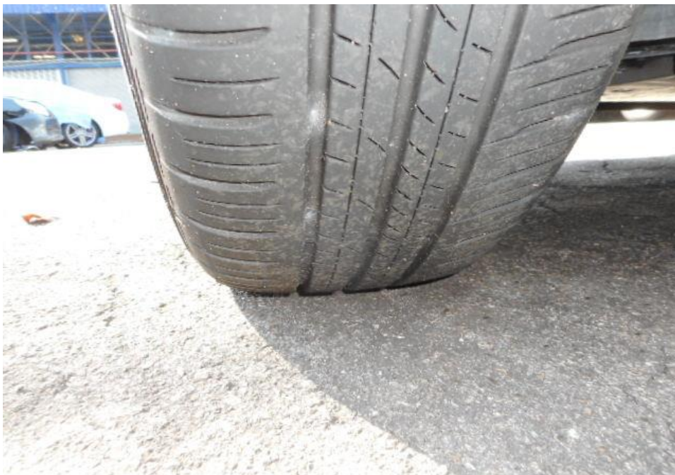
Photo 14 shows the condition of the front left tyre of the Motor Car, which was observed to be in serviceable condition with remaining tread depth of approximately 5.1mm. The tyre, which was wrapped around alloy wheel rim, was also observed to be sufficiently inflated for vehicular operation.
