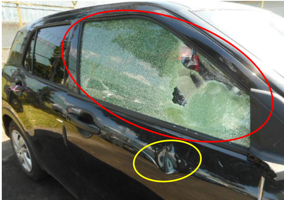
Photo 5 shows a close up view of the Motor Car's right body at the time of my inspection. The Motor Car was observed to have sustained damage at its right portion. Its front right door (yellow circle), its front right door windscreen (red circle) was the body parts that were damaged as a result of the accident.
