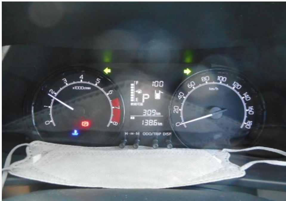
Photo 27 shows no warning lights illuminated on the instrument panel of the Motor Car after the engine was cranked. This would suggest that there was no abnormality to the electronic operating system of the Motor Car, like the ABS, EPS, TCS and SRS etc.
