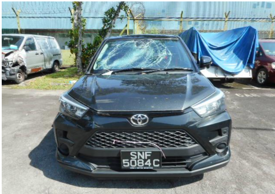
Photo 2 shows a general view of the Motor Car's front body at the time of my inspection. Its front and right portion. Its front windscreen, front right front door, its front right door windscreen, front right fender and right rear view mirror was the body parts that were damaged as a result of the accident.
