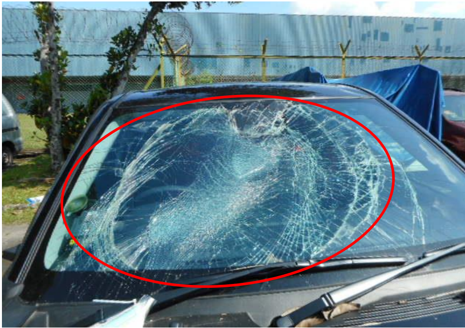
Photo 3 shows a close up view of the Motor Car's front body at the time of my inspection. The front portion of the Motor Car was observed to have sustained damage. Its front windscreen (circled) was the body parts that were damaged as a result of the accident.
