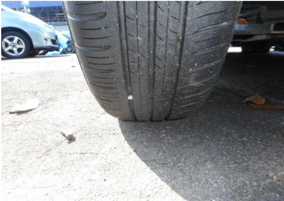
Photo 13 shows the condition of the rear left tyre of the Motor Car, which was observed to be in serviceable condition with remaining tread depth of approximately 5.7mm. The tyre, which was wrapped around alloy wheel rim, was also observed to be sufficiently inflated for vehicular operation.
