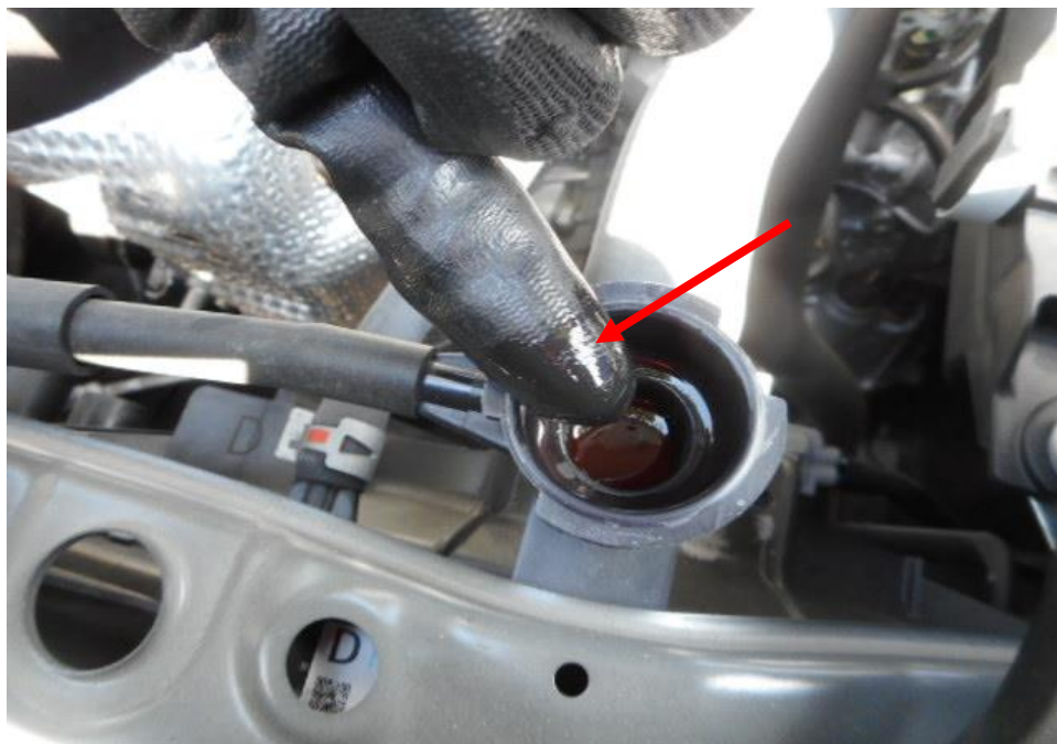
Photo 17 shows checks being carried out to the engine coolant of the Motor Car at the time of my inspection. The engine coolant was observed to be of sufficient level (arrowed) and without any visible contamination.
