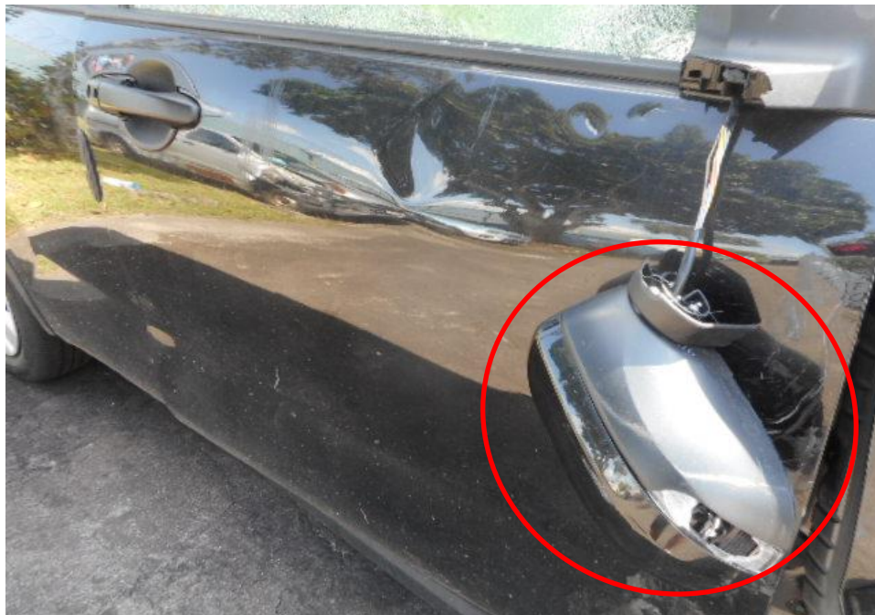
Photo 6 shows a close up view of the Motor Car's right body at the time of my inspection. The Motor Car was observed to have sustained damage at its right portion. Its right rear view mirror (circled) was the body parts that were damaged as a result of the accident.
