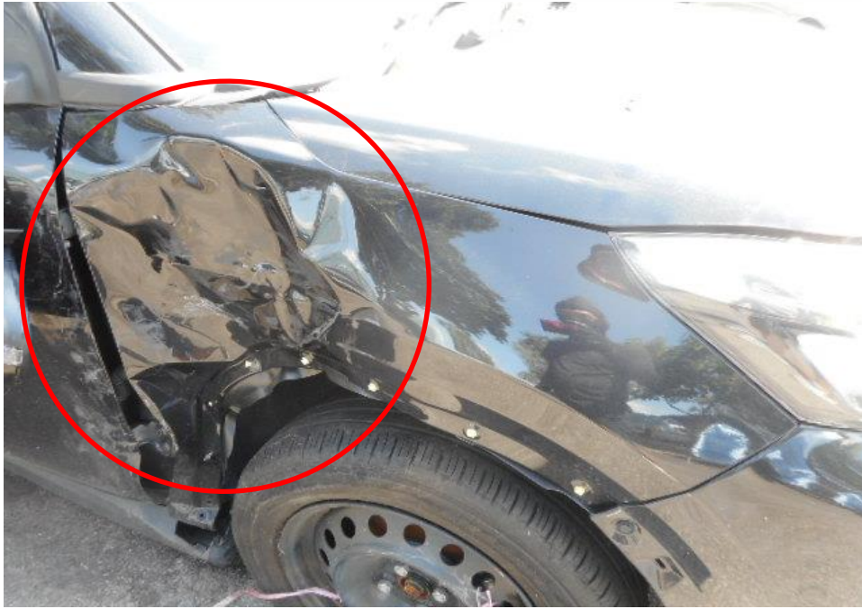
Photo 7 shows a close up view of the Motor Car's right body at the time of my inspection. The Motor Car was observed to have sustained damage at its right portion. Its front right fender (circled) was the body parts that were damaged as a result of the accident.
