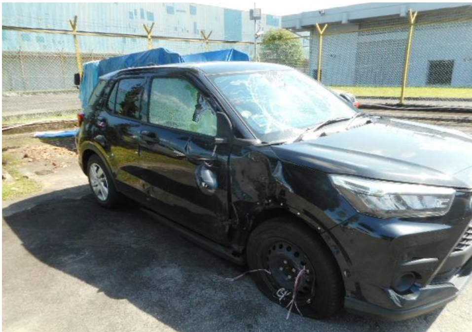
Photo 4 shows a general view of the Motor Car's right body at the time of my inspection. The Motor Car was observed to have sustained damage at its right portion. Its front right door, its front right door windscreen, front right fender and right rear view mirror was the body parts that were damaged as a result of the accident.
