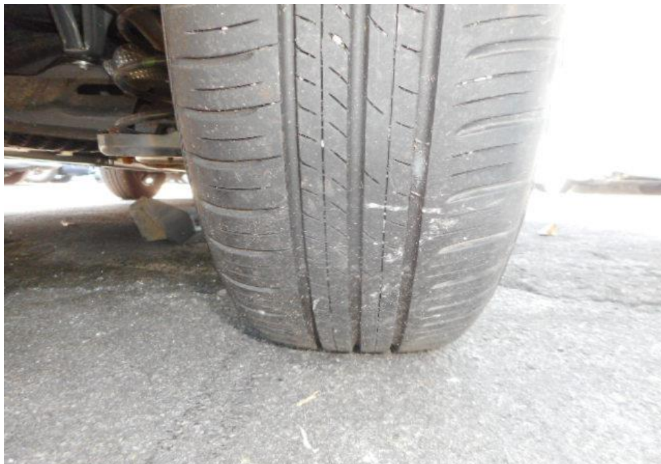
Photo 12 shows the condition of the rear right tyre of the Motor Car, which was observed to be in serviceable condition with remaining tread depth of approximately 5.8mm. The tyre was also observed to be sufficiently inflated for vehicular operation with no tear, cut or burst mark(s).
