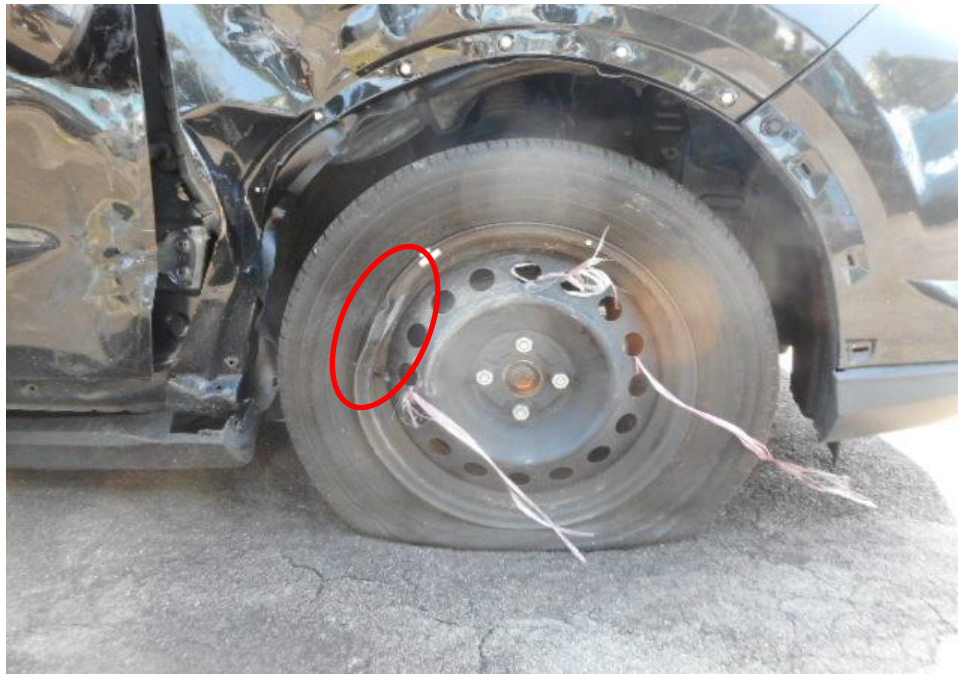
Photo 10 shows the general view of the front right tyre and wheel rim which was damaged with a burst mark on the outer side wall of the tyre and a dent on the wheel rim (circled) due to the impact sustain as a result of the accident. Its remaining tread depth was of approximately 4.8mm.
