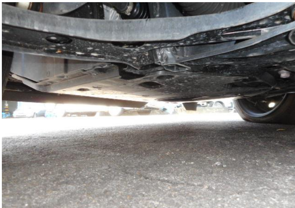
Photo 19 shows the undercarriage of the Motor Car, at the area where the engine housing and transmission housing are located. I did not find any sign(s) or indication(s) of fluid leak and/or fluid stain(s) on the underside of the Motor Car.
