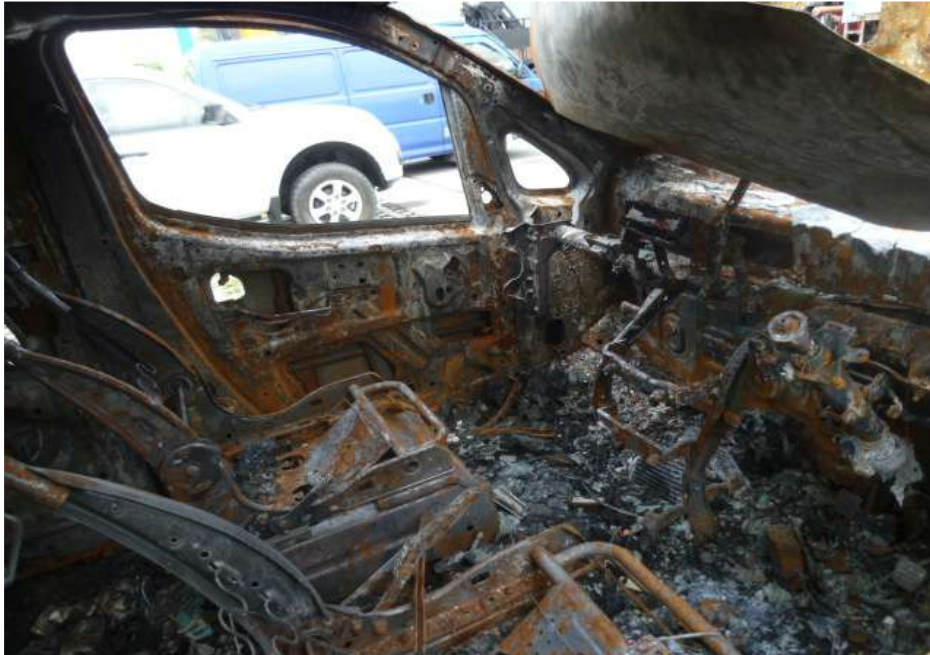
Photo 3 shows the general view of the interior compartment of the Insured Vehicle at the time of our inspection. Its interior compartment was completely burnt.
