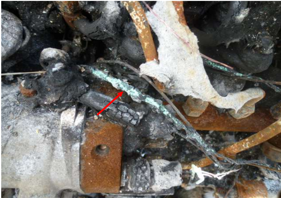
Photo 9 shows a close up view of the greenish residue found on some of the burnt wirings at the centre portion of the engine compartment (arrowed). The presence of such greenish residue suggests occurrence of an electrical short circuit.
