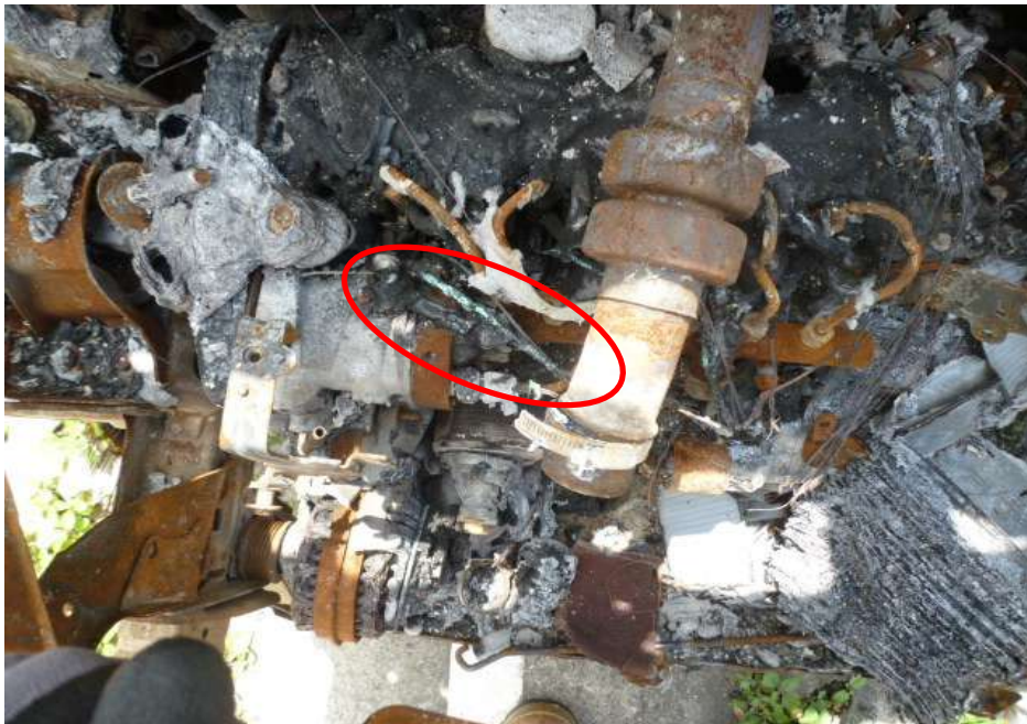
Photo 7 shows a closer view of the burnt stretches of original factory fitted wirings at the centre portion of the engine compartment, which is in the immediate vicinity where the fire to the Insured Vehicle had likely started. Traces of greenish residue were found on some of the wirings (circled).
