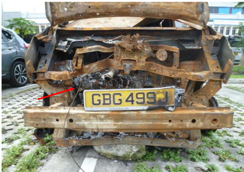
Photo 5 shows a closer view of the frontal portion of the Insured Vehicle. The fire appears to have originated within the engine compartment of the Insured Vehicle due to the nature of the fire damage which was more extensive at the engine compartment (arrowed).
