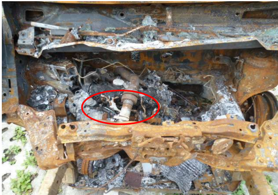
Photo 6 shows the burnt stretches of original factory fitted wirings at the centre portion of the engine compartment, which is in the immediate vicinity where the fire to the Insured Vehicle had likely started. Traces of greenish residue were found on some of the wirings (circled). The presence of greenish residue indicates internal heating of copper wires, a sign of an electrical short circuit occurring. The greenish residue is normally left behind from oxidation as a result of chemical reaction involving the copper wires.
