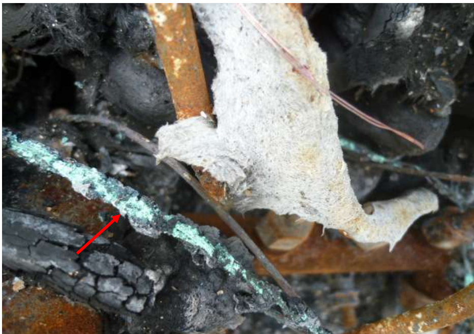
Photo 10 show shows a close up view of the greenish residue found on some of the burnt wirings at the centre portion of the engine compartment (arrowed). The presence of such greenish residue suggests occurrence of an electrical short circuit.
