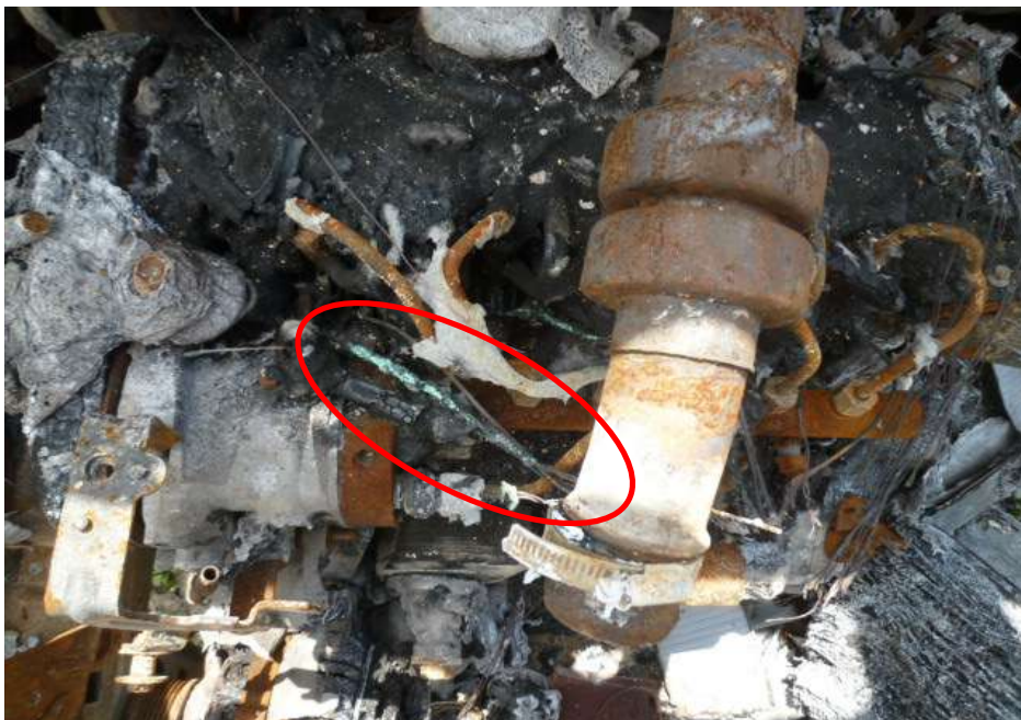
Photo 8 shows a closer view of the greenish residue found on some of the burnt wirings at the centre portion of the engine compartment (circled). The presence of such greenish residue suggests occurrence of an electrical short circuit.
