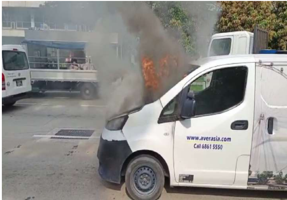
Photo 12 shows the Insured Vehicle on fire before the arrival of the SCDF. In general, the information that could be gathered from this photograph had corresponded to the events that were related to us by Mr Tan which is the fire had started from the engine compartment of the Insured Vehicle (arrowed).
