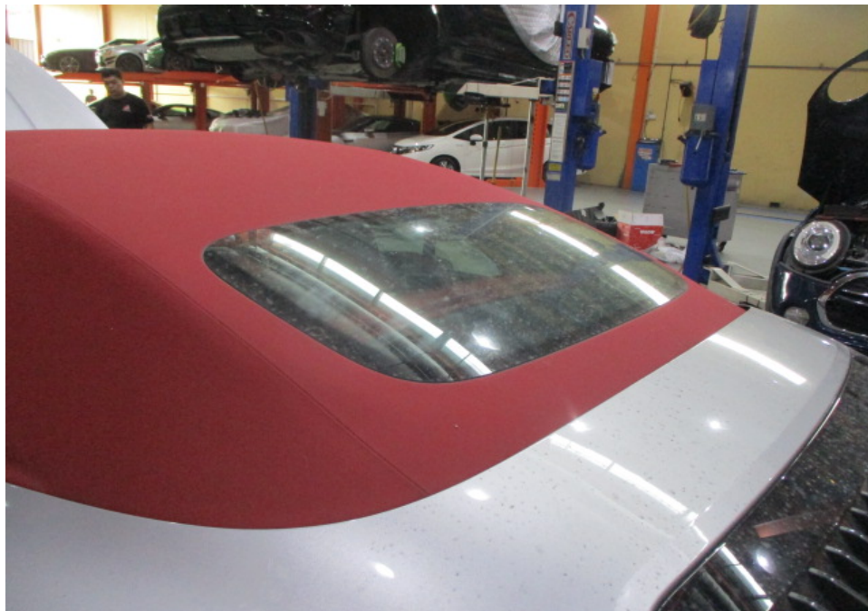
Photo 14 shows a closer view of the Motor Car's rear windscreen and soft top roof. The body parts at the rear portion of the Motor Car were visually examined and it was observed that the repair/restoration works carried out to the damaged area of the Motor Car (refer to photograph 3 & 4 above) were reasonably adequate and in order.
