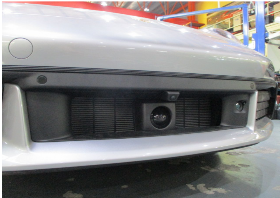
Photo 10 shows a closer view of the Motor Car's front bumper, front bumper centre lower air duct and front radar/sensor unit. The body parts at the frontal portion of the Motor Car were visually examined and it was observed that the repair/restoration works carried out to the damaged area of the Motor Car (refer to photograph 1 & 2 above) were reasonably adequate and in order.
