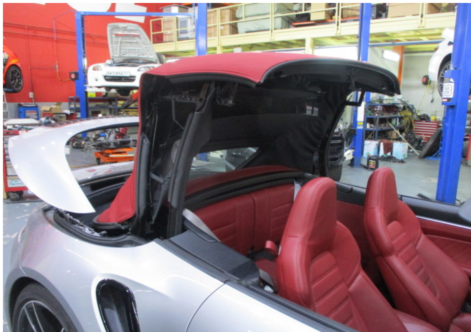
Photo 18 shows the Motor Car's soft top roof being tested. It was observed that as a safety feature, the soft top roof could only open and close when the Motor Car was in a stationary position. When opened, the soft top roof is completely folded into the rear compartment with no parts protruding out of the Motor Car's body. The soft top roof was also found adequately secured to the "A" pillar after closing.
