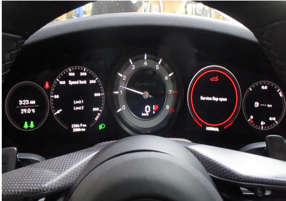
Photo 21 shows the respective warning lights no longer illuminated, indicating that there is no fault detected to the ABS, SRS, EPS, TPM and TCS systems of the Motor Car during the self-test. These electronic systems were hence in working condition at the time of my inspection.
