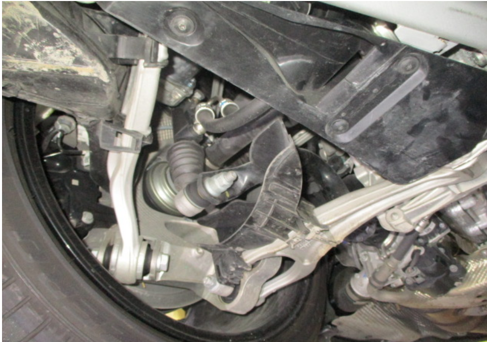
Photo 23 shows a general view of the control arms and linkages at the rear right wheel of the Motor Car. I did not observe any fluid leak and/or fluid stain on the underside of the Motor Car. All of the Motor Car's undercarriage components were observed to be intact and secured in an appropriate manner.
