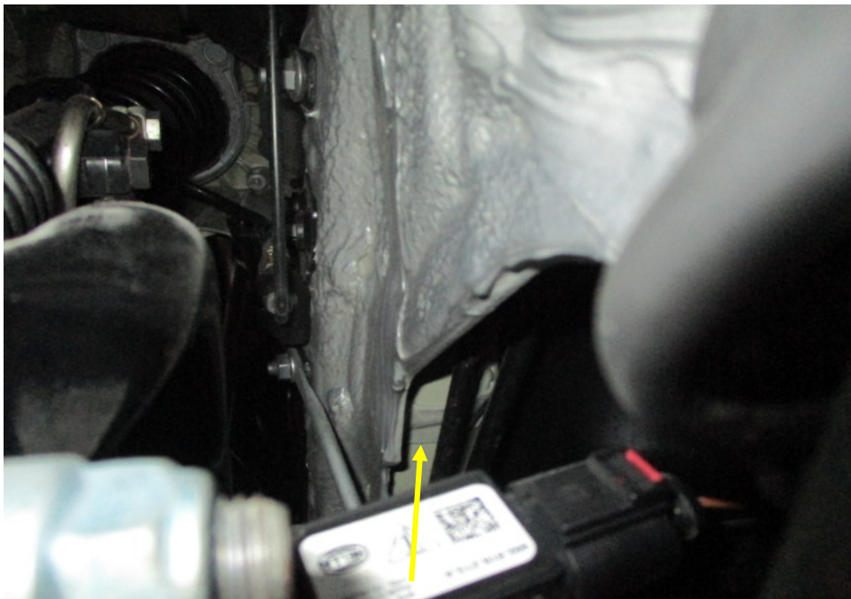
Photo 32 shows the chassis/structural body at the underside front left of the Motor Car. I did not find any weld marks other than original spot weld marks on the chassis/structural body of the Motor Car. The original factory sealant (arrowed) at the joints along the chassis/structural body was untouched, indicating no work was done on the chassis/structural body of the Motor Car and that the chassis/structural body was originally fitted.
