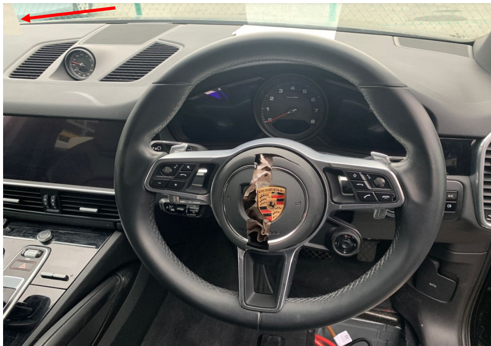
Photo 7 shows the interior compartment of the Motor Car (photograph provided to me). The driver's airbag and front left passenger airbag (arrowed) were deployed as seen from the photographs that were provided to me.
