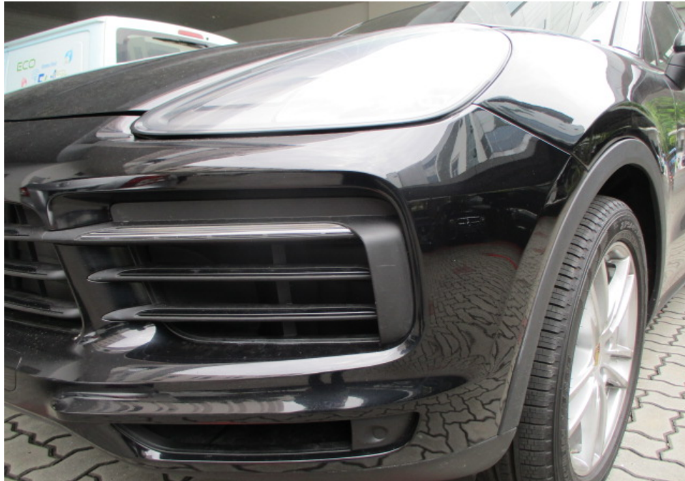
Photo 9 shows a closer view of the Motor Car's front bumper, front bumper left upper grille, front bumper left lower grille, front bumper left sensor, front left day light and front left headlamp. The body parts at the left front portion of the Motor Car were visually examined and it was observed that the repair/restoration works carried out to the damaged area of the Motor Car (refer to photograph 1 & 2 above) were reasonably adequate and in order.
