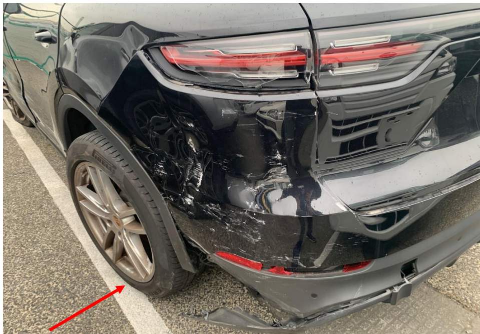
Photo 5 shows a closer view of the damage at the left rear portion of the Motor Car (photograph provided to me). The rear left wheel rim, rear left fender, rear left fender wheel arc garnish, rear bumper and rear left taillamp were amongst the body parts that were observed to have been damaged. The rear left wheel (arrowed) was observed to be orientated towards the left, suggesting damage to the undercarriage parts at the rear left wheel of the Motor Car.
