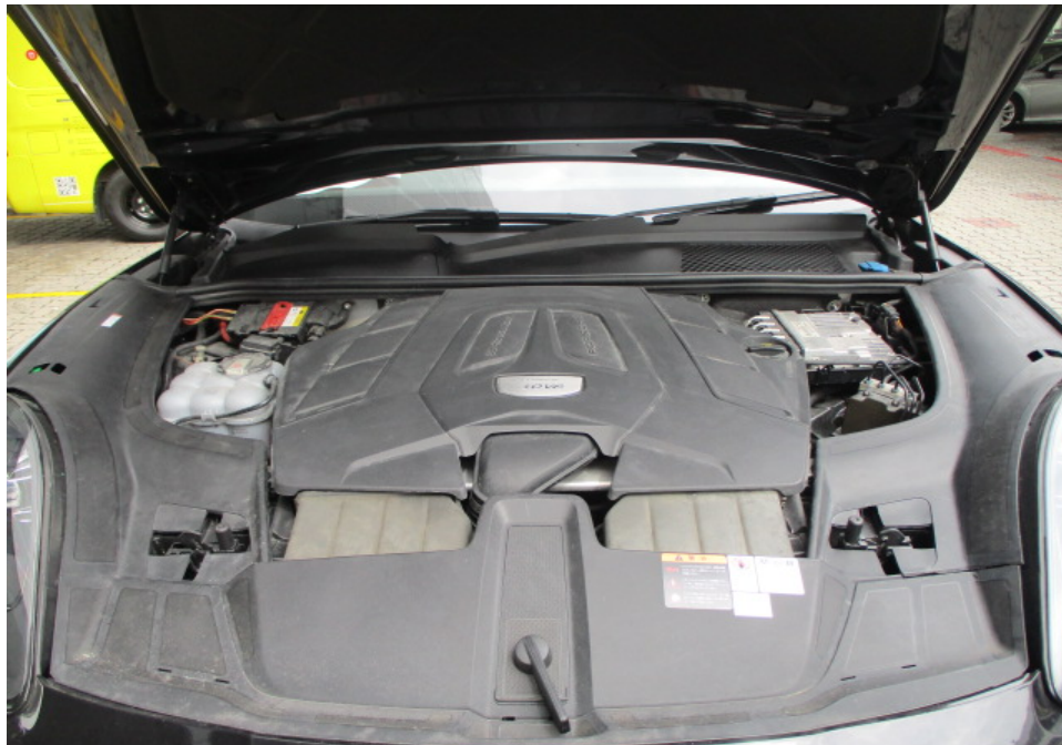
Photo 18 shows a general view of the engine compartment of the Motor Car at the time of my inspection. The various parts and components inside the engine compartment were all observed to be intact and properly fitted. There was also no sign(s) or indication(s) of fluid leak and/or fluid stain found inside the engine compartment.
