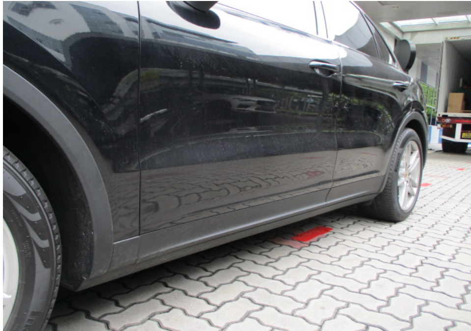
Photo 11 shows a closer view of the Motor Car's front left fender, front left door, rear left door and left side rocker panel garnish. The body parts at the left centre portion of the Motor Car were visually examined and it was observed that the repair/restoration works carried out to the damaged area of the Motor Car (refer to photograph 3 above) were reasonably adequate and in order.
