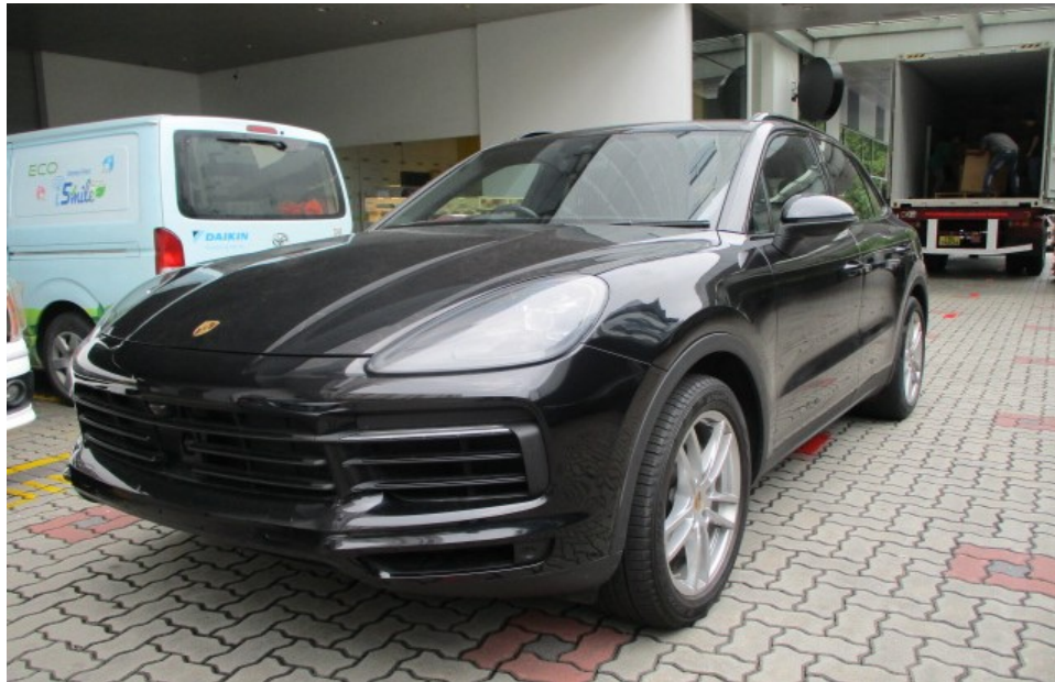
Photo 8 shows a general view of the front left body of the Motor Car at the time of my inspection. The Motor Car was observed to be in a relatively good general condition with no loose exterior fittings observed. The body parts along the entire left side portion of the Motor Car were visually examined and it was observed that the repair/restoration works carried out to the damaged area of the Motor Car (refer to photograph 1 – 5 above) were reasonably adequate and in order.
