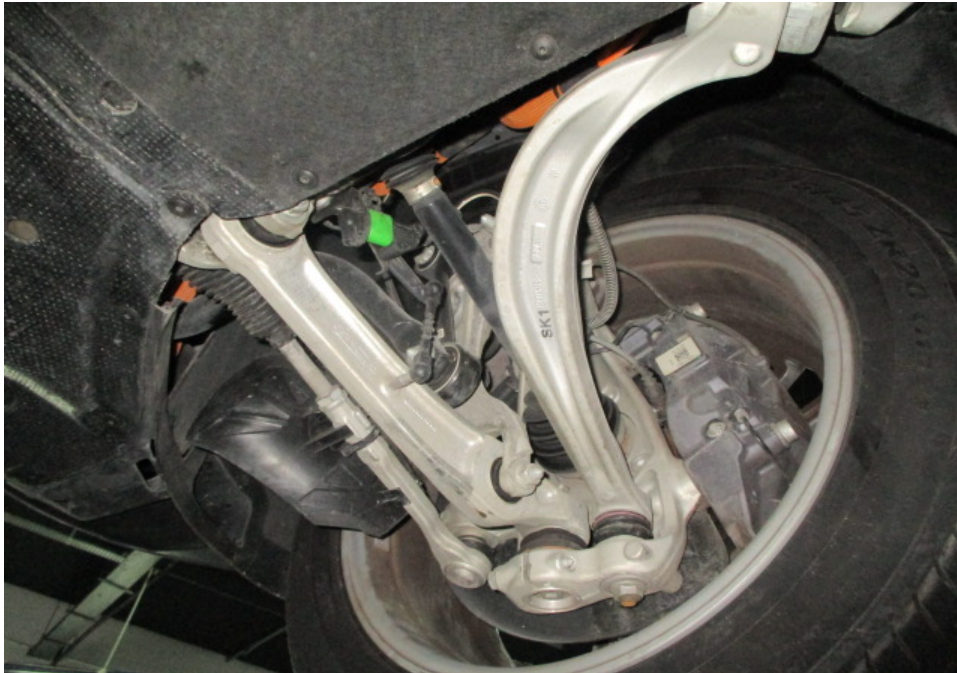
Photo 27 shows the various undercarriage components at the front right wheel of the Motor Car. The mechanical components, control arms and linkages were all found to be intact and secured in an appropriate manner. I also did not observe any fluid leak and/or fluid stain on the underside of the Motor Car.
