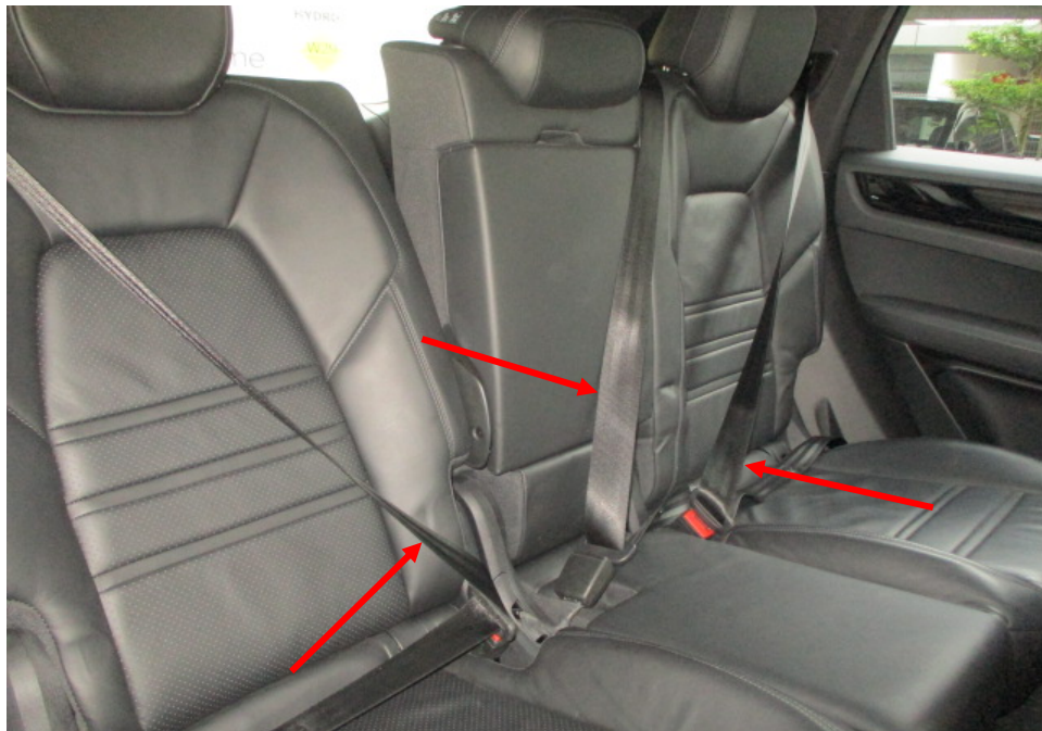
Photo 20 shows the rear seats of the Motor Car. All the seats of the Motor Car were secured via seat rails to the floorboard. They were also fitted with a retractable seat belt reel and a pre-tensioner. The seat belts (arrowed) were tested and were able to be fastened into the respective pre-tensions that were fitted on the side of each individual seat.
