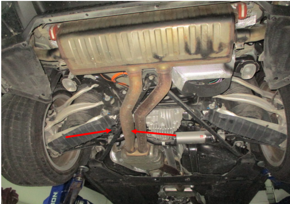
Photo 28 shows the rear section of the Motor Car's exhaust system. My examination of the Motor Car's exhaust system revealed no sign(s) or indication(s) of any cut or weld marks along its exhaust pipes (arrowed), on its rear muffler, on its centre resonator boxes and on its catalytic converter.
