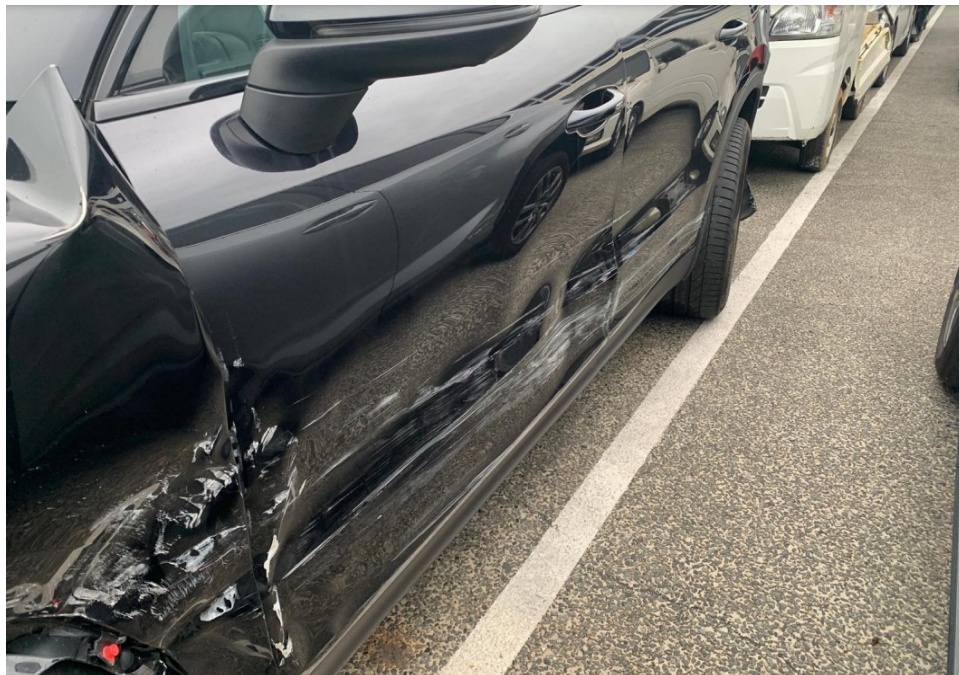
Photo 3 shows a closer view of the damage at the left centre portion of the Motor Car (photograph provided to me). The front left door and rear left door were amongst the body parts that were observed to have been damaged.
