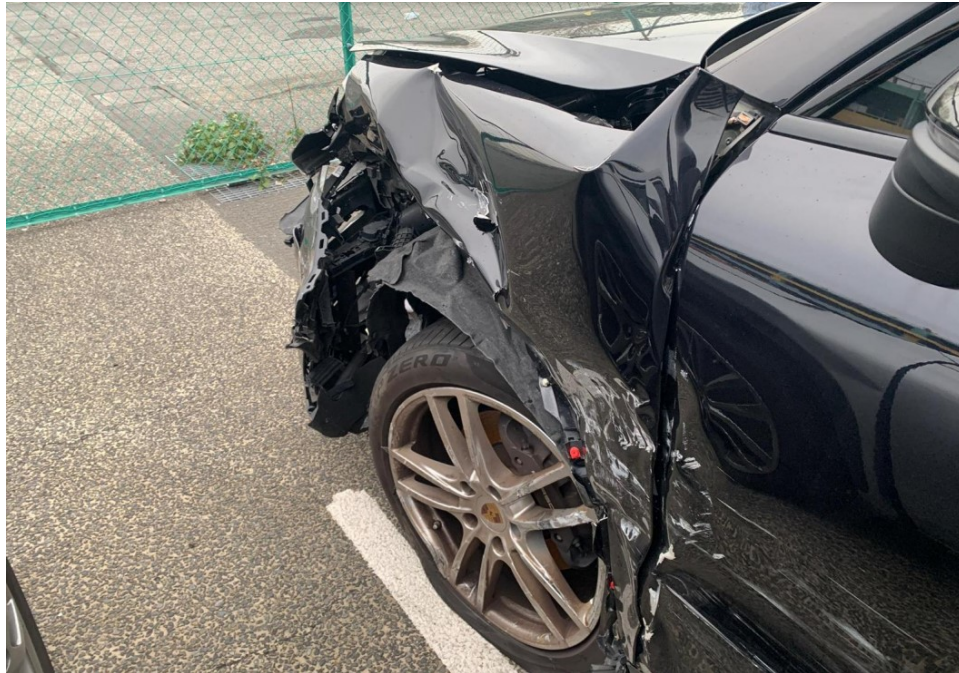
Photo 2 shows a closer view of the damage at the left front portion of the Motor Car (photograph provided to me). The front left door, front left fender, front left fender wheel arc garnish, front left fender inner shield, front left wheel rim and front left tyre were amongst the body parts that were observed to have been damaged. The front left wheel was observed to be orientated towards the left while the front right wheel (refer to photograph 6 below) was observed to be orientated straight. This would suggest damage to the undercarriage parts at the front left wheel of the Motor Car.
