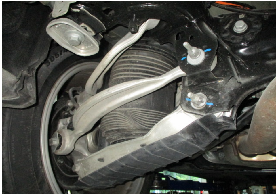
Photo 25 shows a general view of the control arms and linkages at the rear left wheel of the Motor Car. I did not observe any fluid leak and/or fluid stain on the underside of the Motor Car. All of the Motor Car's undercarriage components were observed to be intact and secured in an appropriate manner.
