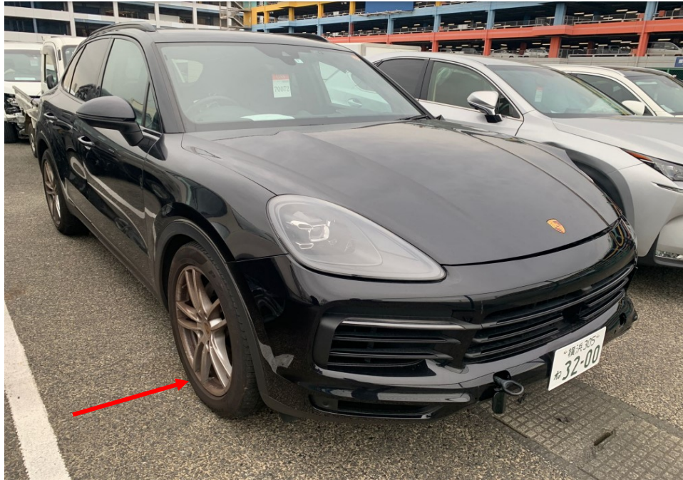
Photo 6 shows the front right body of the Motor Car (photograph provided to me). Apart for the left side portion, there was no physical damage observed to other areas of the Motor Car. The front right wheel (arrowed) was observed to be orientated straight while the front left wheel (refer to photograph 1 & 2 above) was orientated towards the left, suggesting damage to the undercarriage parts at the front left wheel of the Motor Car.
