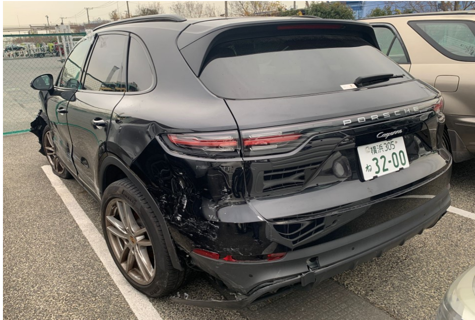
Photo 4 shows the rear left body of the Motor Car (photograph provided to me). The photographs provided to me had showed damage along the entire left side portion of the Motor Car. The rear left wheel rim, rear left fender, rear left fender wheel arc garnish, rear bumper, rear bumper lower cover, rear bumper left reflector, rear left taillamp and rear left tailgate lamp were amongst the body parts that were observed to have been damaged.
