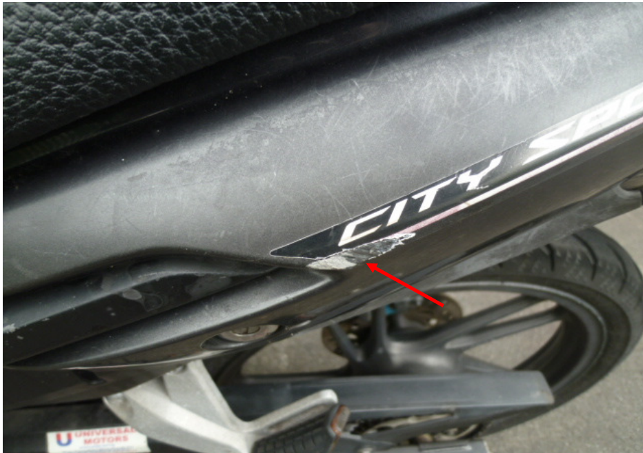
Photo 12 shows a closer view of the grazed left rear side cover of the Motorcycle as a result of the accident (arrowed).
