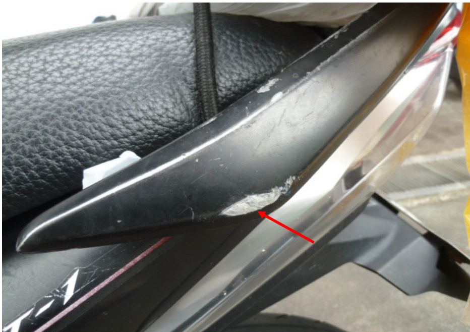
Photo 13 shows a closer view of the grazed left pillion grab rail of the Motorcycle as a result of the accident (arrowed).
