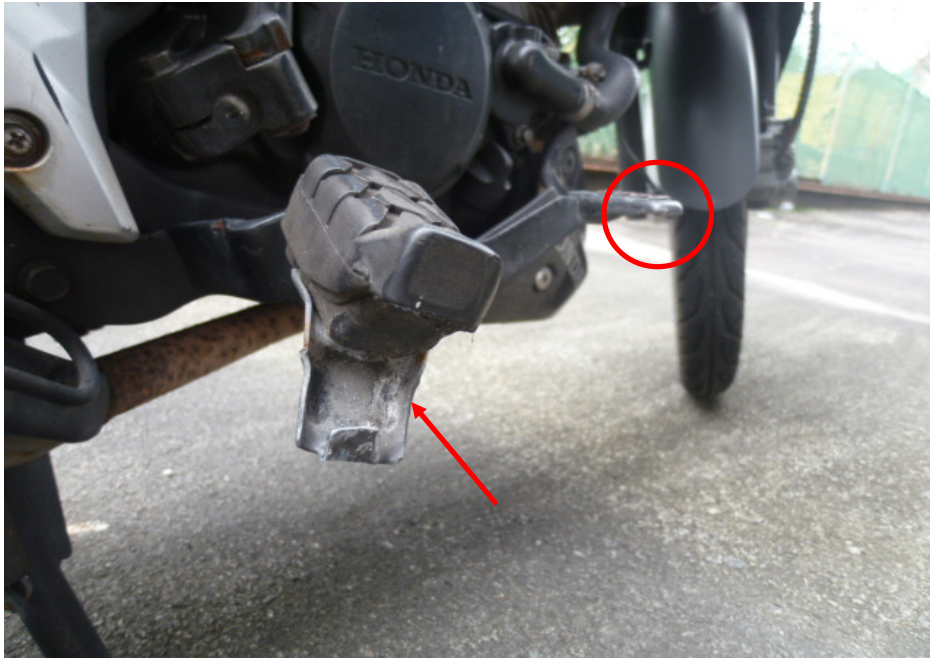
Photo 16 shows the grazed rear brake pedal (circled) and deformed right front footrest (arrowed) of the Motorcycle as a result of the accident.
