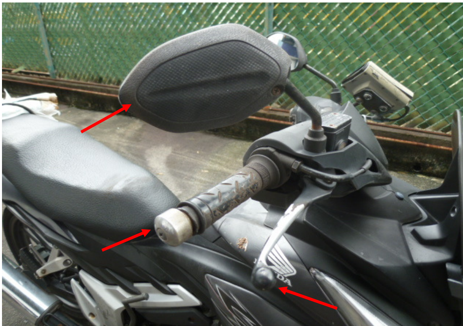
Photo 9 shows the right handlebar end, front brake lever and right side mirror (arrowed), which were amongst the body parts of the Motorcycle that had sustained damage as a result of the accident.
