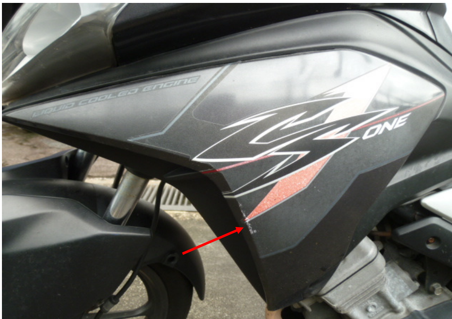
Photo 11 shows a closer view of the grazed left cowling of the Motorcycle as a result of the accident (arrowed).
