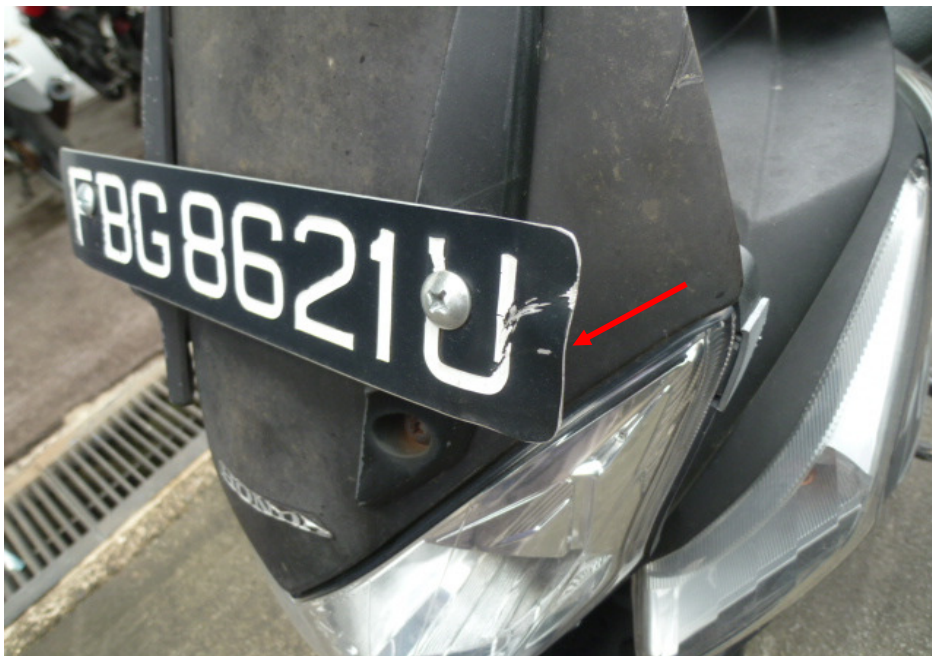
Photo 7 shows the dented front number plate (arrowed) of the Motorcycle as a result of the accident.
