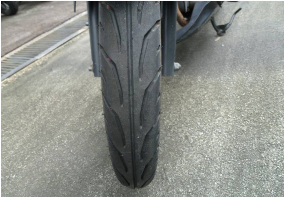
Photo 17 shows the front tyre of the Motorcycle at the time of our inspection. The front tyre was observed to be in serviceable condition with remaining tread depth of approximately 2mm. The pattern of the tread was also clearly visible. There was no tear, burst mark(s) and/or punctured hole(s) on the sidewalls as well as across the tread of the front tyre.
