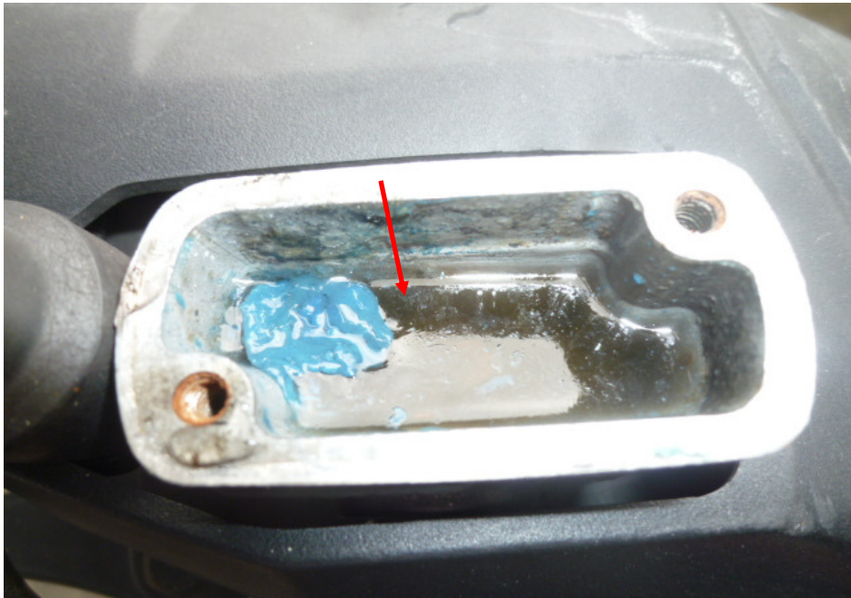
Photo 27 shows a close up view of the brake fluid reservoir for the front brake of the Motorcycle. The front brake fluid was observed to be of sufficient level for operational purposes. However it was found to be contaminated (arrowed).
