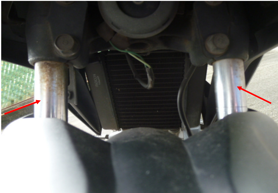
Photo 23 shows the front forks (arrowed) of the Motorcycle. The front forks and fork bracket of the Motorcycle were both found to be intact and undamaged. Turning the Motorcycle's handle bar towards the left and right did not produce any abnormal free play. The steering system of the Motorcycle was in serviceable condition at the time of our inspection.
