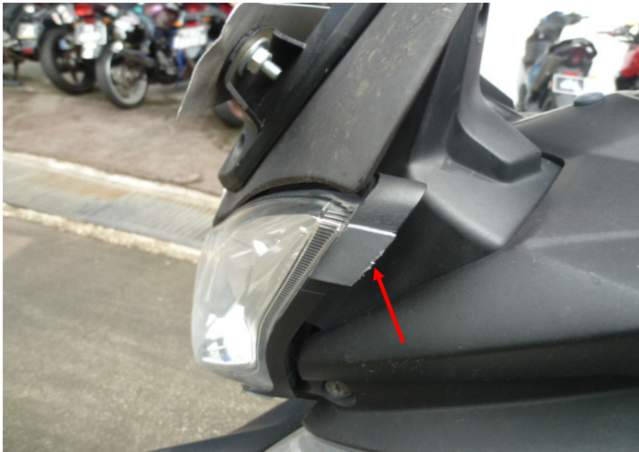
Photo 10 shows a closer view of the grazed head cowl of the Motorcycle as a result of the accident (arrowed).
