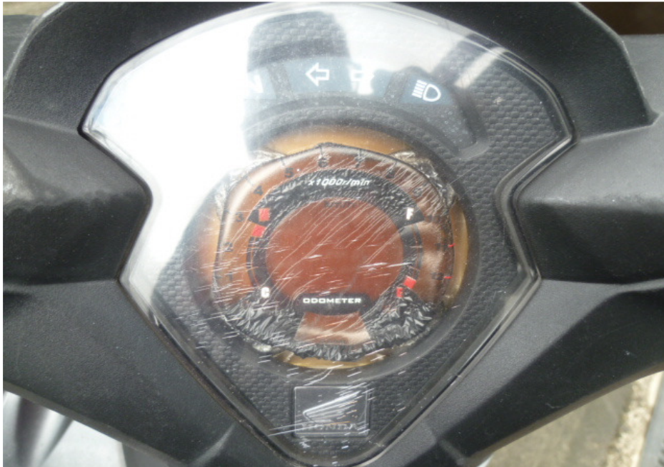
Photo 1 shows the damaged screen of the speedometer gauge of the Motorcycle. Hence the mileage of the Motorcycle could not be recorded at the time of our inspection.
