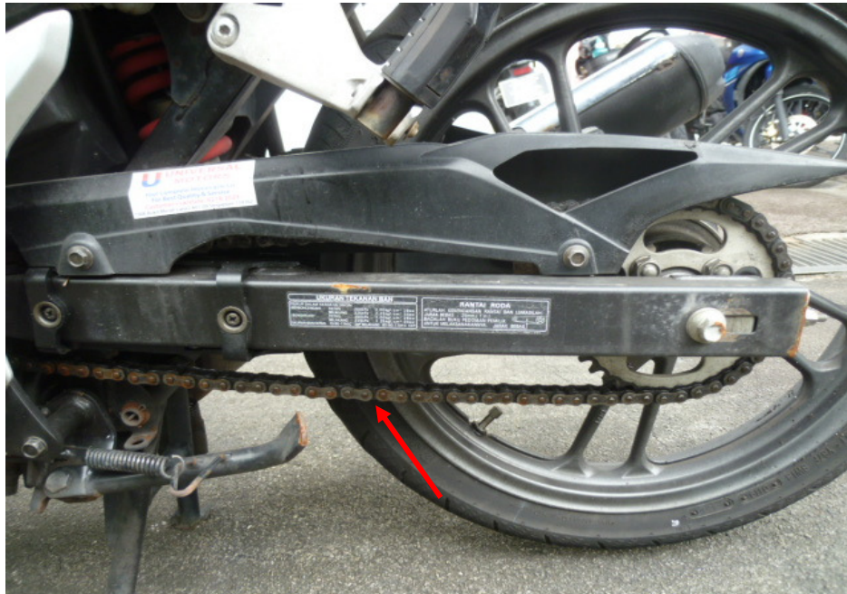
Photo 21 shows the general view of the gear train (arrowed) of the Motorcycle, which was observed to be intact with no misalignment. It was also adequately lubricated for operating purposes. The gear train rotates the rear wheel of the Motorcycle
