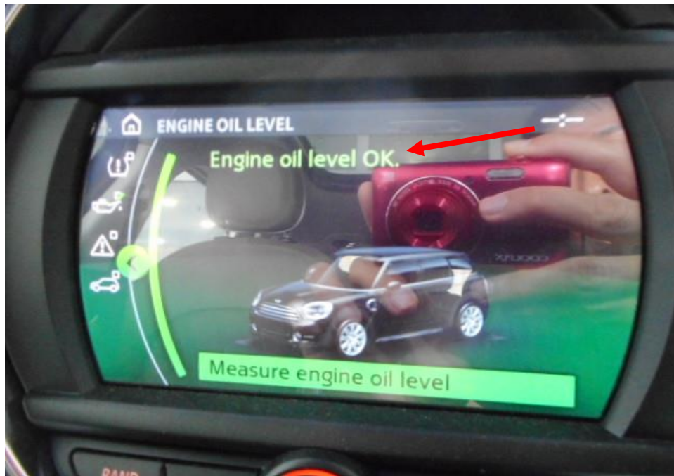
Photo 13 shows the instrument panel display of the engine oil level (arrowed) of the Motor Car at the time of my inspection. The engine oil was observed to be of sufficient level and without any visible contamination.
