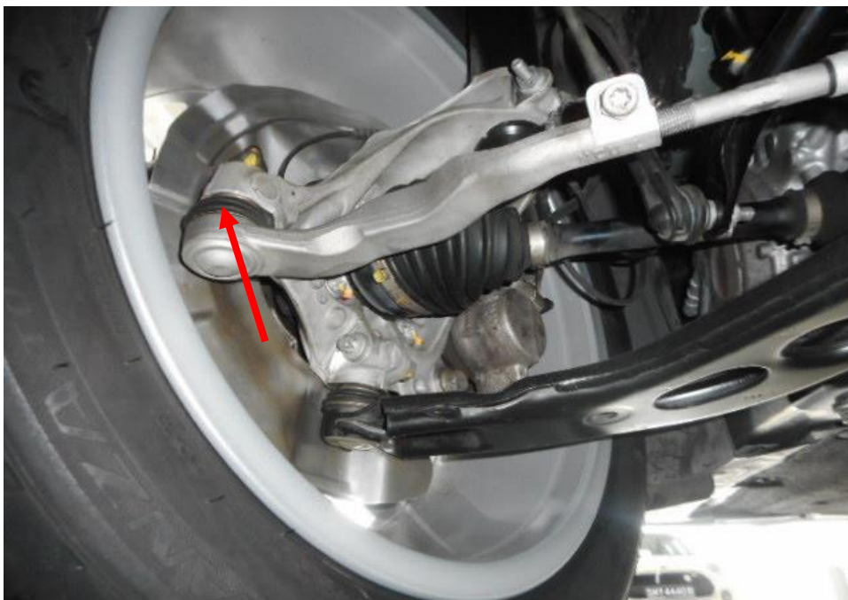
Photo 21 shows the various undercarriage components at the front left wheel of the Motor Car, which had included the steering tie rod (arrowed). The various undercarriage components of the Motor Car were all found to be intact without any visible damage.
