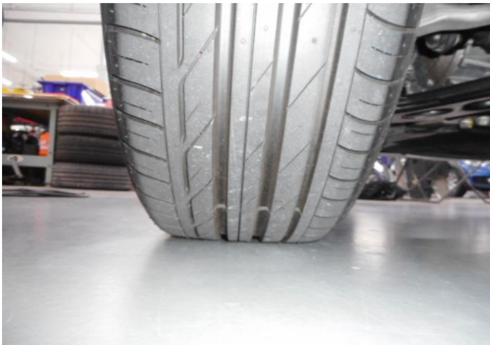
Photo 9 shows the condition of the front left tyre of the Motor Car, which was observed to be in serviceable condition with remaining tread depth of approximately 6.9mm. There was also no tear, cut or burst mark(s) on the outer and the inner sidewalls as well as across the tread of the Motor Car's 4 tyres.
