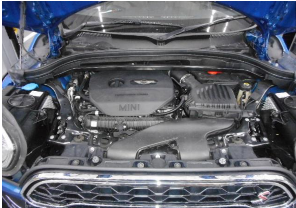
Photo 10 shows a general view of the Motor Car's engine compartment. The various parts and components inside the engine compartment were intact. There was also no sign(s) or indication(s) of fluid leakage and/or fluid stain within the engine compartment.
