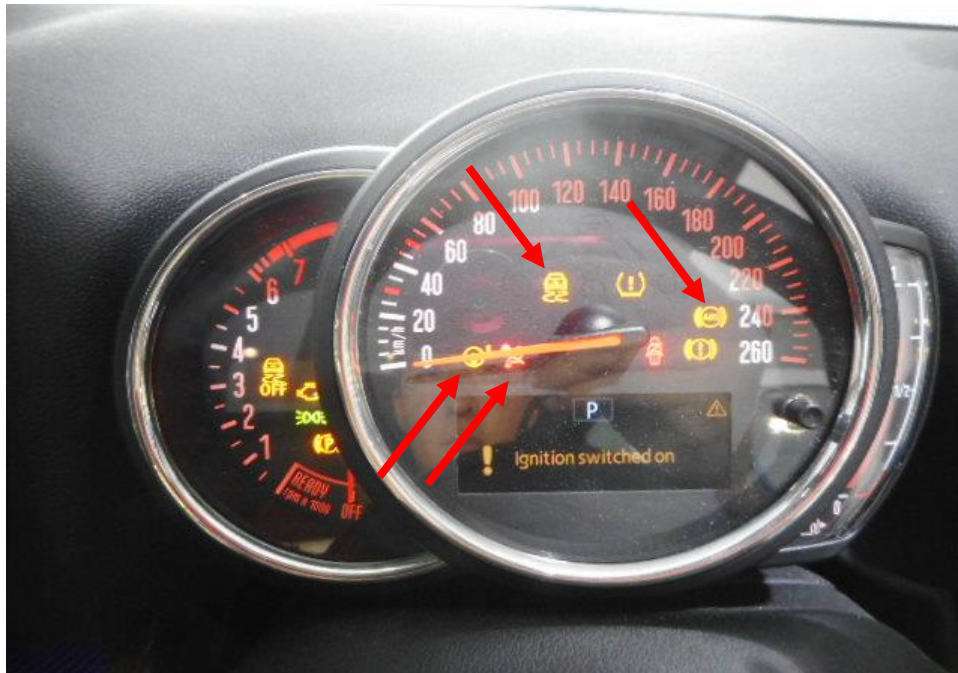
Photo 22 shows the warning light for Anti-Lock Brake System (ABS), Traction Control System (TCS), Electrical Power Steering (EPS) and Supplemental Restraint System (SRS) (arrowed) appearing on the instrument panel of the Motor Car during the self-test of its various electronic operating systems when its engine was cranked.
