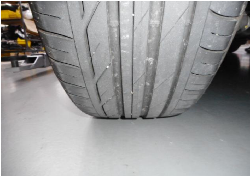
Photo 8 shows the condition of the rear left tyre of the Motor Car, which was observed to be in serviceable condition with remaining tread depth of approximately 5mm. The tyre, which was wrapped around alloy wheel rim, was also observed to be sufficiently inflated for vehicular operation. The 4 tyres of the Motor Car were wrapped around standard alloy wheel rims.
