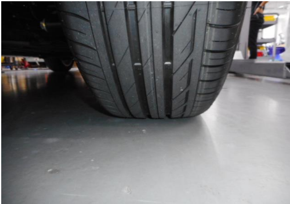
Photo 7 shows the condition of the rear right tyre of the Motor Car, which was observed to be in serviceable condition with remaining tread depth of approximately 6.6mm. The tyre was also observed to be sufficiently inflated for vehicular operation with no tear, cut or burst mark(s).
