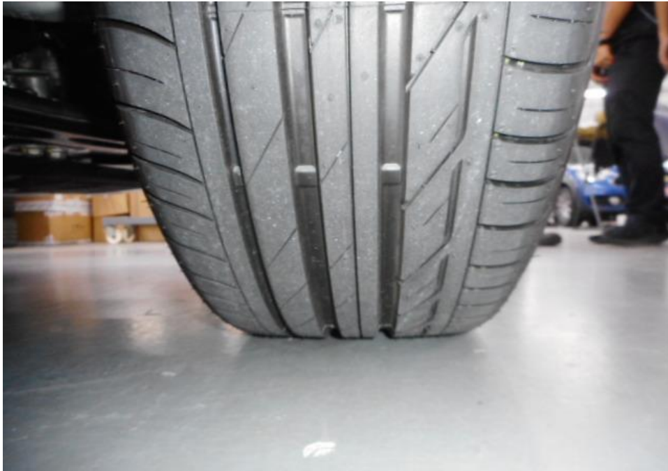
Photo 6 shows the condition of the front right tyre of the Motor Car, which was observed to be in serviceable condition with remaining tread depth of approximately 6.7mm. The tyre was also observed to be sufficiently inflated for vehicular operation with no tear, cut or burst mark(s).
