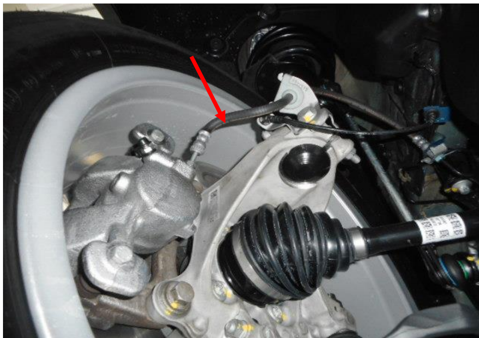
Photo 17 shows the brake hose/pipe (arrowed) at the front right wheel of the Motor Car. I did not observe any leakage of brake fluid at the time of my inspection of the Motor Car. Static tests of the Motor Car's braking system had indicated that there was no internal leakage of pressure/vacuum.
