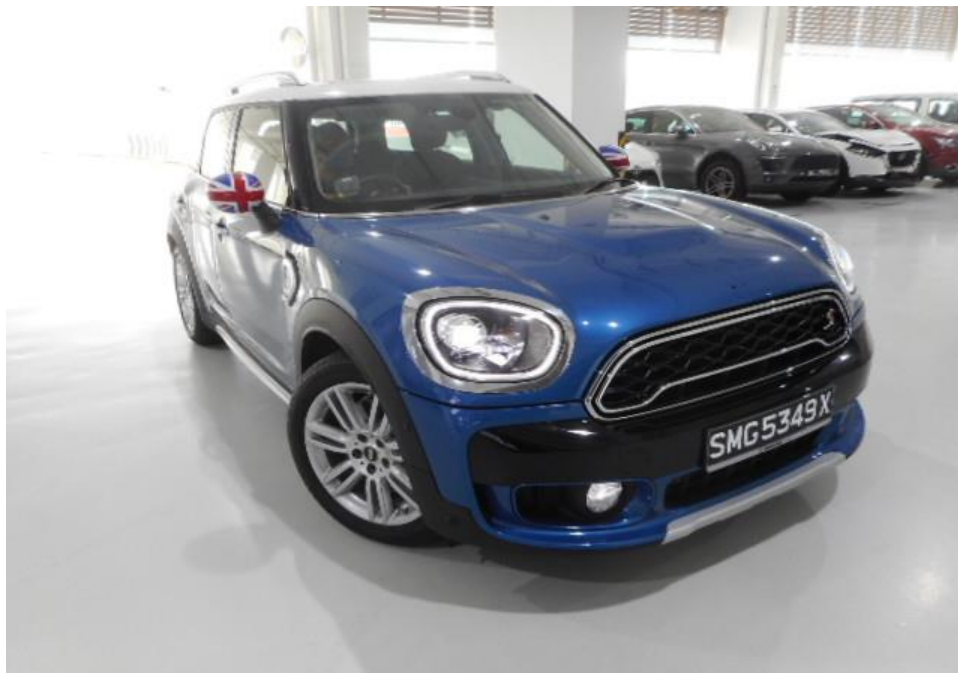
Photo 19 shows the front right wheel of the Motor Car turned to its full left. During my steering system test, I did not experience any abnormal free play and/or resistance when I had turned the steering wheel towards the left and right. This would suggest that the steering system of the Motor Car was in serviceable condition.
