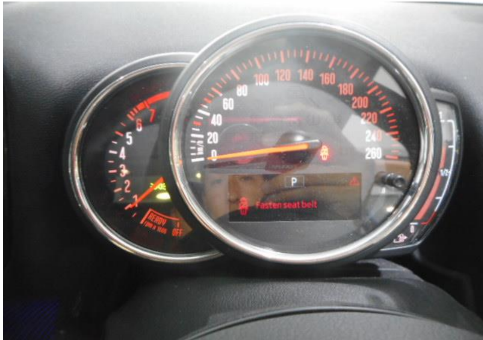
Photo 23 shows no warning lights illuminated on the instrument panel of the Motor Car after the engine was cranked. This would suggest that there was no abnormality to the electronic operating system of the Motor Car, like the ABS, TCS, EPS and SRS etc.
