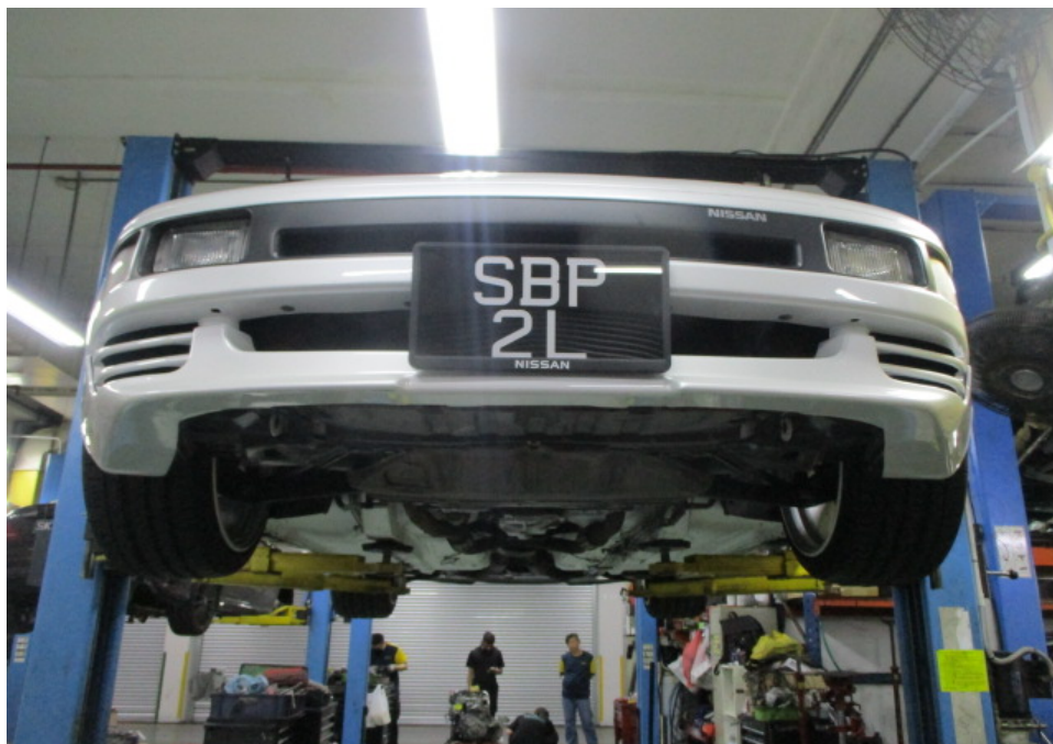
Photo 1 shows the Motor Car hoisted up for checks on its undercarriage, in particular to its transmission assembly. It was noted that the Motor Car was fitted with a 5-speed manual transmission system.
