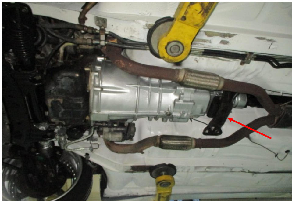
Photo 3 shows another view of the transmission assembly that was fitted on the Motor Car. The front (input) side of the transmission assembly is bolted to the crankshaft side of the engine block while the rear (output) side of the transmission assembly, connects to the propeller shaft, which links to the differential at the rear axle of the Motor Car. A bracket (arrowed) mounted to the underside of the Motor Car's floorboard, via bolts and nuts, supports the rear (output) side of the transmission assembly.
