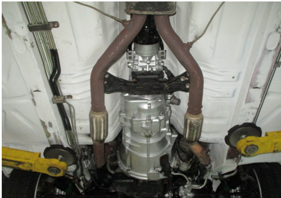
Photo 9 shows a general view of the transmission assembly that was fitted on the Motor Car, as viewed from the rear to front. The front (input) side of the transmission assembly is bolted to the crankshaft side of the engine block while the rear (output) side of the transmission assembly, connects to the propeller shaft, which links to the differential at the rear axle of the Motor Car.
