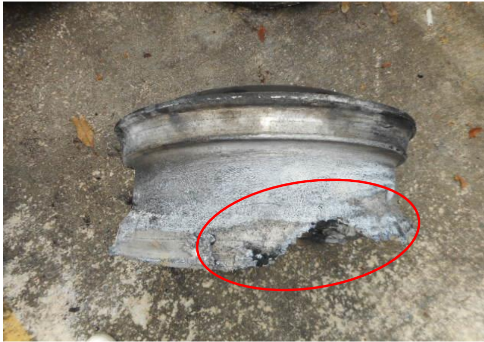
Photo 15 shows a general view of the rear right outer wheel rim of the Insured Vehicle. Upon closer examination, we observed that the dent and cracked wheel rim (circled) was caused by an impact that had caused the deformed damage to it.
