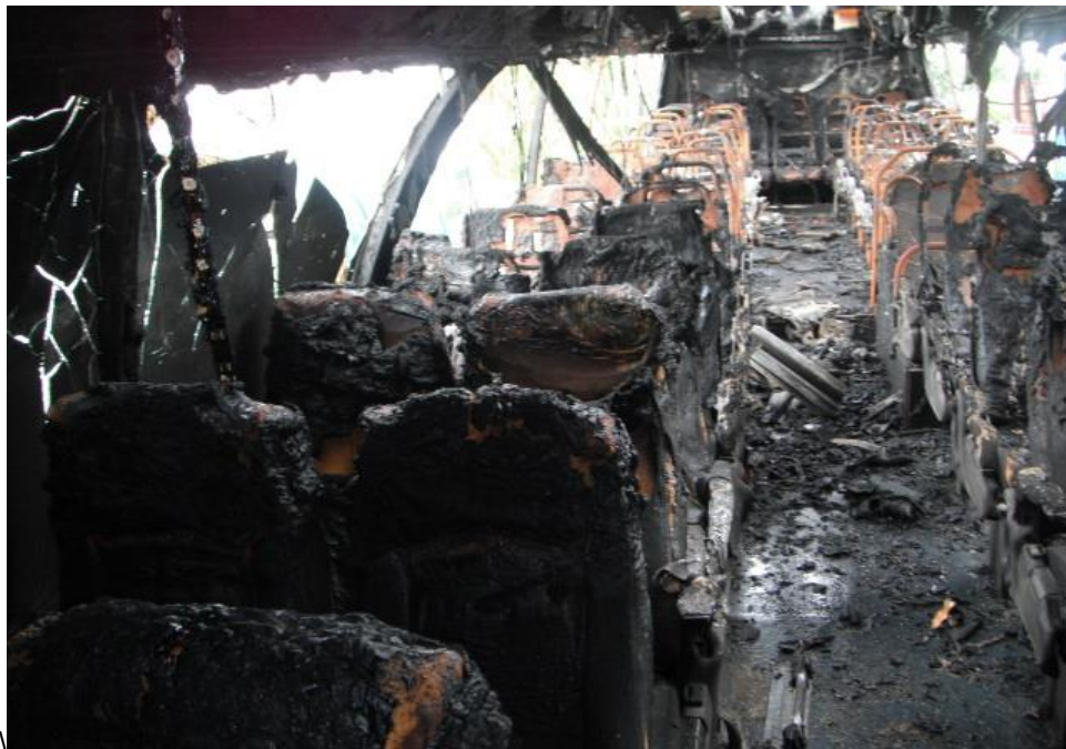
Photo 3 shows the interior cabin of the Insured Vehicle at the time of inspection. The interior rear cabin including its seats and windows was completely burnt.
