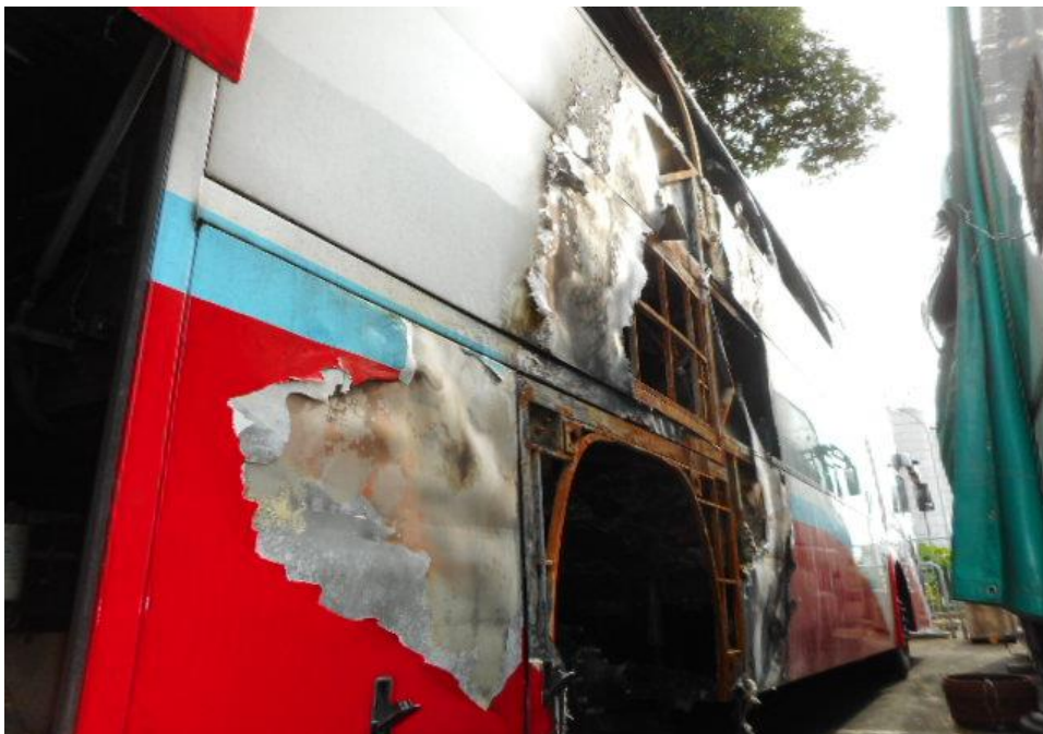
Photo 6 shows the general view of the right portion of the Insured Vehicle at the time of our inspection. The exterior body of the Insured Vehicle had sustained fire damages at the rear right wheel and rim area as well as its rear right body panel portion. Affected parts had included the right rear panels, rear right windows and the rear right wheel and rims.
