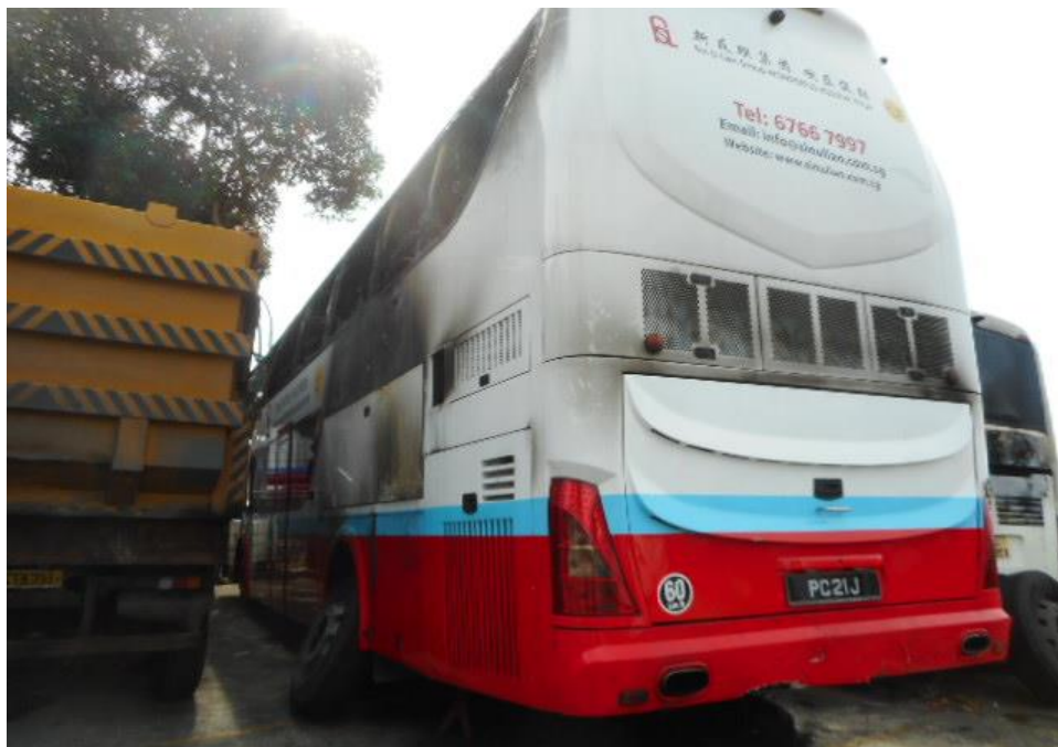
Photo 4 shows the general view of the left portion of the Insured Vehicle at the time of our inspection. The exterior body of the Insured Vehicle had sustained fire damage at the rear portion. Affected parts had included the rear windows and rear left panels.
