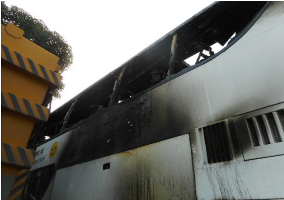
Photo 5 shows the close up view of the left portion of the Insured Vehicle at the time of our inspection. The exterior body of the Insured Vehicle had sustained fire damage at the rear portion. Affected parts had included the rear windows and rear left panels.
