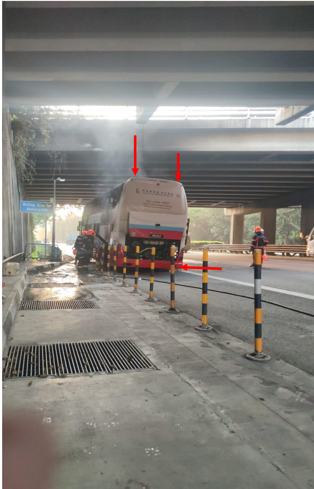
Photo 17 shows that the Insured Vehicle was observed to be tilted down to the right side (arrowed) of the Insured Vehicle at the material time of incident. The photographs had also showed the Insured Vehicle on fire and similar extent of damage and burn pattern to the Insured Vehicle as per what we had observed during our physical inspection of the Insured Vehicle.
