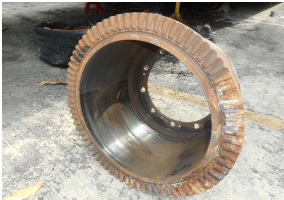
Photo 14 shows a general view of the rear left brake drum of the Insured Vehicle. Upon closer examination, we did not observe any damages to the interior surface of the brake drum.
