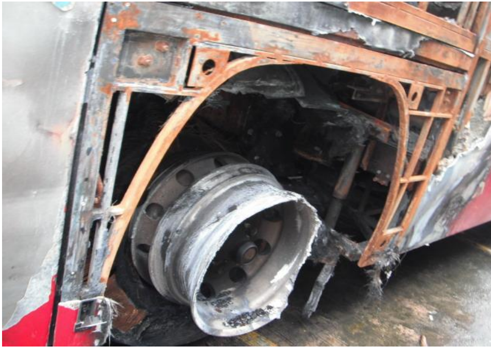
Photo 7 shows the close up view of the rear right portion of the Insured Vehicle at the time of our inspection. The wheel rims and the tyres of the Insured Vehicle had sustained severe fire damage.
