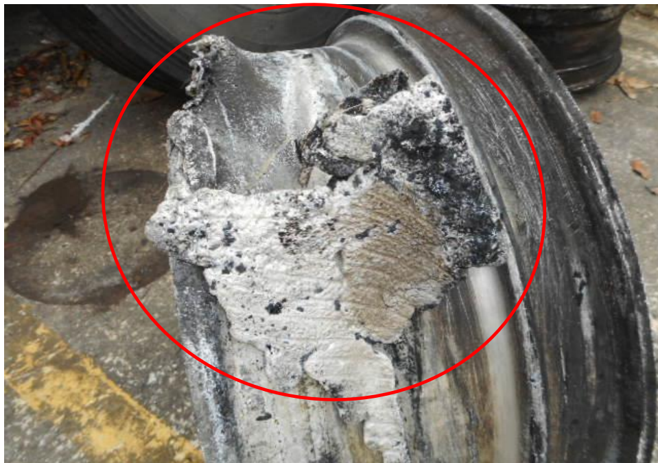
Photo 16 shows a close up view of the rear right outer wheel rim of the Insured Vehicle. Upon closer examination, we observed that the dent and cracked wheel rim (circled) was caused by an impact that had caused the deformed damage to it.
