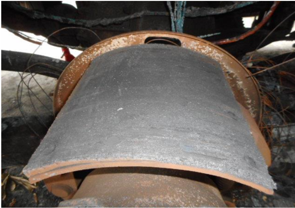
Photo 11 shows a close up view of the rear left top brake drum pad of the Insured Vehicle. Upon closer examination, we did not observed any damages to the brake drum pad.
