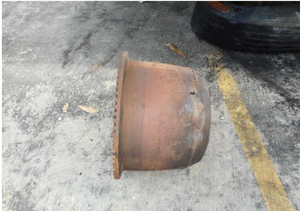
Photo 13 shows a general view of the rear left brake drum of the Insured Vehicle. Upon closer examination, we did not observe any damages to the exterior surface of the brake drum.
