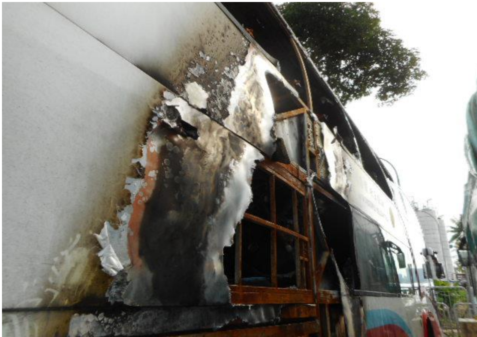
Photo 8 shows a closer view of the right rear portion of the Insured Vehicle at the time of our inspection. The fire damage was observed to be at its rear right portion. The rear right body panel was observed to be affected by the fire.
