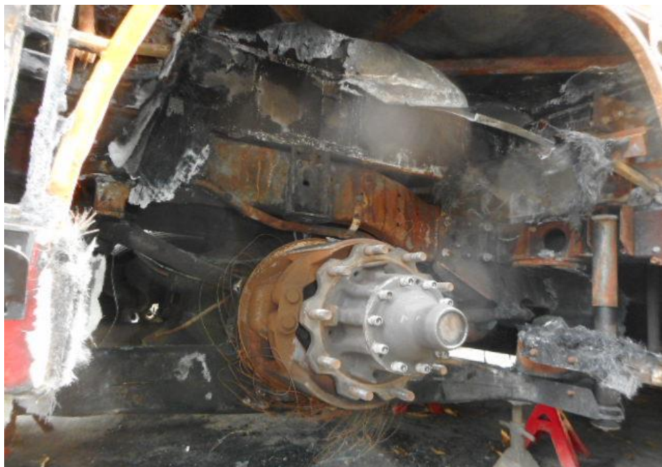
Photo 10 shows a general view of the rear right brake drum and brake pad of the Insured Vehicle after the wheel rim was removed. Upon closer examination, we did not observe any damages to the brake drum or the brake pad.
