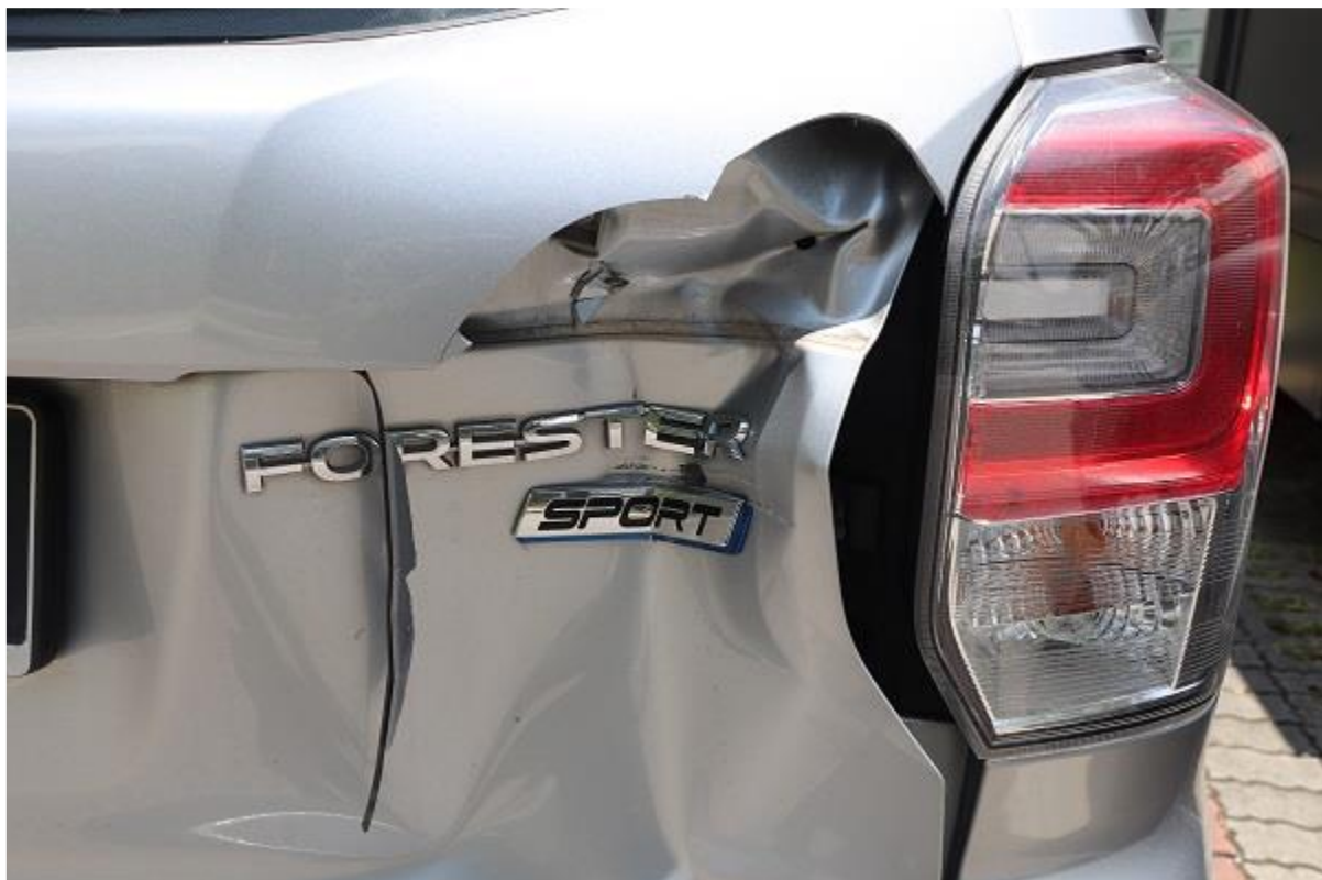
Figure 2K: View of Damaged Tailgate of SMG 7710Y
