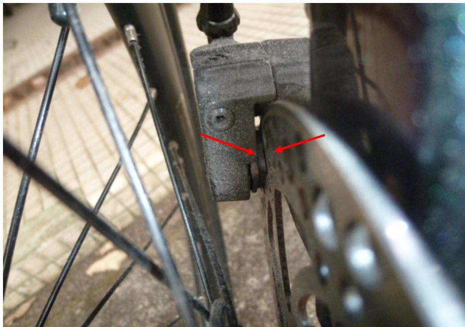
Photo 19 shows a close up view of the front brake pads responding to the gripping action. The front brake pads pressed against the front brake disc (arrowed) upon depressing the right hand brake lever. This had appeared to indicate that the front brake of the Bicycle was in serviceable condition.
