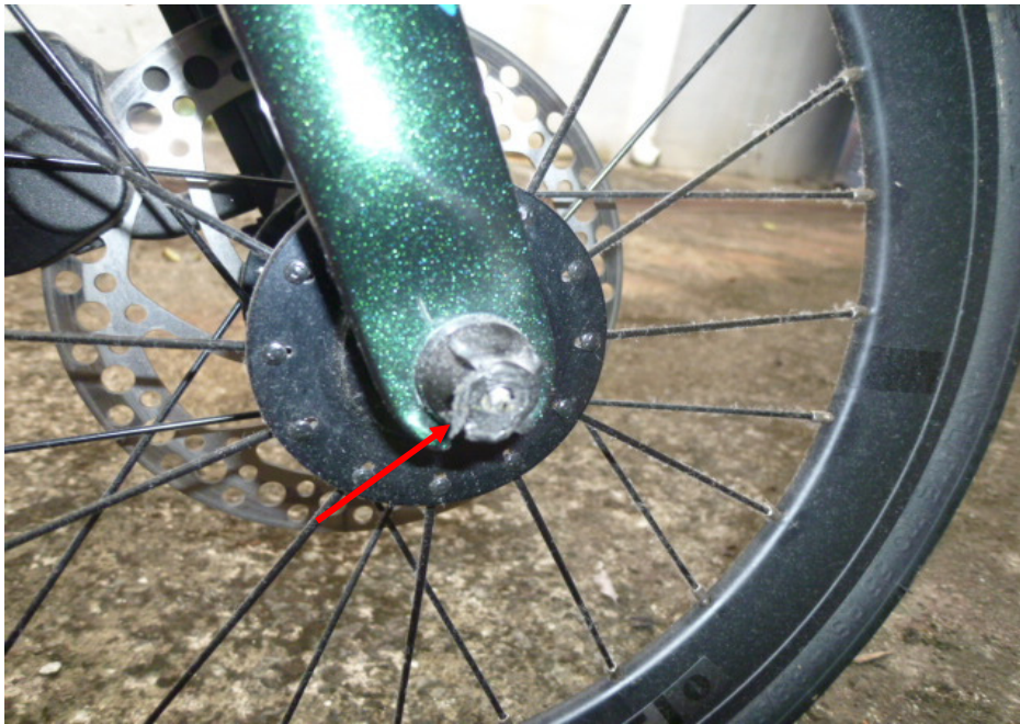
Photo 7 shows the grazed front wheel axle nut (arrowed) of the Bicycle as a result of the accident.
