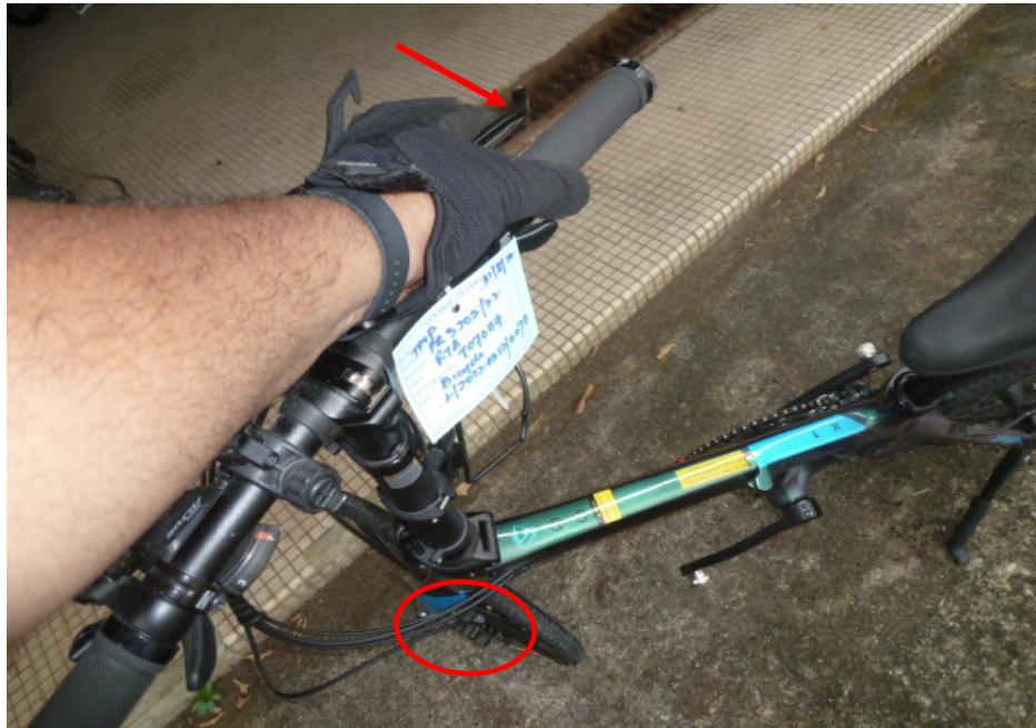
Photo 18 shows a static brake test conducted on the Bicycle's front brake. There was some resistance felt upon pressing the right hand brake lever (arrowed). It also shows that the front brake pads responded to the gripping action (circled) after depressing the right hand brake lever.
