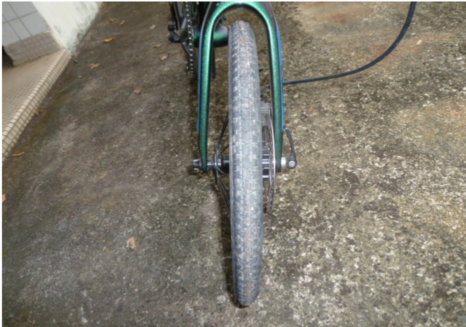
Photo 11 shows the front tyre of the Bicycle. The pattern of the tread was clearly visible. There was no tear, burst mark(s) and/or punctured hole(s) on the sidewalls as well as across the tread of the front tyre. The front tyre was also observed to be sufficiently inflated for vehicular operation.
