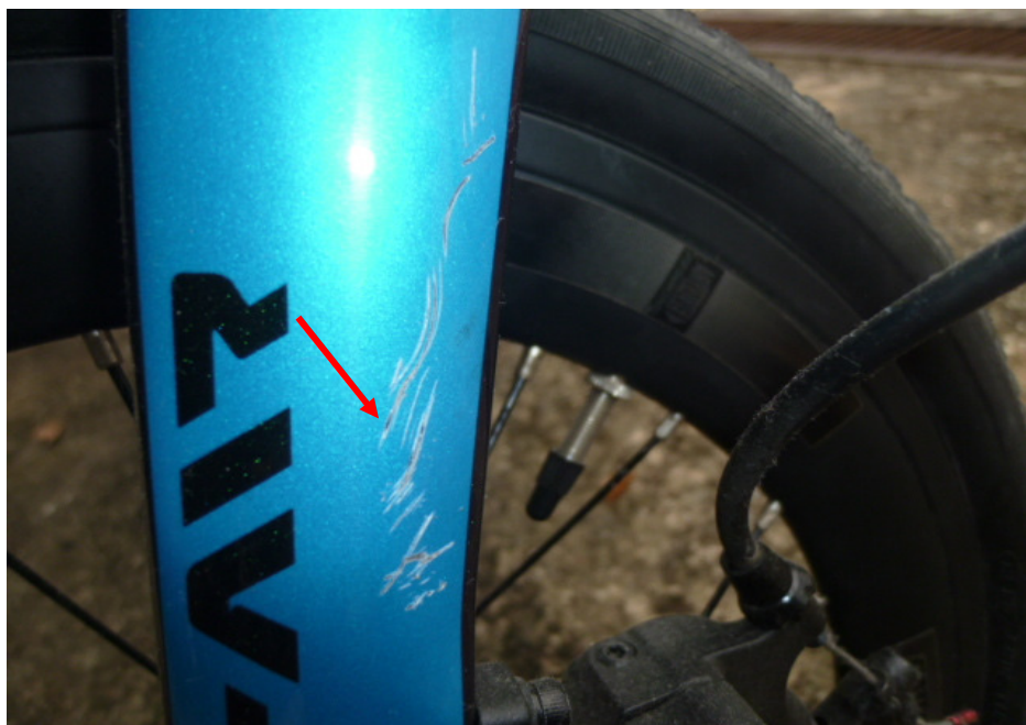
Photo 10 shows a close-up view of the grazed left front fork of the Bicycle as a result of the accident (arrowed).
