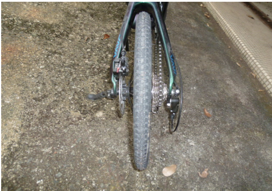
Photo 12 shows the rear tyre of the Bicycle. The pattern of the tread was clearly visible. There was no tear, burst mark(s) and/or punctured hole(s) on the sidewalls as well as across the tread of the rear tyre. The rear tyre was also observed to be sufficiently inflated for vehicular operation.
