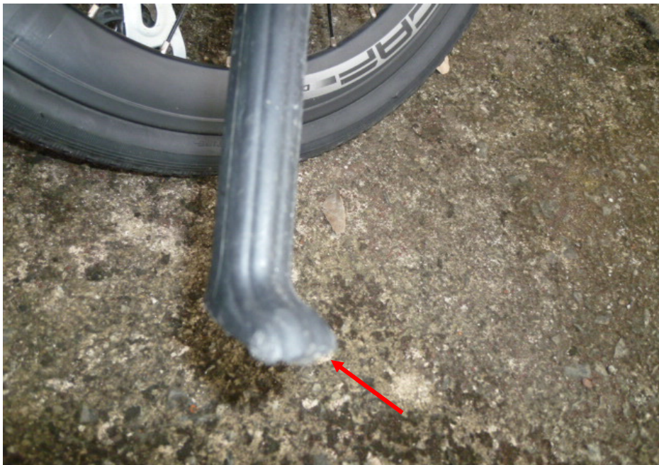
Photo 8 shows the grazed side stand of the Bicycle at the time of our inspection (arrowed).
