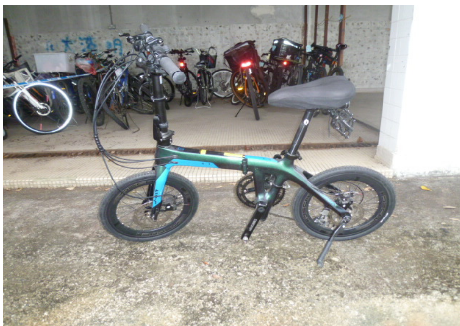
Photo 4 shows the left body of the Bicycle at the time of our inspection. The Bicycle had sustained damages all around. The body parts that were found to have been damaged include its left hand brake lever, right hand brake lever, handlebar grips, left front fork, front wheel axle nut and side stand, amongst others as a result of the accident.
