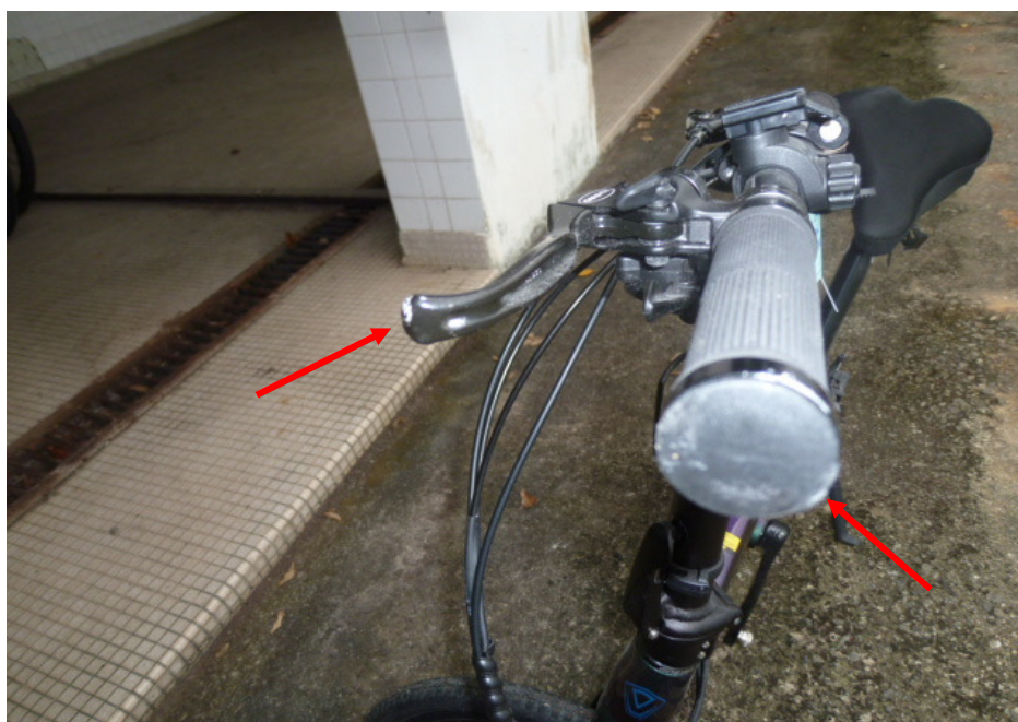
Photo 6 shows the damages of grazing nature on the left hand brake lever and left handlebar grip of the Bicycle at the time of our inspection (arrowed).
