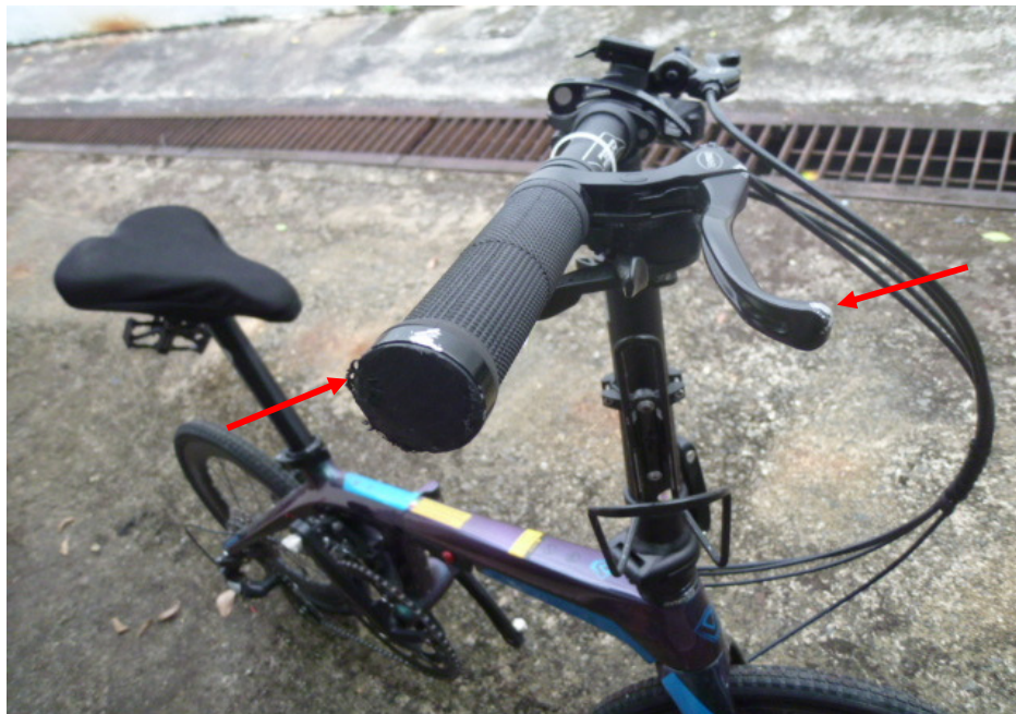
Photo 9 shows the damages of grazing nature on the right hand brake lever and right handlebar grip of the Bicycle at the time of our inspection (arrowed).
