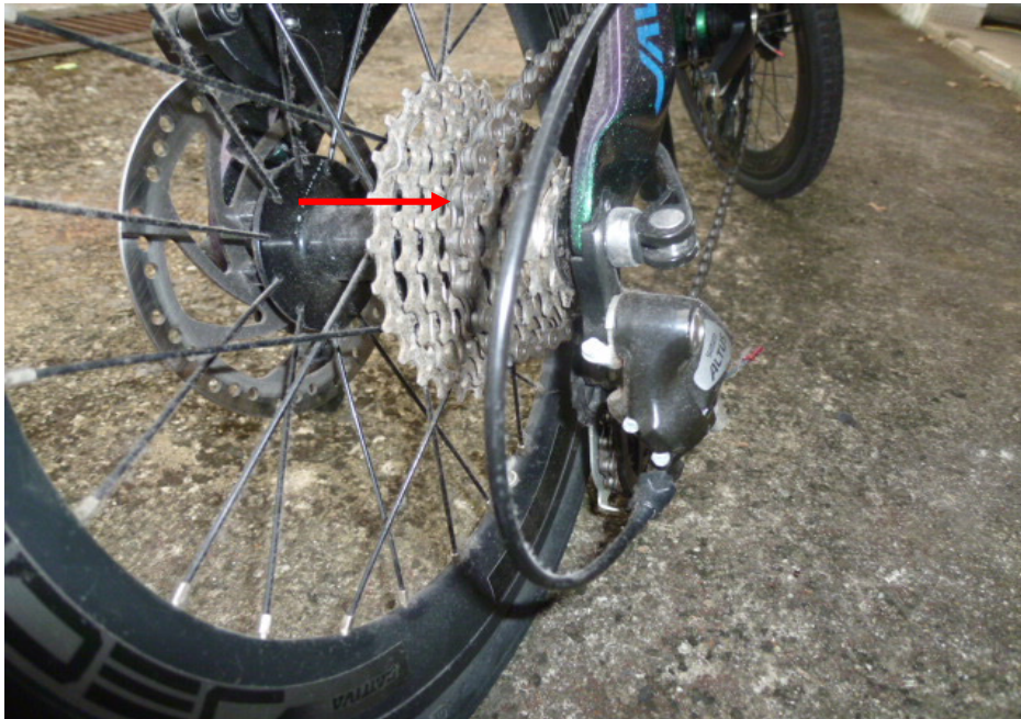
Photo 14 shows a closer view of the gear train of the Bicycle, which was observed to be intact with no misalignment (arrowed). It was also adequately lubricated for operating purposes.
