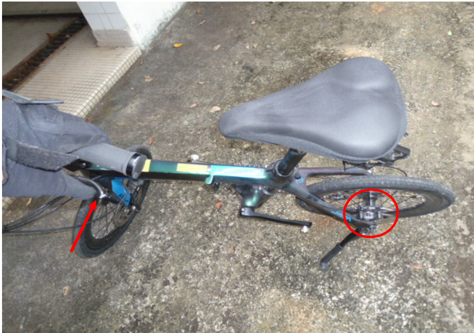
Photo 20 shows a static brake test conducted on the Bicycle's rear brake. There was some resistance felt upon pressing the left hand brake lever (arrowed). It also shows that the rear brake pads responded to the gripping action (circled) after depressing the left hand brake lever.
