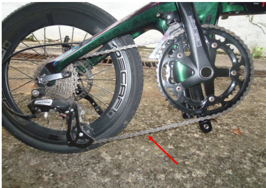
Photo 13 shows the general view of the gear train of the Bicycle, which was observed to be intact with no misalignment (arrowed). It was also adequately lubricated for operating purposes.
