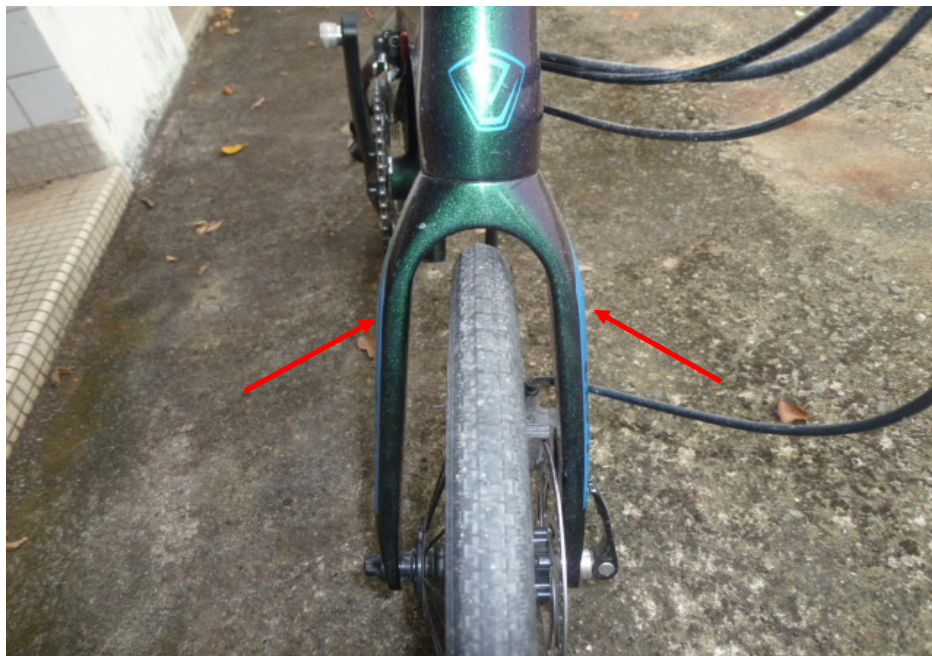
Photo 15 shows the front fork assembly (arrowed) of the Bicycle. The front forks and fork bracket of the Bicycle were both found to be intact and undamaged. Turning the Bicycle's handle bar towards the left and right did not produce any abnormal free play. The steering system of the Bicycle was in serviceable condition at the time of our inspection.
