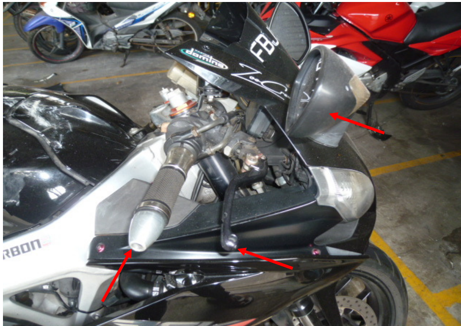
Photo 10 shows a closer view of the front brake lever, right side mirror and right handlebar end (arrowed) which were amongst the body parts at the front body of the Motorcycle that had sustained damage as a result of the accident.
