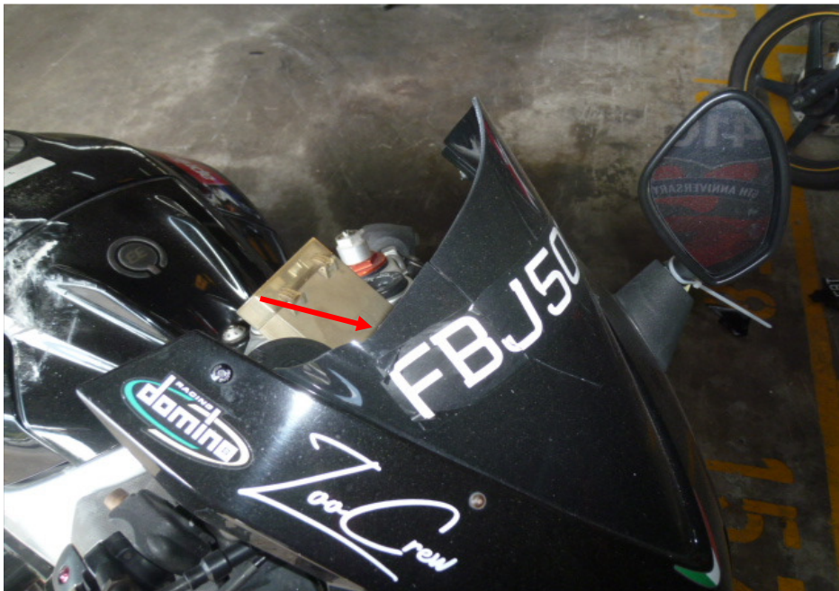
Photo 5 shows a closer view of the cracked windshield (arrowed) of the Motorcycle as a result of the accident.
