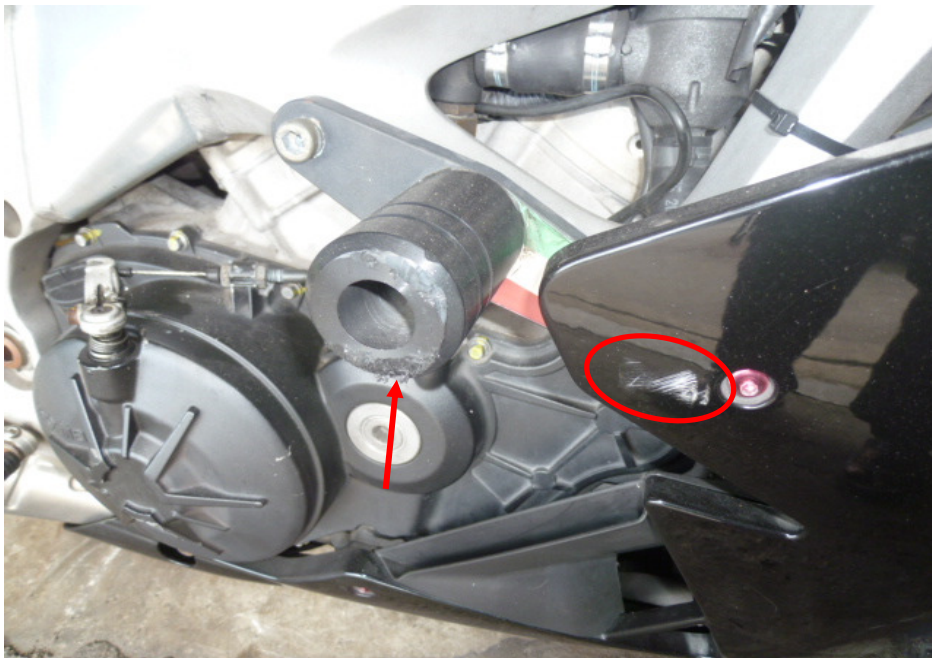
Photo 9 shows the grazed left frame slider (arrowed) and right cowling (circled) of the Motorcycle as a result of the accident
