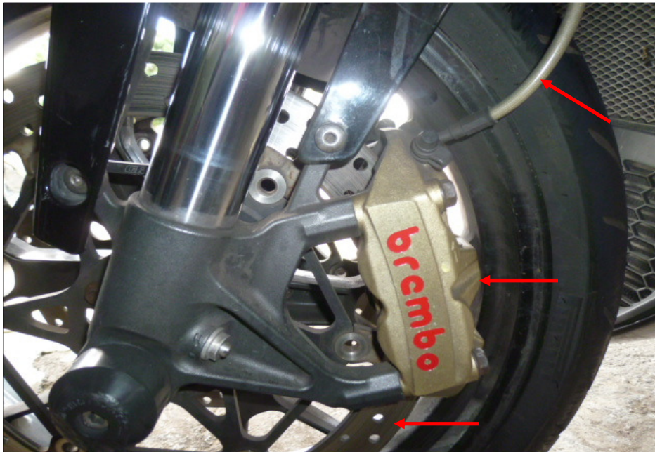
Photo 25 shows a close up view of the front brake caliper, front brake disc and front brake hose (arrowed) at the left side of the Motorcycle's front wheel, which are all part of the components in the hydraulic front brake system of the Motorcycle. Our visual checks of these various components had revealed all to be intact with no visible damage. No leakage of brake fluid was also observed.
