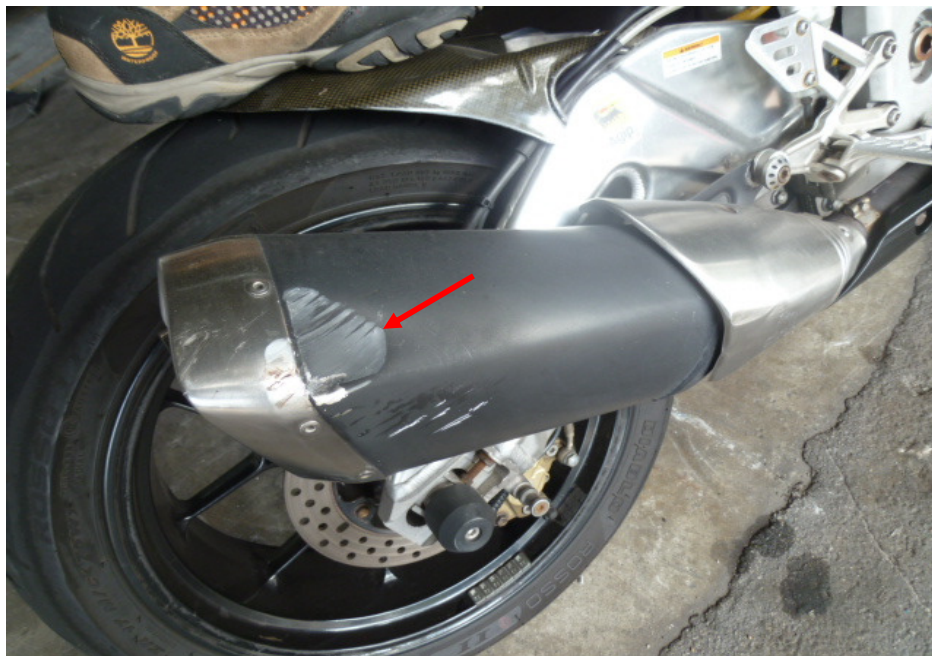
Photo 13 shows the dented exhaust muffler (arrowed) of the Motorcycle as a result of the accident.
