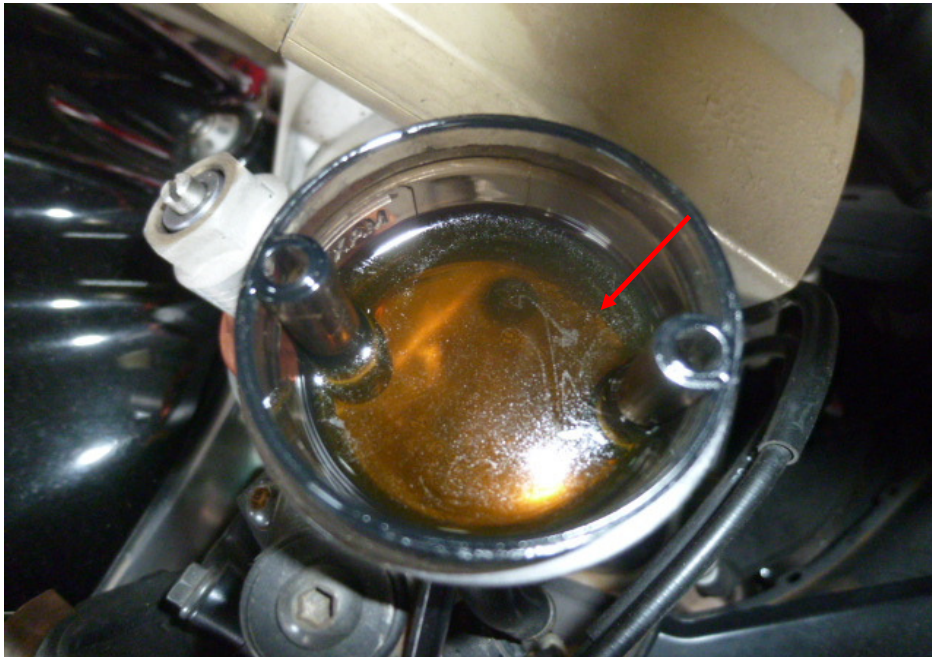
Photo 26 shows the brake fluid reservoir for the front brake of the Motorcycle. The brake fluid was observed to be of sufficient level for operational purposes. However it was found to be slightly contaminated (arrowed).
