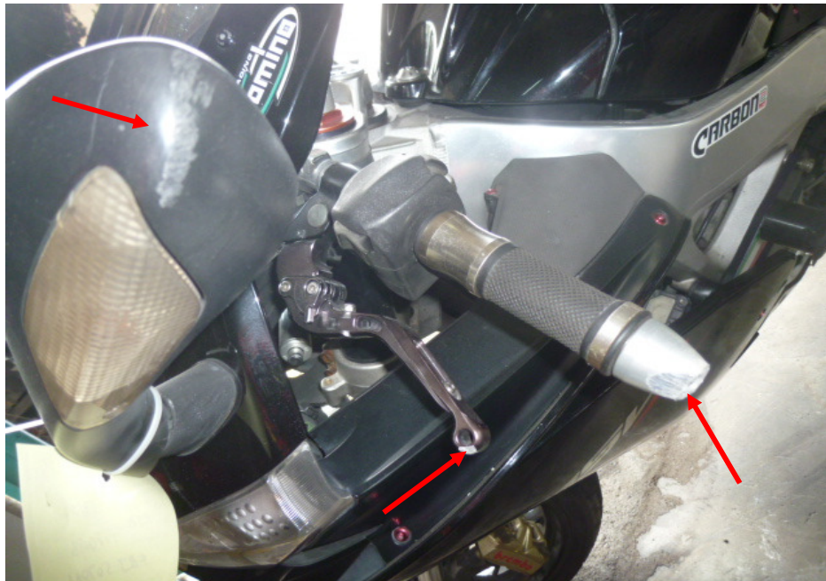
Photo 7 shows a closer view of the clutch lever, left side mirror and left handlebar end (arrowed) which were amongst the body parts at the front body of the Motorcycle that had sustained damage as a result of the accident.
