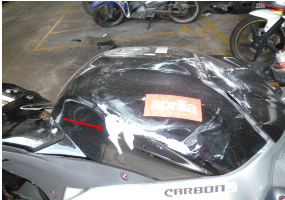
Photo 6 shows a closer view of the petrol tank which was amongst the body parts at the front body of the Motorcycle that had sustained damage as a result of the accident (arrowed).
