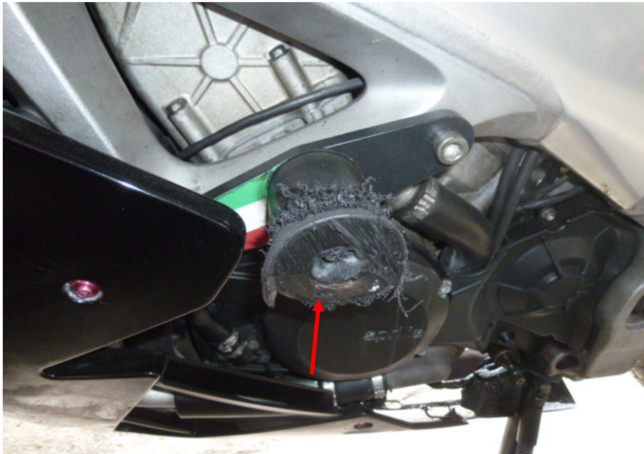
Photo 8 shows the grazed left frame slider of the Motorcycle as a result of the accident (arrowed).
