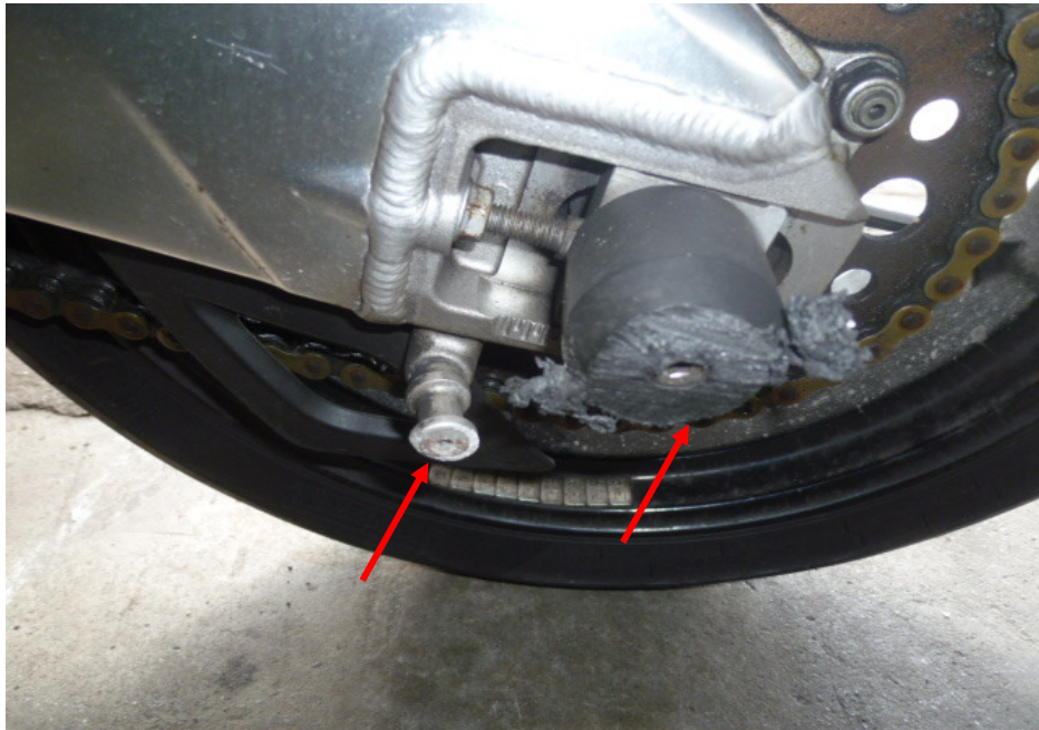
Photo 12 shows a closer view of the grazed left swingarm spool and slider (arrowed) which were amongst the body parts of the Motorcycle that had sustained damage as a result of the accident.
