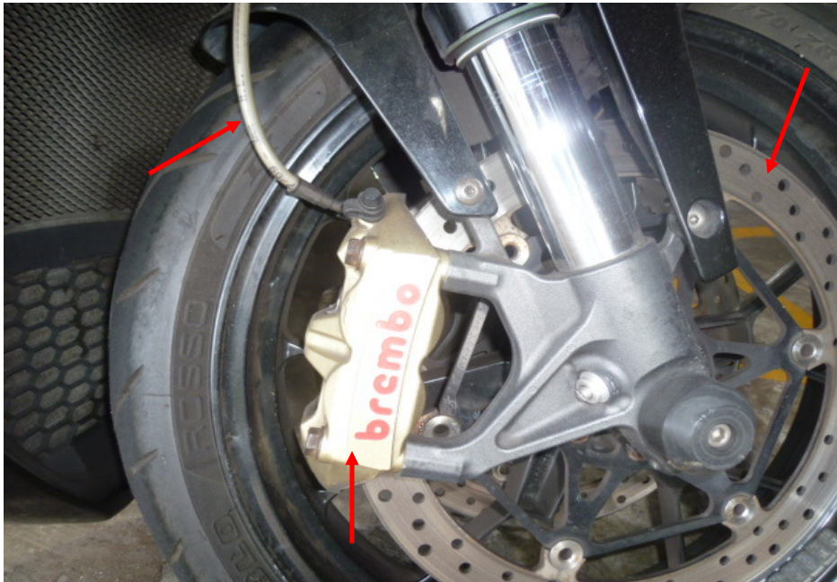
Photo 24 shows a close up view of the front brake caliper, front brake disc and front brake hose (arrowed) at the right side of the Motorcycle's front wheel, which are all part of the components in the hydraulic front brake system of the Motorcycle. Our visual checks of these various components had revealed all to be intact with no visible damage. No leakage of brake fluid was also observed.
