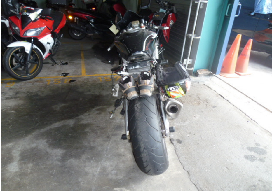
Photo 4 shows a general view of the rear portion of the Motorcycle at the time of our inspection. The Motorcycle was observed to have sustained damages all around. The body parts that were found to have been damaged include its windshield, petrol tank, handlebar ends, side mirrors, front brake lever, clutch lever, frame sliders, gear shift pedal and exhaust muffler, amongst others.
