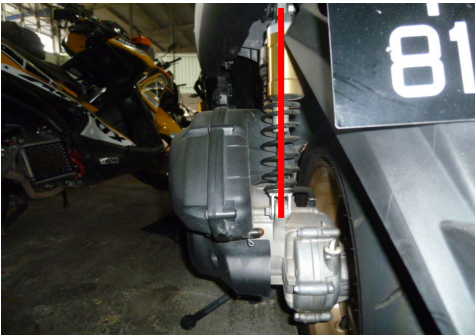
Photo 21 shows the left shock absorber of the Motorcycle which was found to be intact without any misalignment.
