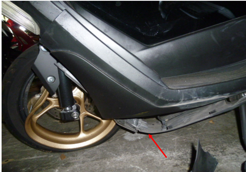
Photo 11 shows a closer view of the deformed left bottom cowling of the Motorcycle as a result of the accident (arrowed).
