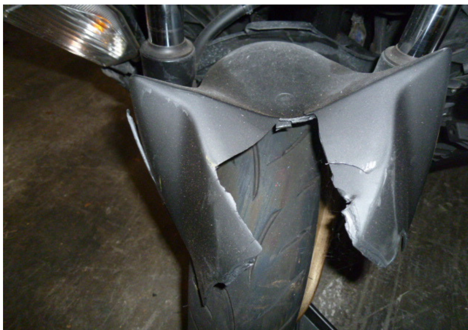
Photo 6 shows a closer view of the cracked front mudguard of the Motorcycle as a result of the accident.
