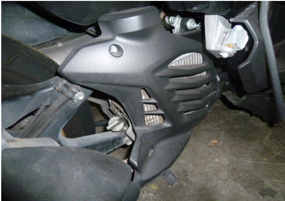
Photo 18 shows the radiator of the Motorcycle at the time of our inspection. The radiator was found to be intact with no visible damage. There was also no sign(s) or indication(s) of fluid leak observed around the radiator of the Motorcycle.
