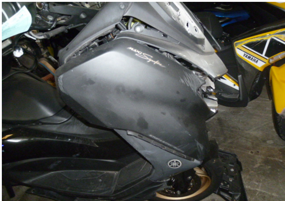
Photo 8 shows a closer view of the right cowling of the Motorcycle that had sustained damage as a result of the accident.
