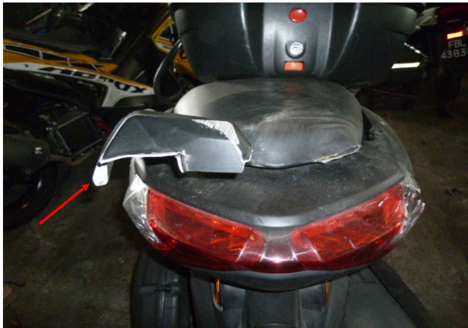
Photo 12 shows the broken left pillion grab rail of the Motorcycle as a result of the accident (arrowed).
