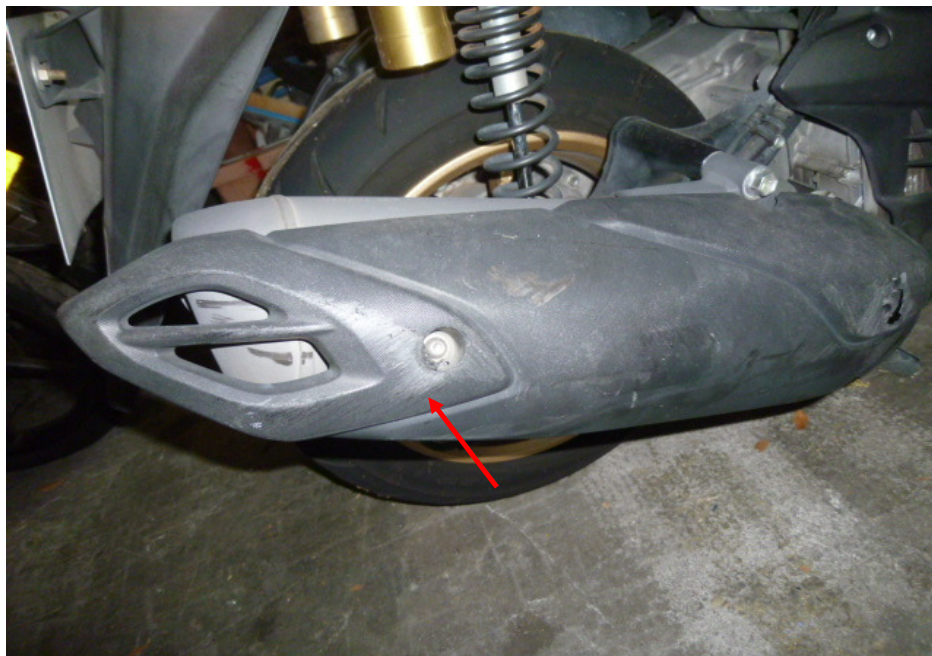
Photo 14 shows a closer view of the grazed exhaust muffler heat shield of the Motorcycle at the time of our inspection.
