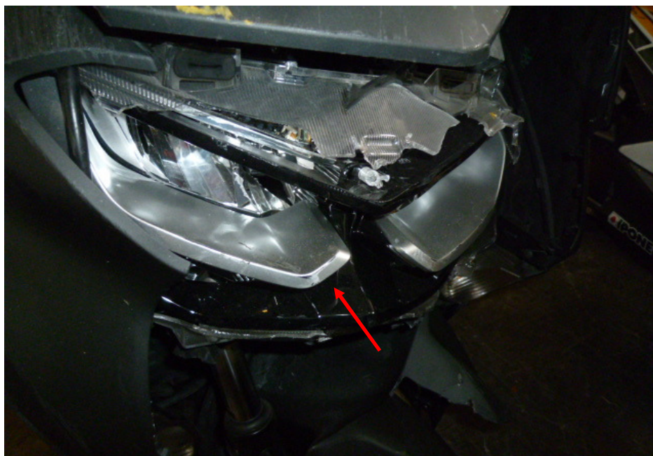
Photo 5 shows a closer view of the cracked headlight (arrowed) which was amongst the body parts at the front body of the Motorcycle that had sustained damage as a result of the accident.
