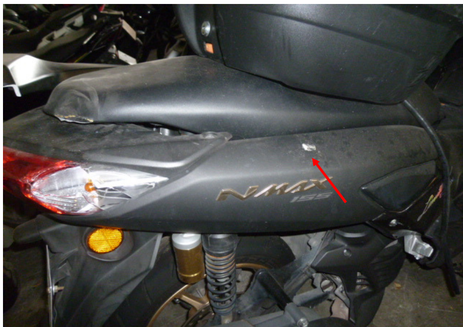
Photo 10 shows a closer view of grazed right rear side cover (arrowed) of the Motorcycle at the time of our inspection.
