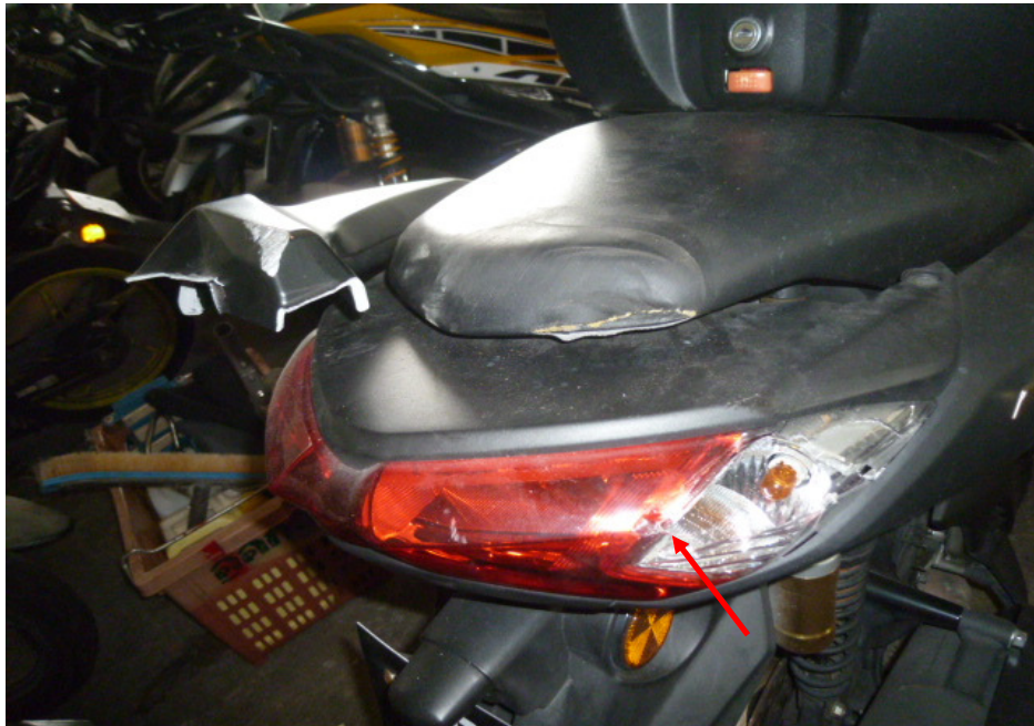
Photo 13 shows a closer view of the cracked tail light of the Motorcycle as a result of the accident (arrowed).
