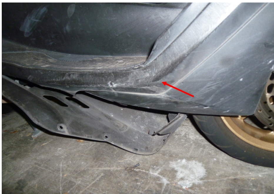
Photo 9 shows a closer view of the grazed right bottom cowling of the Motorcycle as a result of the accident (arrowed).
