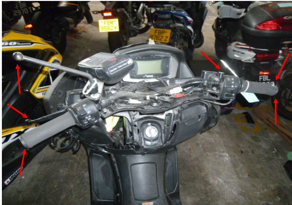
Photo 7 shows a closer view of the handlebar, hand brake levers, side mirrors and handlebar ends of the Motorcycle which were observed to be damaged due to the accident (arrowed).
