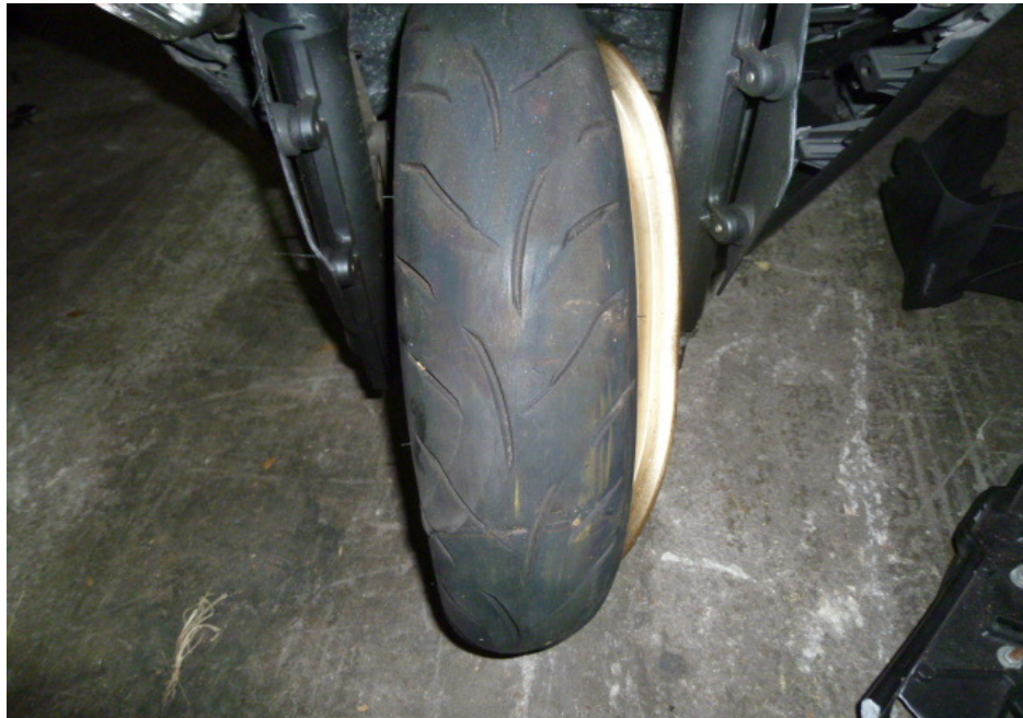
Photo 15 shows the condition of the Motorcycle's front tyre. The front tyre was observed to be in serviceable condition with remaining tread depth of approximately 4mm. There was no tear, burst mark(s) and/or punctured hole(s) on the sidewalls as well as across the tread of the front tyre. However the front tyre was observed to be deflated.
