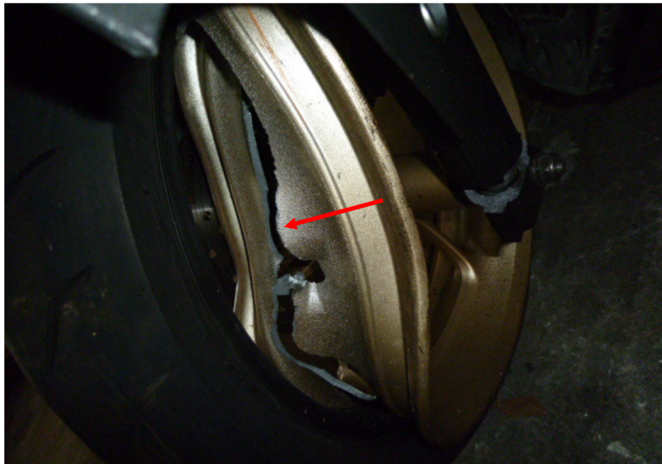
Photo 16 shows the broken front wheel rim and deflated front tyre (arrowed) of the Motorcycle at the time of our inspection.
