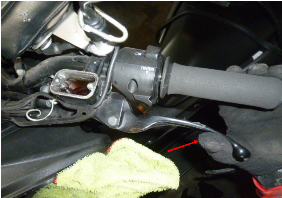
Photo 28 shows the rear brake lever being depressed. There was some resistance felt (spongy like feel) upon pressing the front brake lever (arrowed). This would indicate that there is no leakage of pressure/vacuum in the brake system.
