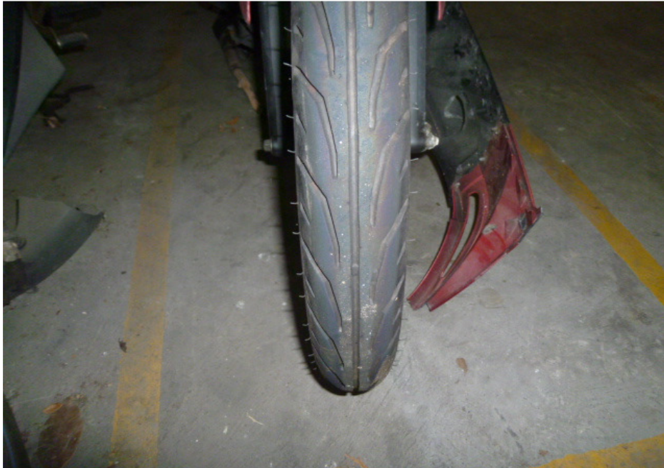
Photo 18 shows the front tyre of the Motorcycle at the time of our inspection. The front tyre was observed to be in serviceable condition with remaining tread depth of approximately 3mm. The pattern of the tread was also clearly visible. There was no tear, burst mark(s) and/or punctured hole(s) on the sidewalls as well as across the tread of the front tyre.
