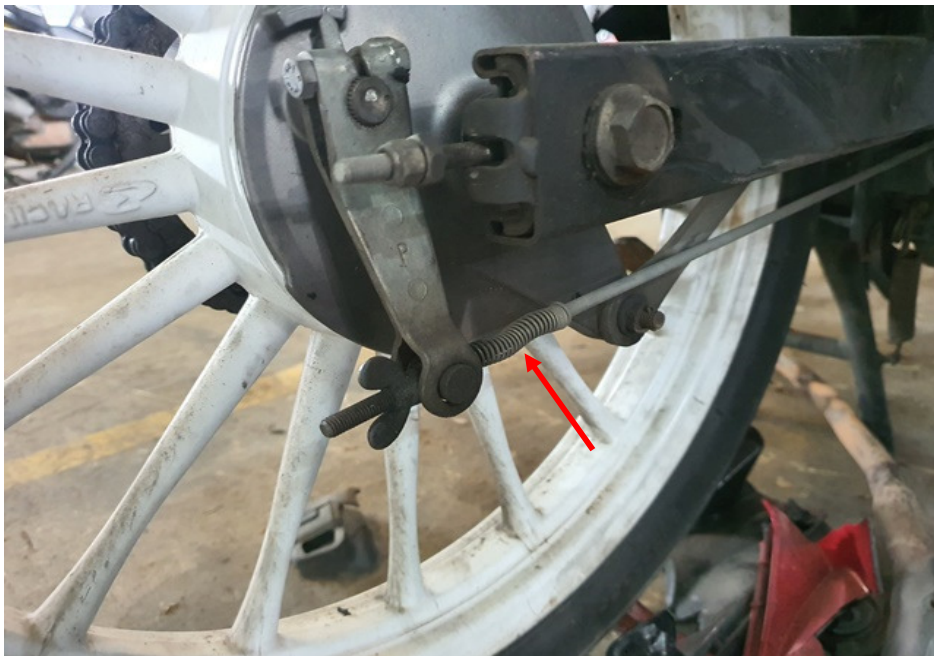
Photo 28 shows the rear wheel of the Motorcycle. The type of brake system for the rear wheel was of a mechanical type, controlled by the brake foot pedal of the Motorcycle. Our checks of the cable (arrowed), spring and drum which are all part of the components in the rear brake system of the Motorcycle reveal all to be intact and without damage.
