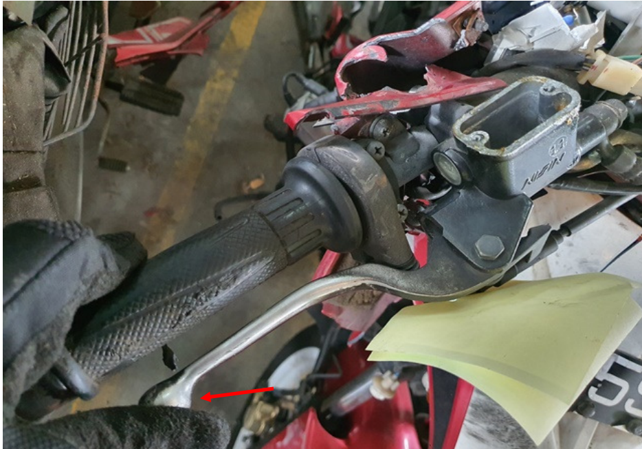
Photo 27 shows the front brake lever being depressed. There was no resistance felt (spongy like feel) upon pressing the front brake lever (arrowed). This would indicate that there may be a leakage of pressure/vacuum in the front brake system.
