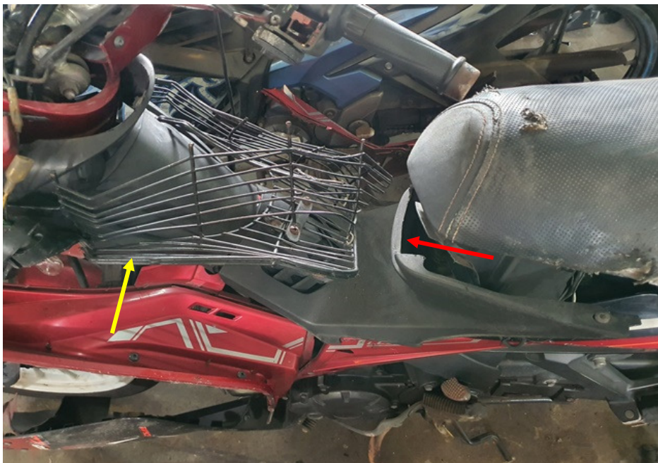
Photo 9 shows a closer view of the front basket and centre inner panel of the Motorcycle (arrowed). These parts were amongst the body parts of the Motorcycle which were damaged as a result of the accident.
