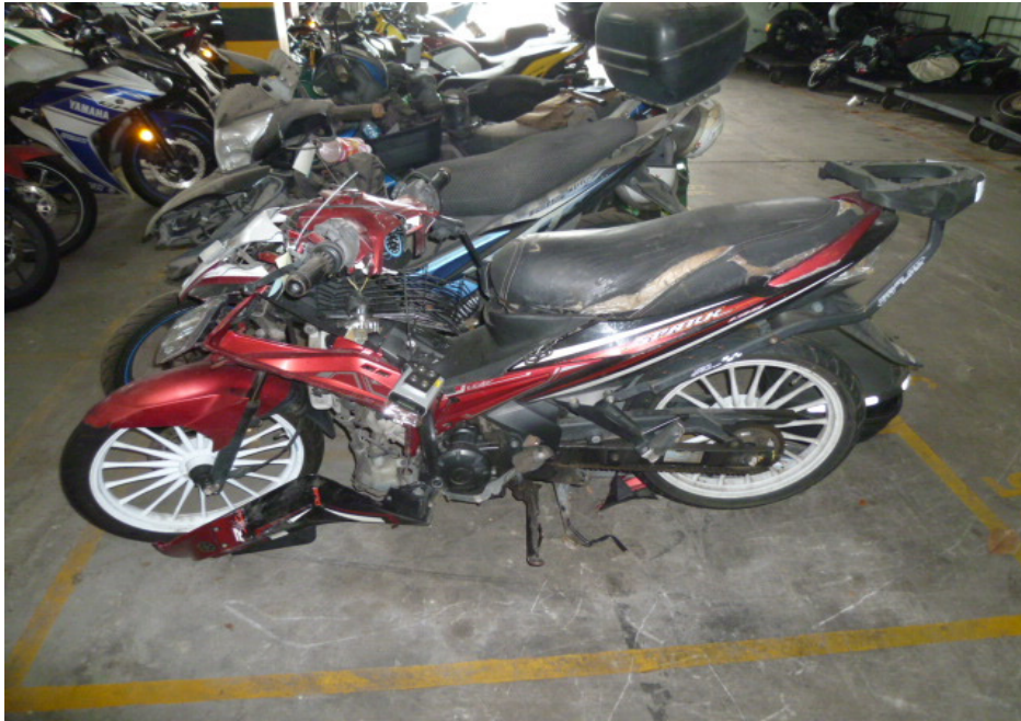
Photo 4 shows a general view of the left body of the Motorcycle at the time of our inspection. The Motorcycle had sustained damages all around. Body parts that were found to have been damaged include its headlight assembly, front cowlings, steering stem, front mudguard, handlebar, side mirrors, side cowlings, front footrests, front basket, rear side covers and exhaust muffler, amongst others.
