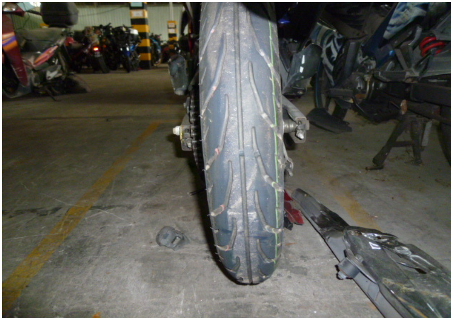
Photo 19 shows the condition of the Motorcycle's rear tyre. The rear tyre was observed to be in serviceable condition with remaining tread depth of approximately 2mm. The tyre was also observed to be sufficiently inflated for vehicular operation. We did not observe any tear, burst mark(s) and/or punctured hole(s) on the sidewalls as well as across the tread of the rear tyre.
