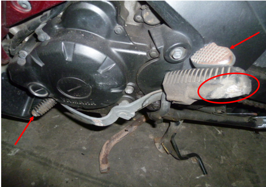
Photo 14 shows a closer view of the gear shift pedal (arrowed) and right front footrest (circled) which were amongst the body parts of the Motorcycle that had sustained damage as a result of the accident.
