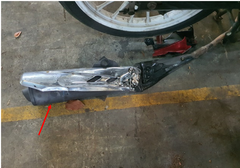
Photo 17 shows a closer view of the dislodged exhaust muffler of the Motorcycle as a result of the accident (arrowed).
