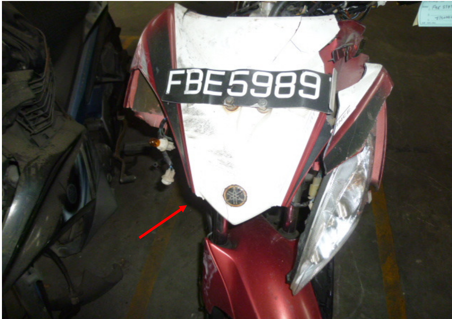
Photo 6 shows the cracked front cowling of the Motorcycle at the time of our inspection (arrowed).
