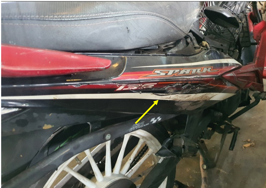
Photo 13 shows a closer view of the cracked right rear side cover which was amongst the body parts of the Motorcycle as a result of the accident (arrowed).
