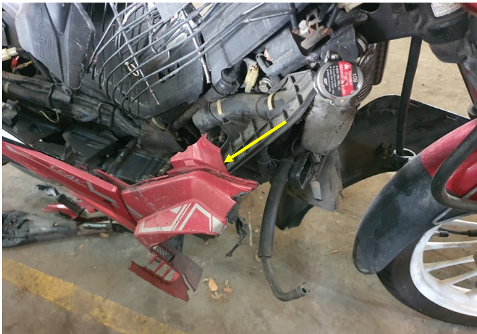
Photo 11 shows a closer view of the cracked right cowling of the Motorcycle as a result of the accident (arrowed).
