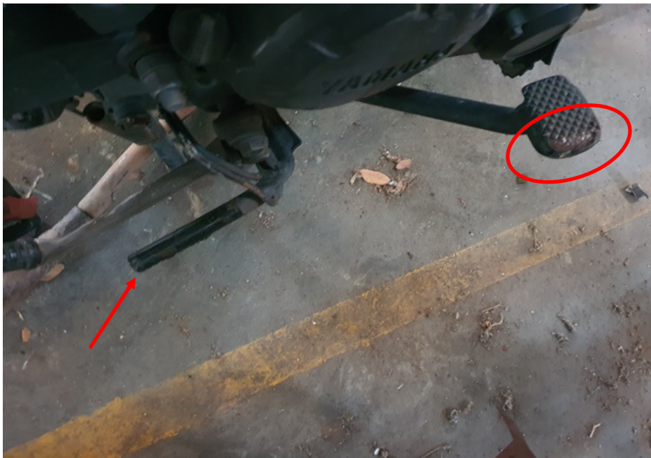
Photo 15 shows a closer view of the rear brake pedal (circled) and right front footrest (arrowed) which were amongst the body parts of the Motorcycle that had sustained damage as a result of the accident.
