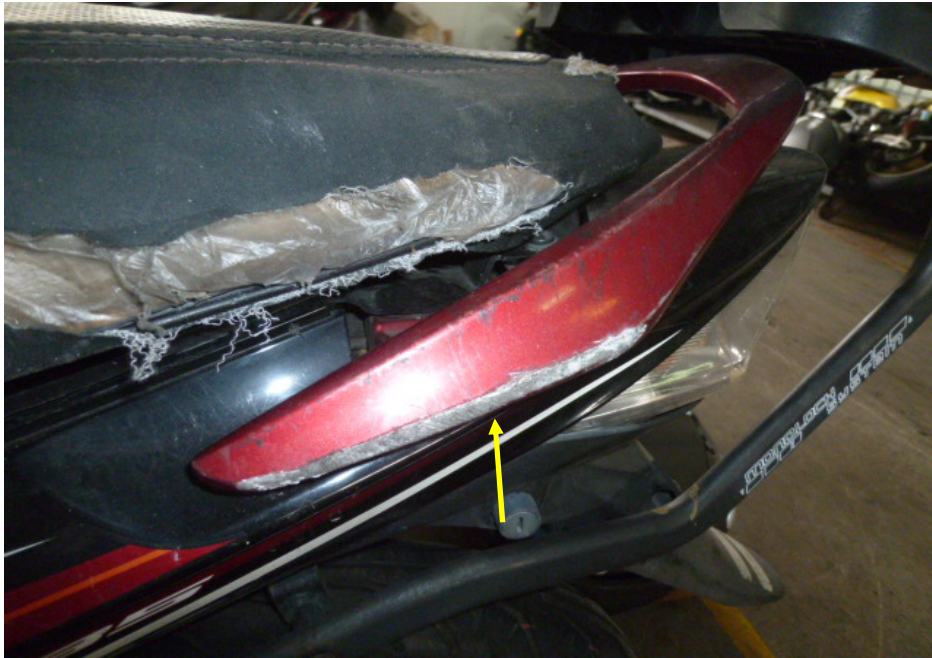
Photo 16 shows a closer view of the left pillion grab rail which was amongst the body parts of the Motorcycle that had sustained damages of grazing nature as a result of the accident (arrowed).
