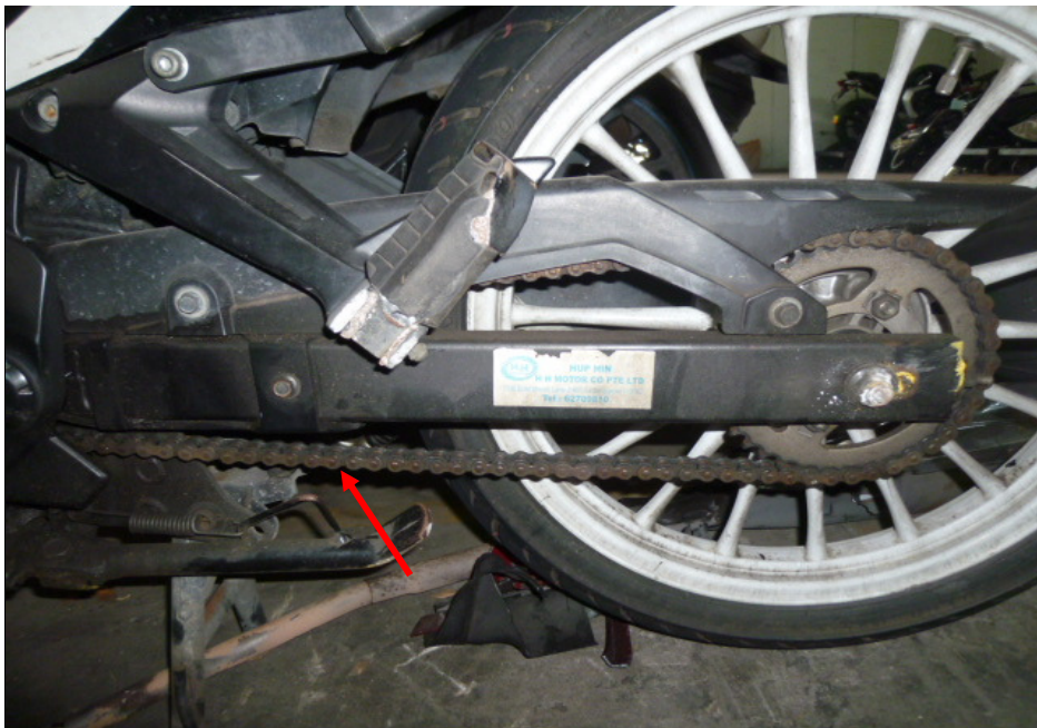
Photo 22 shows the gear train (arrowed) of the Motorcycle, which was observed to be intact with no misalignment. It was also adequately lubricated for operating purposes. The gear train rotates the rear wheel of the Motorcycle.
