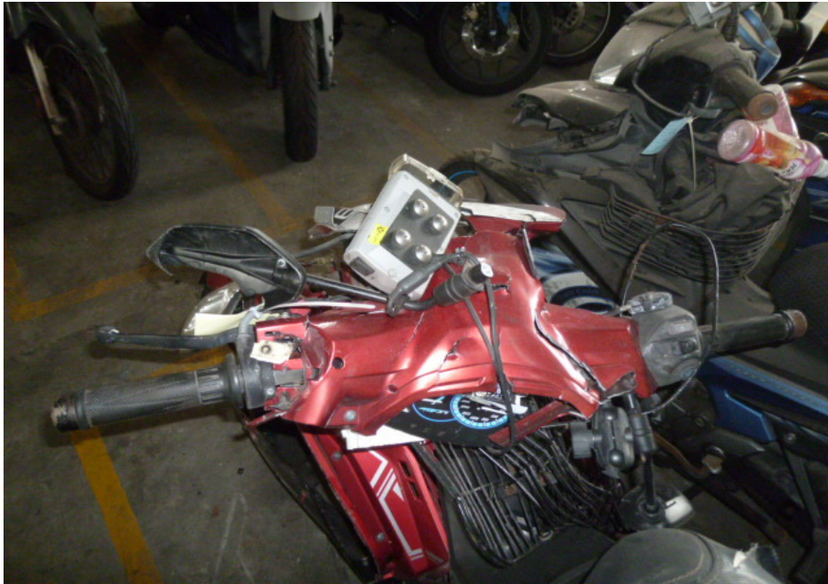
Photo 8 shows a closer view of the handlebar, handlebar ends, side mirrors, clutch lever and front brake lever which were amongst the body parts of the Motorcycle that had sustained damage as a result of the accident.
