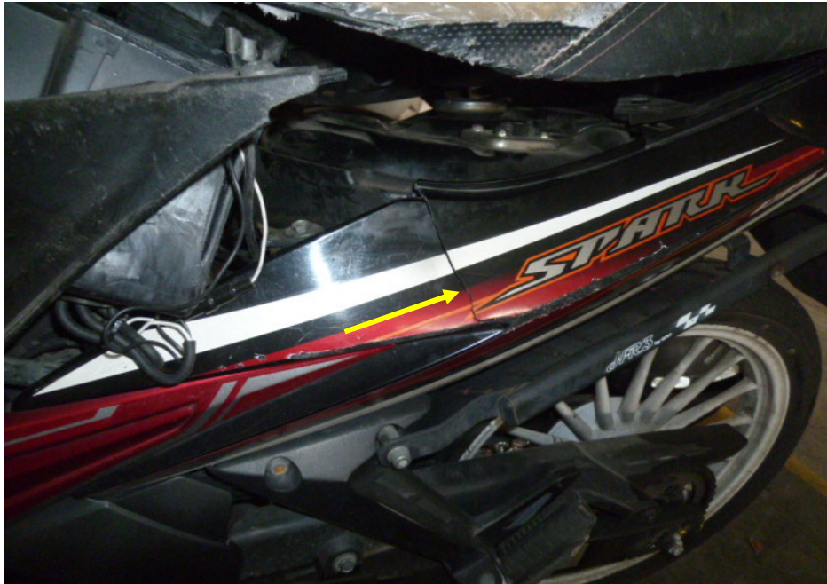
Photo 12 shows a closer view of the cracked left rear side cover which was amongst the body parts of the Motorcycle as a result of the accident (arrowed).
