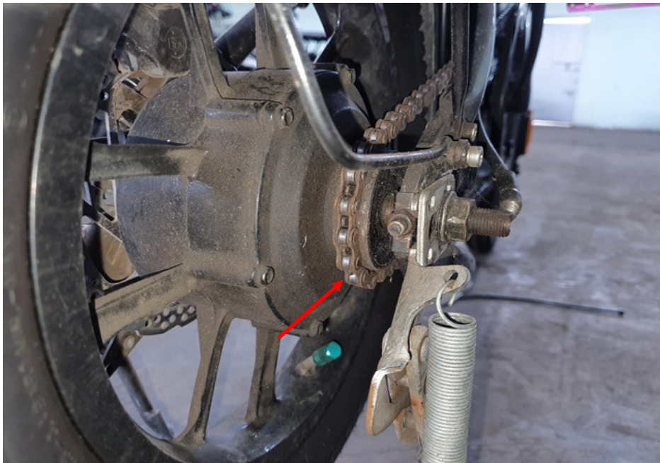
Photo 15 shows a closer view of the gear train of the PAB, which was observed to be intact with no misalignment (arrowed). It was also adequately lubricated for operating purposes.
