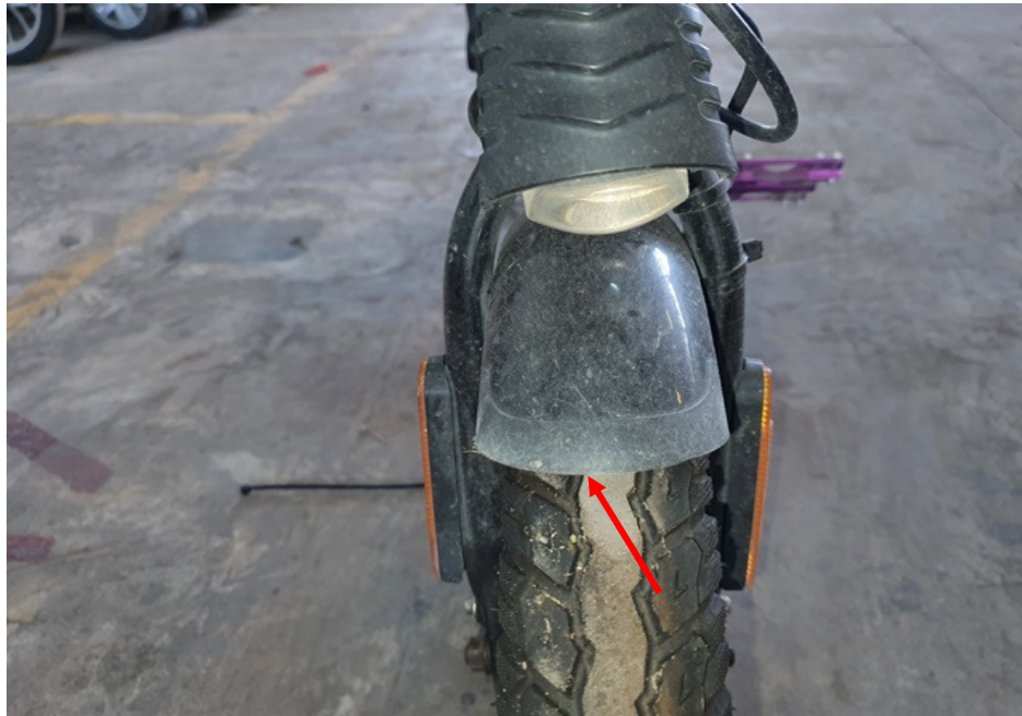
Photo 7 shows the grazed front mudguard (arrowed) of the PAB as a result of the accident.
