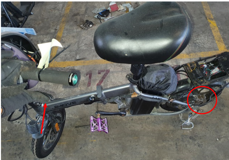
Photo 21 shows a static brake test conducted on the PAB's rear brake. There was some resistance felt upon pressing the left hand brake lever (arrowed). It also shows that the rear brake pads responded to the gripping action (circled) after depressing the left hand brake lever.
