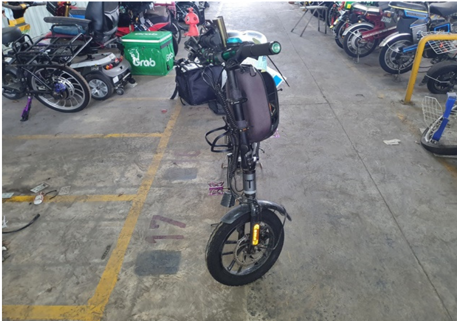
Photo 17 shows the front wheel of the PAB turned towards its full right. Turning the PAB's handle bar towards the right did not produce any abnormal free play and/or resistance. This would indicate that the steering system of the PAB was in serviceable condition at the time of our inspection.
