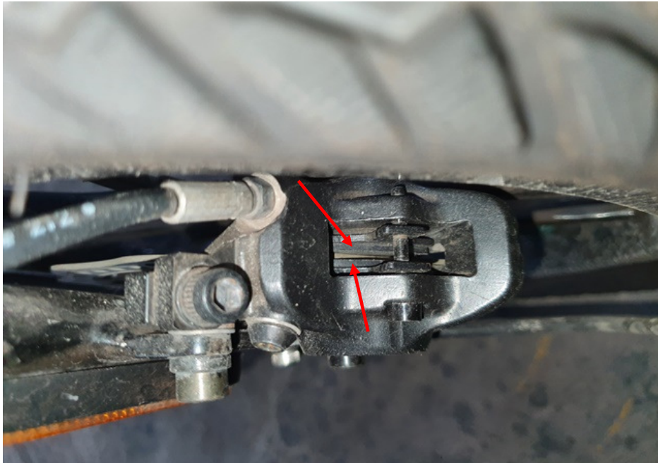
Photo 20 shows a close up view of the front brake pads responding to the gripping action. The front brake pads pressed against the front brake disc (arrowed) upon depressing the right hand brake lever. This had appeared to indicate that the front brake of the PAB was in serviceable condition.
