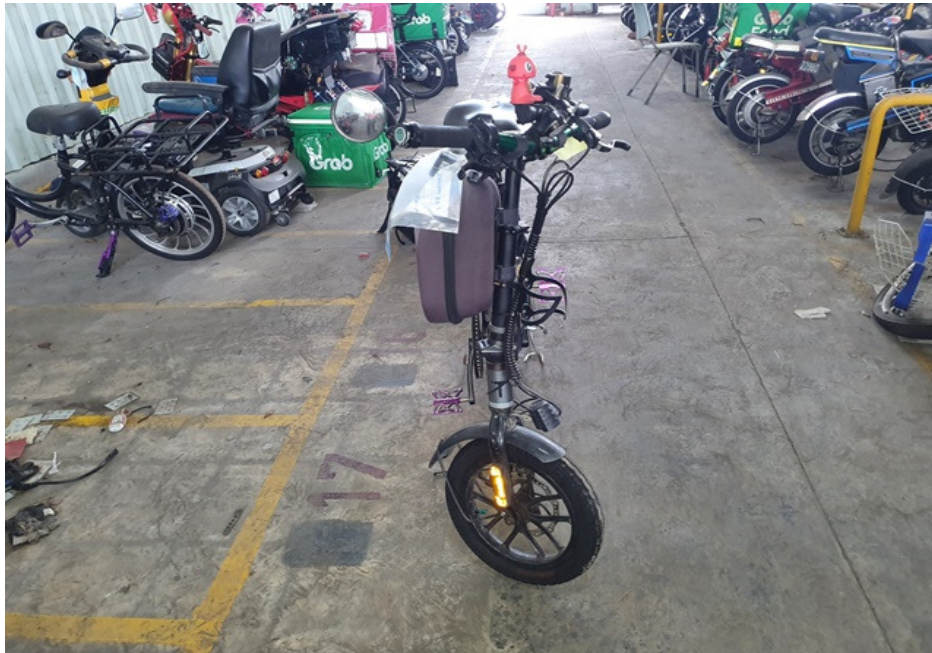
Photo 18 shows the front wheel of the PAB turned towards its full left. Turning the PAB's handle bar towards the left did not produce any abnormal free play and/or resistance. This would indicate that the steering system of the PAB was in serviceable condition at the time of our inspection.
