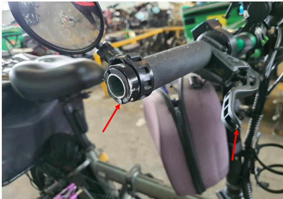
Photo 8 shows the damages on the right hand brake lever and right handlebar end (arrowed) of the PAB as a result of the accident.
