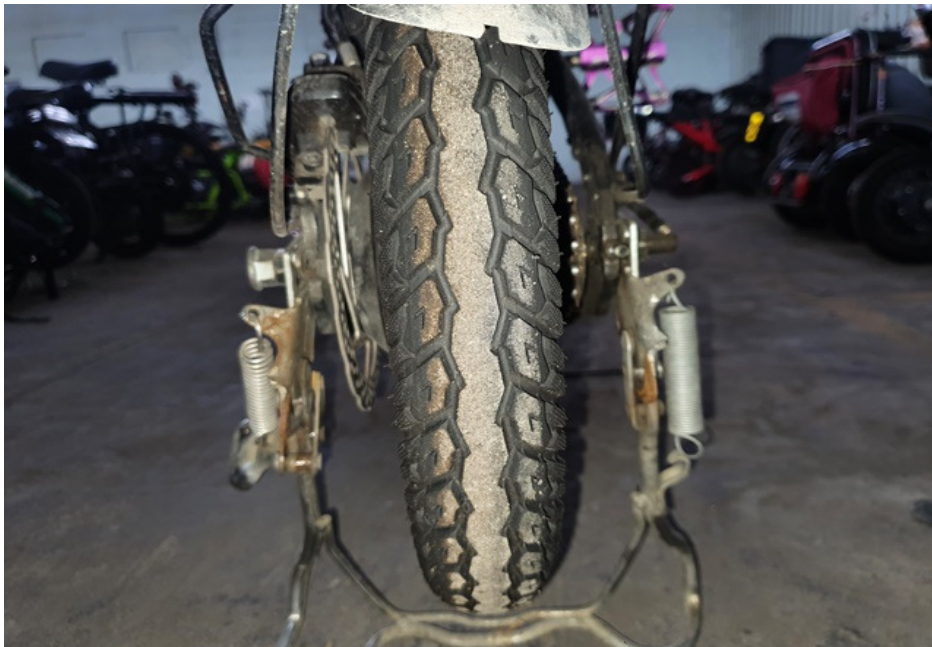
Photo 12 shows the rear tyre of the PAB at the time of our inspection. The rear tyre was observed to be in serviceable condition with remaining tread depth of approximately 2mm. The tyre was also observed to be sufficiently inflated for vehicular operation. We did not observe any tear, burst mark(s) and/or punctured hole(s) on the sidewalls as well as across the tread of the rear tyre.
