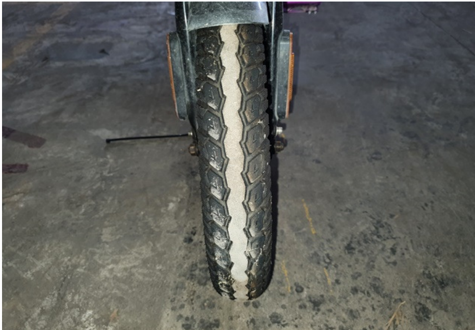
Photo 11 shows the front tyre of the PAB at the time of our inspection. The front tyre was observed to be in serviceable condition with remaining tread depth of approximately 3mm. The tyre was also observed to be sufficiently inflated for vehicular operation. We did not observe any tear, burst mark(s) and/or punctured hole(s) on the sidewalls as well as across the tread of the front tyre.
