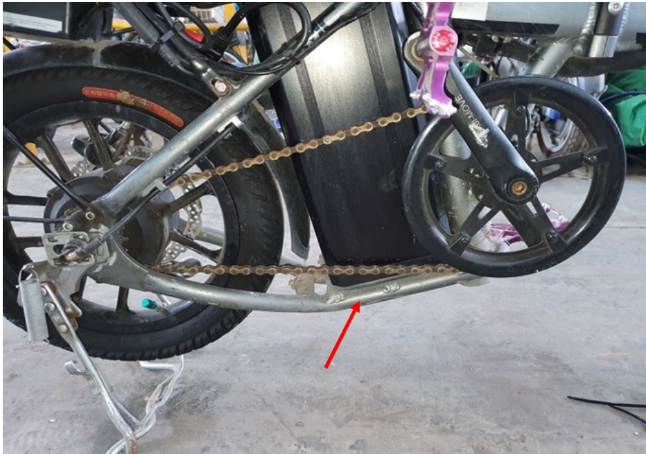
Photo 14 shows the general view of the gear train of the PAB, which was observed to be intact with no misalignment (arrowed). It was also adequately lubricated for operating purposes.
