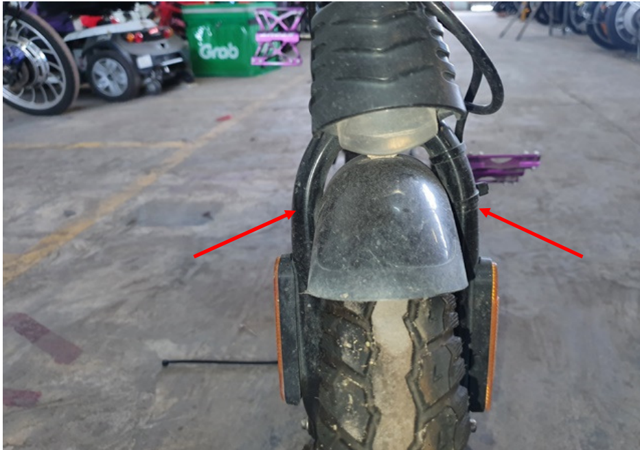
Photo 16 shows the front fork assembly (arrowed) of the PAB. The front forks and fork bracket of the PAB were both found to be intact and undamaged. Turning the PAB's handle bar towards the left and right did not produce any abnormal free play. The steering system of the PAB was in serviceable condition at the time of our inspection.
