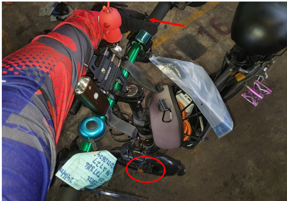
Photo 19 shows a static brake test conducted on the PAB's front brake. There was some resistance felt upon pressing the right hand brake lever (arrowed). It also shows that the front brake pads responded to the gripping action (circled) after depressing the right hand brake lever.
