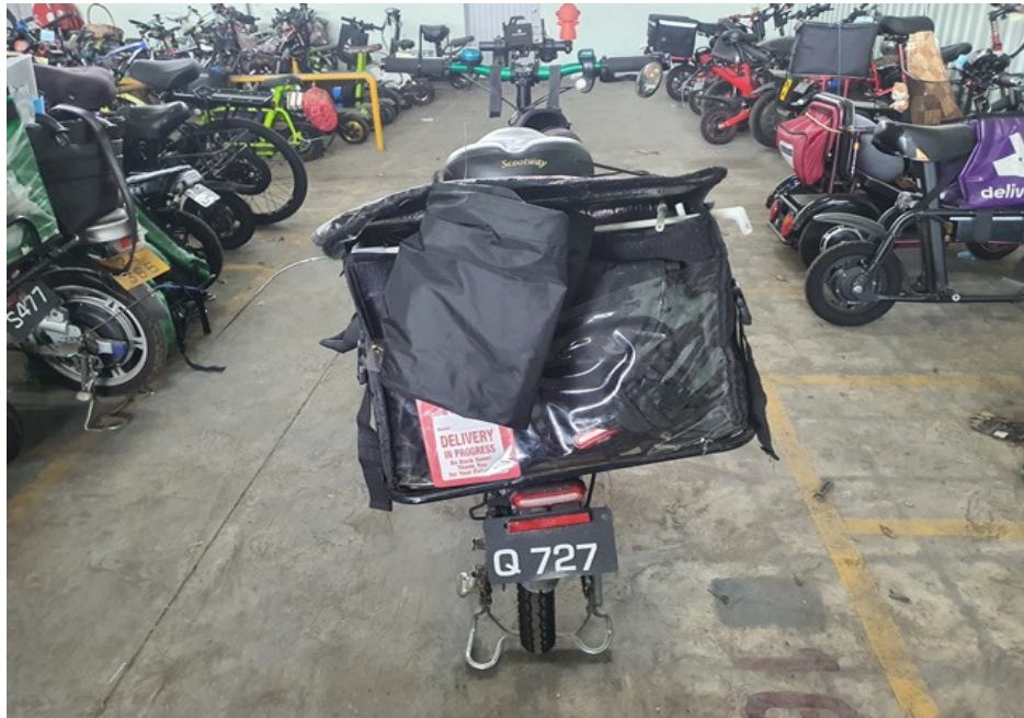
Photo 5 shows the rear portion of the PAB at the time of our inspection. The body parts that were found to have been damaged include its front mudguard, right hand brake lever, right handlebar end, right pedal and seat, amongst others as a result of the accident.
